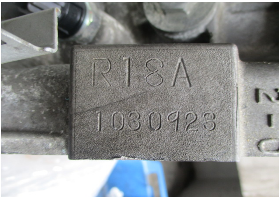
Photo 4 shows the engine number engraved on the housing of the Honda engine that I had inspected. The engine number was R18A1030923.
