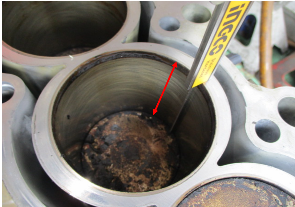
Photo 16 shows measurement of the stroke (arrowed) for cylinder 3 of the Honda engine that I had inspected. The bore and stroke measurements of the Honda engine were carried out using a digital Vernier Caliper that was calibrated before the start of measurements.
