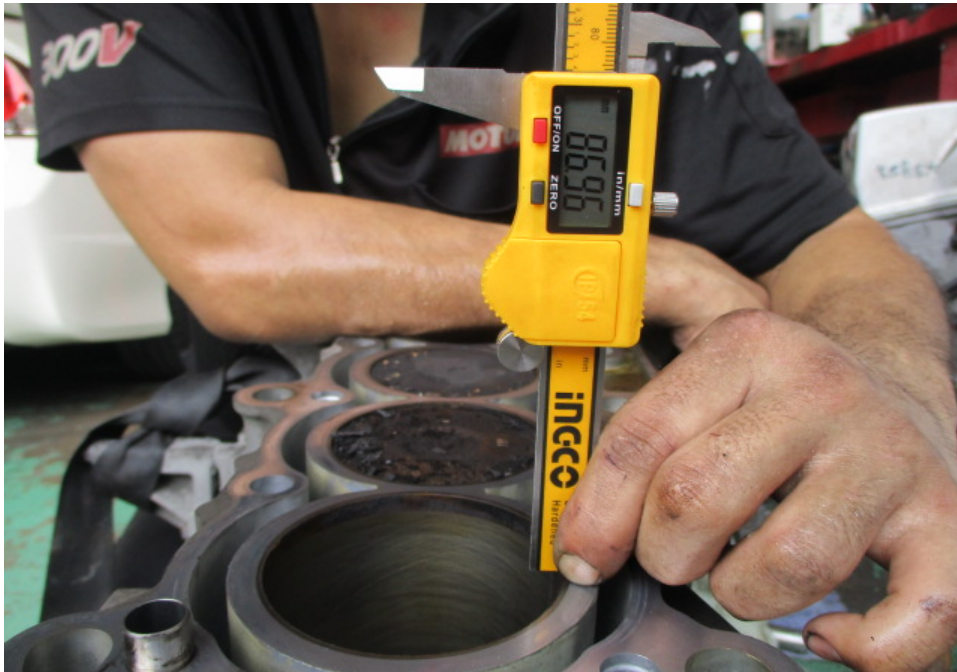
Photo 20 shows the stroke measurement of cylinder 4, which was recorded to be 86.96mm.
