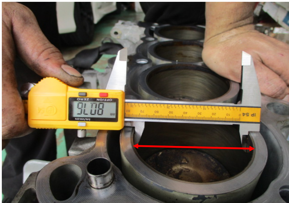
Photo 18 shows measurement being carried out to the bore (arrowed) of cylinder 4 of the Honda engine. The bore and stroke measurements of the Honda engine were carried out using a digital Vernier Caliper that was calibrated before the start of measurements. The bore measurement of cylinder 4 was recorded to be 80.76mm.
