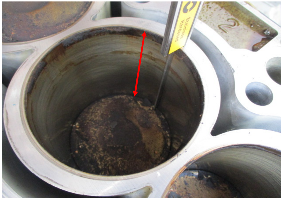
Photo 12 shows measurement of the stroke (arrowed) for cylinder 2 of the Honda engine that I had inspected. The bore and stroke measurements of the Honda engine were carried out using a digital Vernier Caliper that was calibrated before the start of measurements.
