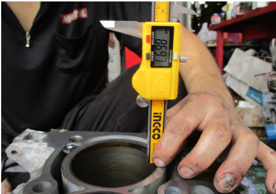
Photo 10 shows the stroke measurement of cylinder 1, which was recorded to be 86.97mm.
