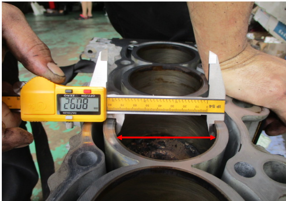
Photo 14 shows measurement being carried out to the bore (arrowed) of cylinder 3 of the Honda engine. The bore and stroke measurements of the Honda engine were carried out using a digital Vernier Caliper that was calibrated before the start of measurements. The bore measurement of cylinder 3 was recorded to be 80.92mm.
