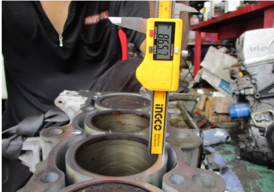
Photo 17 shows the stroke measurement of cylinder 3, which was recorded to be 86.57mm.
