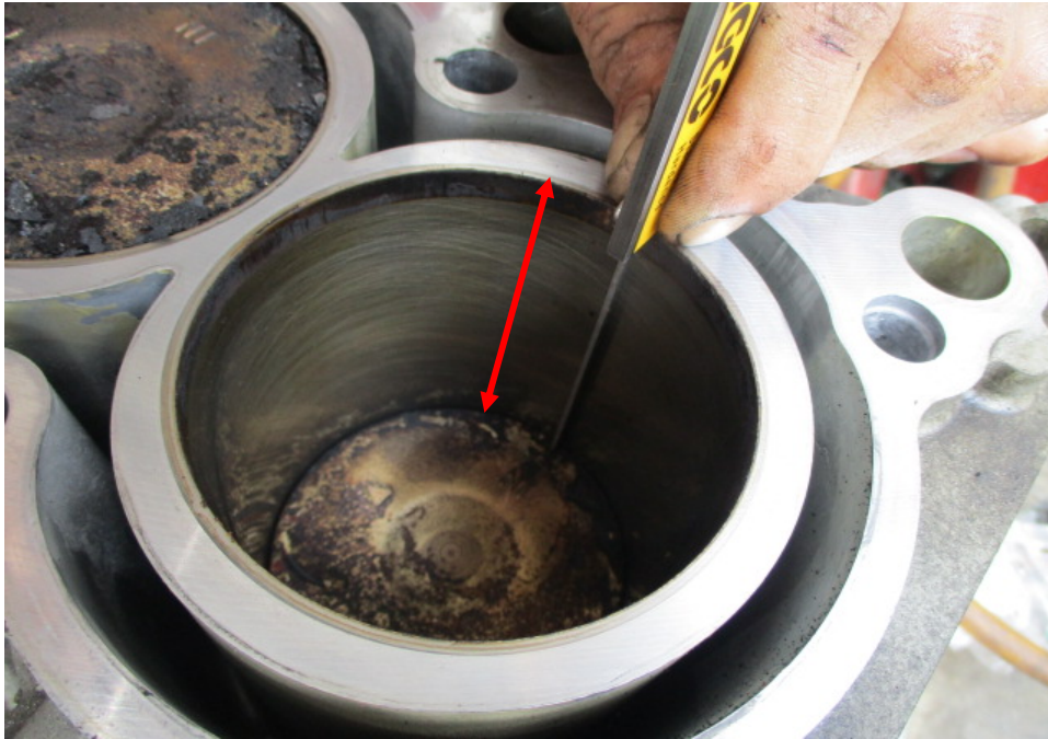
Photo 19 shows measurement being carried out to the stroke (arrowed) of cylinder 4 of the Honda engine. The bore and stroke measurements of the Honda engine were carried out using a digital Vernier Caliper that was calibrated prior to the start of measurements.
