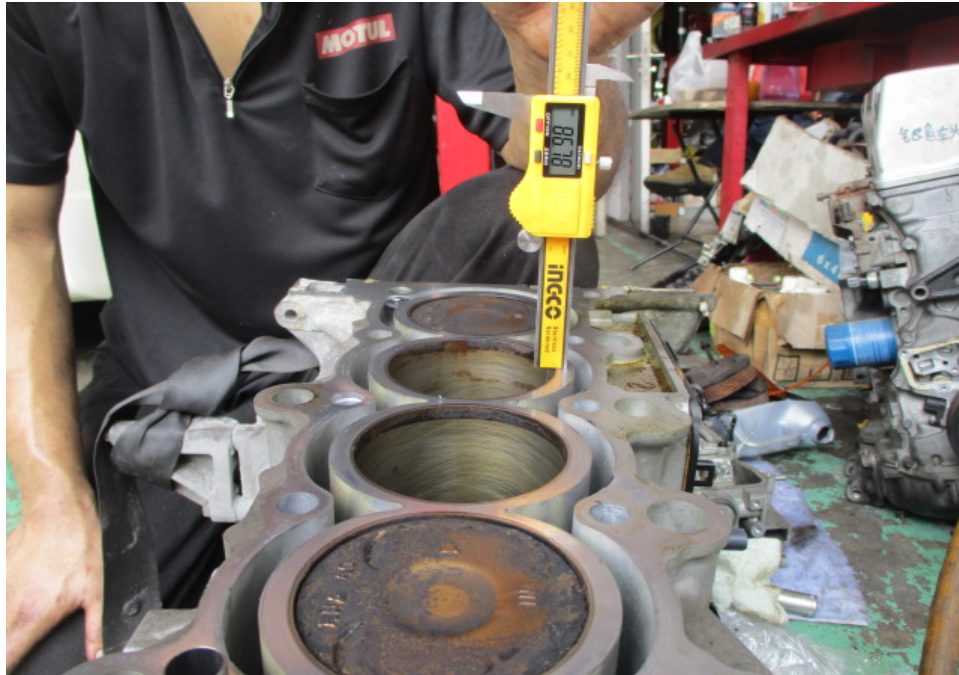
Photo 13 shows the stroke measurement of cylinder 2, which was recorded to be 86.78mm.
