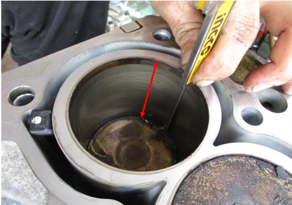
Photo 9 shows measurement being carried out to the stroke (arrowed) of cylinder 1 of the Honda engine. The bore and stroke measurements of the Honda engine were carried out using a digital Vernier Caliper that was calibrated before the start of the measurements.
