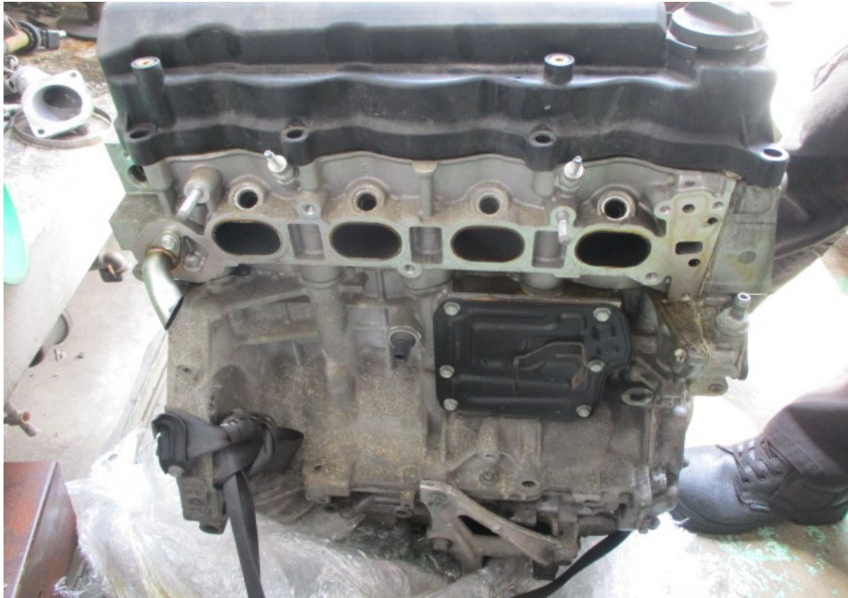
Photo 3 shows another view of the Honda engine that I had inspected. My visual examination of the engine housing revealed the housing to be of serviceable/satisfactory condition. There was no crack and/or hole observed on the engine housing.
