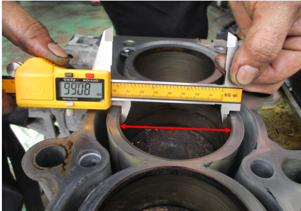
Photo 11 shows measurement being carried out to the bore (arrowed) of cylinder 2 of the Honda engine. The bore measurement of cylinder 2 was recorded to be 80.66mm.
