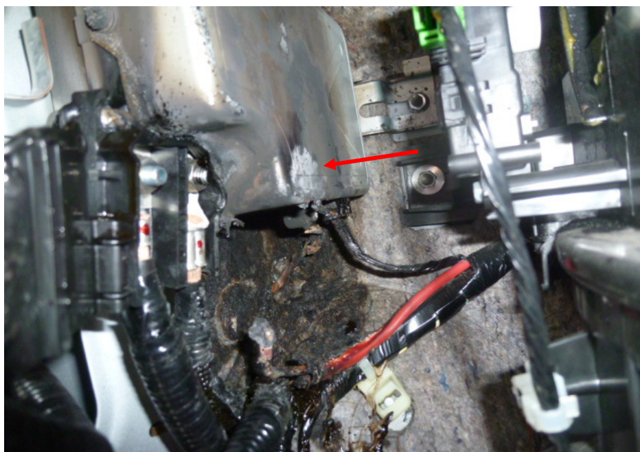
Photo 8 shows a close up view of the left portion of the interior compartment of the Insured Vehicle which had sustained fire damage (arrowed).
