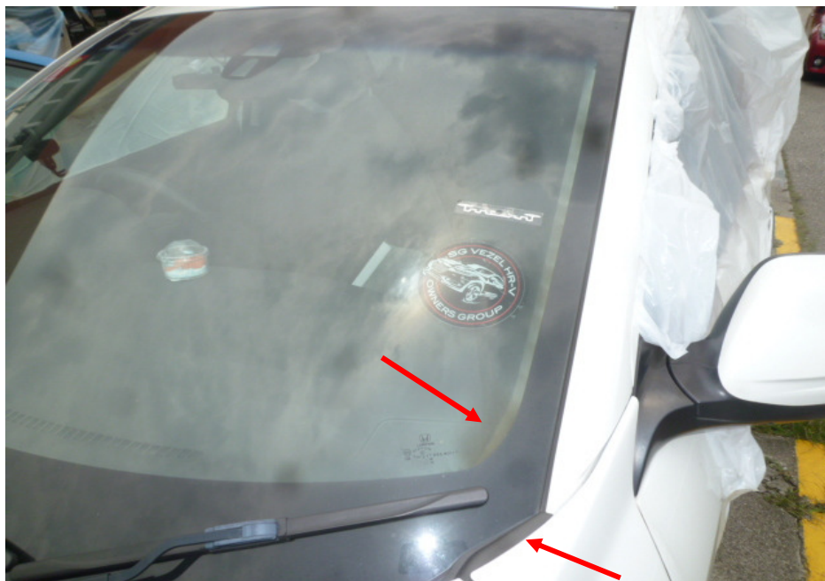
Photo 3 shows a closer view of the front windscreen of the Insured Vehicle at the time of our inspection. The front windscreen and wiper panel had sustained minimal fire damage (arrowed).
