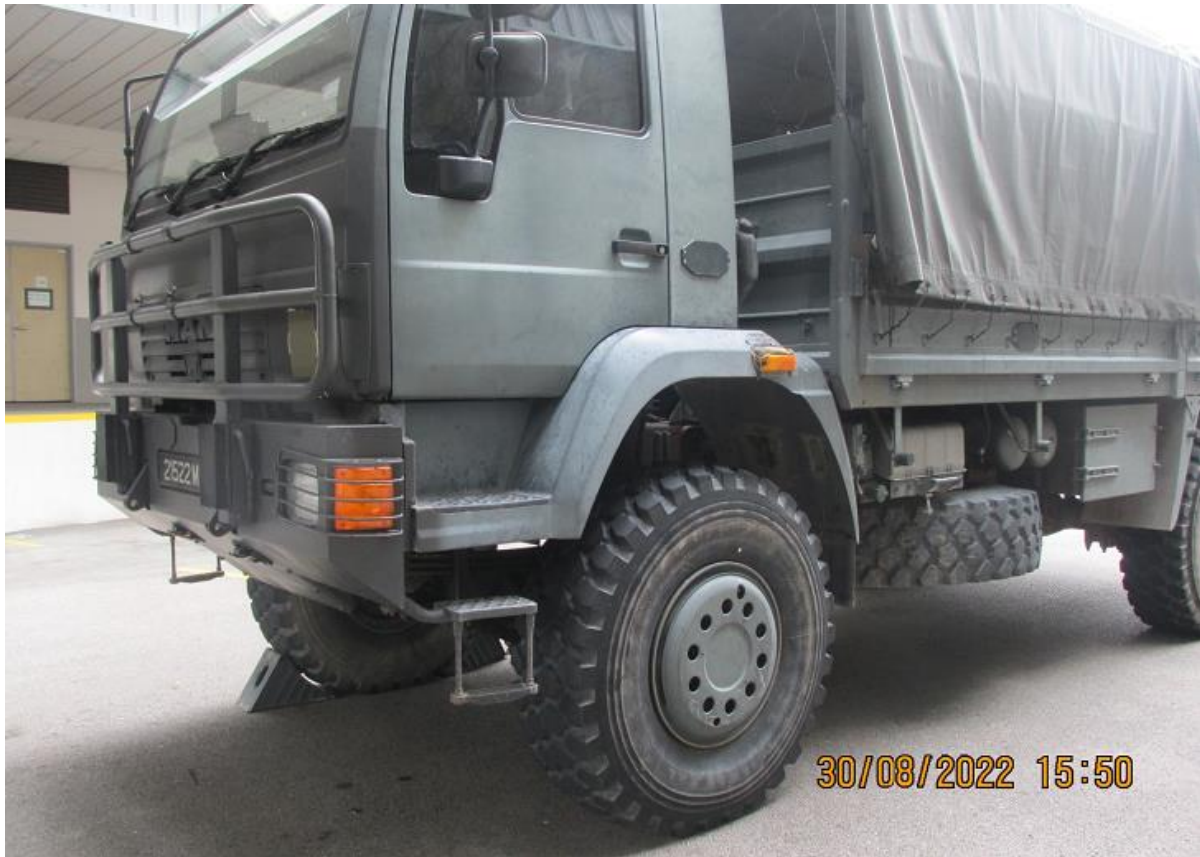
Figure 2G: Damages to front Left Bumper of MID21522
