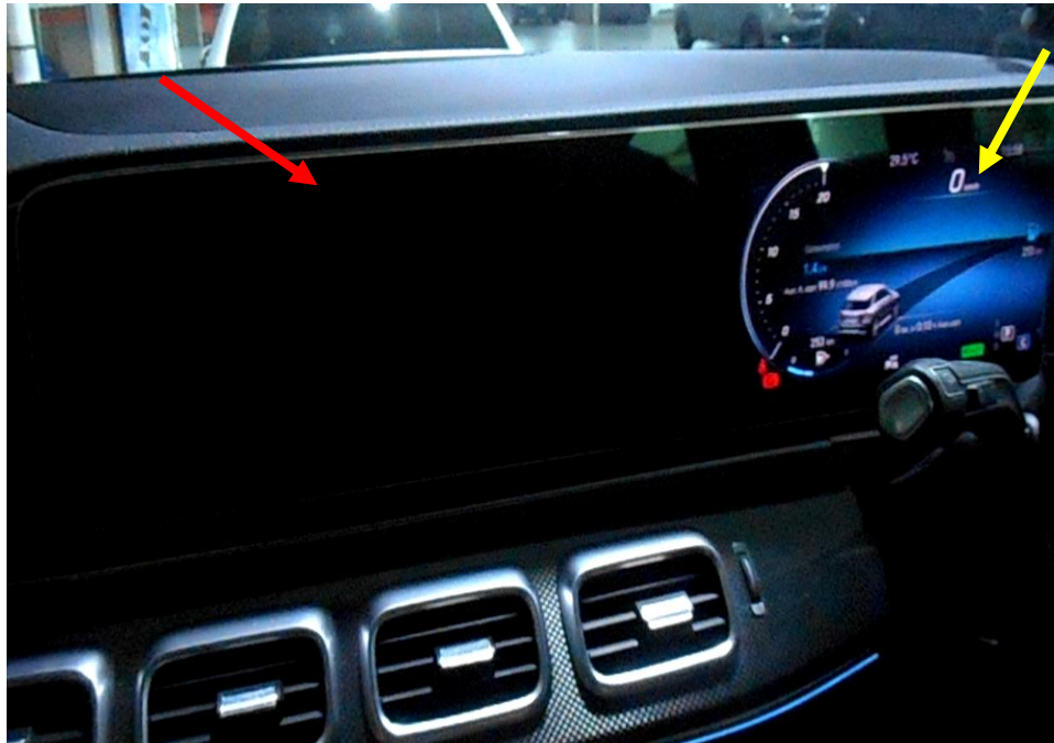
Photo 6 shows the close up view of the vehicle instrument portion of the Insured Vehicle at the time of our inspection. The infotainment instrument display (red arrowed) remained turned off even when the vehicle's engine is turned on as compared to the driver's display panel (yellow arrow).
