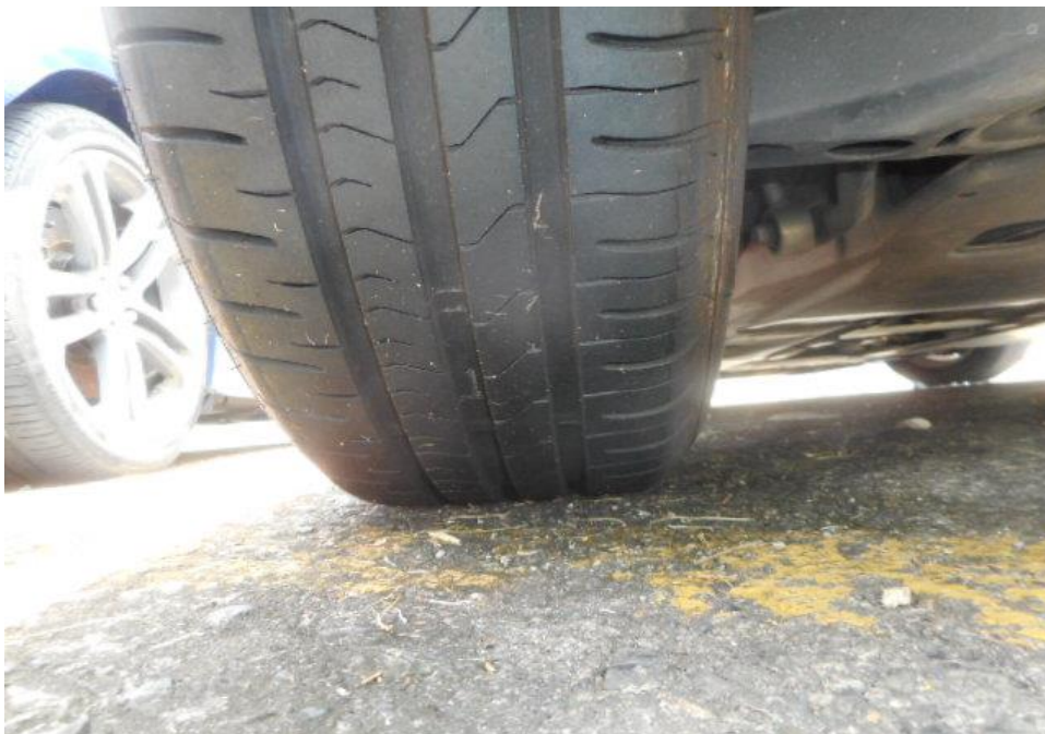
Photo 11 shows the condition of the rear left tyre of the Motor Car, which was observed to be in serviceable condition with remaining tread depth of approximately 7.3mm. The tyre, which was wrapped around alloy wheel rim, was also observed to be sufficiently inflated for vehicular operation. The 4 tyres of the Motor Car were wrapped around standard alloy wheel rims.
