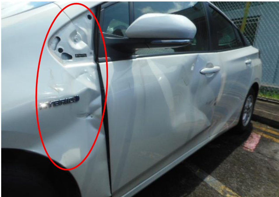
Photo 5 shows a close up view of the Motor Car's left body at the time of my inspection. The left portion of the Motor Car was observed to have sustained damage. Its front left fender (circled) was amongst the body parts that were damaged as a result of the accident.
