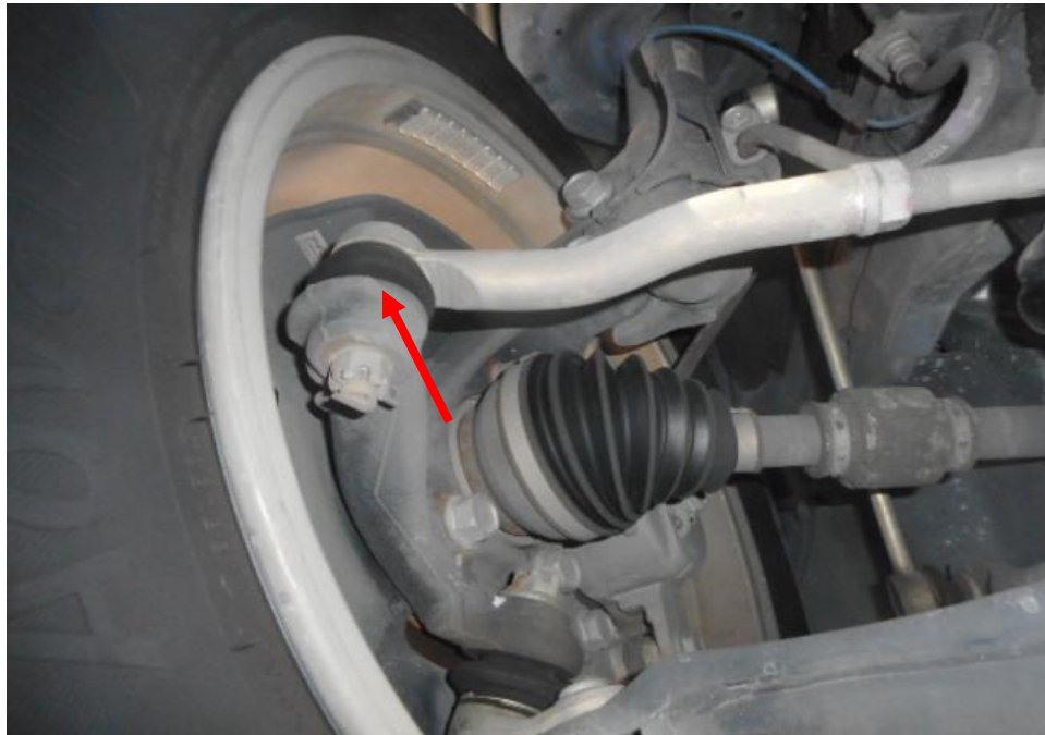
Photo 24 shows the various undercarriage components at the front left wheel of the Motor Car, which had included the steering tie rod (arrowed). The various undercarriage components of the Motor Car were all found to be intact without any visible damage.
