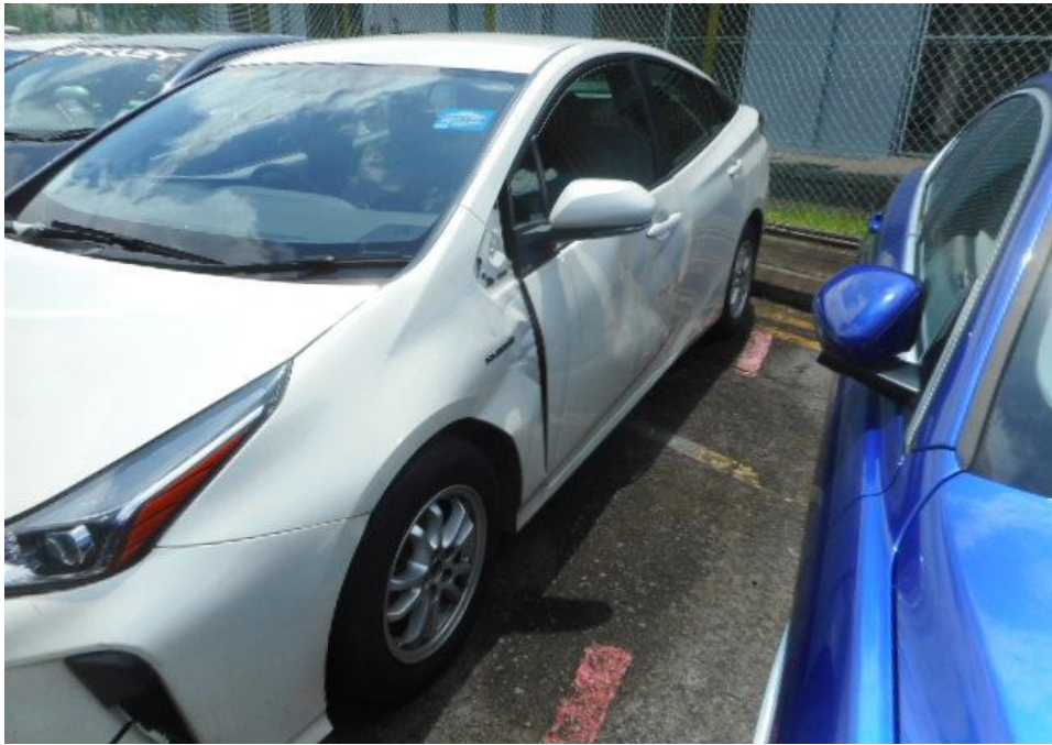
Photo 4 shows a general view of the Motor Car's left body at the time of my inspection. The Motor Car was observed to have sustained damage at its left portion. Its left front door and front left fender was amongst the body parts that were damaged as a result of the accident.
