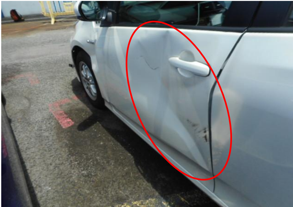
Photo 6 shows a close up view of the Motor Car's left body at the time of my inspection. The left portion of the Motor Car was observed to have sustained damage. Its left front door (circled) was amongst the body parts that were damaged as a result of the accident.
