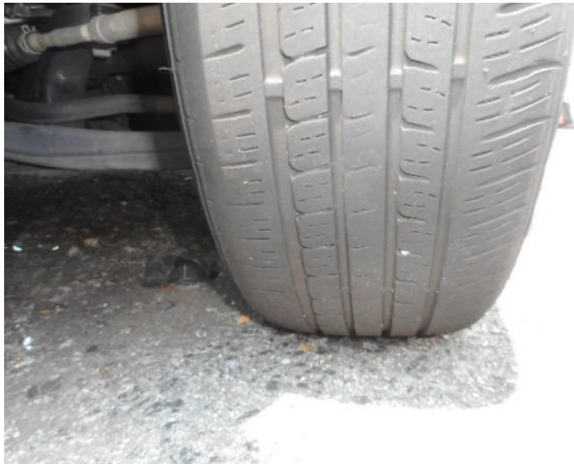
Photo 9 shows the condition of the front right tyre of the Motor Car, which was observed to be in serviceable condition with remaining tread depth of approximately 4.2mm. The tyre was sufficiently inflated for vehicular operation with no tear, cut or burst mark(s) on the outer and the inner sidewalls as well as across the tread. The 4 tyres of the Motor Car were wrapped around standard alloy wheel rims without any damage.
