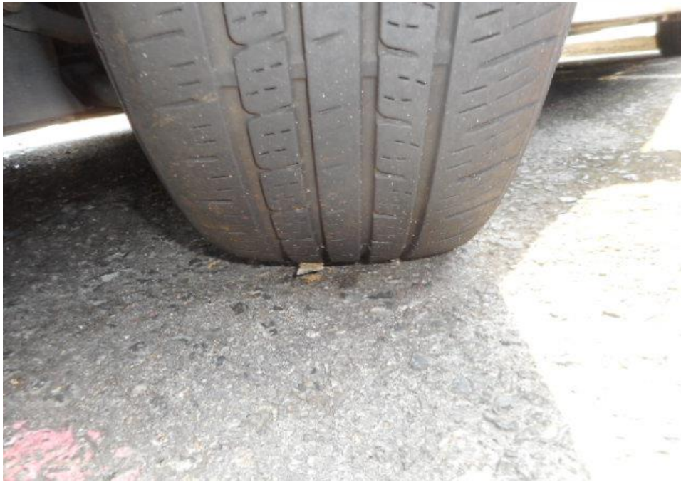
Photo 12 shows the condition of the front left tyre of the Motor Car, which was observed to be in serviceable condition with remaining tread depth of approximately 4.1mm. There was also no tear, cut or burst mark(s) on the outer and the inner sidewalls as well as across the tread of the Motor Car's 4 tyres.
