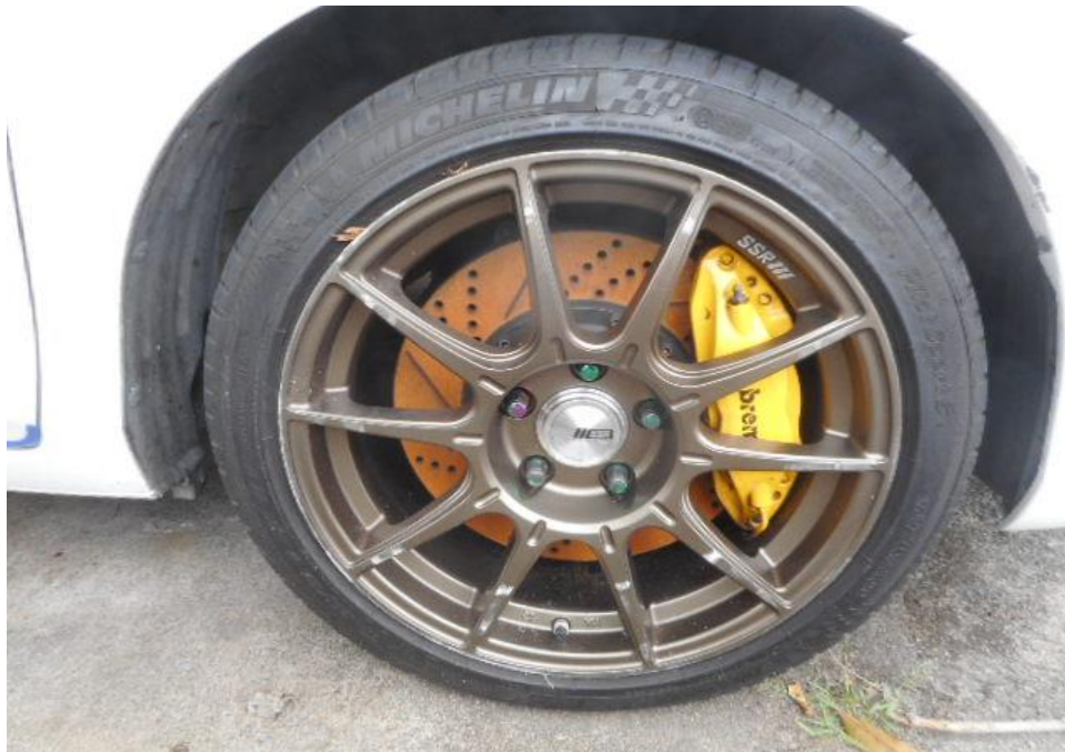
Photo 7 shows the condition of the front right tyre of the Motor Car, which was observed to be in serviceable condition with remaining tread depth of approximately 5.4mm. The tyre was sufficiently inflated for vehicular operation with no tear, cut or burst mark(s) on the outer and the inner sidewalls as well as across the tread. However, the wheel rim was observed to sustained minor scathes as a result of the accident.
