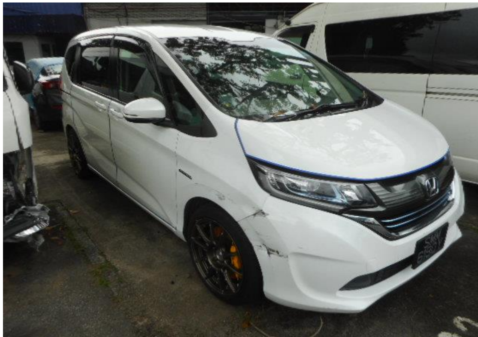
Photo 3 shows a general view of the Motor Car's right body at the time of my inspection. The Motor Car was observed to have sustained damage at its right portion. Its front right bumper portion and its right fender was amongst the body parts that were damaged as a result of the accident.
