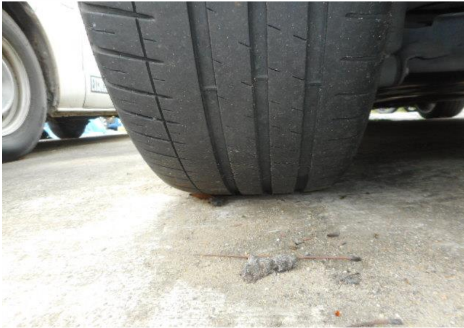
Photo 10 shows the condition of the rear left tyre of the Motor Car, which was observed to be in serviceable condition with remaining tread depth of approximately 3.7mm. The tyre, which was wrapped around alloy wheel rim, was also observed to be sufficiently inflated for vehicular operation. The 4 tyres of the Motor Car were wrapped around standard alloy wheel rims.
