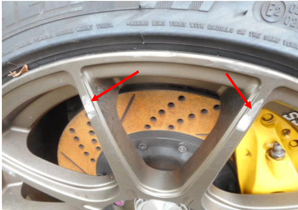
Photo 8 shows the close up view of the front right tyre of the Motor Car, which was observed to be in serviceable condition with remaining tread depth of approximately 5.4mm. The tyre was sufficiently inflated for vehicular operation with no tear, cut or burst mark(s) on the outer and the inner sidewalls as well as across the tread. However, the wheel rim (arrowed) was observed to sustained minor scathes as a result of the accident.
