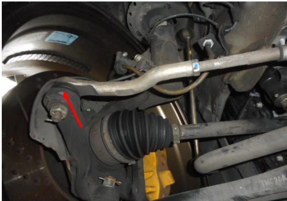
Photo 23 shows the various undercarriage components at the front left wheel of the Motor Car, which had included the steering tie rod (arrowed). The various undercarriage components of the Motor Car were all found to be intact without any visible damage.
