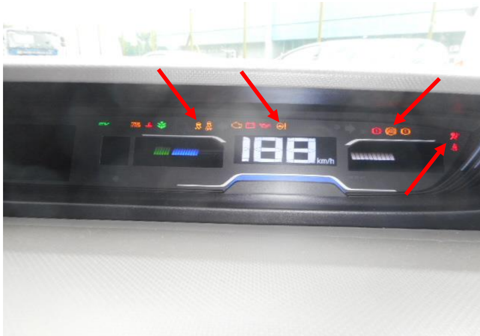
Photo 24 shows the warning light for Anti-Lock Brake System (ABS), Electronic Power Steering (EPS), Traction Control System (TCS), and Supplemental Restraint System (SRS) (arrowed) appearing on the instrument panel of the Motor Car during the self-test of its various electronic operating systems when its engine was cranked.
