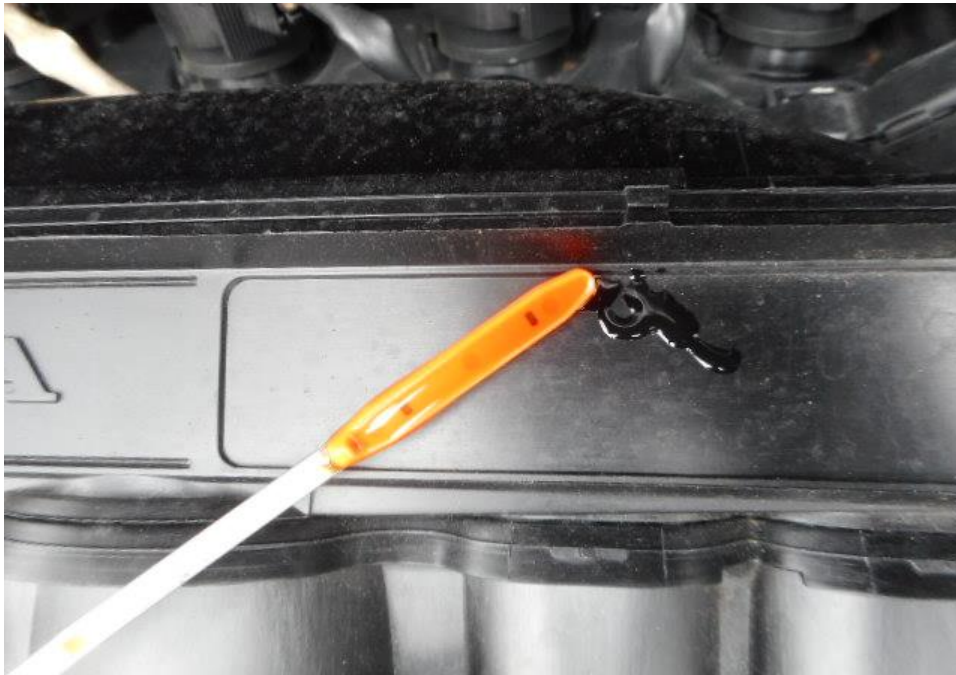
Photo 15 shows the engine oil level dipstick of the Motor Car at the time of my inspection. The engine oil was observed to be of sufficient level and without any visible contamination.
