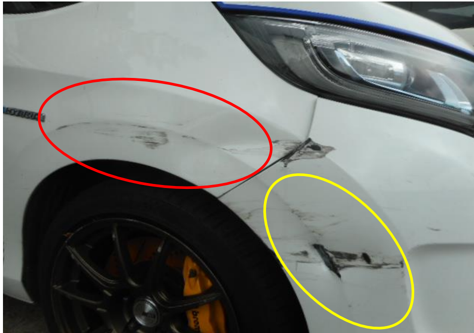
Photo 4 shows a close up view of the Motor Car's front body at the time of my inspection. The front portion of the Motor Car was observed to have sustained damage. Its front right bumper (yellow circle) and right fender (red arrow) was the body parts that were damaged as a result of the accident.
