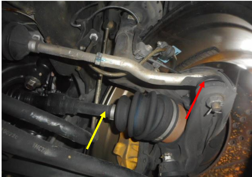
Photo 22 shows the various undercarriage components at the front right wheel of the Motor Car, in particular the steering tie rod (red arrow) and in particular the drive shaft (yellow arrow). The various steering components were all found to be intact, suggesting that the steering system of the Motor Car was likely to be in serviceable condition at the material time of accident. There was also no sign of fluid stain observed on the various undercarriage components at the front right wheel of the Motor Car.
