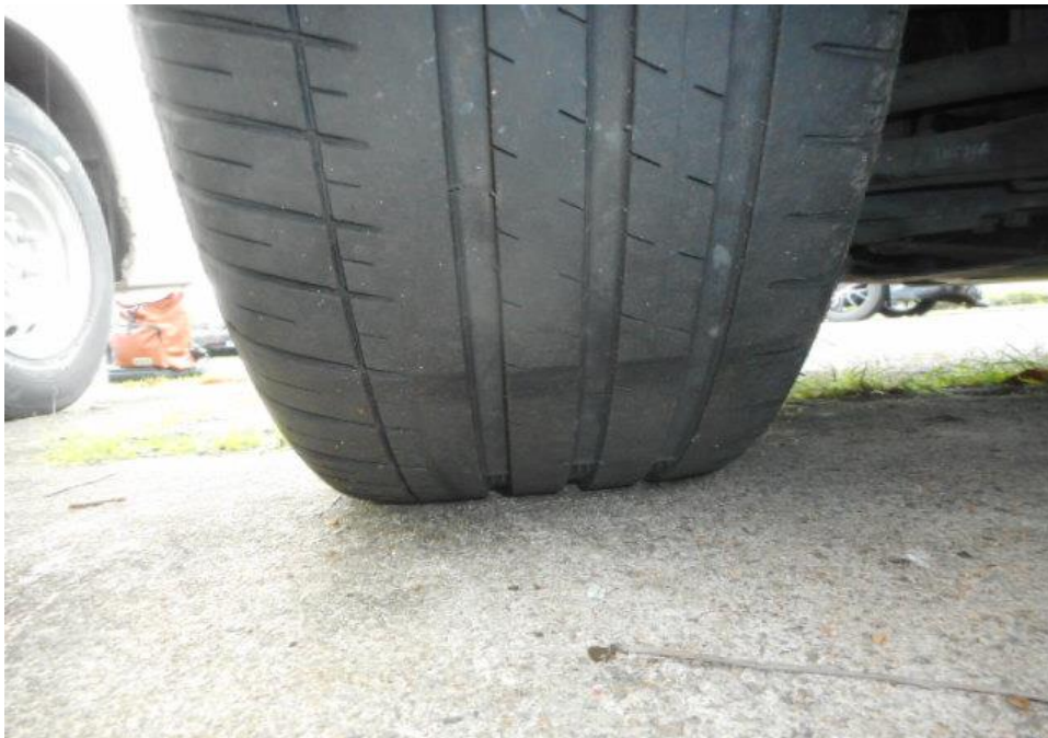
Photo 11 shows the condition of the front left tyre of the Motor Car, which was observed to be in serviceable condition with remaining tread depth of approximately 4.6mm. There was also no tear, cut or burst mark(s) on the outer and the inner sidewalls as well as across the tread of the Motor Car's 4 tyres.
