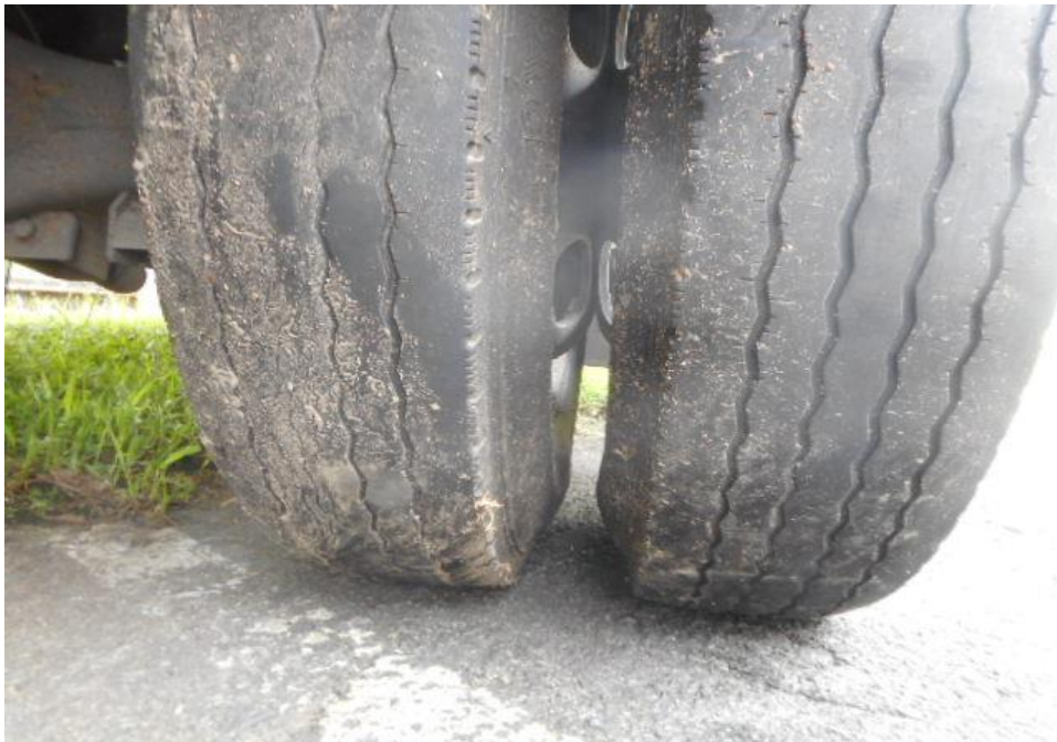
Photo 10 shows the condition of the rear left tyres of the Motor Lorry, which were observed to be in serviceable condition with remaining, tread depth of approximately 2.3mm.
