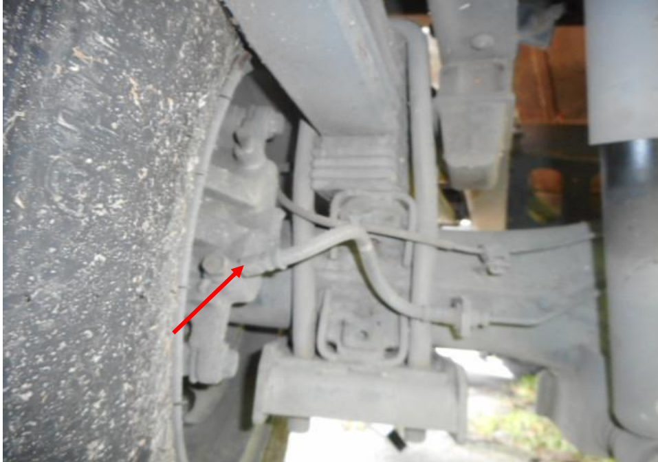
Photo 19 shows the brake pipe (arrowed) at the rear left wheel of the Motor Lorry. I did not observe any leakage of brake fluid at the time of my inspection of the Motor Lorry. My visual examination of the various mechanical components in the braking system and they were all found to be intact without any visible damage.
