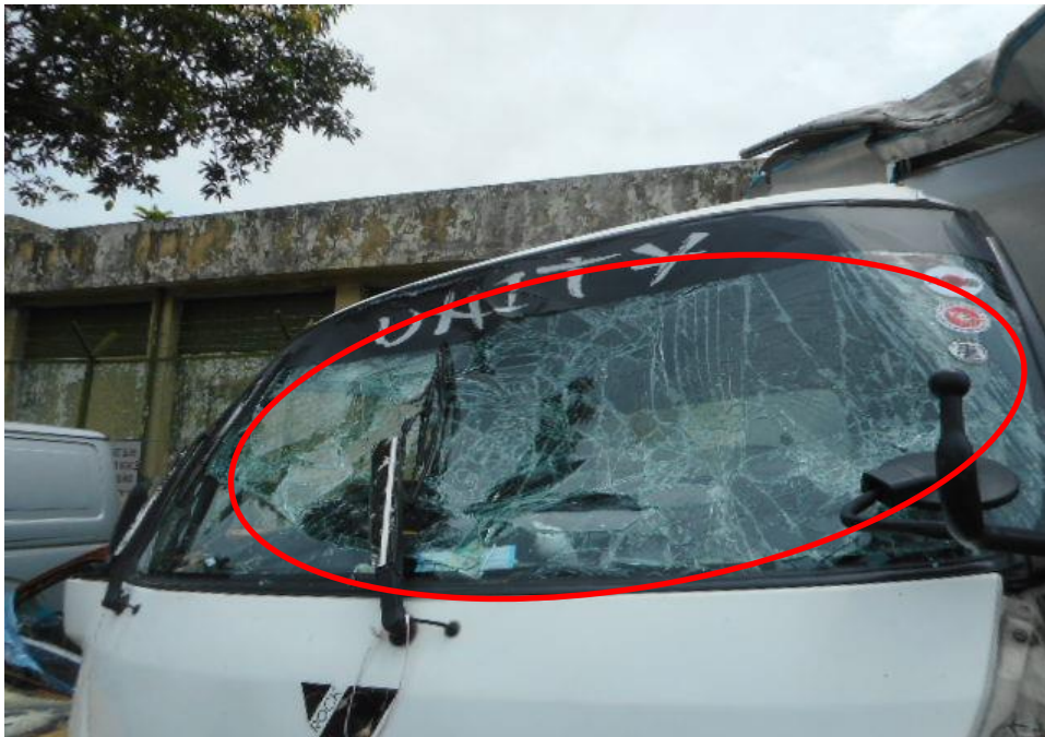
Photo 2 shows the close up view of the front portion of the Motor Lorry at the time of our inspection. The Motor Lorry was observed to have sustained major damages to its front windscreen (circled) that was damaged as a result of the accident's impact.
