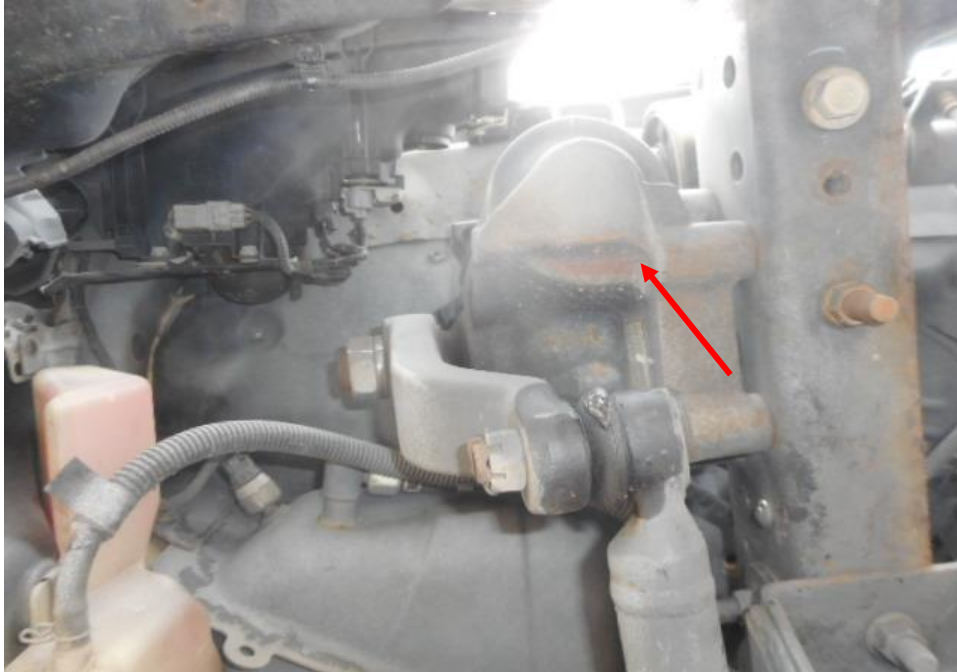
Photo 17 shows the various undercarriage components at the front right wheel of the Motor Lorry, in particular the steering box (arrowed). The various undercarriage components of the Motor Lorry were all found to be intact without any visible damage. There was also no sign of fluid stain(s) observed on the various undercarriage components.
