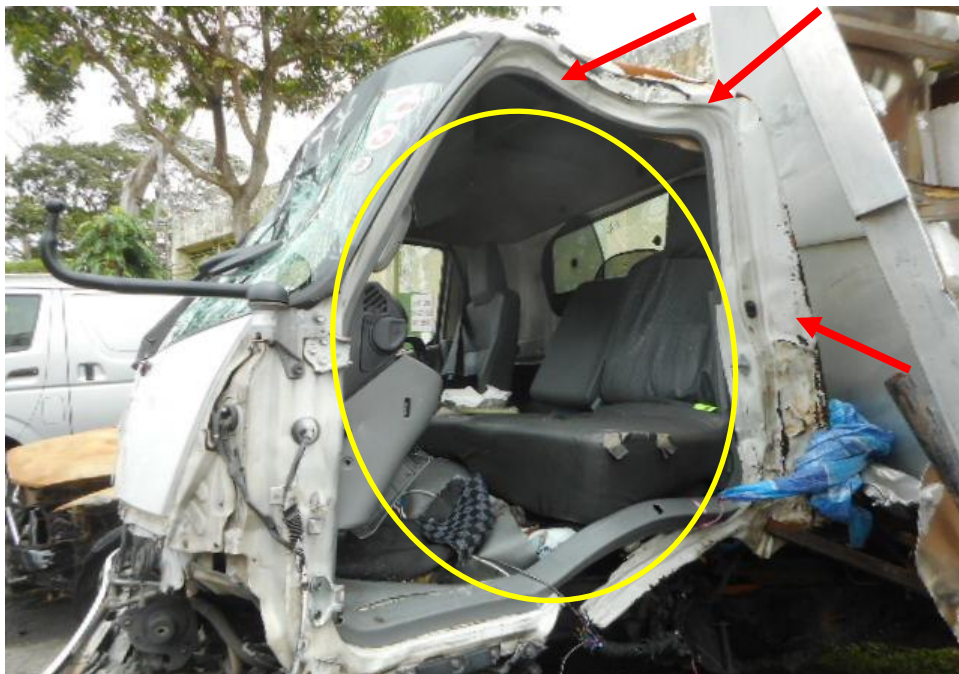
Photo 4 shows the close up view of the front portion of the Motor Lorry at the time of our inspection. The Motor Lorry was observed to have sustained major damages to its front left door (circled) and its front cabin (arrowed) that was crushed due to the accident's impact.
