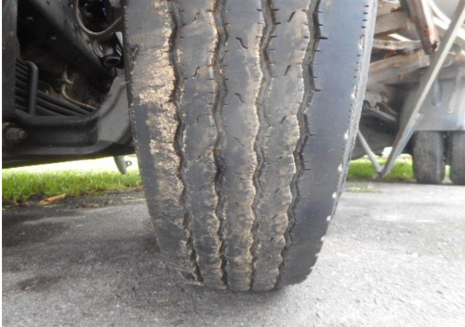
Photo 11 shows the condition of the front left tyre of the Motor Lorry, which were observed to be in serviceable condition with remaining, tread depth of approximately 6.5mm. There was also no tear, cut or burst mark(s) on the outer and the inner sidewalls as well as across the tread of the 6 tyres that were fitted on the Motor Lorry.
