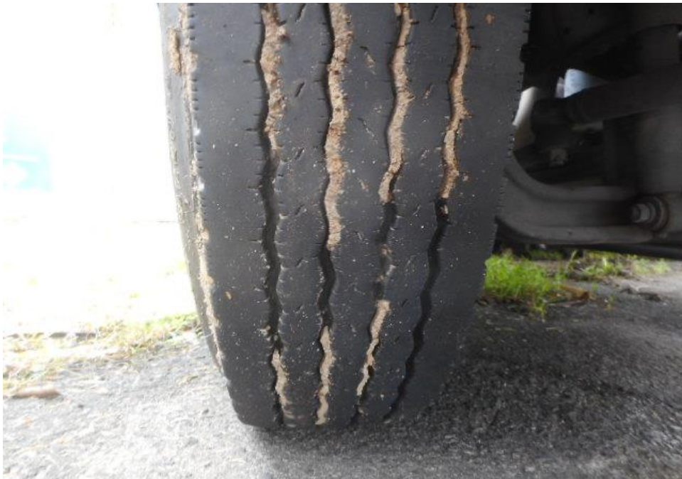
Photo 8 shows the condition of the front right tyre of the Motor Lorry, which were observed to be in serviceable condition with remaining, tread depth of approximately 4.1mm. The tyre, which was wrapped around standard steel wheel rim, it was observed to be sufficiently inflated for vehicular operation.
