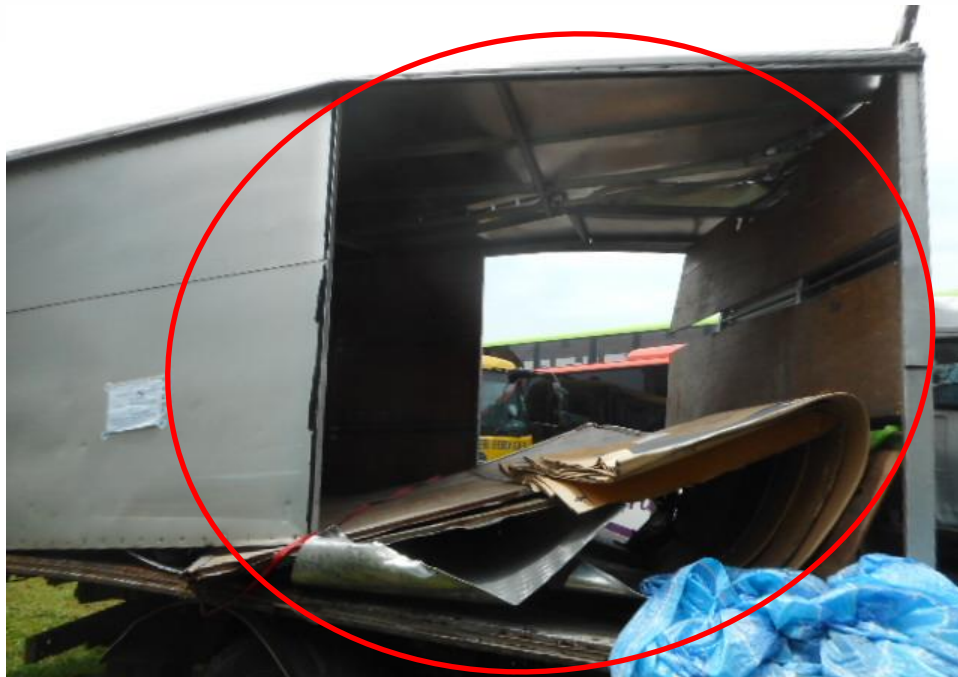
Photo 5 shows a general view of the Motor Lorry's right body at the time of my inspection. The right body panel of the rear cabin (circled) of the Motor Lorry was observed to sustain damage as a result of the accident.
