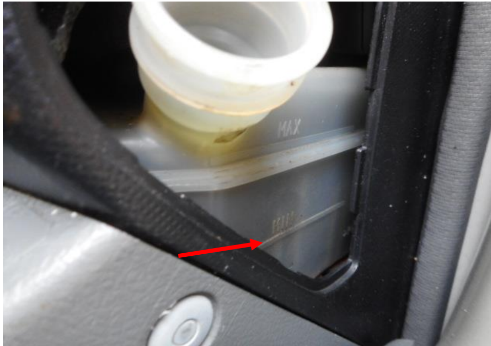
Photo 14 shows the brake fluid reservoir of the Motor Lorry at the time of my inspection. The brake fluid was observed to be of sufficient level (arrowed) and without any visible contamination.
