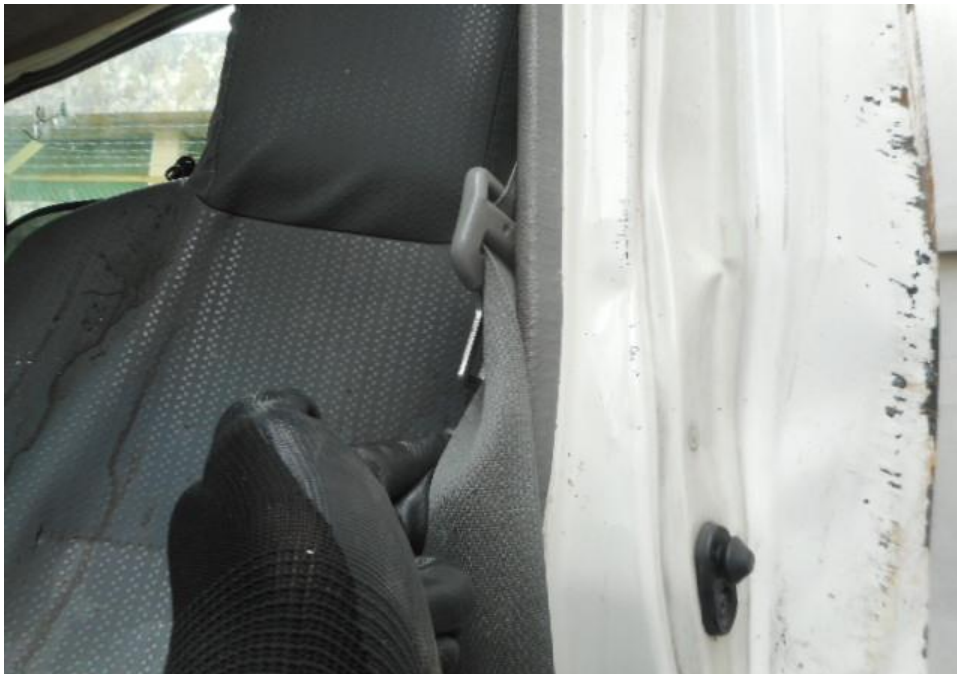
Photo 24 shows that the seat belt on the left seat was not worn at the material time of accident as the safety pre-tensioners was activated at the moment of impact and caused the seat belt to be locked into the last position.
