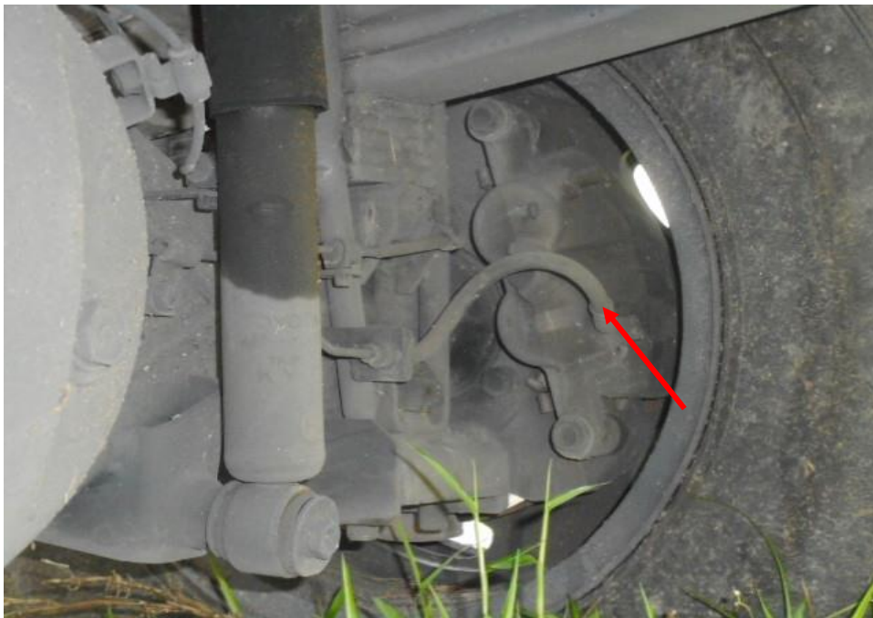
Photo 18 shows the brake pipe (arrowed) at the rear right wheel of the Motor Lorry. I did not observe any leakage of brake fluid at the time of my inspection of the Motor Lorry. My visual examination of the various mechanical components in the braking system and they were all found to be intact without any visible damage.
