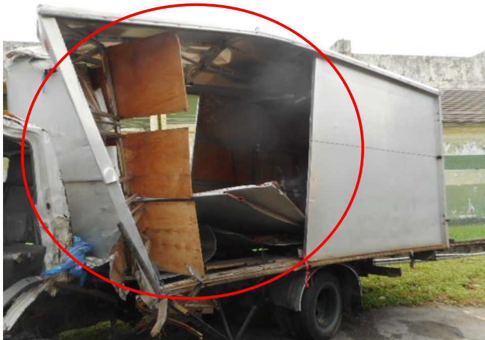
Photo 6 shows a general view of the Motor Lorry's left body at the time of my inspection. The left body panel of the rear cabin (circled) of the Motor Lorry was observed to sustain damage as a result of the accident.
