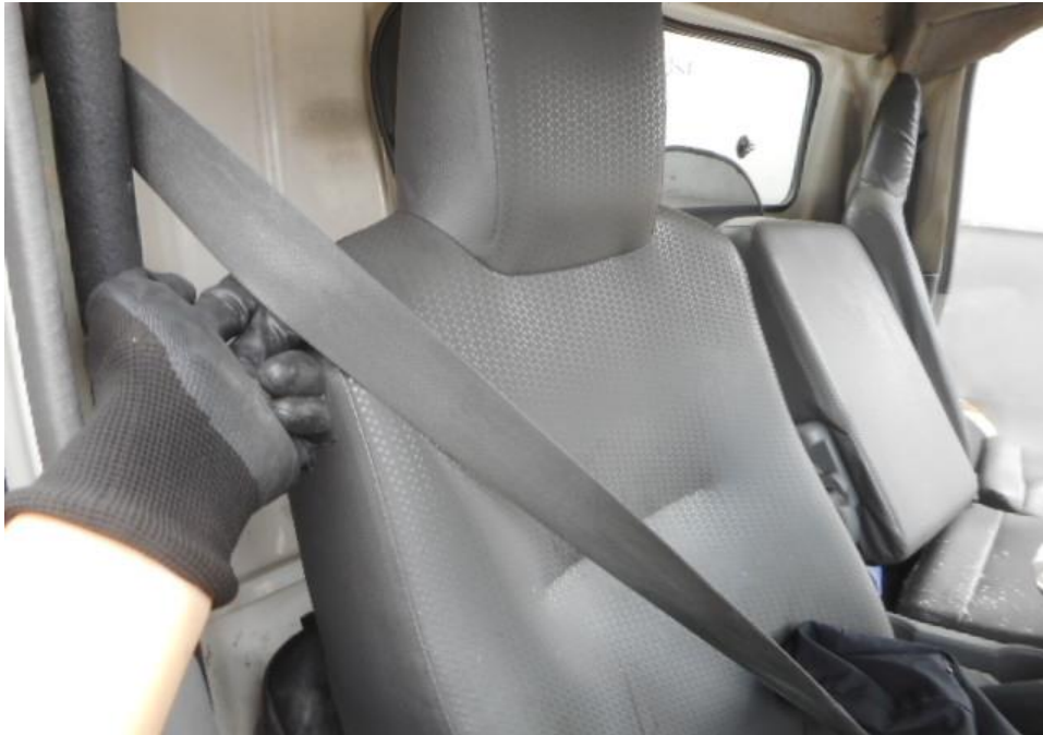
Photo 23 shows that the seat belt on the right seat was worn at the material time of accident as the safety pre-tensioners was activated at the moment of impact and caused the seat belt to be locked into the last position.
