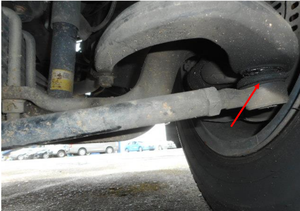
Photo 15 shows the various undercarriage components at the front right wheel of the Motor Lorry, in particular the steering tie rod end (arrowed). The various steering components were all found to be intact, suggesting that the steering system of the Motor Lorry was likely to be in serviceable condition at the material time of accident. There was also no sign of fluid stain(s) observed on the various undercarriage components.
