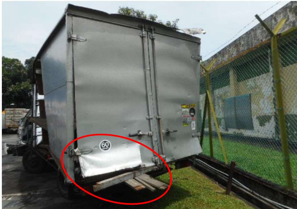
Photo 7 shows the general view of the Motor Lorry's rear body at the time of my inspection. The rear body panel of the rear cabin (circled) of the Motor Lorry was observed to sustain damage as a result of the accident.
