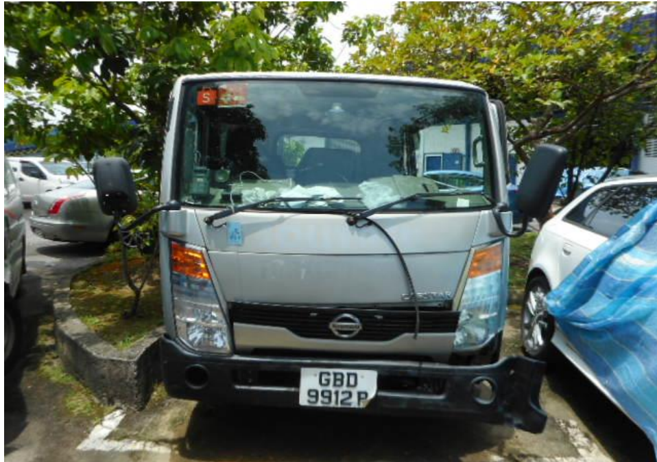
Photo 1 shows a general view of the front portion of the Motor Lorry at the time of our inspection. The Motor Lorry was observed to sustained major damage at its front and rear cabin, its front windscreen, front body panel, front bumper, front left door as well as its rear cabin were also damaged as a result of the accident.
