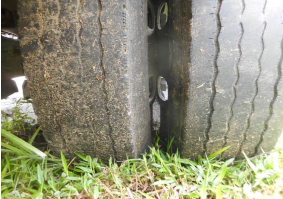
Photo 9 shows the condition of the rear right tyres of the Motor Lorry, which were observed to be in serviceable condition with remaining, tread depth of approximately 4mm. The tyre, which was wrapped around standard steel wheel rim, it was observed to be sufficiently inflated for vehicular operation.
