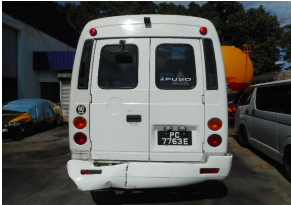
Photo 2 shows a general view of the rear body of the Motor Bus at the time of my inspection. The Motor Bus was observed to have sustained damages at its rear bumper was observed to be damaged at time of our inspection.
