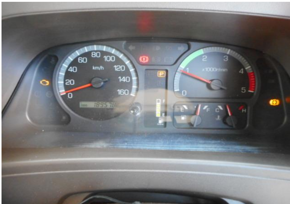
Photo 26 shows no warning lights illuminated on the instrument panel of the Motor Bus after the engine was cranked. This would suggest that there was no abnormality to the various electronic operating systems of the Motor Bus, like the ABS and etc.
