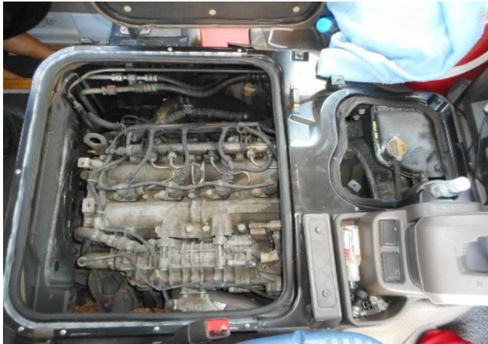
Photo 12 shows a general view of the Motor Bus's engine compartment, which was accessed by lifting the rear of the Motor Bus. The various parts and components inside the engine compartment were unaffected by the accident. There was also no sign(s) or indication(s) of fresh fluid leakage and/or fluid stain within the engine compartment
