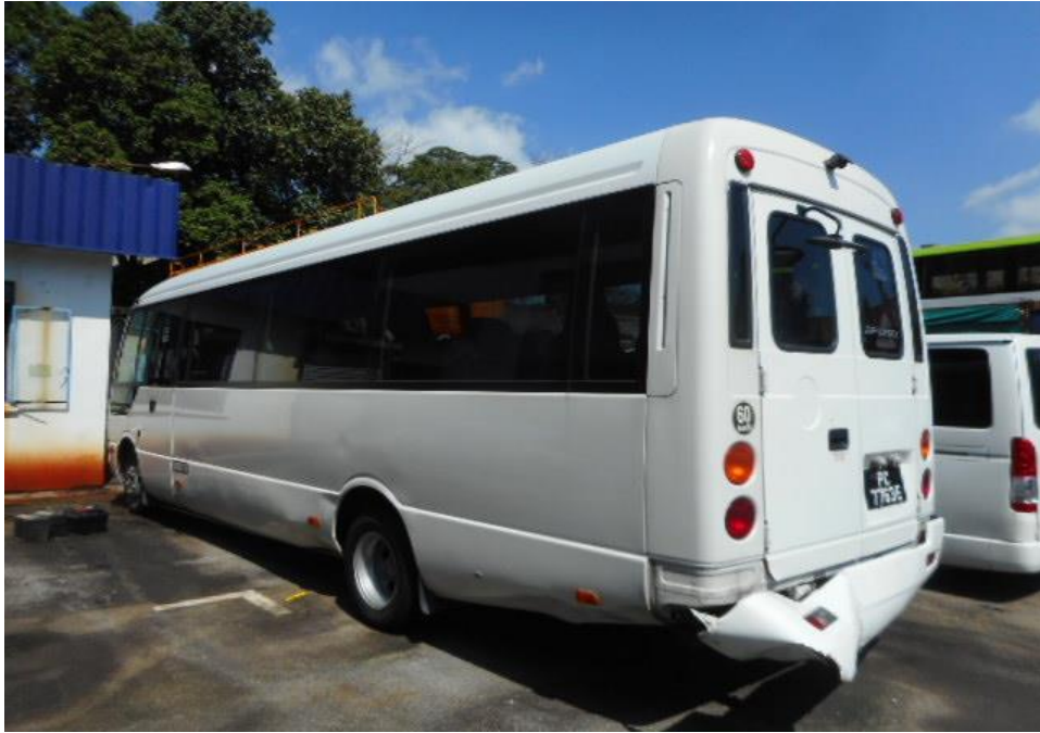
Photo 4 shows a general view of the left body of the Motor Bus at the time of my inspection. The Motor Bus was observed to have sustained damages at its left rear body panel was observed to be damaged at time of our inspection.
