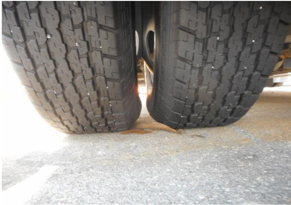
Photo 10 shows the condition of the rear left tyres of the Motor Bus, which was observed to be in serviceable condition with remaining tread depth of approximately 4.4mm. The tyres, which were wrapped around standard steel wheel rim, were also observed to be sufficiently inflated for vehicular operation. There was also no damage found on all 6 steel wheel rims of the Motor Bus.
