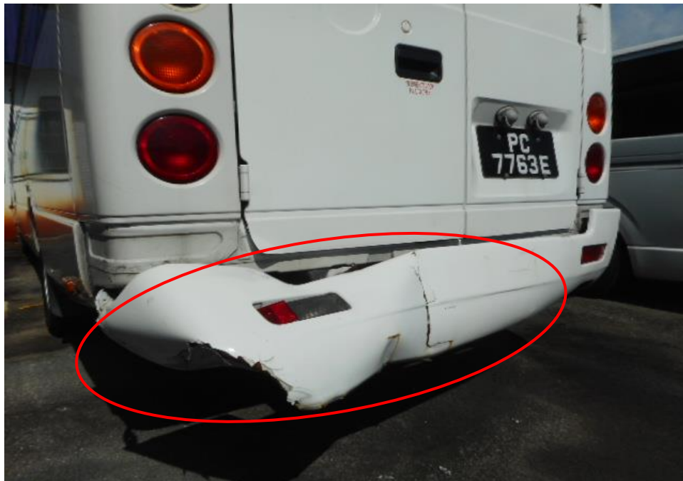
Photo 3 shows a close up view of the rear body of the Motor Bus at the time of our inspection. The Motor Bus was observed to have sustained damages at its rear bumper (circled) as a result of the accident.
