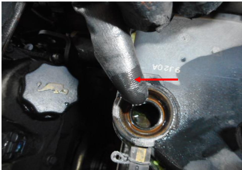
Photo 14 shows the engine coolant reservoir of the Motor Bus at the time of my inspection. The engine coolant was observed to be of sufficient level (arrowed) and without any visible contamination.
