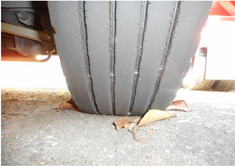
Photo 8 shows the condition of the front right tyre of the Motor Bus, which was observed to be in serviceable condition with remaining tread depth of approximately 4mm. The tyre, which was wrapped around standard steel wheel rim, was also observed to be sufficiently inflated for vehicular operation. There was no tear, cut or burst mark(s) on the outer and the inner sidewalls as well as across the tread of the 6 tyres that were fitted on the Motor Bus.
