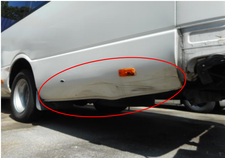
Photo 5 shows a close up view of the left body of the Motor Bus at the time of our inspection. The Motor Bus was observed to have sustained damages at its left rear body panel (circled) as a result of the accident.
