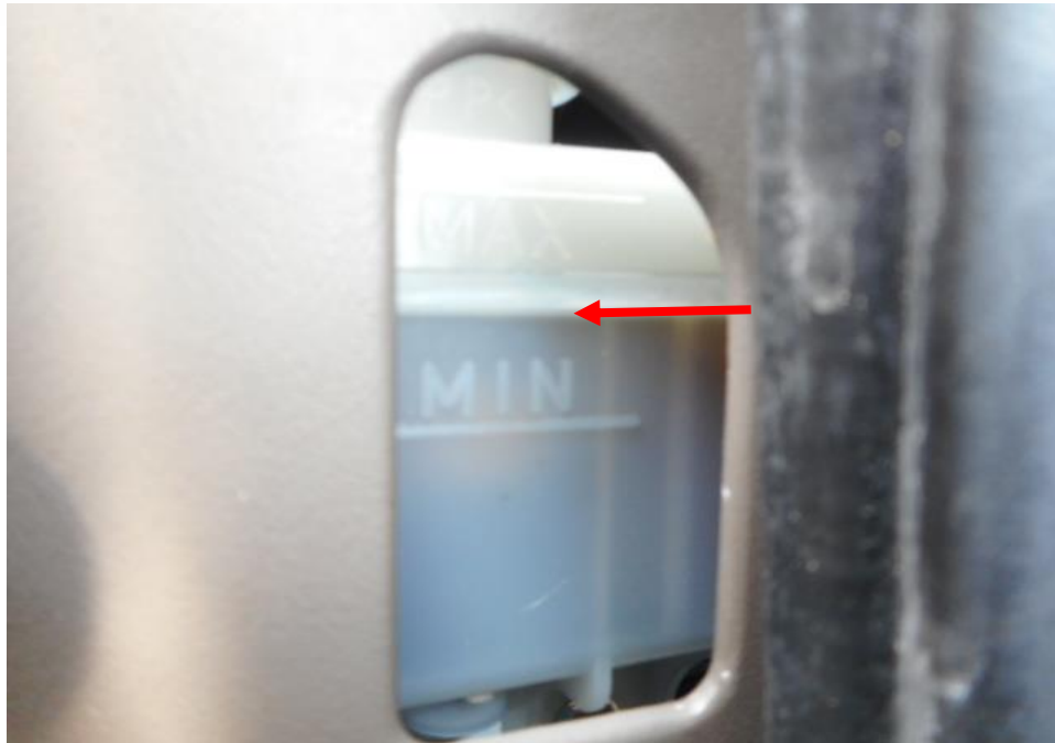
Photo 13 shows the brake fluid reservoir of the Motor Bus at the time of my inspection. The brake fluid was observed to be of sufficient level (arrowed) and without any visible contamination.
