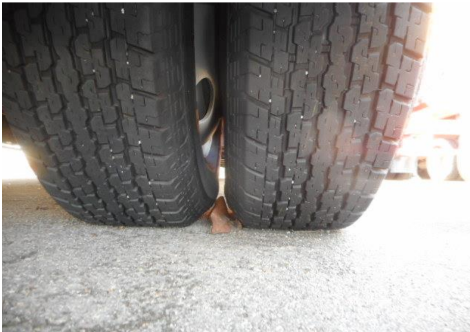
Photo 9 shows the condition of the rear right tyre of the Motor Bus, which was observed to be in serviceable condition with remaining tread depth of approximately 4.6mm. The tyre, which was wrapped around standard steel wheel rim, was also observed to be sufficiently inflated for vehicular operation.
