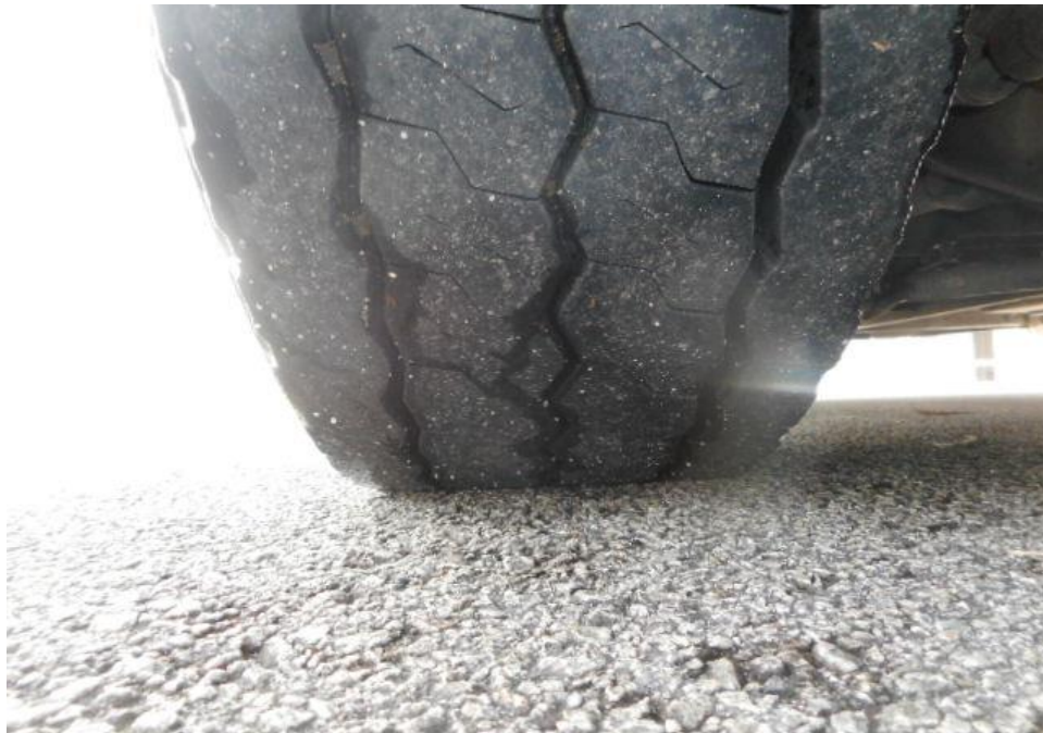
Photo 11 shows the condition of the front left tyres of the Motor Bus, which were observed to be in serviceable condition with remaining tread depth of approximately 3.6mm. There was also no tear, cut or burst mark(s) on the outer and the inner sidewalls as well as across the tread of the 6 tyres that were fitted on the Motor Bus.
