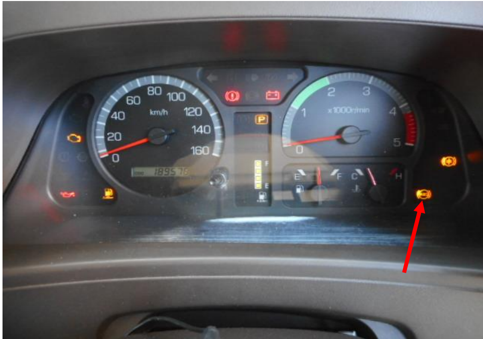
Photo 25 shows the warning light for Anti-Lock Braking System (ABS) appearing on the instrument panel of the Motor Bus during the self-test of its various electronic operating systems when its engine was cranked.
