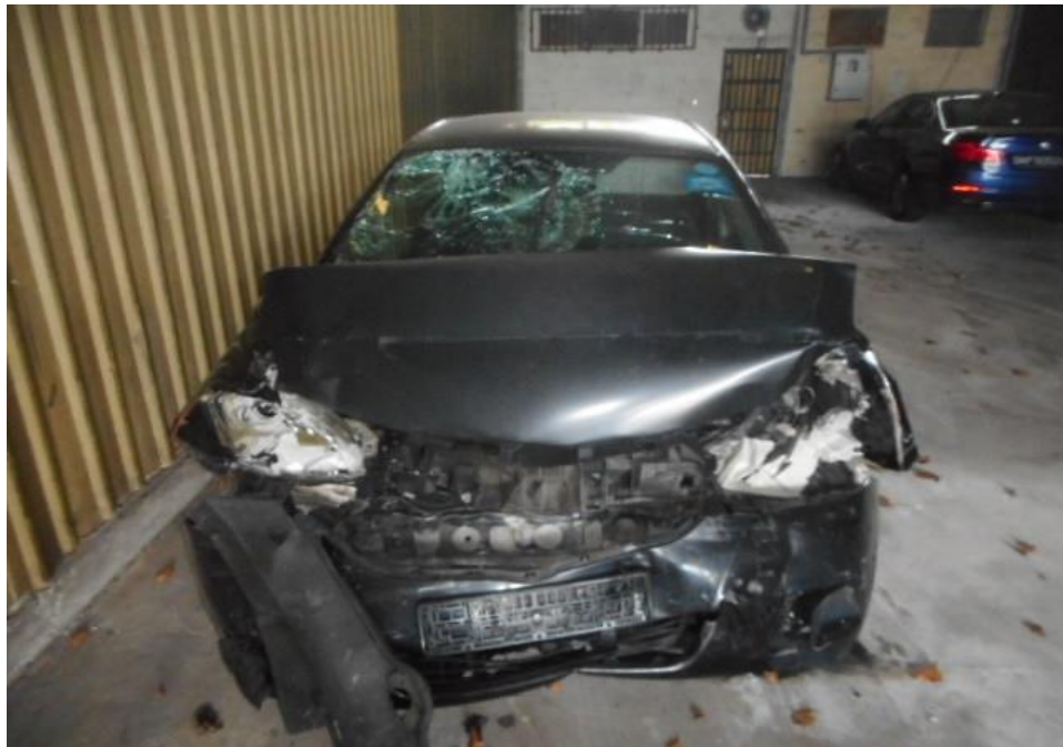
Photo 2 shows a general view of the Motor Car's front body at the time of my inspection. The Motor car was observed to have sustained damage at its front portion. Its front windscreen, front bonnet, front bumper, front left and right fender, front left and right headlamp was amongst the body parts and various engine components were also damaged as a result of the accident. The Supplemental Restraint System (SRS) was activated as a result of the accident.
