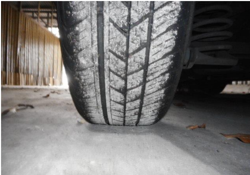
Photo 12 shows the condition of the rear left tyre of the Motor Car, which was observed to be in serviceable condition with remaining tread depth of approximately 4.2mm. The tyre was also observed to be sufficiently inflated for vehicular operation with no tear, cut or burst mark(s).
