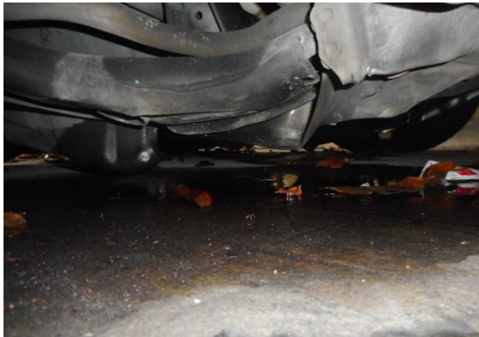
Photo 17 shows the undercarriage of the Motor Car, at the area where the engine housing and transmission housing are located. I found sign(s) or indication(s) of fluid leak and/or fluid stain(s) on the underside of the Motor Car due to the damaged engine as a result of the accident.
