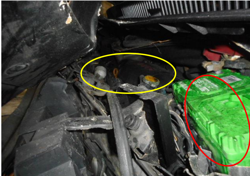
Photo 16 shows the close up view of the Motor Car's front body at the time of my inspection. The Motor car was observed to have sustained damage at its front portion. Its ignition system battery (red circle) and engine (yellow circle) was amongst the various components in the engine compartments were also damaged as a result of the accident.
