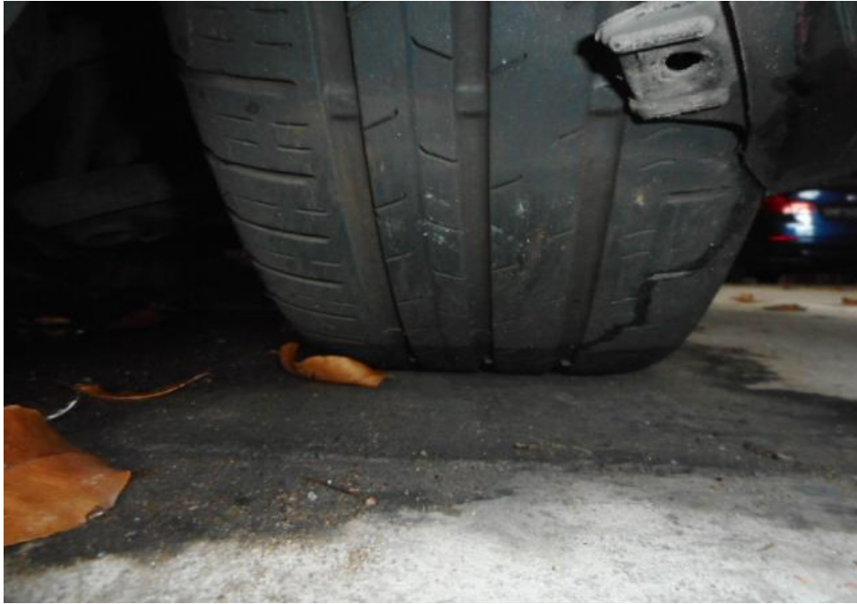
Photo 13 shows the condition of the front left tyre of the Motor Car, which was observed to be in serviceable condition with remaining tread depth of approximately 3.1mm. The tyre was also observed to be sufficiently inflated for vehicular operation with no tear, cut or burst mark(s).
