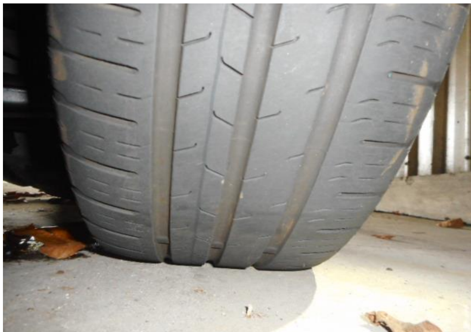
Photo 10 shows the condition of the front right tyre of the Motor Car, which was observed to be in serviceable condition with remaining tread depth of approximately 4.5mm. The tyre, which was wrapped around alloy wheel rim, was also observed to be sufficiently inflated for vehicular operation.
