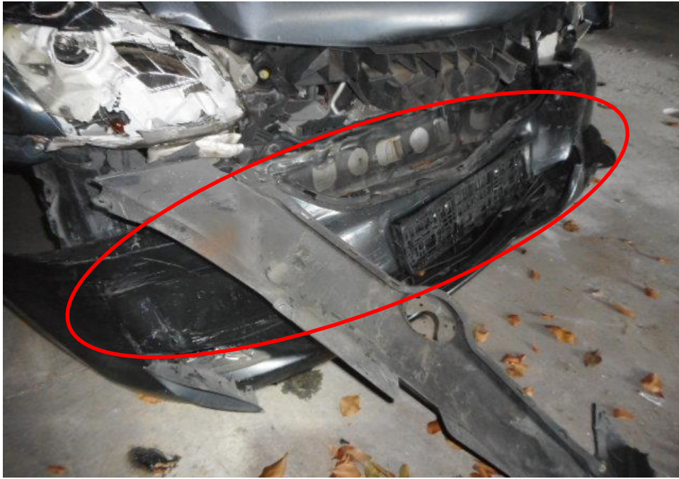
Photo 5 shows the close up view of the Motor Car's front body at the time of my inspection. The Motor car was observed to have sustained damage at its front portion. Its front bumper (circled) was damaged as a result of the accident.
