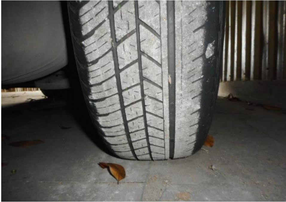
Photo 11 shows the condition of the rear right tyre of the Motor Car, which was observed to be in serviceable condition with remaining tread depth of approximately 3.3mm. The tyre was also observed to be sufficiently inflated for vehicular operation with no tear, cut or burst mark(s).
