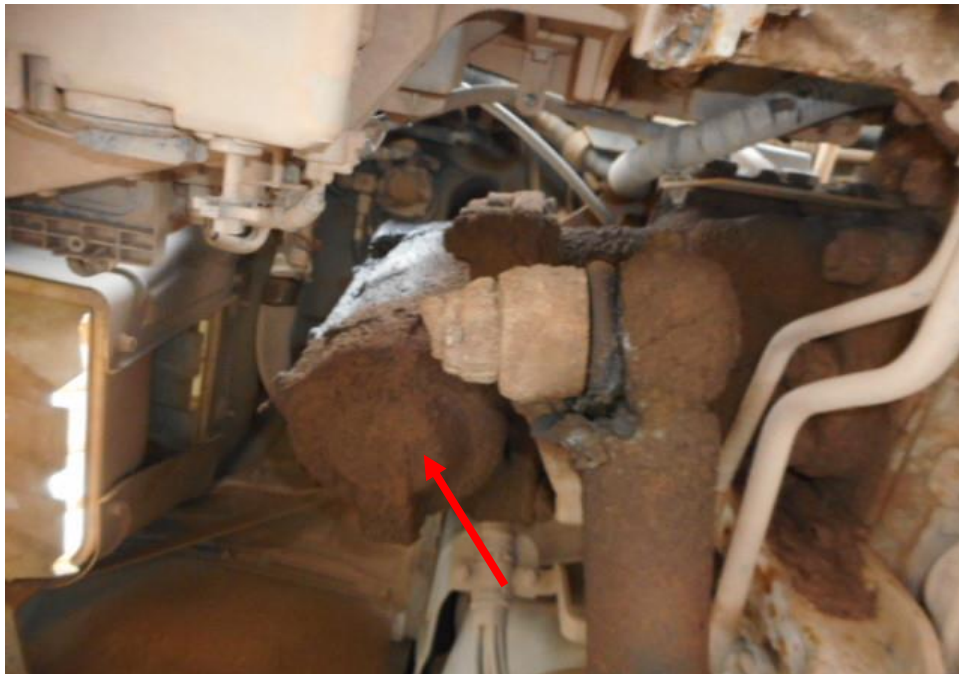
Photo 23 shows the steering box component (arrowed) at the undercarriage of the Tipper Truck was found to be intact without any visible damage. There was also no sign of fluid stain(s) observed on the various undercarriage components.
