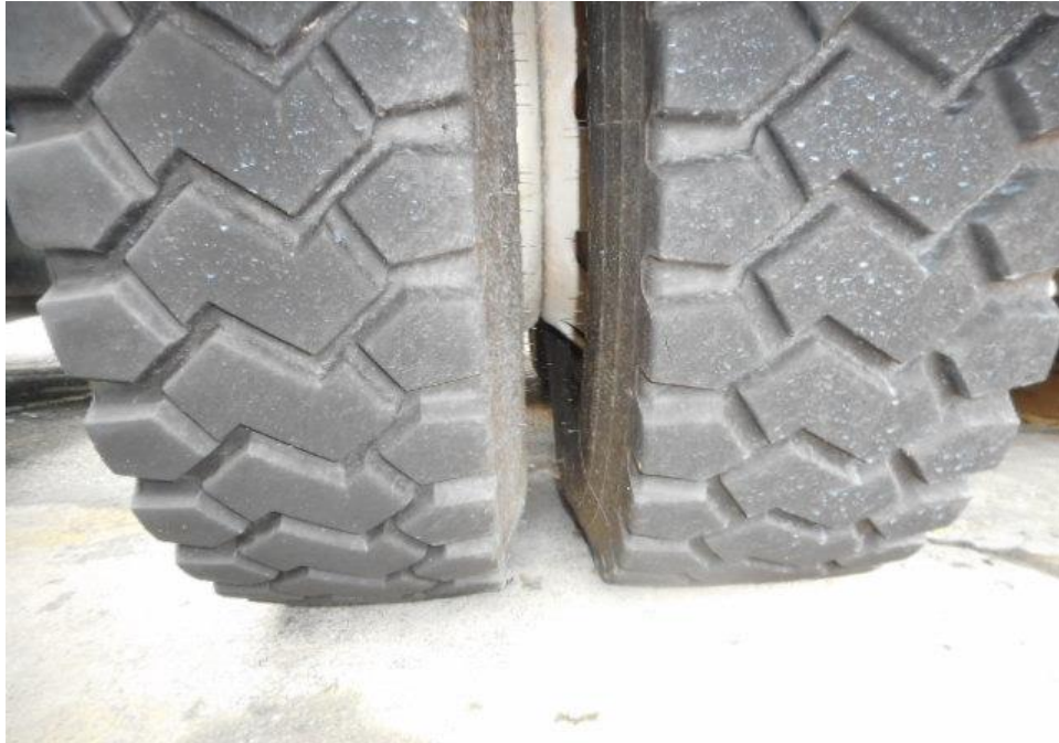
Photo 8 shows the condition of the rear left tyres of the Tipper Truck, which was observed to be in serviceable condition with remaining tread depth of approximately 14.2mm. The tyres, which were wrapped around standard steel wheel rim, were also observed to be sufficiently inflated for vehicular operation. There was also no damage found on all 6 steel wheel rims of the Tipper Truck.
