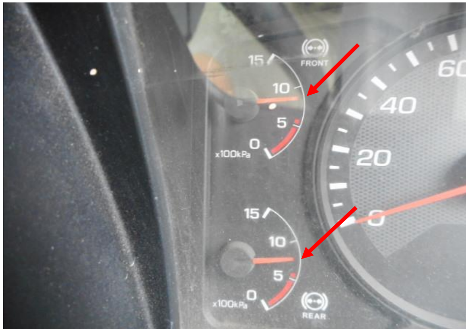
Photo 11 shows the air in the air brake cylinders of the Tipper Truck at the time of my inspection. The air in the cylinder was observed to be of sufficient level & serviceable at the time of the accident.
