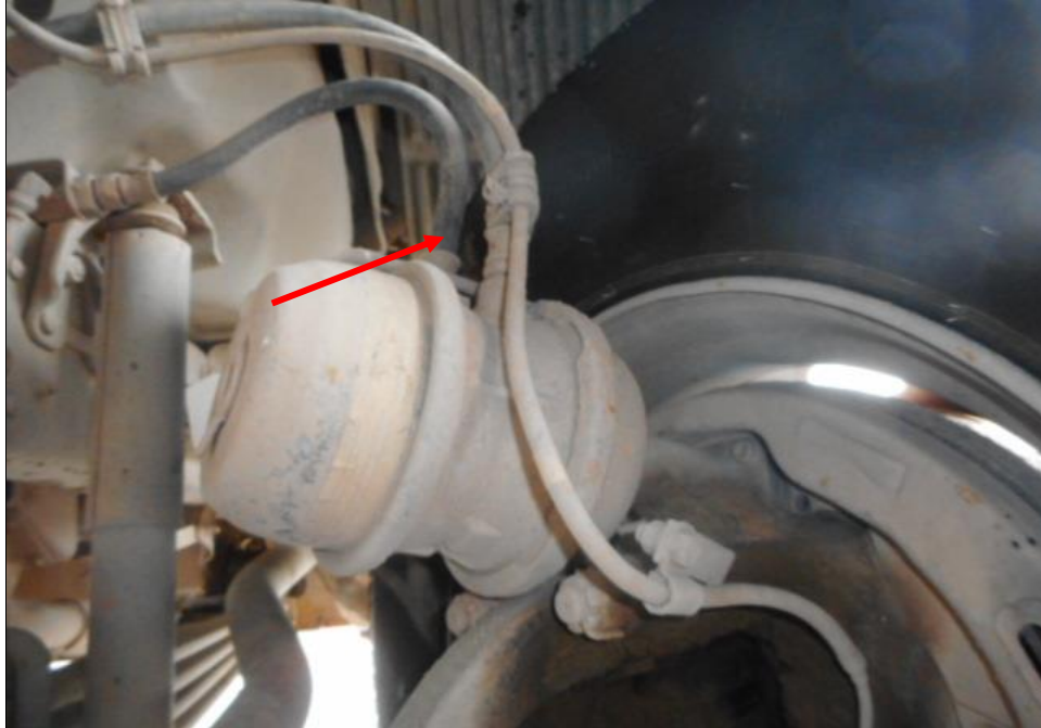
Photo 18 shows the brake pipe (arrowed) at the front right wheel of the Tipper Truck. I did not observe any leakage of brake fluid at the time of my inspection of the Tipper Truck. My static tests of the Tipper Truck's braking system, along with my visual examination of the various mechanical components in the braking system, had indicated that there was no internal leakage of pressure/vacuum. Hence the braking system of the Tipper Truck was likely to be in serviceable condition at the material time of accident.
