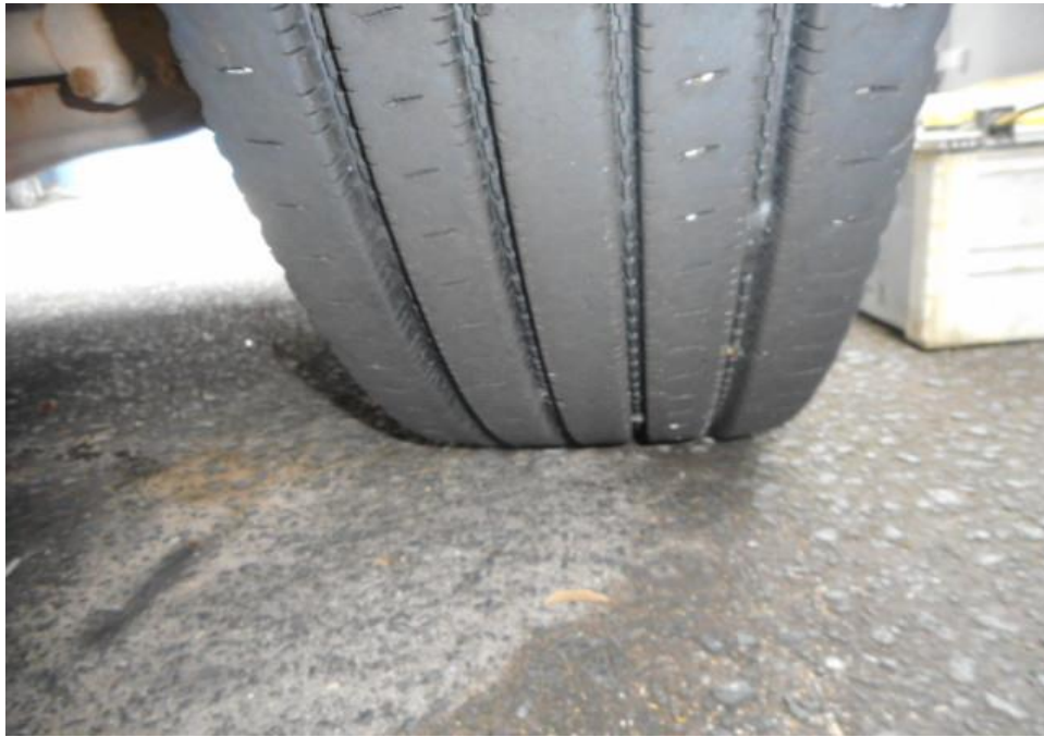
Photo 6 shows the condition of the front right tyre of the Tipper Truck, which was observed to be in serviceable condition with remaining tread depth of approximately 8.9mm. The tyre, which was wrapped around standard steel wheel rim, was also observed to be sufficiently inflated for vehicular operation. There was no tear, cut or burst mark(s) on the outer and the inner sidewalls as well as across the tread of the 6 tyres that were fitted on the Tipper Truck.
