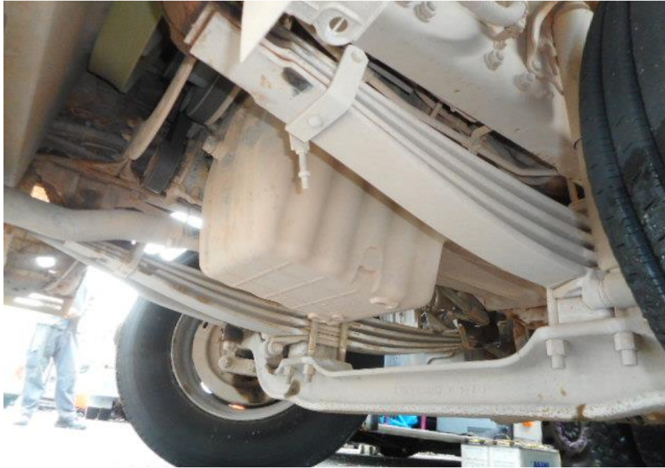
Photo 15 shows the undercarriage of the Tipper Truck, at the area where the engine housing located. I did not find any sign(s) or indication(s) of fluid leak, however old fluid stain(s) was observed on the underside of the Tipper Truck.
