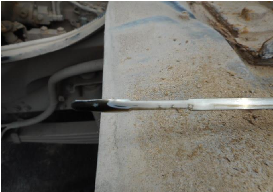
Photo 14 shows the engine oil dip stick of the Tipper Truck at the time of my inspection. The engine oil was observed to be of insufficient level at the time of our inspection.
