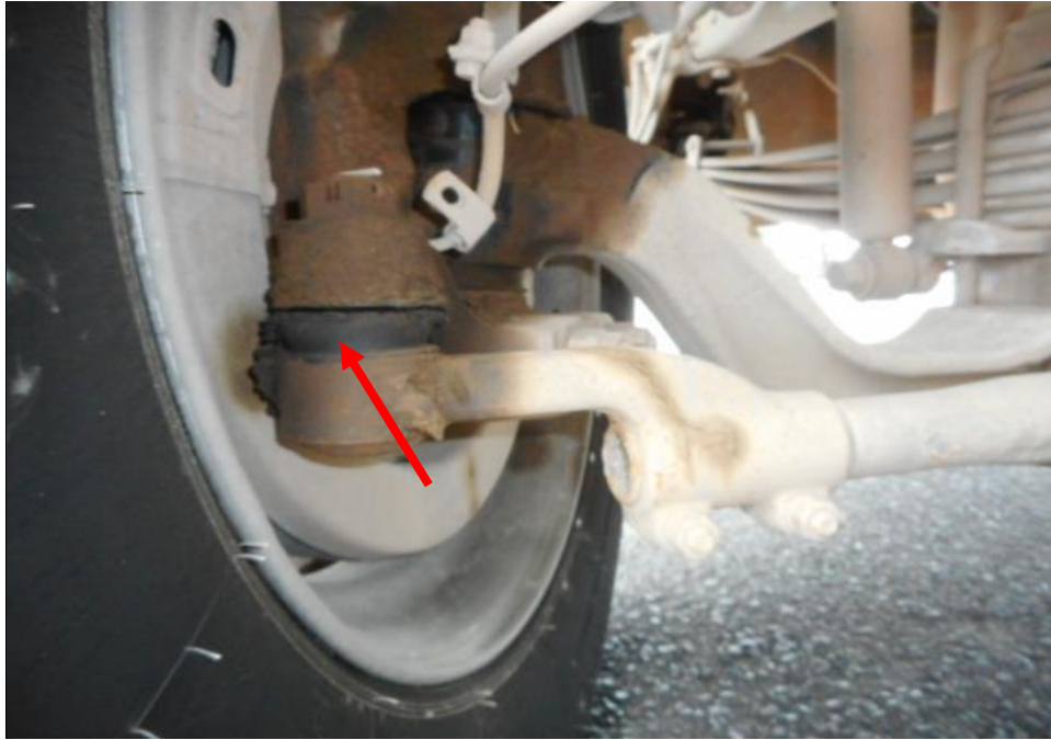
Photo 22 shows the various undercarriage components at the front left wheel of the Tipper Truck, in particular the steering tie rod end (arrowed). The various undercarriage components of the Tipper Truck were all found to be intact without any visible damage. There was also no sign of fluid stain(s) observed on the various undercarriage components.
