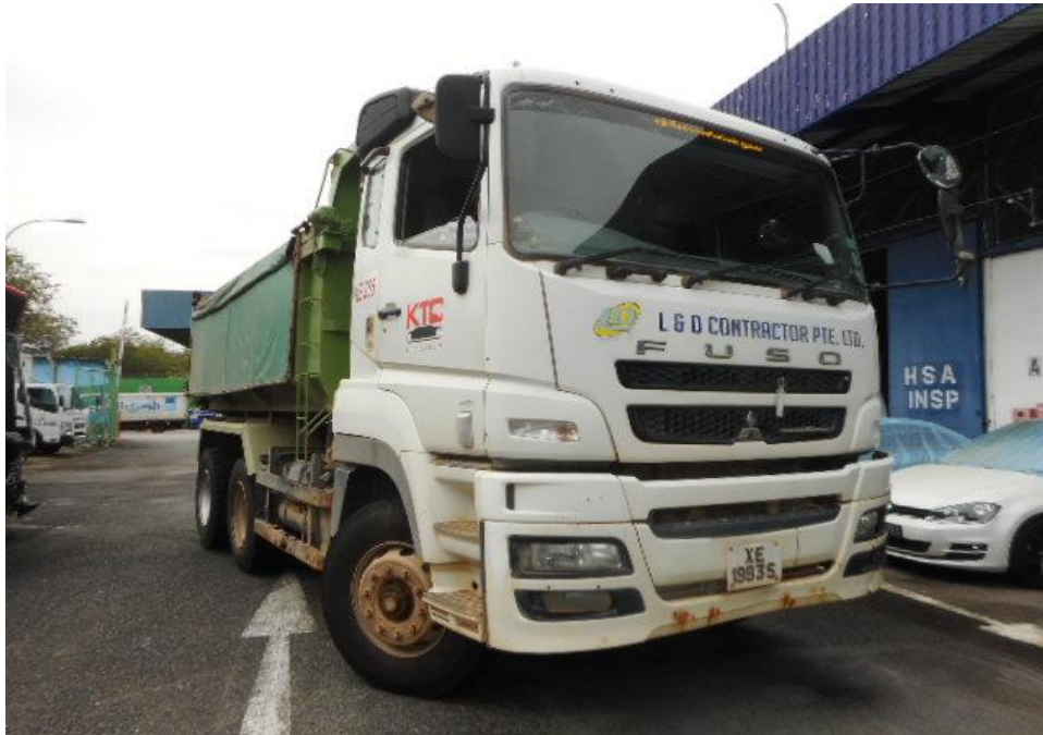
Photo 24 shows the front right wheel of the Tipper Truck turned to its full left. During my steering system test, I did not experience any abnormal free play and/or resistance when I had turned the steering wheel towards full left and full right. This would suggest that the steering system of the Tipper Truck was likely to be in serviceable condition at the material time of accident.
