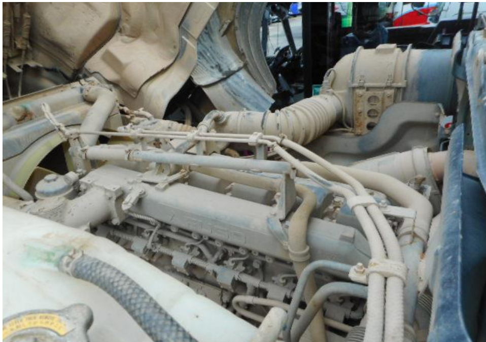
Photo 10 shows a general view of the Tipper Truck's engine compartment, which was accessed by lifting the front cabin of the Tipper Truck. The various parts and components inside the engine compartment were unaffected by the accident. There was also no sign(s) or indication(s) of fresh fluid leakage and/or fluid stain within the engine compartment
