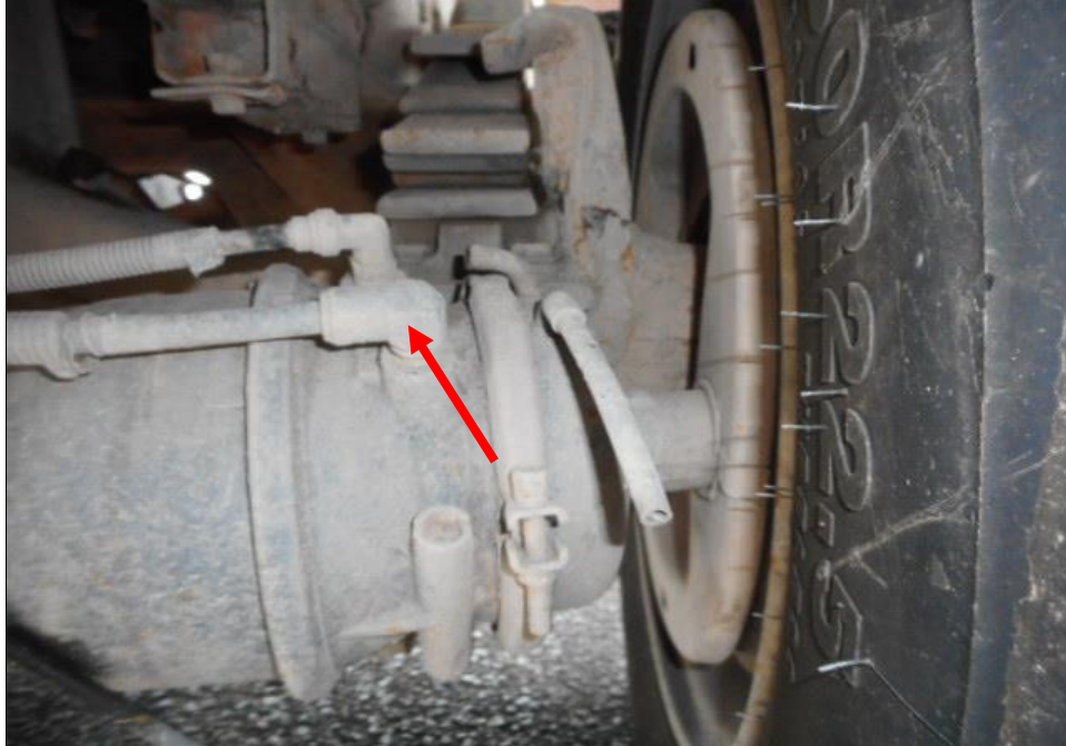
Photo 16 shows the brake pipe (arrowed) at the rear right wheel of the Tipper Truck. I did not observe any leakage of brake fluid at the time of my inspection of the Tipper Truck. My static tests of the Tipper Truck's braking system, along with my visual examination of the various mechanical components in the braking system, had indicated that there was no internal leakage of pressure/vacuum. Hence the braking system of the Tipper Truck was likely to be in serviceable condition at the material time of accident.
