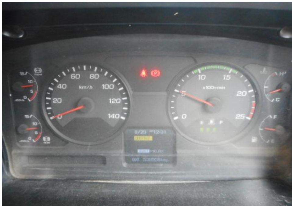
Photo 26 shows the Anti-Lock Braking System (ABS) warning lights had went off on the instrument panel of the Prime Mover after the engine was cranked. This would suggest that there was no abnormality to the electronic operating system of the Prime Mover, like the ABS, and etc.
