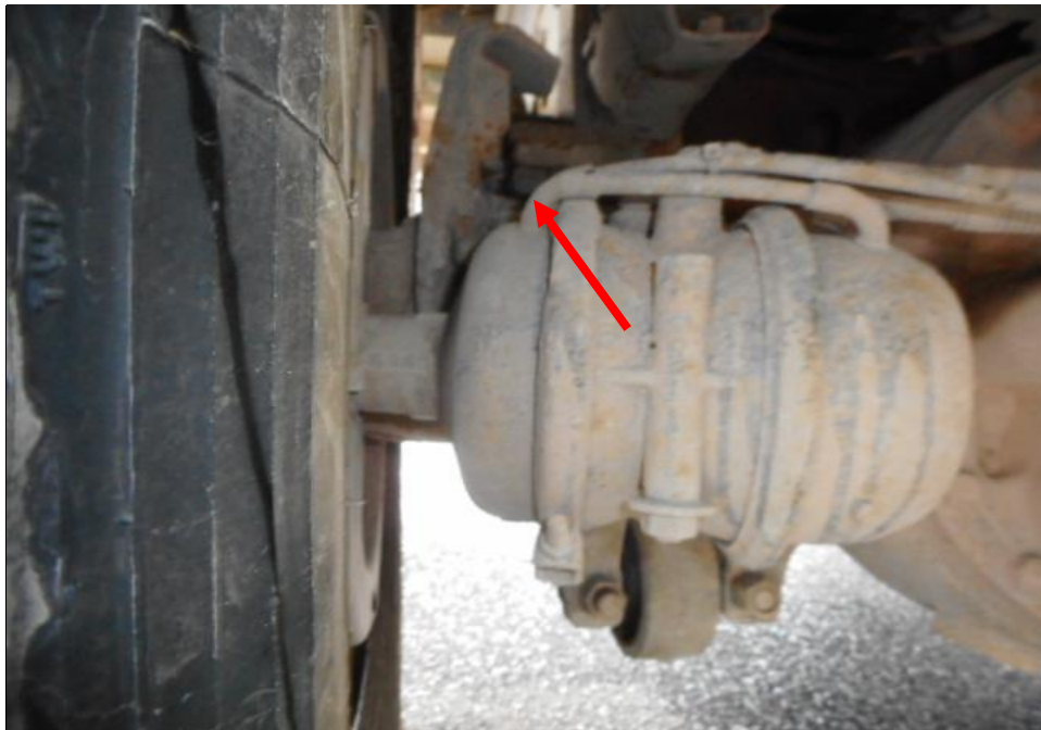
Photo 17 shows the brake pipe (arrowed) at the rear left wheel of the Tipper Truck. I did not observe any leakage of brake fluid at the time of my inspection of the Tipper Truck. My static tests of the Tipper Truck's braking system, along with my visual examination of the various mechanical components in the braking system, had indicated that there was no internal leakage of pressure/vacuum. Hence the braking system of the Tipper Truck was likely to be in serviceable condition at the material time of accident.
