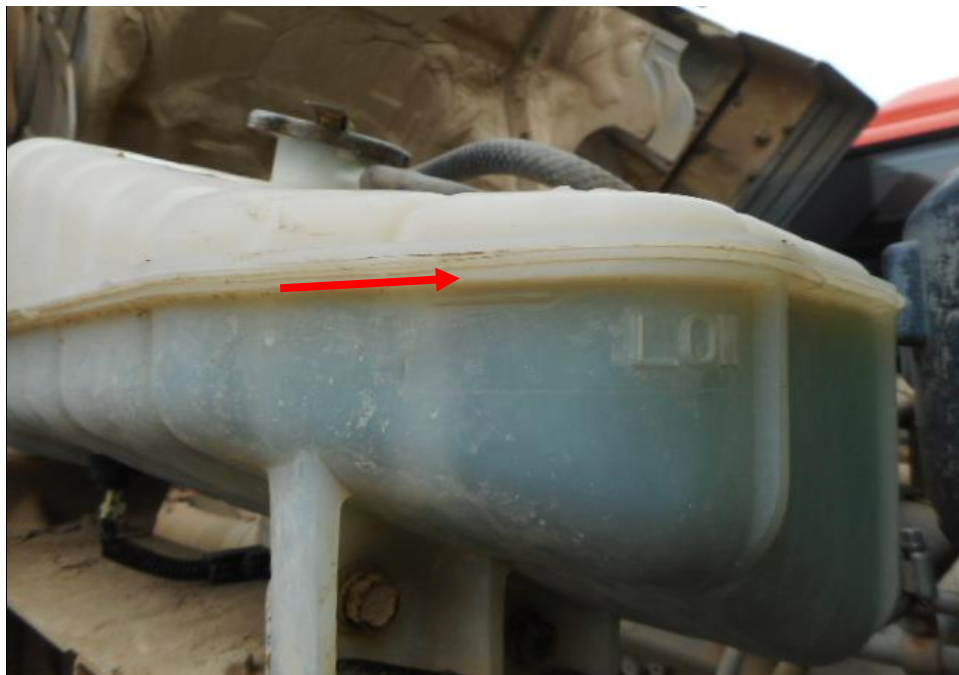
Photo 12 shows the engine coolant reservoir of the Tipper Truck at the time of my inspection. The engine coolant was observed to be of sufficient level (arrowed) and without any visible contamination.
