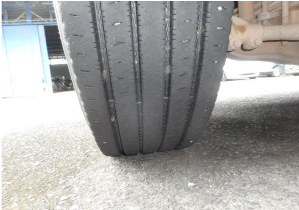
Photo 9 shows the condition of the front left tyres of the Tipper Truck, which were observed to be in serviceable condition with remaining tread depth of approximately 11.8mm. There was also no tear, cut or burst mark(s) on the outer and the inner sidewalls as well as across the tread of the 6 tyres that were fitted on the Tipper Truck.
