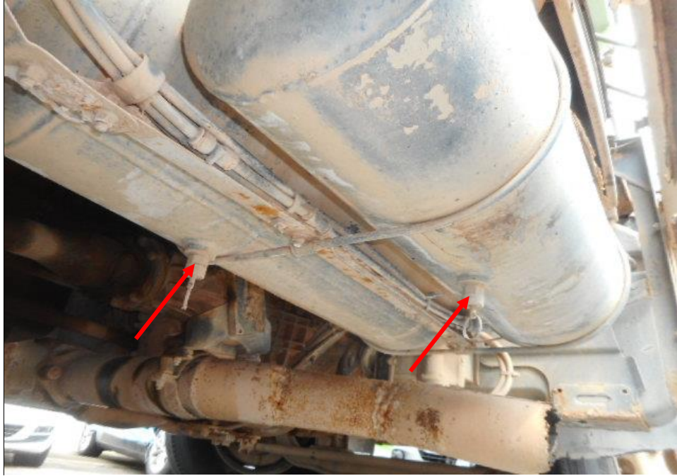
Photo 20 shows the air brake cylinders (arrowed) at the undercarriage of the Tipper Truck. I did not observe any leakage of air brake fluid at the time of my inspection of the Tipper Truck. My static tests of the Tipper Truck's braking system, along with my visual examination of the various mechanical components in the braking system had indicated that there was no internal leakage of pressure/vacuum. Hence the braking system of the Tipper Truck was likely to be in serviceable condition at the material time of accident.
