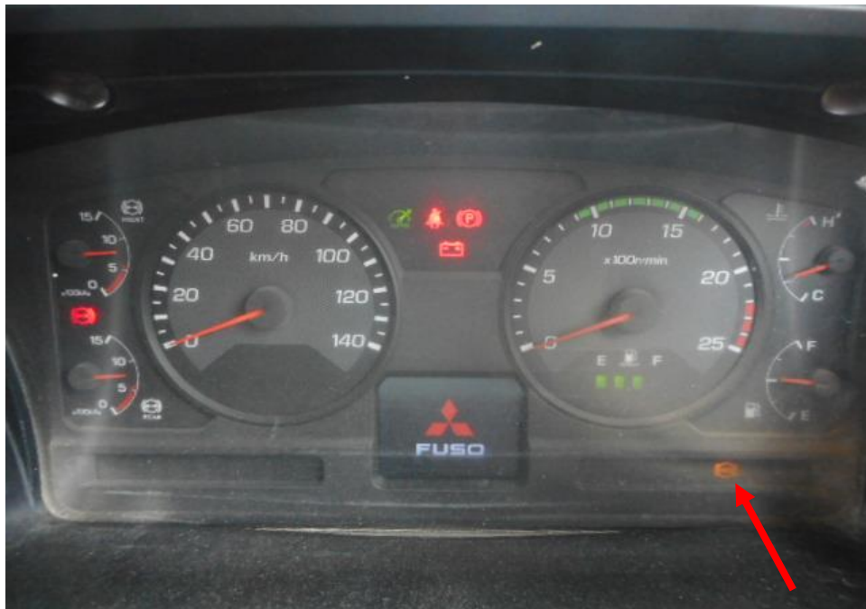
Photo 25 shows the warning light for Anti-Lock Braking System (ABS) (arrowed) appearing on the instrument panel of the Prime Mover during the self-test of its various electronic operating systems when its engine was cranked.
