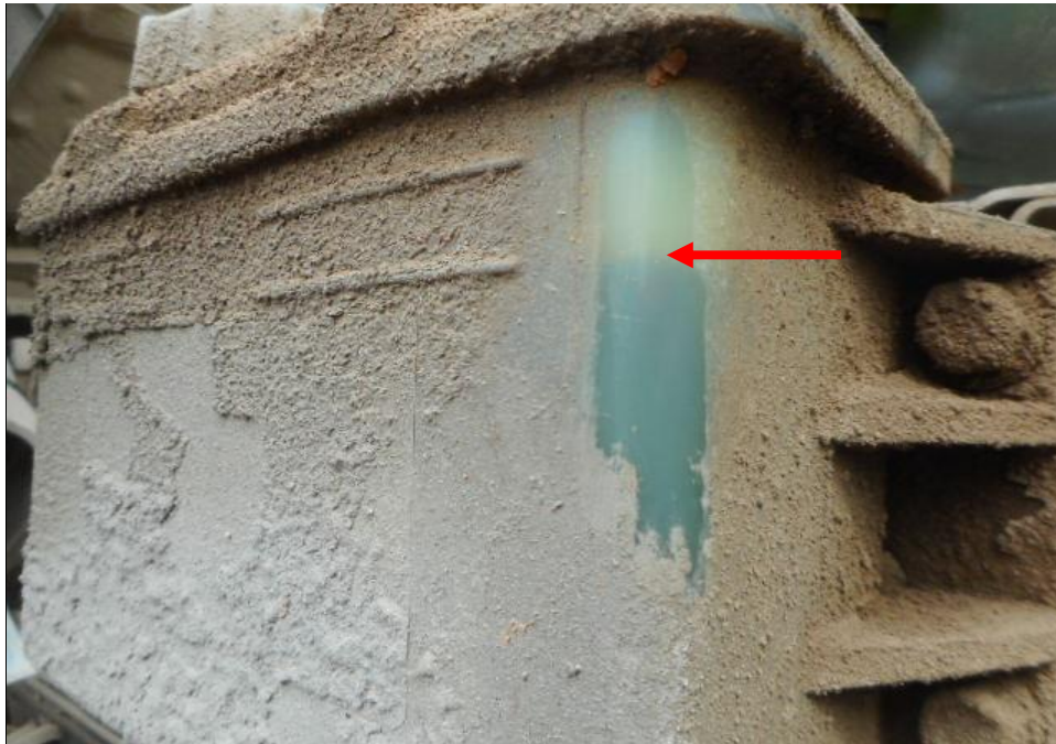
Photo 13 shows the power steering fluid reservoir of the Tipper Truck at the time of my inspection. The power steering fluid was observed to be of sufficient level (arrowed) and without any visible contamination.
