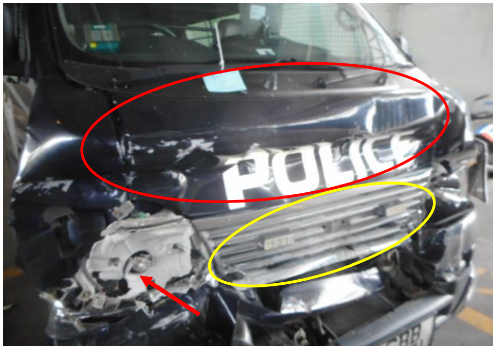
Photo 3 shows a close up view of the Police Van's frontal portion at the time of my inspection. It appeared to have sustained damage at its frontal portion. Its front grille (yellow circle), its front body panel (red circle) and front right headlamp (arrowed) was damaged at the time of my inspection as a result of the accident.
