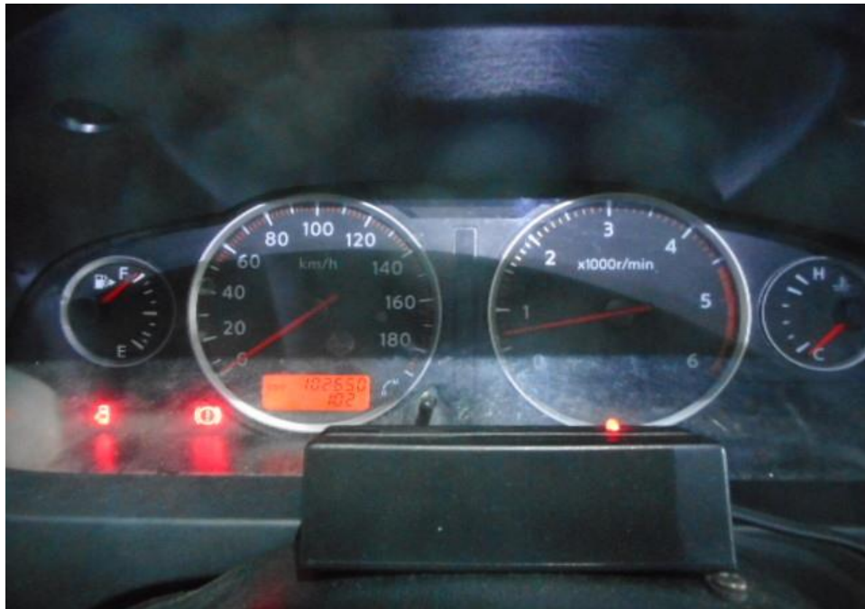
Photo 28 shows no warning lights illuminated on the instrument panel of the Police Van after the engine was cranked. This would suggest that there was no abnormality to the electronic operating system of the Police Van, like the ABS, and etc.
