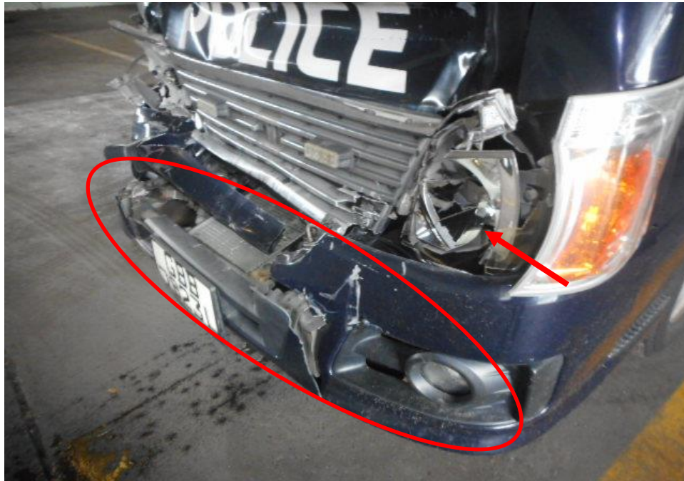
Photo 4 shows a close up view of the Police Van's frontal portion at the time of my inspection. It appeared to have sustained damage at its frontal portion. Its front left headlamp (arrowed) and front bumper (circled) was damaged at the time of my inspection as a result of the accident.
