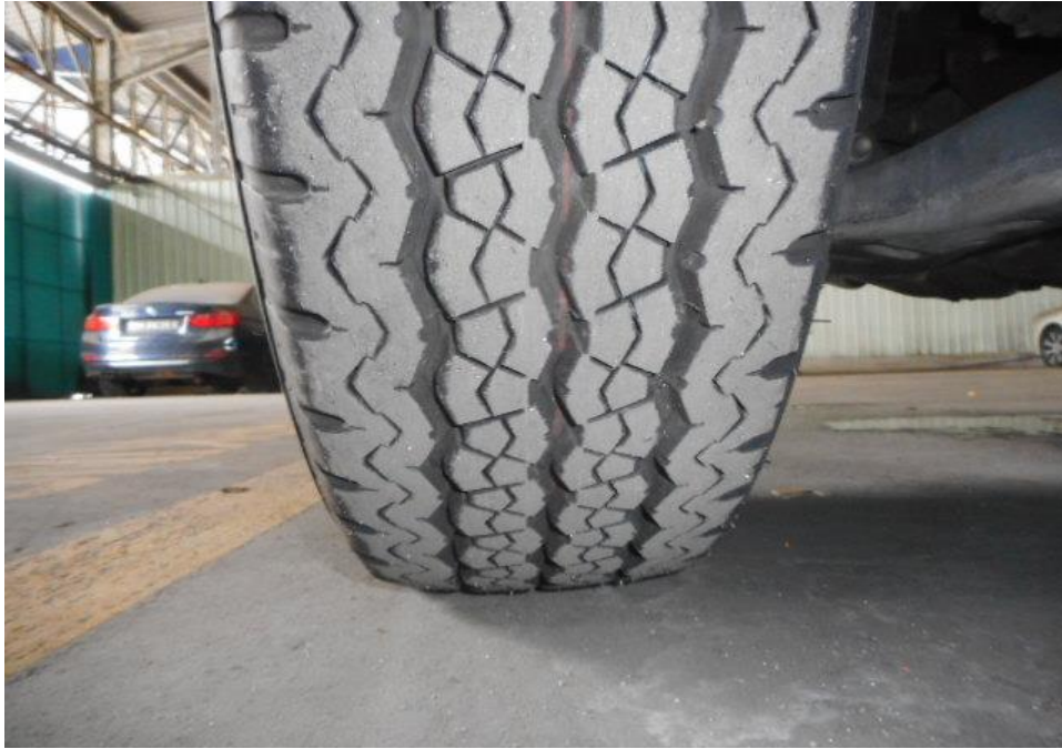
Photo 12 shows the condition of the front left tyres of the Police Van, which was observed to be in serviceable condition with remaining tread depth of approximately 7.7mm. The tyres, which were wrapped around standard steel wheel rim, were also observed to be sufficiently inflated for vehicular operation. There was also no damage found on all 4 steel wheel rims of the Police Van.
