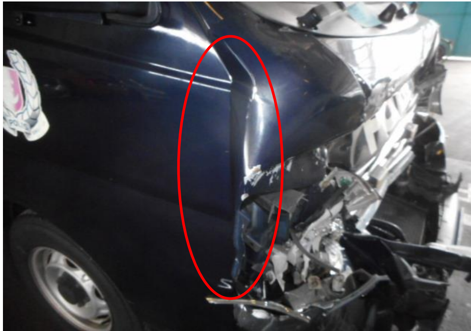
Photo 6 shows a close up view of the right body of the Police Van at the time of my inspection. The front right door (circled) of the Police Van was observed to be damaged as a result of the accident.
