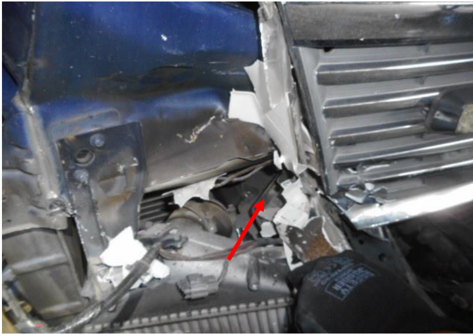
Photo 24 shows the general view of the steering column box (arrowed) at the front portion of the Police Van, it was observed to be damaged as a result of the impact sustained from the accident.
