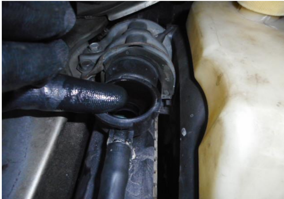
Photo 14 shows the engine coolant of the Police Van at the time of my inspection. The engine coolant was observed to be of sufficient level and without any visible contamination.
