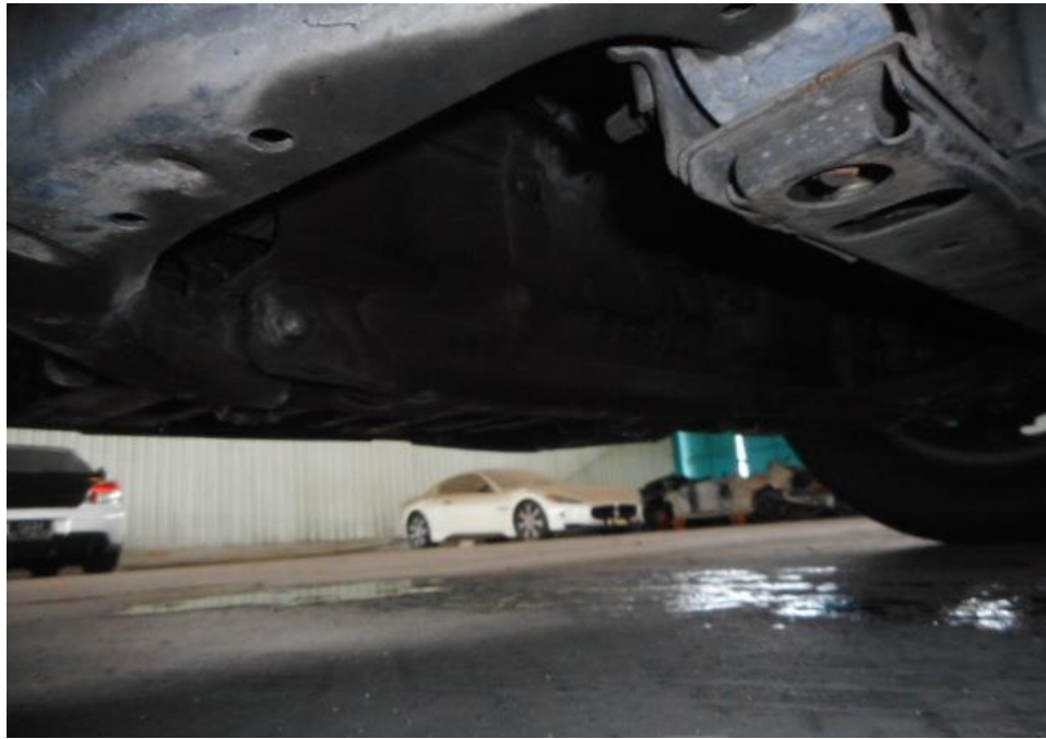
Photo 17 shows the undercarriage of the Police Van, at the area where the engine housing and transmission housing are located. . I did not find any sign(s) or indication(s) of fluid leak and/or fluid stain(s) on the underside of the Police Van.
