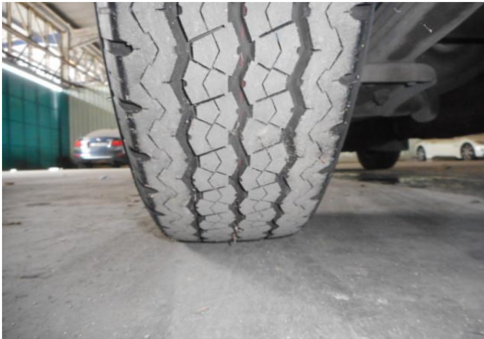
Photo 11 shows the condition of the rear left tyres of the Police Van, which was observed to be in serviceable condition with remaining tread depth of approximately 7.7mm. The tyres, which were wrapped around standard steel wheel rim, were also observed to be sufficiently inflated for vehicular operation. There was also no damage found on all 4 steel wheel rims of the Police Van.
