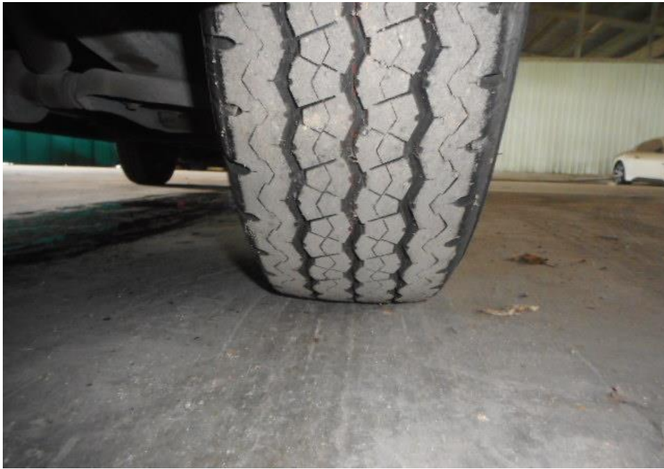
Photo 10 shows the condition of the rear right tyre of the Police Van, which was observed to be in serviceable condition with remaining tread depth of approximately 7.3mm. The tyre, which was wrapped around standard steel wheel rim, it was observed to be sufficiently inflated for vehicular operation.
