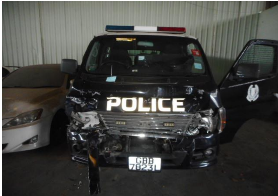
Photo 2 shows a general view of the Police Van's frontal portion at the time of my inspection. It appeared to have sustained damage at its frontal portion. Its front body panel, front grille, front bumper, both front left headlamp and its front right door were observed to be damaged at the time of my inspection.
