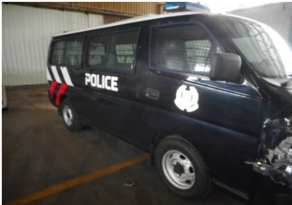
Photo 5 shows a general view of the right body of the Police Van at the time of my inspection. The front right door of the Police Van was observed to be damaged as a result of the accident.
