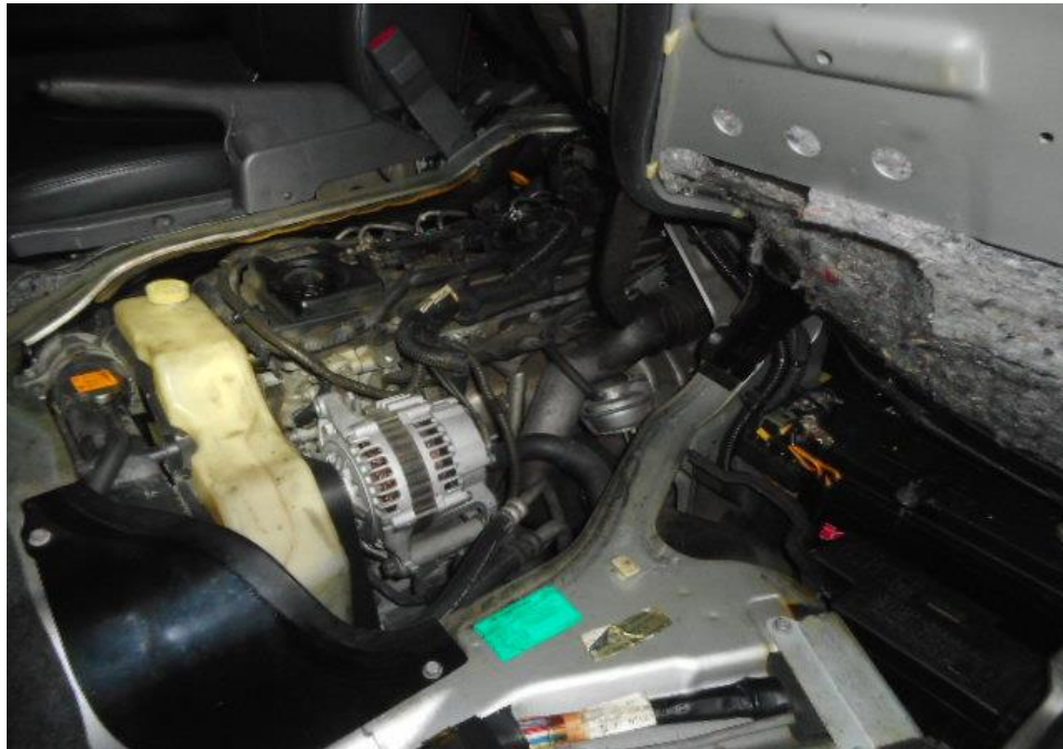
Photo 13 shows a general view of the Police Van's engine compartment, which was accessed by lifting the front cabin of the Police Van. The various parts and components inside the engine compartment were unaffected by the accident. There was also no sign(s) or indication(s) of fresh fluid leakage and/or fluid stain within the engine compartment
