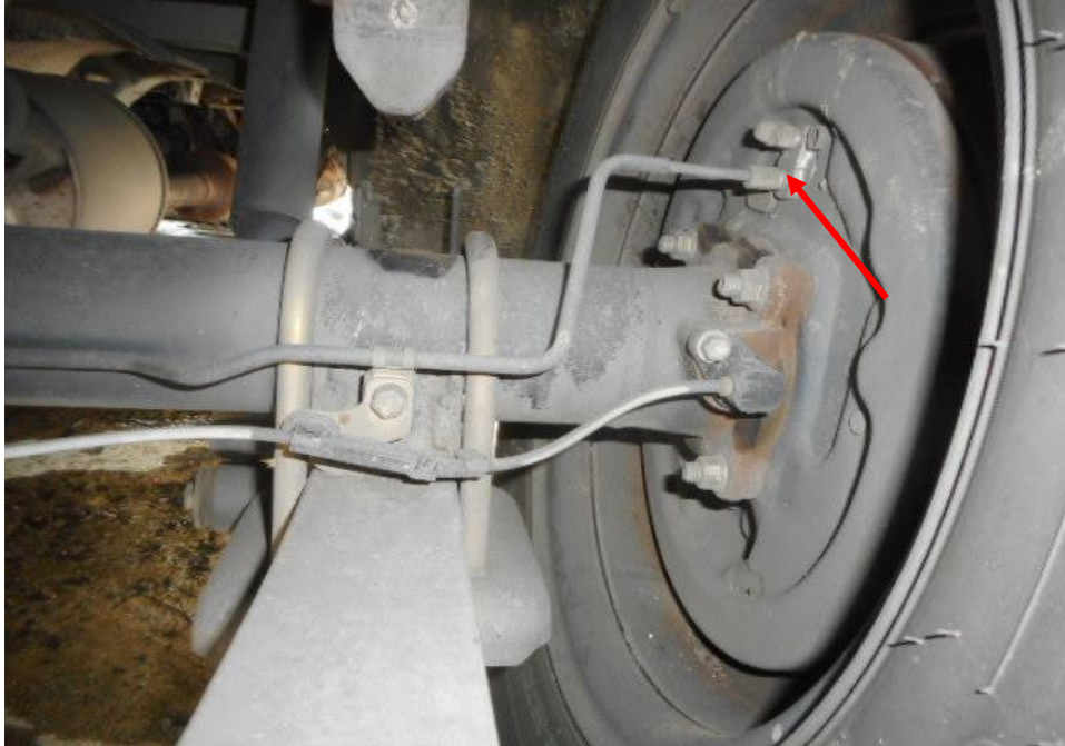
Photo 20 shows the brake pipe (arrowed) at the rear right wheel of the Police Van. I did not observe any leakage of brake fluid at the time of my inspection of the Police Van. My static tests of the Police Van's braking system, along with my visual examination of the various mechanical components in the braking system, had indicated that there was no internal leakage of pressure/vacuum. Hence the braking system of the Police Van was likely to be in serviceable condition at the material time of accident.
