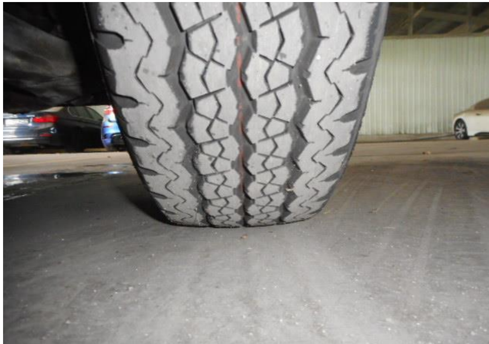
Photo 9 shows the condition of the front right tyre of the Police Van, which was observed to be in serviceable condition with remaining tread depth of approximately 7.7mm. The tyre, which was wrapped around standard steel wheel rim, was also observed to be sufficiently inflated for vehicular operation. There was no tear, cut or burst mark(s) on the outer and the inner sidewalls as well as across the tread of the 4 tyres that were fitted on the Police Van.
