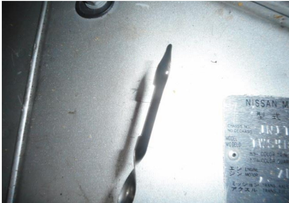
Photo 15 shows the engine oil dip stick of the Police Van at the time of my inspection. The engine oil was observed to be of sufficient level and without any visible contamination.
