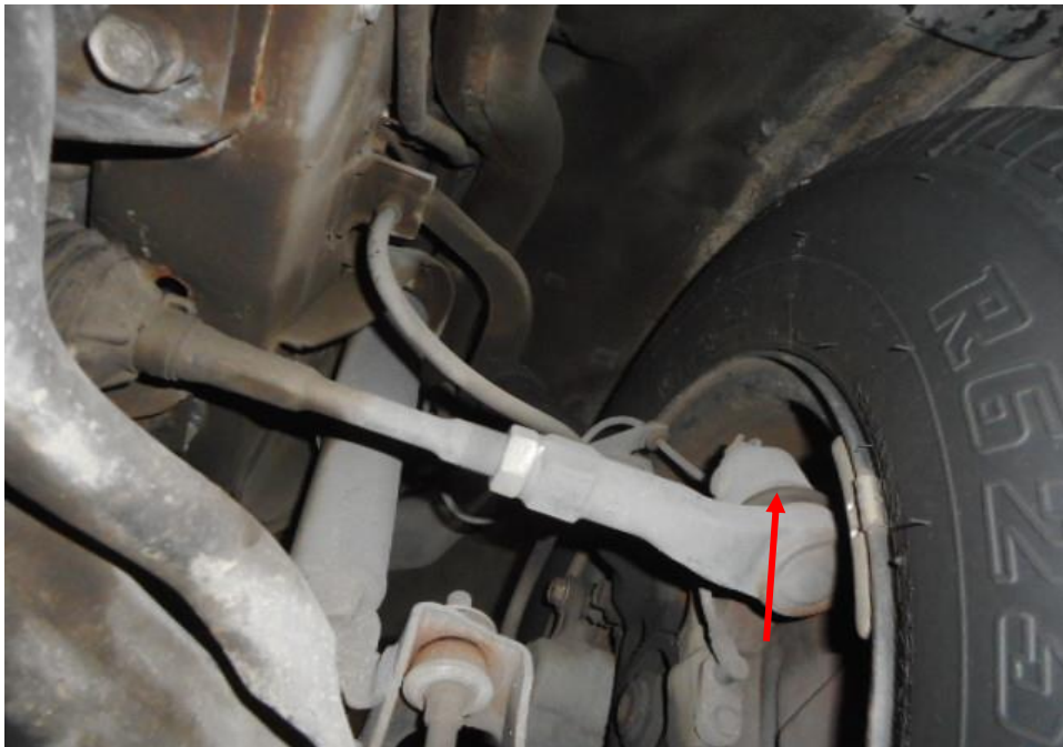
Photo 19 shows the various undercarriage components at the front left wheel of the Police Van, in particular the steering tie rod end (red arrow). The various steering components were all found to be intact. There was also no sign of fluid stain(s) observed on the various undercarriage components.
