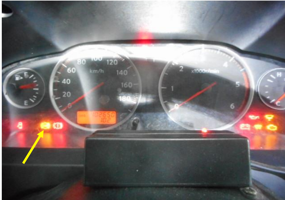
Photo 27 shows the warning light for Anti-Lock Braking System (ABS) (arrowed) appearing on the instrument panel of the Police Van during the self-test of its various electronic operating systems when its engine was cranked.
