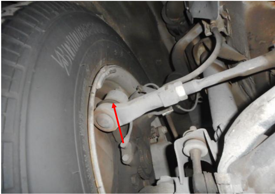
Photo 18 shows the various undercarriage components at the front right wheel of the Police Van, in particular the steering tie rod end (red arrow). The various steering components were all found to be intact. There was also no sign of fluid stain(s) observed on the various undercarriage components.
