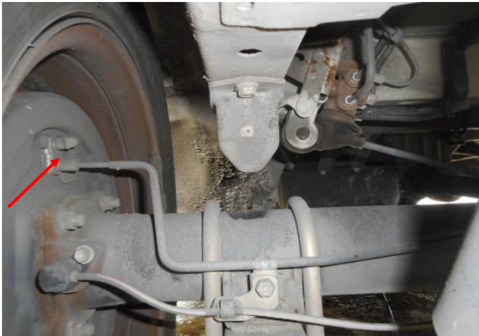
Photo 21 shows the brake pipe (arrowed) at the rear left wheel of the Police Van. I did not observe any leakage of brake fluid at the time of my inspection of the Police Van. My static tests of the Police Van's braking system, along with my visual examination of the various mechanical components in the braking system had indicated that there was no internal leakage of pressure/vacuum. Hence the braking system of the Police Van was likely to be in serviceable condition at the material time of accident.
