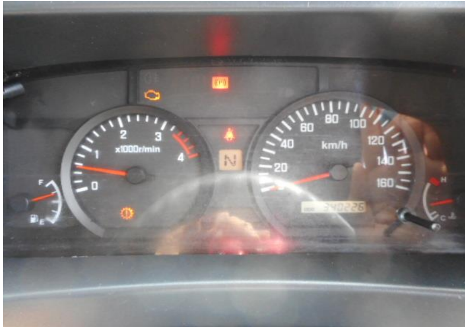
Photo 27 shows no warning lights illuminated on the instrument panel of the Motor Lorry after the engine was cranked. This would suggest that there was no abnormality to the electronic operating system of the Motor Lorry, like the ABS, ASR, SRS etc.
