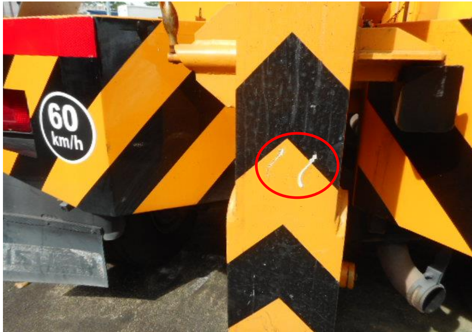
Photo 3 shows a close up view of the Motor Lorry's rear portion at the time of my inspection. Its rear tow fork (circled) was damage at the time of my inspection as a result of the accident.
