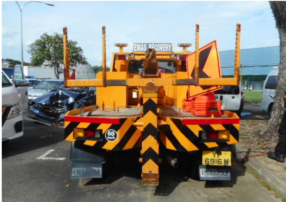
Photo 2 shows a general view of the Motor Lorry's rear portion at the time of my inspection. It appeared to have sustained damage at its rear portion. Its rear tow fork was damage at the time of my inspection as a result of the accident.
