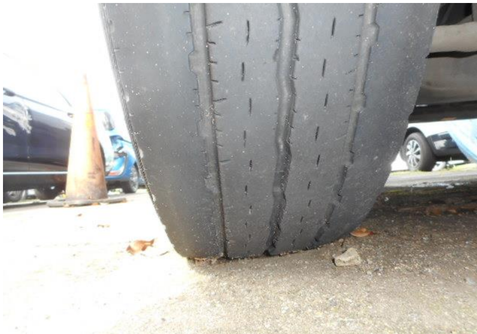
Photo 11 shows the condition of the rear right tyres of the Motor Lorry, which were observed to be in serviceable condition with remaining tread depth of approximately 5.7mm. There was also no tear, cut or burst mark(s) on the outer and the inner sidewalls as well as across the tread of the 6 tyres that were fitted on the Motor Lorry.
