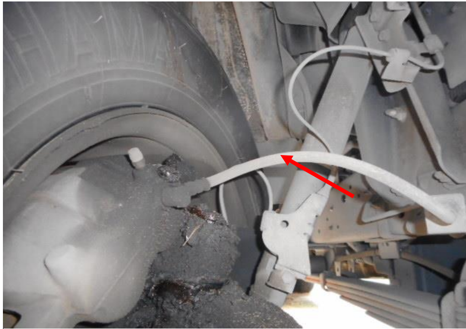
Photo 24 shows the brake hose/pipe (arrowed) at the front left wheel of the Motor Lorry. No leakage of brake fluid was observed. Visual examination of the various components of the braking system like the brake caplier, brake booster, brake pedal etc had revealed all to be intact and without visible damage at the time of accident. There was sign of old fluid stain(s) observed on the various undercarriage components.
