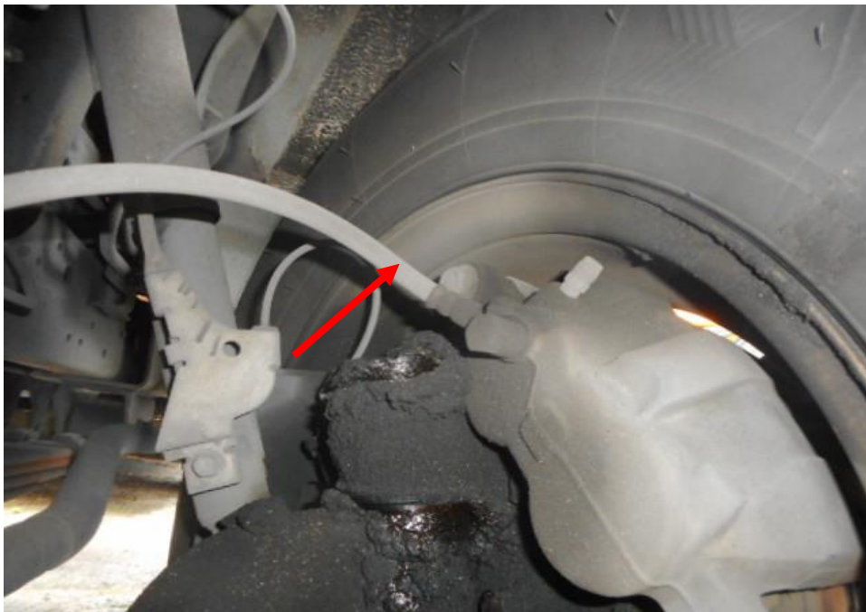
Photo 23 shows the brake hose/pipe (arrowed) at the front right wheel of the Motor Lorry. No leakage of brake fluid was observed. Visual examination of the various components of the braking system like the brake caliper, brake booster, brake pedal etc had revealed all to be intact and without visible damage at the time of accident. There was also no sign of fluid stain(s) observed on the various undercarriage components.
