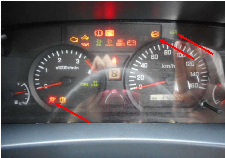
Photo 26 shows the warning light for Anti-Lock Braking System (ABS) and Supplemental Restraint System (SRS) (arrowed) appearing on the instrument panel of the Motor Lorry during the self-test of its various electronic operating systems when its engine was cranked.
