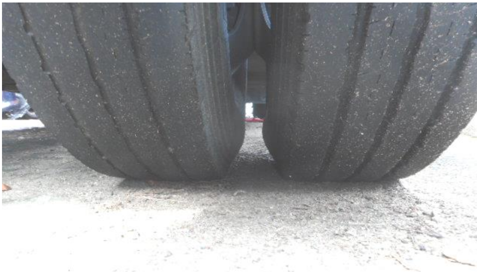
Photo 8 shows the condition of the front right tyre of the Motor Lorry, which was observed to be in serviceable condition with remaining tread depth of approximately 3mm. The tyre, which was wrapped around standard steel wheel rim, was also observed to be sufficiently inflated for vehicular operation. There was no tear, cut or burst mark(s) on the outer and the inner sidewalls as well as across the tread of the 6 tyres that were fitted on the Motor Lorry.
