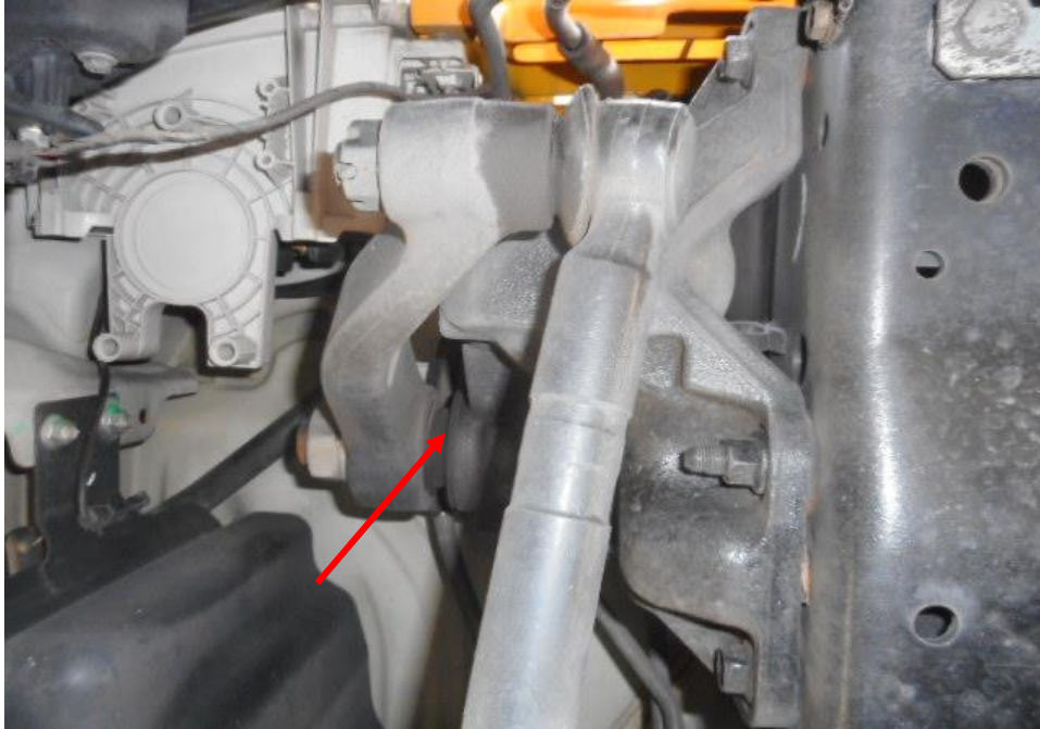
Photo 20 shows the various undercarriage components at the front right wheel of the Motor Lorry, in particular the steering box (arrowed). The various undercarriage components of the Motor Lorry were all found to be intact without any visible damage. There was also no sign of fluid stain(s) observed on the various undercarriage components.
