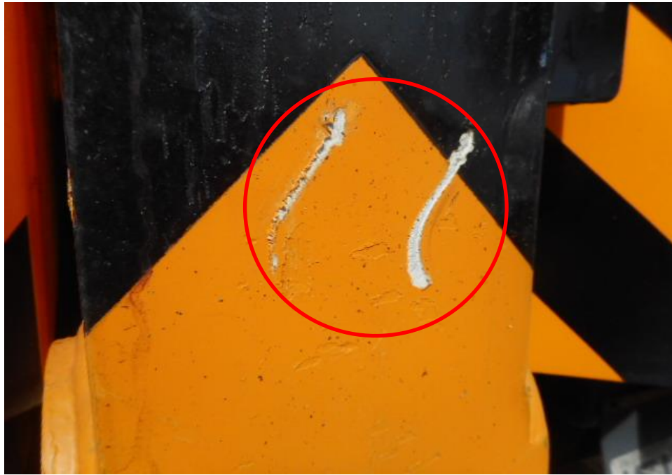
Photo 4 shows a close up view of the Motor Lorry's rear portion at the time of my inspection. Its rear tow fork (circled) was damage at the time of my inspection as a result of the accident.
