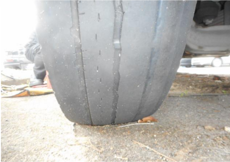
Photo 8 shows the condition of the front right tyre of the Motor Lorry, which was observed to be in serviceable condition with remaining tread depth of approximately 3mm. The tyre, which was wrapped around standard steel wheel rim, was also observed to be sufficiently inflated for vehicular operation. There was no tear, cut or burst mark(s) on the outer and the inner sidewalls as well as across the tread of the 6 tyres that were fitted on the Motor Lorry.
