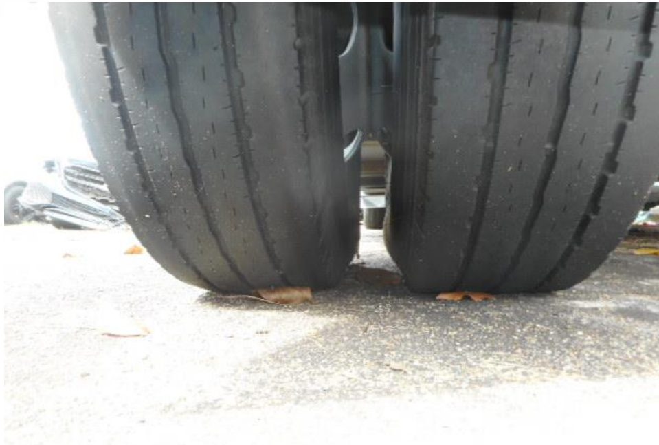
Photo 10 shows the condition of the rear left tyres of the Motor Lorry, which was observed to be in serviceable condition with remaining tread depth of approximately 4.2mm. The tyres, which were wrapped around standard steel wheel rim, were also observed to be sufficiently inflated for vehicular operation.
