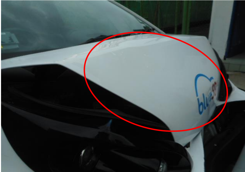
Photo 3 shows the close up view of the Motor Car's front body at the time of my inspection. The Motor Car was observed to have sustained damage at its front portion. Its front bonnet (circled) were amongst the body parts that were damaged as a result of the accident.
