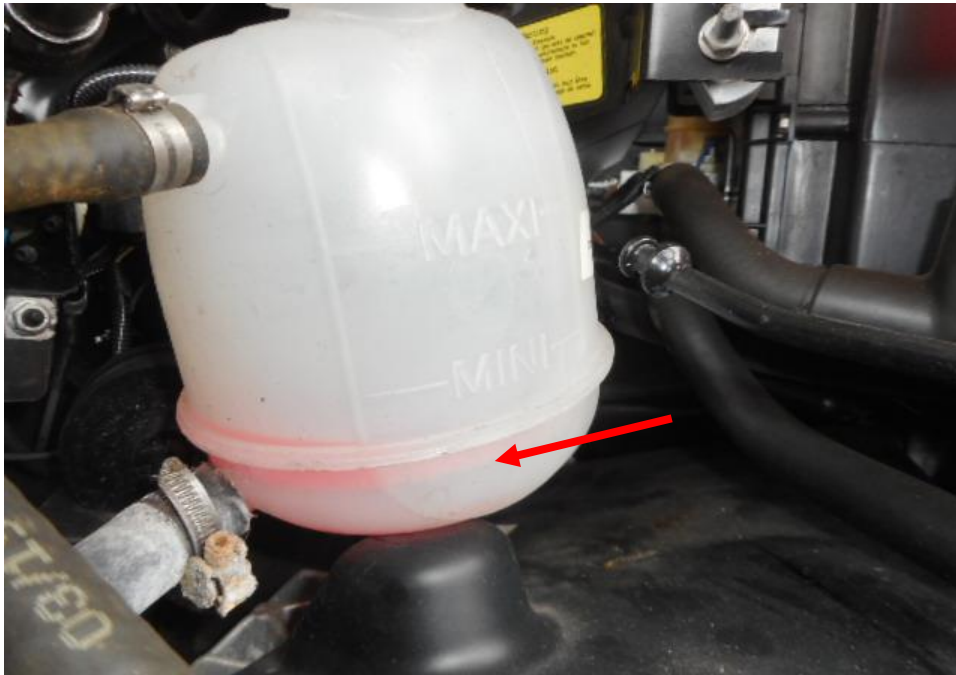
Photo 13 shows the coolant reservoir of the Motor Car at the time of my inspection. The coolant fluid was observed to be of insufficient level (arrowed) due to the damaged radiator as a result of the accident.
