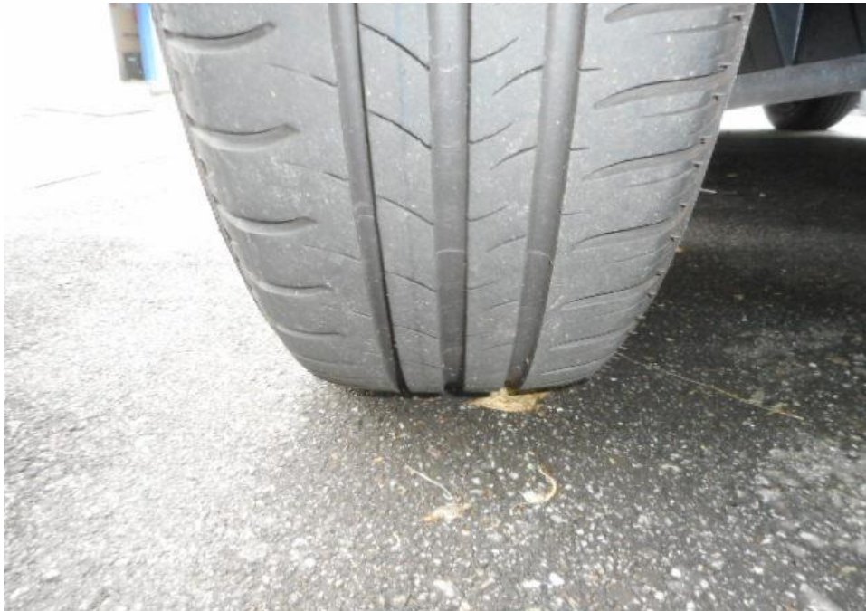
Photo 9 shows the condition of the rear left tyre of the Motor Car, which was observed to be in serviceable condition with remaining tread depth of approximately 5.5mm. The tyre, which was wrapped around standard steel wheel rim, was also observed to be sufficiently inflated for vehicular operation.
