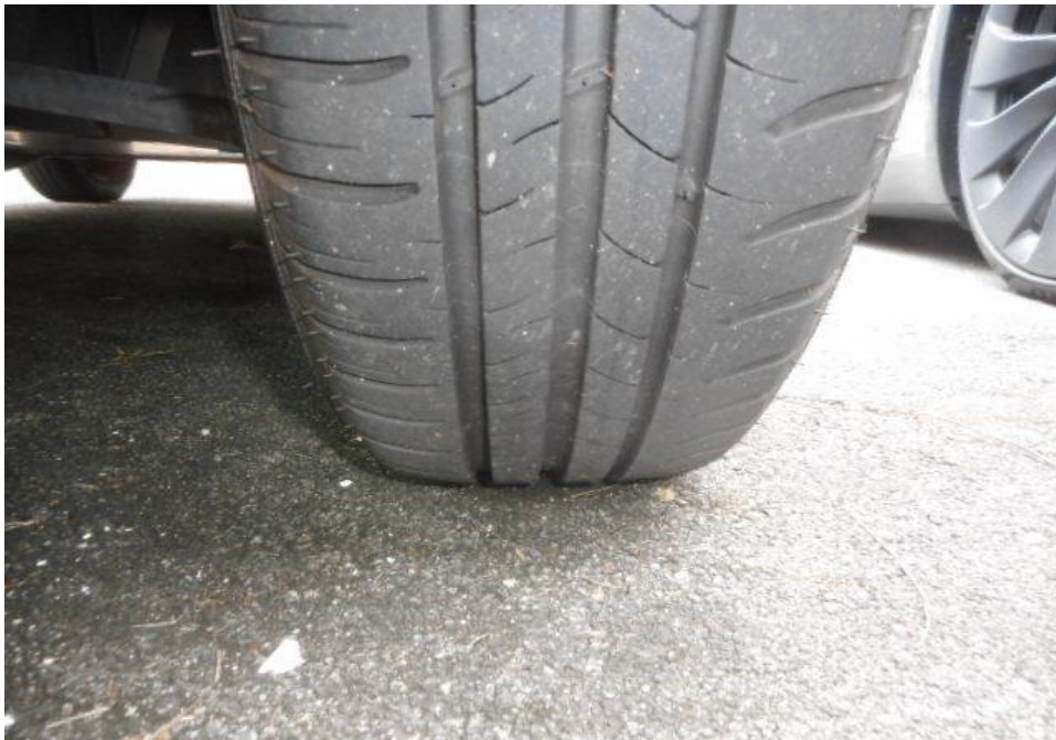
Photo 8 shows the condition of the rear right tyre of the Motor Car, which was observed to be in serviceable condition with remaining tread depth of approximately 5.9mm. The tyre, which was wrapped around standard steel wheel rim, was also observed to be sufficiently inflated for vehicular operation.
