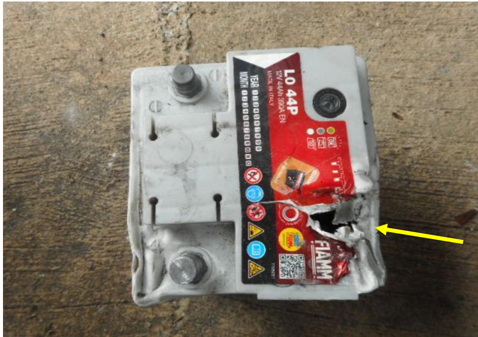
Photo 15 shows checks being carried out to the original 12V battery of the Motor Car at the time of my inspection. The 12V battery was observed to be pieced by the bend coolant radiator as result of the induced impact from the accident (arrowed).
