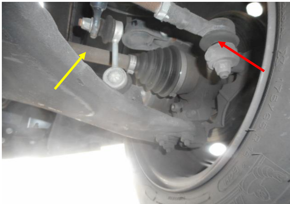
Photo 24 shows the various undercarriage components at the front right wheel of the Motor Car, in particular the steering tie rod (red arrow) and its driveshaft (yellow arrow). The various steering components were all found to be intact. There was also no sign of fluid stain observed on the various undercarriage components at the front right wheel of the Motor Car.
