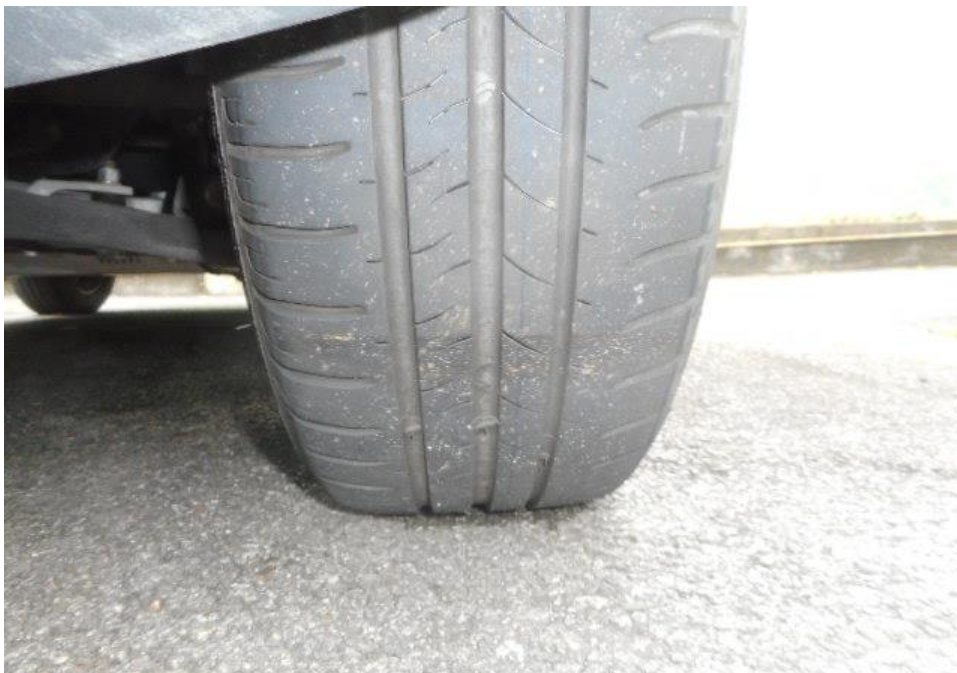
Photo 10 shows the condition of the front left tyre of the Motor Car, which was observed to be in serviceable condition with remaining tread depth of approximately 3.8mm. The tyre, which was wrapped around standard steel wheel rim, was also observed to be sufficiently inflated for vehicular operation.
