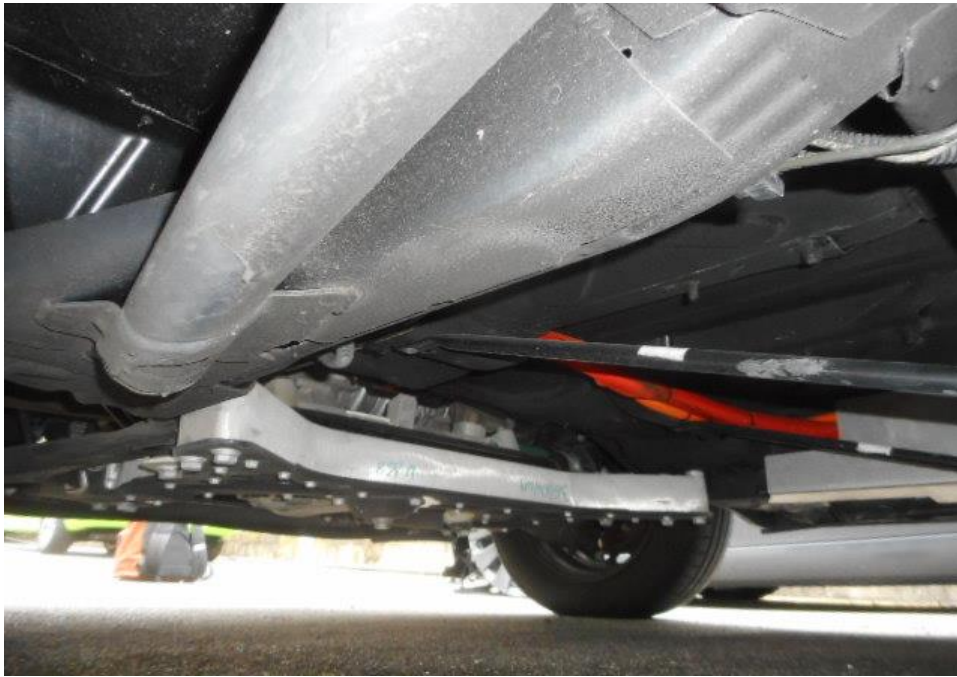
Photo 19 shows the undercarriage of the Motor Car, at the area where the electric motor housing and transmission housing are located. I did not find any sign(s) or indication(s) of fluid leak and/or fluid stain(s) on the underside of the Motor Car.
