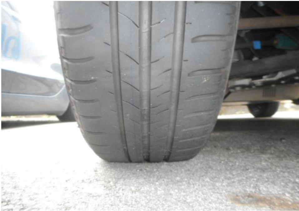
Photo 7 shows the condition of the front right tyre of the Motor Car, which was observed to be in serviceable condition with remaining tread depth of approximately 4.4mm. The tyre, which was wrapped around alloy wheel rim, was also observed to be sufficiently inflated for vehicular operation.
