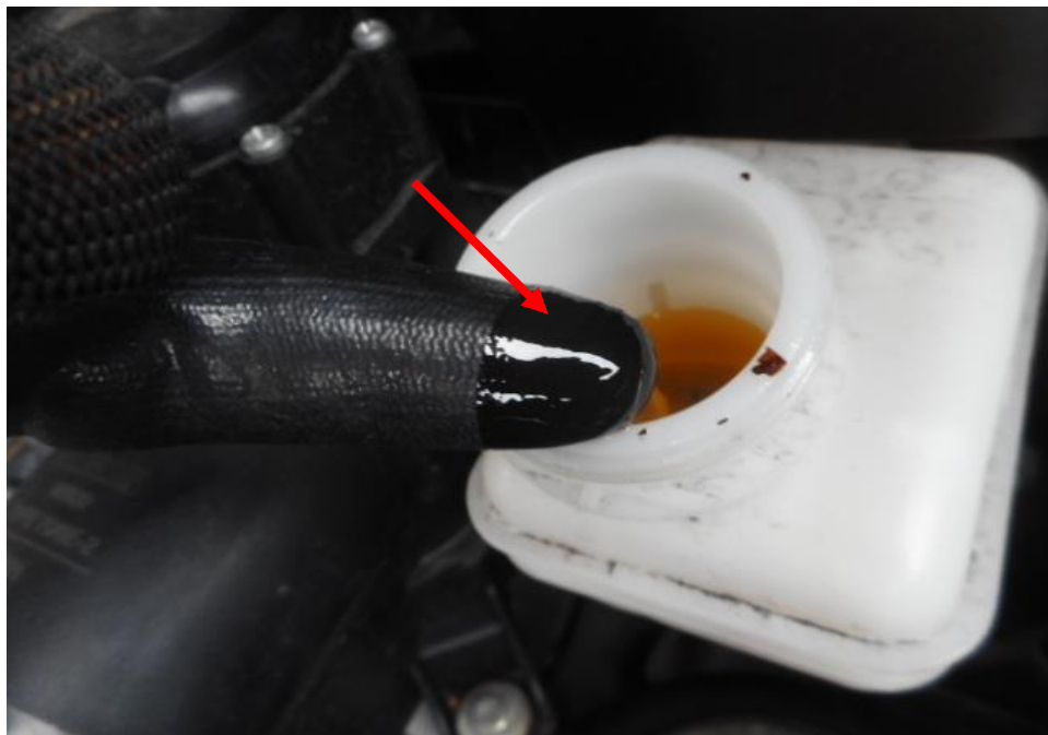
Photo 18 shows the brake fluid reservoir of the Motor Car at the time of my inspection. The brake fluid was observed to be of sufficient level (arrowed) and without any visible contamination.
