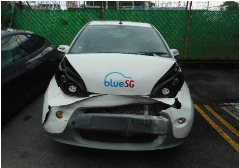
Photo 2 shows a general view of the Motor Car's front body at the time of my inspection. The Motor Car was observed to have sustained damage at its front portion. Its front bonnet, front body panel and front bumper were amongst the body parts and various engine components were damaged as a result of the accident.
