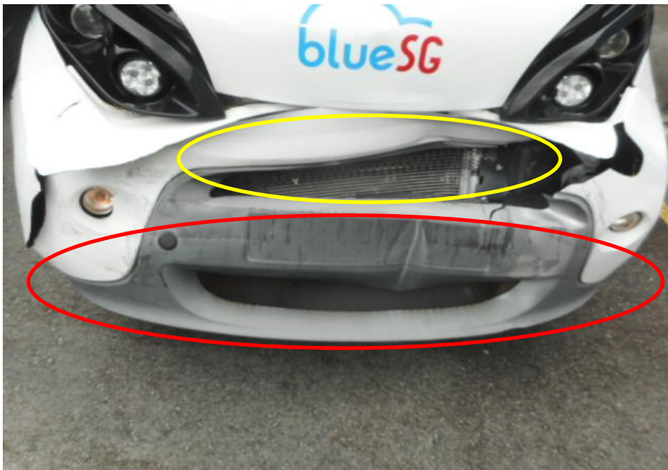
Photo 4 shows the close up view of the Motor Car's front body at the time of my inspection. The Motor Car was observed to have sustained damage at its front portion. Its front bumper (red circle) and front body panel (yellow circle) were amongst the body parts that were damaged as a result of the accident.
