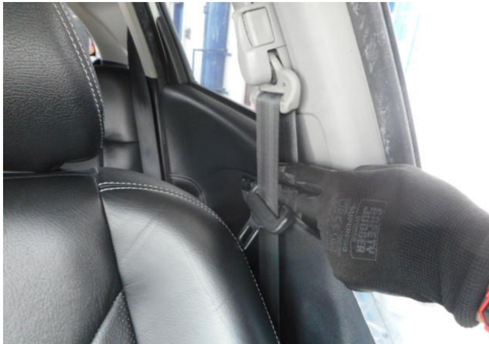
Photo 25 shows that the seat belt on the left seat was not worn at the material time of accident as the safety pre-tensioners was activated at the moment of impact and caused the seat belt to be locked into the last position.
