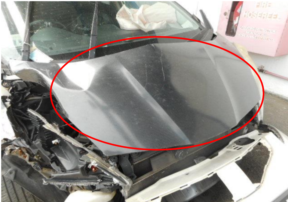
Photo 2 shows the close up view of the Motor Car's front body at the time of my inspection. The Motor car was observed to have sustained damage at its front portion. Its front bonnet (circled) was damaged as a result of the accident.
