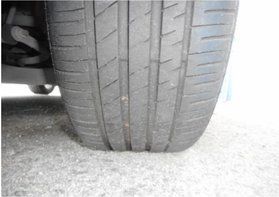
Photo 11 shows the condition of the front left tyre of the Motor Car, which was observed to be in serviceable condition with remaining tread depth of approximately 5.2mm. The tyre was also observed to be sufficiently inflated for vehicular operation with no tear, cut or burst mark(s).
