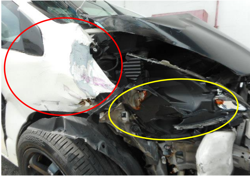
Photo 3 shows the close up view of the Motor Car's front body at the time of my inspection. The Motor car was observed to have sustained damage at its front portion. Its front right fender (red circle) and front right headlamp (yellow circle) was damaged as a result of the accident.
