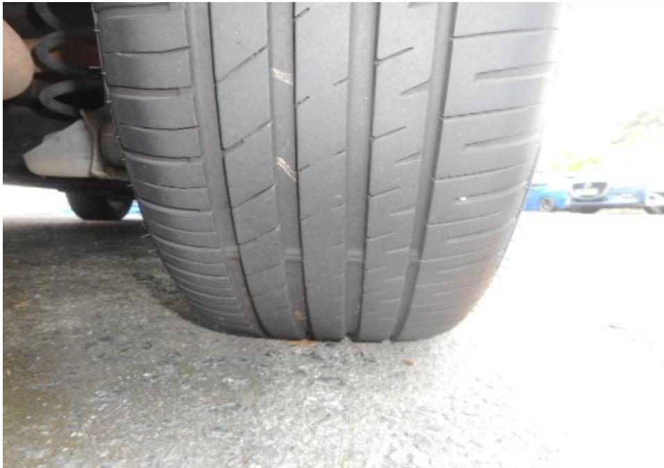
Photo 9 shows the condition of the rear right tyre of the Motor Car, which was observed to be in serviceable condition with remaining tread depth of approximately 4.8mm. The tyre was also observed to be sufficiently inflated for vehicular operation with no tear, cut or burst mark(s).
