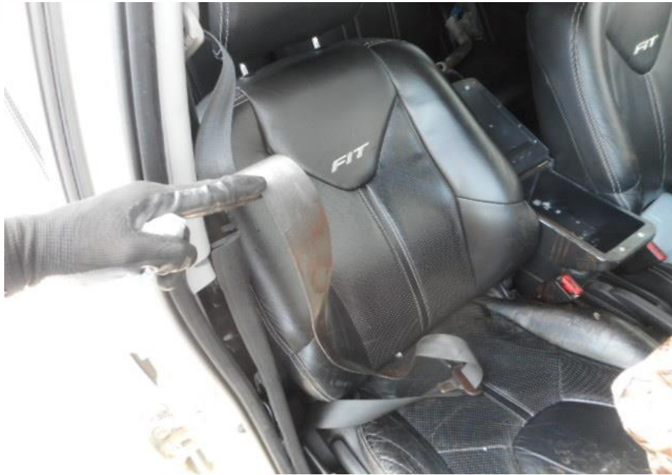
Photo 24 shows that the seat belt on the right seat was worn at the material time of accident as the safety pre-tensioners was activated at the moment of impact and caused the seat belt to be locked into the last position.
