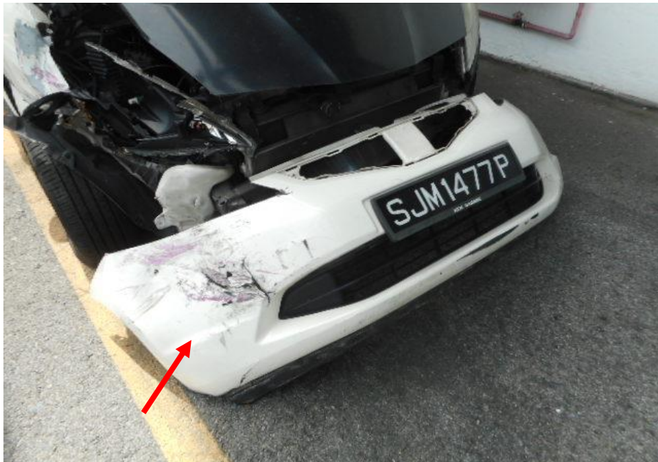
Photo 4 shows the close up view of the Motor Car's front body at the time of my inspection. The Motor car was observed to have sustained damage at its front portion. Its front bumper (arrowed) was damaged as a result of the accident.
