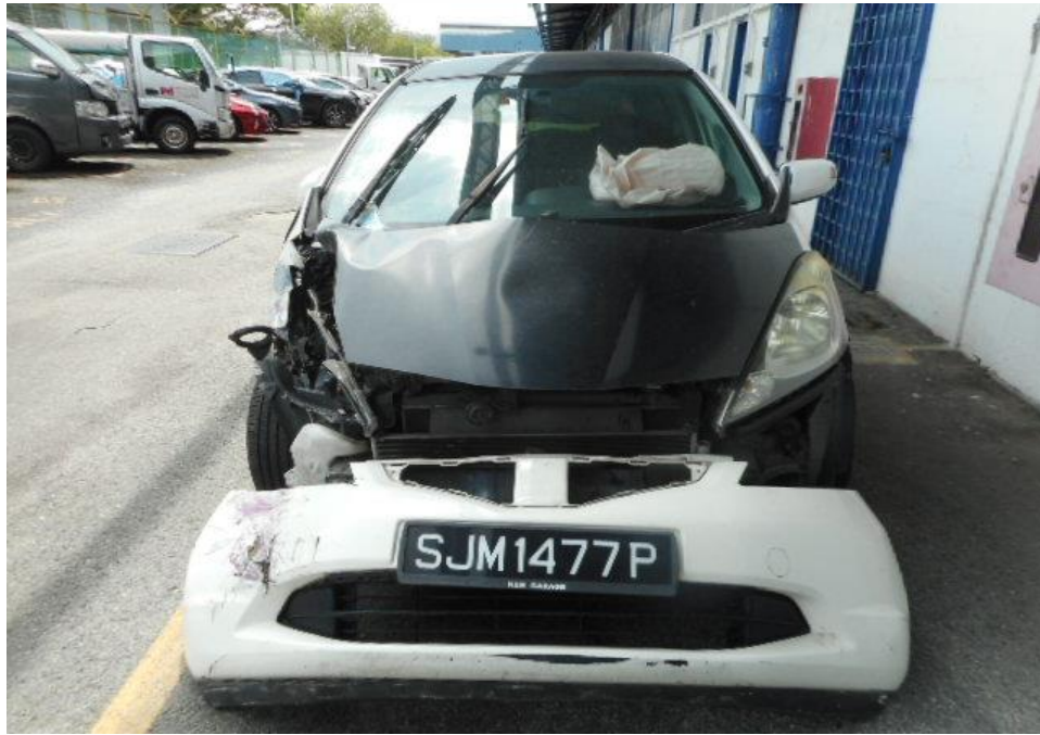
Photo 1 shows a general view of the Motor Car's front body at the time of my inspection. The Motor car was observed to have sustained damage at its front portion. Its front bonnet, front bumper, front right fender and front right headlamp was amongst the body parts damaged as a result of the accident.
