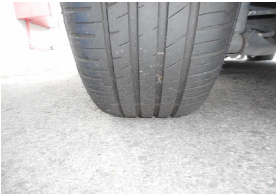
Photo 10 shows the condition of the rear left tyre of the Motor Car, which was observed to be in serviceable condition with remaining tread depth of approximately 4.6mm. The tyre was also observed to be sufficiently inflated for vehicular operation with no tear, cut or burst mark(s).
