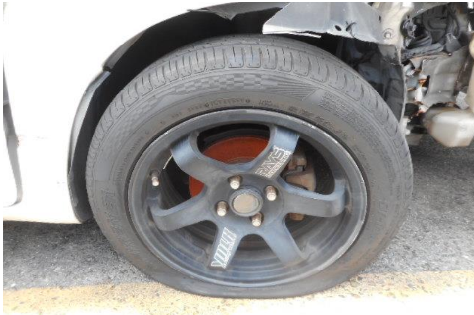
Photo 8 shows the condition of the front right tyre of the Motor Car, which was observed to be deflated due to an induce impact sustained as a result of the accident. The remaining tread depth is approximately 5.3mm.
