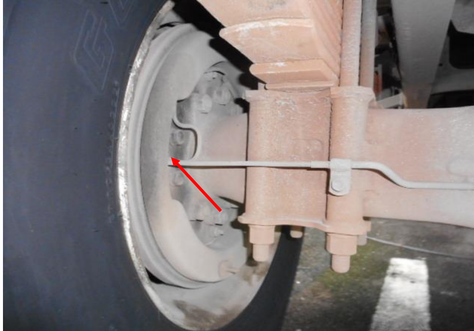
Photo 22 shows the brake pipe (arrowed) at the rear left wheel of the Motor Lorry. I did not observe any leakage of air brake at the time of my inspection of the Motor Lorry. My static tests of the Motor Lorry's braking system, along with my visual examination of the various mechanical components in the braking system, had indicated that there was no internal leakage of pressure/vacuum. Hence the braking system of the Motor Lorry was likely to be in serviceable condition at the material time of accident.
