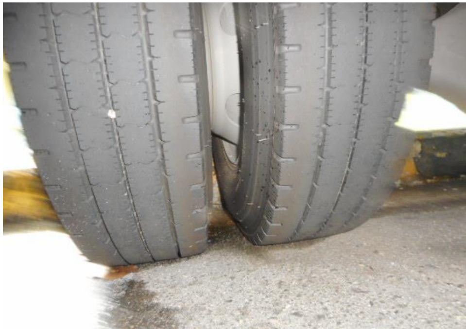
Photo 9 shows the condition of the rear right tyres of the Motor Lorry, which was observed to be in serviceable condition with remaining tread depth of approximately 6mm. The tyre, which was wrapped around standard steel wheel rim, it was observed to be sufficiently inflated for vehicular operation.
