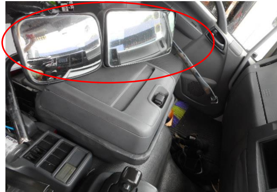
Photo 5 shows a close up view of the Motor Lorry's left rear view mirror at the time of my inspection. Its left rear view mirror (circled) was damage at the time of my inspection as a result of the accident.
