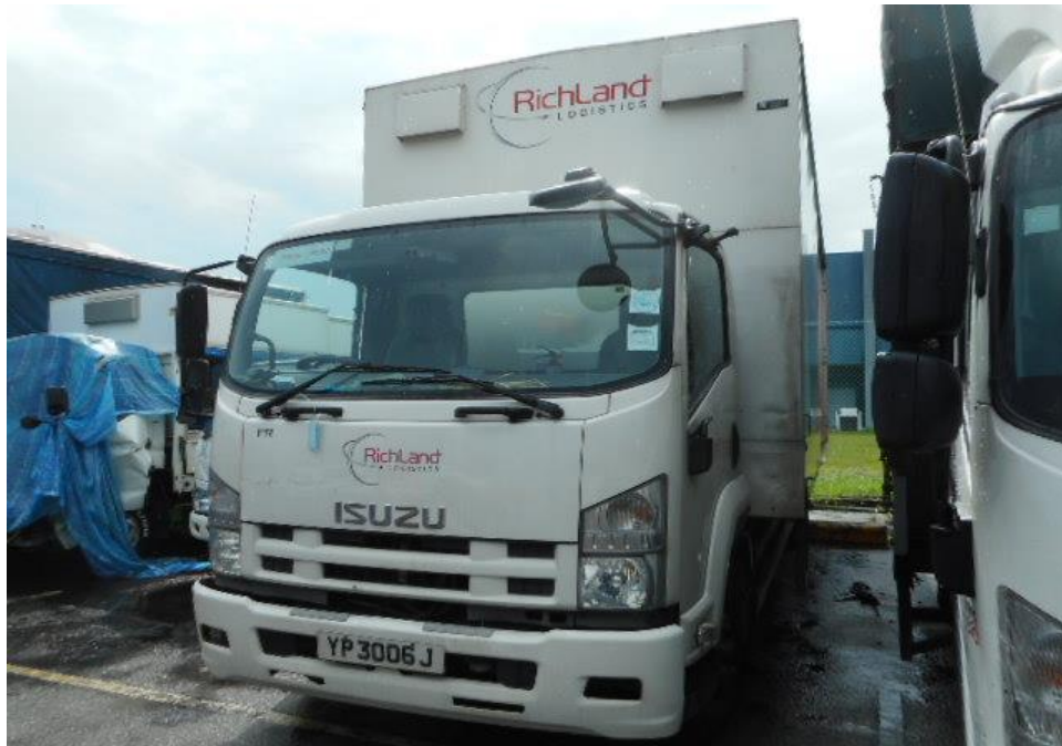
Photo 3 shows a general view of the Motor Lorry's left portion at the time of my inspection. It appeared to have sustained damage at its left portion. Its left rear view mirror were damage at the time of my inspection as a result of the accident.
