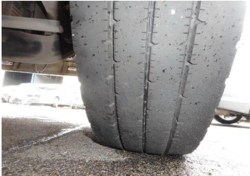
Photo 8 shows the condition of the front right tyre of the Motor Lorry, which was observed to be in serviceable condition with remaining tread depth of approximately 6.5mm. The tyre, which was wrapped around standard steel wheel rim, was also observed to be sufficiently inflated for vehicular operation. There was no tear, cut or burst mark(s) on the outer and the inner sidewalls as well as across the tread of the 6 tyres that were fitted on the Motor Lorry.
