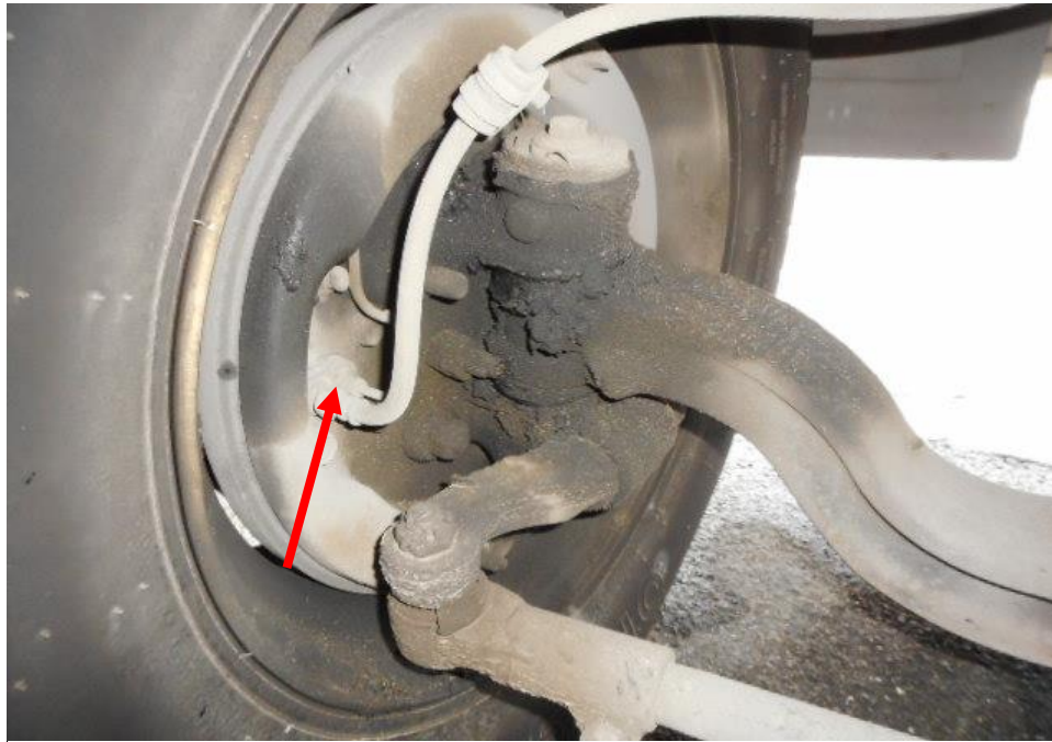
Photo 24 shows the brake hose/pipe (arrowed) at the front left wheel of the Motor Lorry. No leakage of air brake was observed. Visual examination of the various components of the braking system like the brake drum, brake booster, brake pedal etc had revealed all to be intact and without visible damage at the time of accident. There was also no sign of fluid stain(s) observed on the various undercarriage components.
