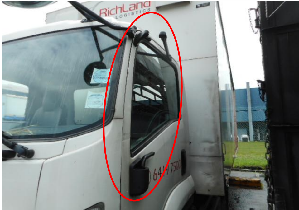
Photo 4 shows a close up view of the Motor Lorry's left portion at the time of my inspection. Its left rear view mirror (circled) was damage at the time of my inspection as a result of the accident.
