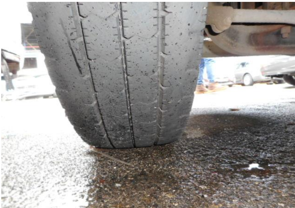
Photo 11 shows the condition of the front left tyre of the Motor Lorry, which were observed to be in serviceable condition with remaining, tread depth of approximately 4.2mm. There was also no tear, cut or burst mark(s) on the outer and the inner sidewalls as well as across the tread of the 6 tyres that were fitted on the Motor Lorry.
