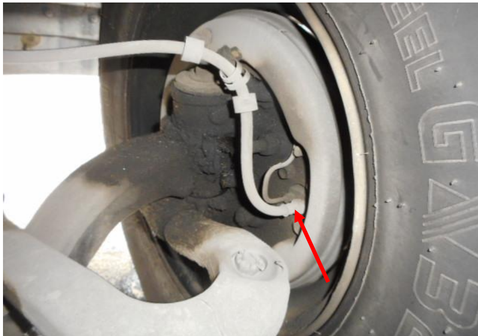
Photo 23 shows the brake hose/pipe (arrowed) at the front right wheel of the Motor Lorry. No leakage of air brake was observed. Visual examination of the various components of the braking system like the brake drum, brake booster, brake pedal etc had revealed all to be intact and without visible damage at the time of accident. There was also no sign of fluid stain(s) observed on the various undercarriage components.
