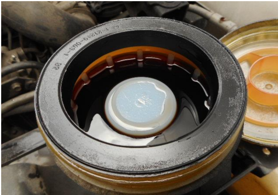
Photo 16 shows the power steering fluid reservoir of the Motor Lorry at the time of my inspection. The power steering fluid was observed to be of sufficient level and without any visible contamination.
