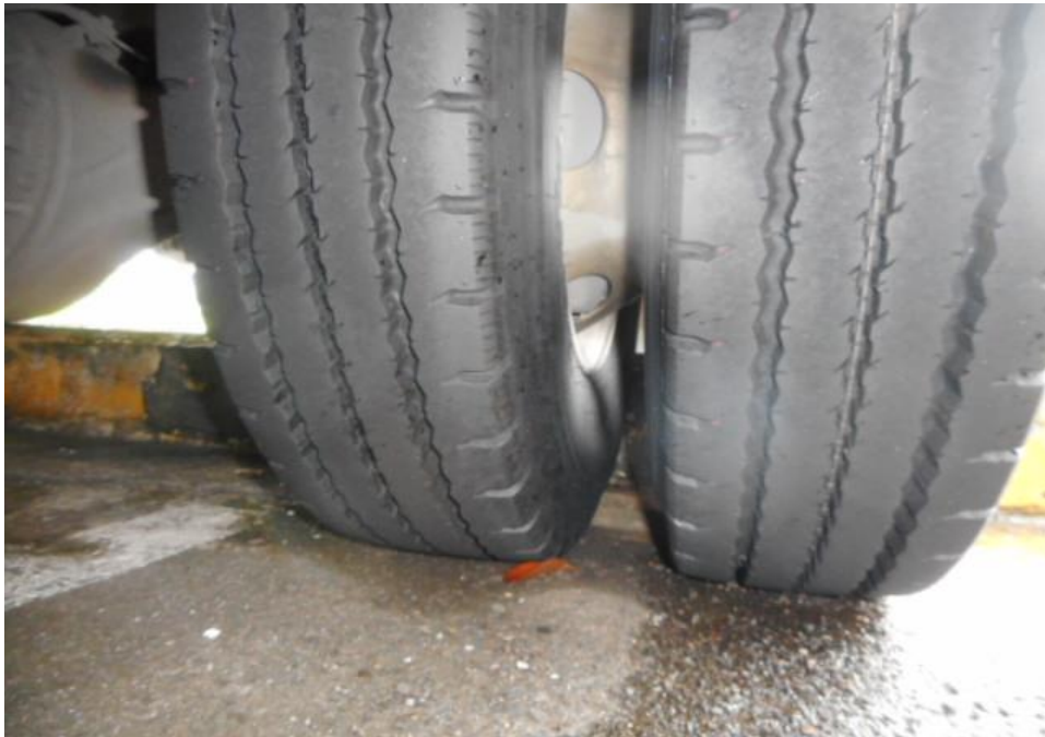
Photo 10 shows the condition of the rear left tyres of the Motor Lorry, which was observed to be in serviceable condition with remaining tread depth of approximately 12.4mm. The tyres, which were wrapped around standard steel wheel rim, were also observed to be sufficiently inflated for vehicular operation.
