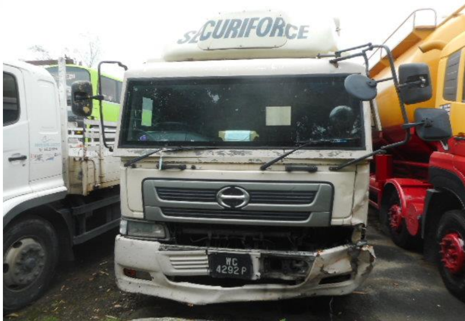
Photo 2 shows a general view of the front body of the Motor Trailer at the time of my inspection. The Motor Trailer was observed to sustain damaged on its Trailer's front portion. Its front bumper, front right headlamp and front left body panel was damaged at the time of my inspection.
