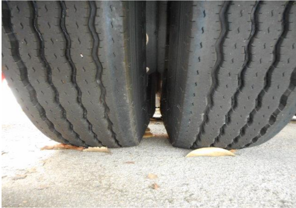
Photo 16 shows the condition of the left tyres of the trailer, which was observed to be in serviceable condition with remaining tread depth of approximately 9.8mm. There was also no tear, cut or burst mark(s) on the outer and the inner sidewalls as well as across the tread of the 8 tyres that were fitted on the trailer.
