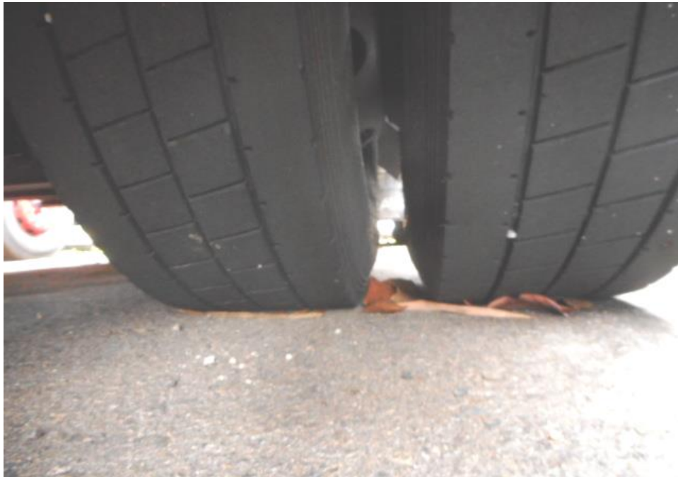
Photo 12 shows the condition of the rear right tyre of the Motor Trailer, which was observed to be in serviceable condition with remaining tread depth of approximately 5.8mm. The tyre, which was wrapped around standard steel wheel rim, was also observed to be sufficiently inflated for vehicular operation.
