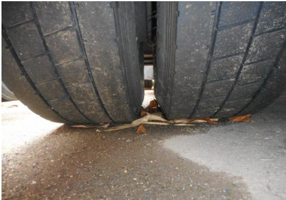
Photo 13 shows the condition of the rear left tyres of the Motor Trailer, which was observed to be in serviceable condition with remaining tread depth of approximately 4.9mm. The tyres, which were wrapped around standard steel wheel rim, were also observed to be sufficiently inflated for vehicular operation. There was also no damage found on all 6 steel wheel rims of the Motor Trailer.
