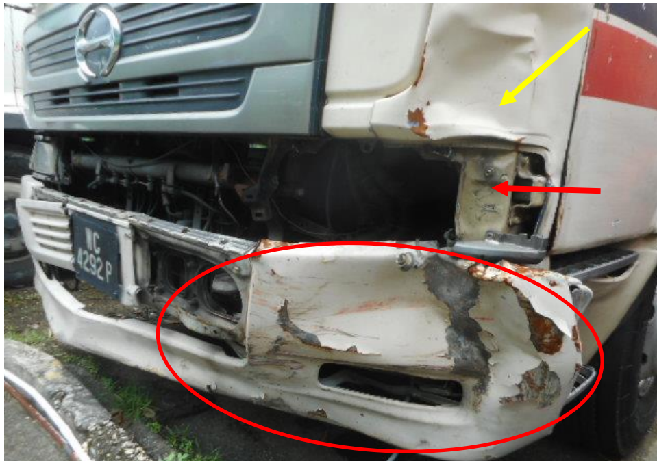
Photo 3 shows a general view of the front body of the Motor Trailer at the time of my inspection. The Motor Trailer was observed to sustain damaged on its Trailer's front portion. Its front bumper (circled), front right headlamp (red arrow) and its front left body panel (yellow arrow) was damaged at the time of my inspection.
