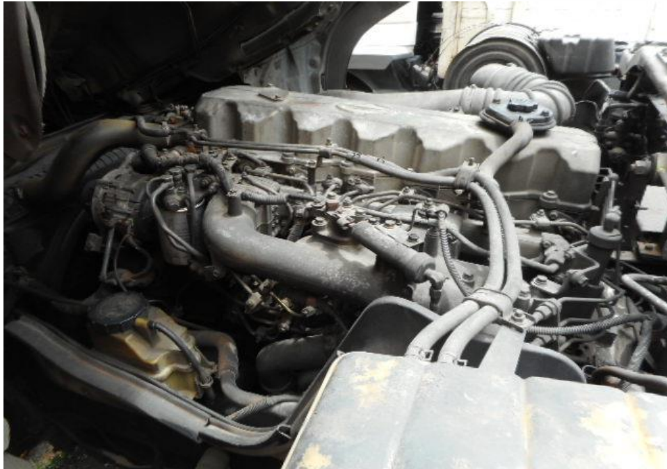
Photo 17 shows a general view of the Motor Trailer's engine compartment, which was accessed by lifting the front cabin of the Motor Trailer. The various parts and components inside the engine compartment were unaffected by the accident. There was also no sign(s) or indication(s) of fresh fluid leakage and/or fluid stain within the engine compartment
