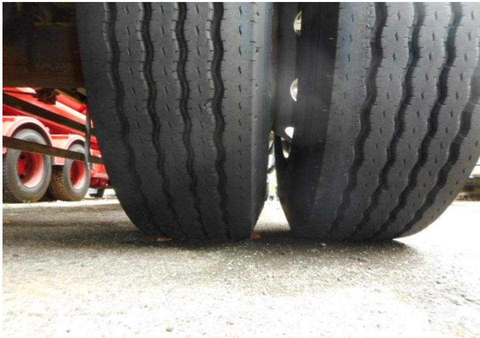
Photo 15 shows the condition of the right tyres of the trailer, which was observed to be in serviceable condition with remaining, tread depth of approximately 10.7mm. There was also no tear, cut or burst mark(s) on the outer and the inner sidewalls as well as across the tread of the 8 tyres that were fitted on the trailer.
