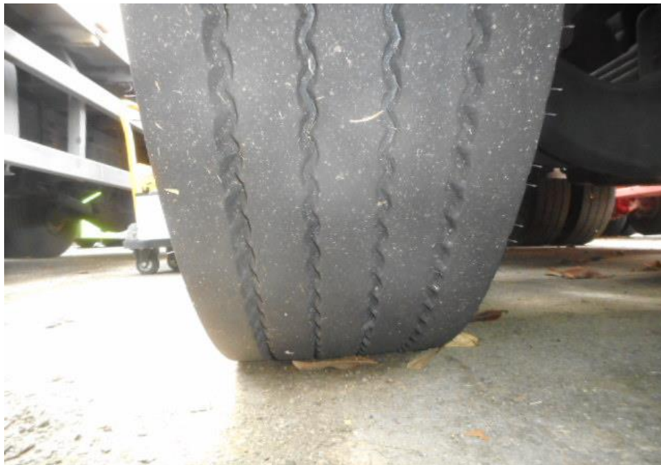
Photo 11 shows the condition of the front right tyre of the Motor Trailer, which was observed to be in serviceable condition with remaining tread depth of approximately 7.4mm. The tyre, which was wrapped around standard steel wheel rim, was also observed to be sufficiently inflated for vehicular operation. There was no tear, cut or burst mark(s) on the outer and the inner sidewalls as well as across the tread of the 6 tyres that were fitted on the Motor Trailer.
