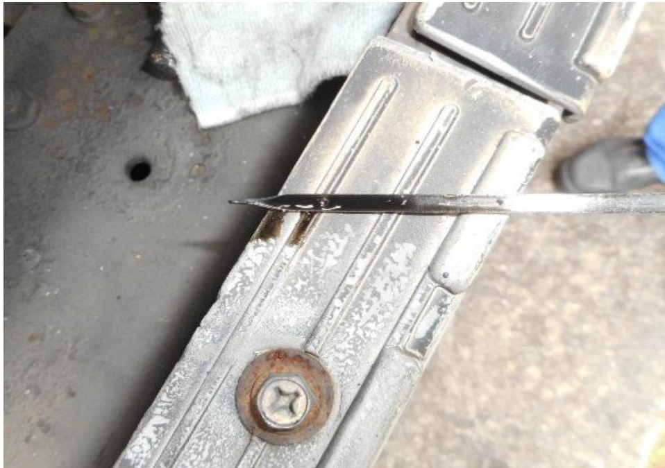
Photo 21 shows the engine oil dip stick of the Motor Trailer at the time of my inspection. The engine oil was observed to be of insufficient level at the time of our inspection.
