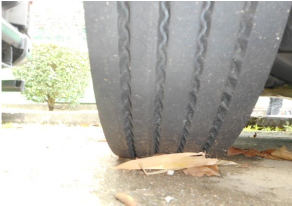
Photo 14 shows the condition of the front left tyres of the Motor Trailer, which were observed to be in serviceable condition with remaining tread depth of approximately 9.9mm. There was also no tear, cut or burst mark(s) on the outer and the inner sidewalls as well as across the tread of the 6 tyres that were fitted on the Motor Trailer.
