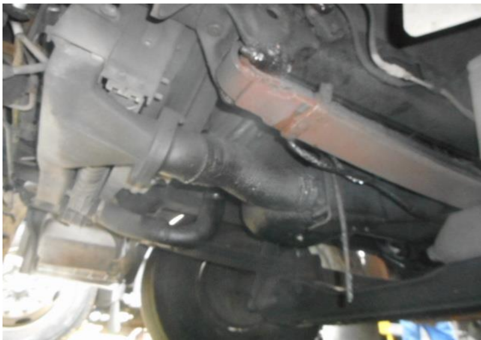
Photo 22 shows the undercarriage of the Motor Trailer, at the area where the engine housing located. I did not find any sign(s) or indication(s) of fluid leak, however old fluid stain(s) was observed on the underside of the Motor Trailer.
