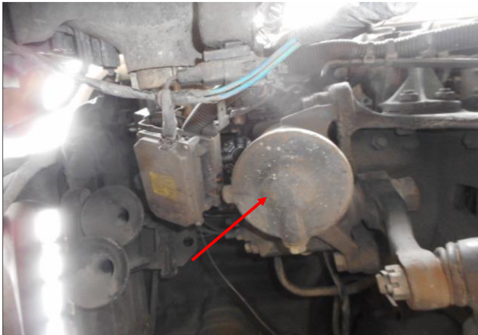
Photo 30 shows the steering box component (arrowed) at the undercarriage of the Motor Trailer was found to be intact without any visible damage. There was also no sign of fluid stain(s) observed on the various undercarriage components.
