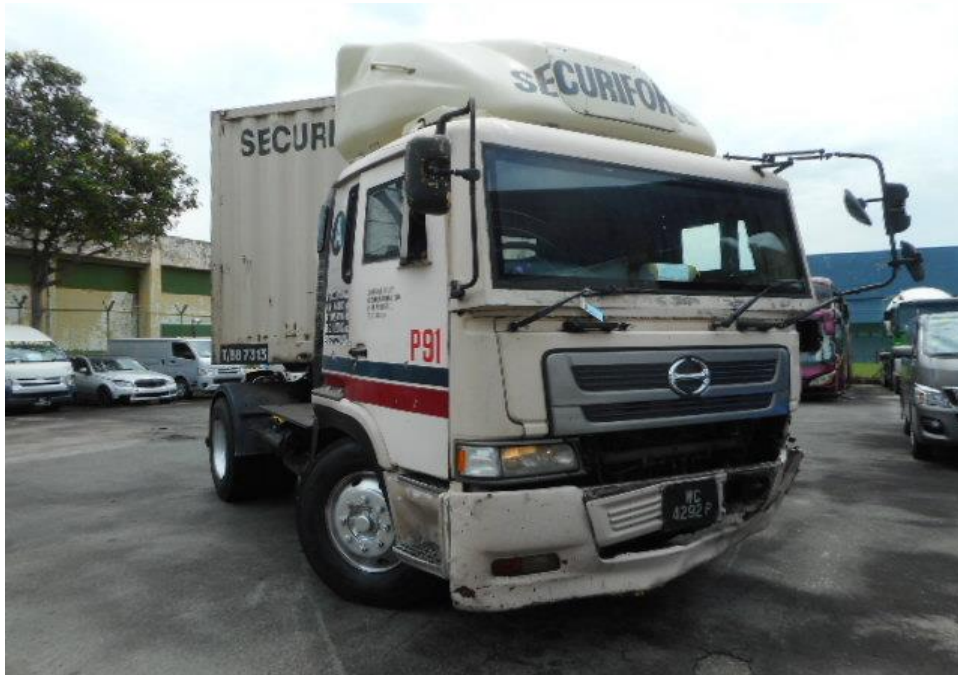
Photo 31 shows the front left wheel of the Motor Trailer turned to its full left. During my steering system test, I did not experience any abnormal free play and/or resistance when I had turned the steering wheel towards full left and full right. This would suggest that the steering system of the Motor Trailer was likely to be in serviceable condition at the material time of accident.
