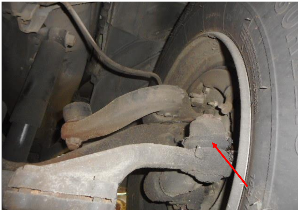
Photo 28 shows the various undercarriage components at the front right wheel of the Motor Trailer, in particular the steering tie rod end (arrowed). The various steering components were all found to be intact, suggesting that the steering system of the Motor Trailer was likely to be in serviceable condition at the material time of accident. There was also no sign of fluid stain(s) observed on the various undercarriage components.
