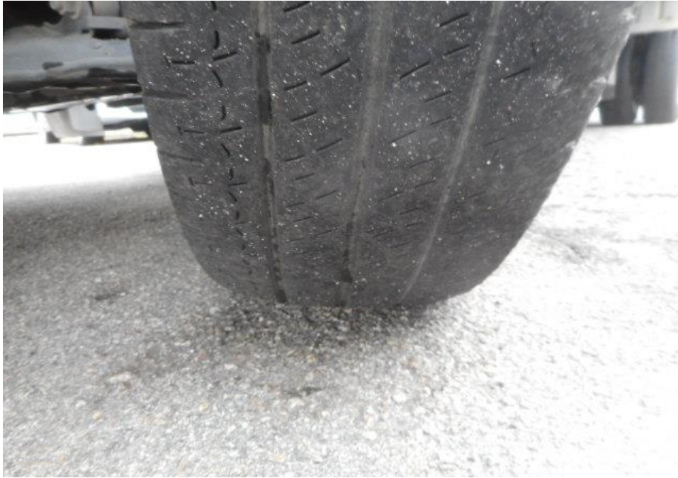
Photo 10 shows the condition of the front right tyre of the Motor Lorry, which was observed to be in serviceable condition with remaining tread depth of approximately 2.6mm. The tyres, which were wrapped around standard steel wheel rim, were also observed to be sufficiently inflated for vehicular operation.
