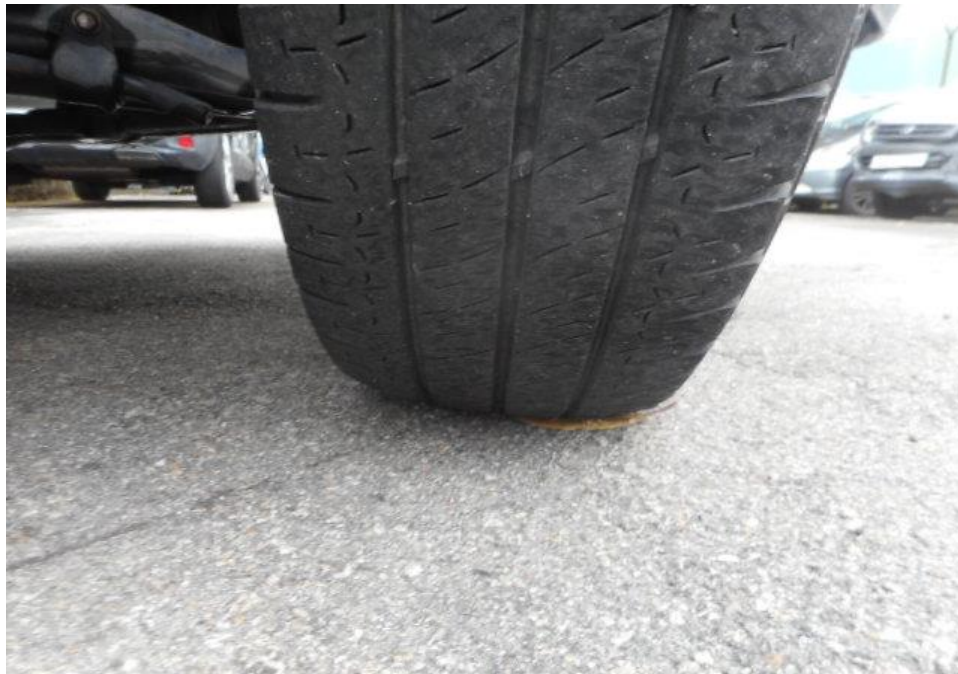
Photo 7 shows the condition of the front right tyre of the Motor Lorry, which was observed to be in serviceable condition with remaining tread depth of approximately 4.7mm. The tyre, which was wrapped around standard steel wheel rim, it was observed to be sufficiently inflated for vehicular operation.
