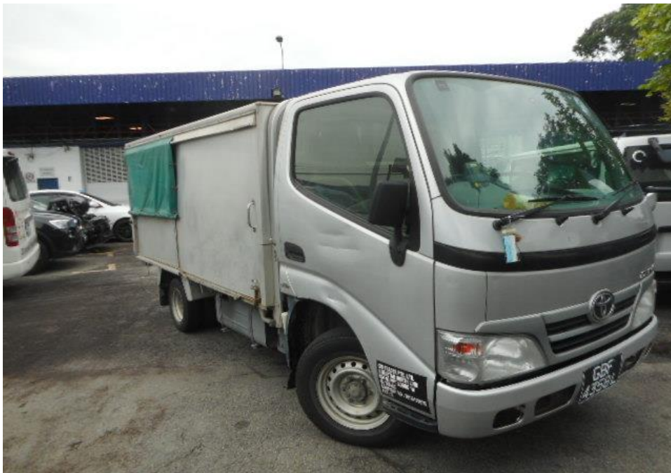
Photo 23 shows the front right wheel of the Motor Lorry turned to its full left. During my steering system test, I did not experience any abnormal free play and/or resistance when I had turned the steering wheel towards the left and right. This would suggest that the steering system of the Motor Lorry was likely to be in serviceable condition at the material time of accident.
