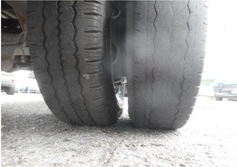
Photo 8 shows the condition of the rear right tyre of the Motor Lorry, which was observed to be in serviceable condition with remaining tread depth of approximately 2.9mm. The tyre, which was wrapped around standard steel wheel rim, it was observed to be sufficiently inflated for vehicular operation.
