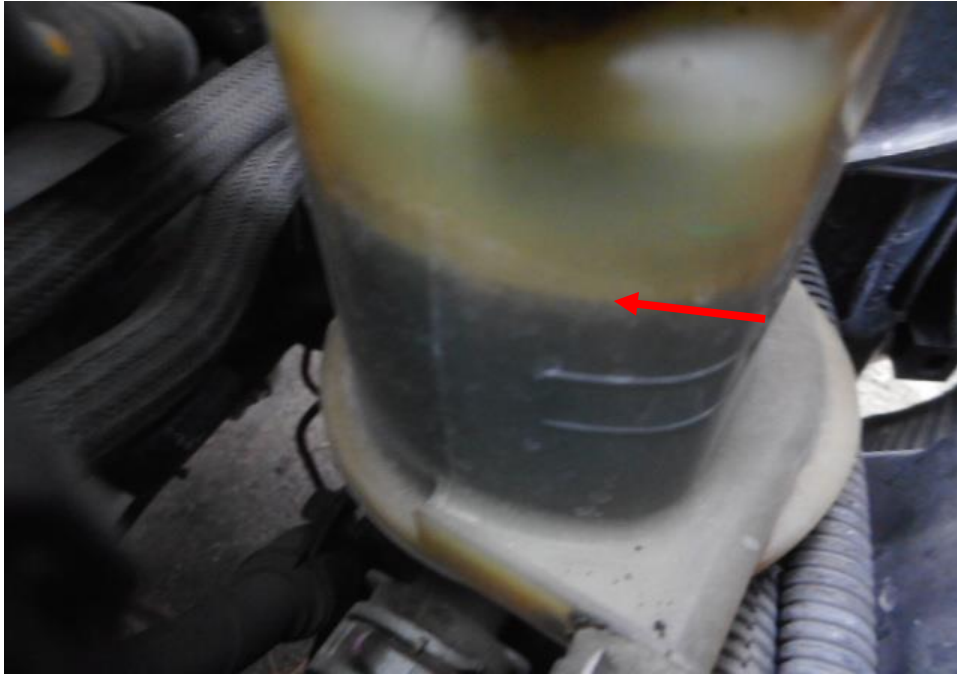
Photo 15 shows the power steering fluid reservoir of the Motor Lorry at the time of my inspection. The power steering fluid (arrowed) was observed to be of sufficient level and without any visible contamination.
