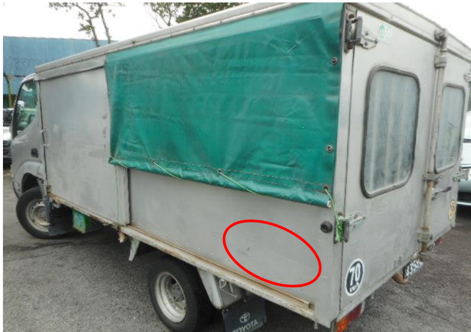
Photo 3 shows a general view of the left body of the Motor Lorry at the time of my inspection. The Motor Lorry was observed to sustained damage at its left portion. Its rear left door panel (circled) was damage at the time of my inspection as a result of the accident.
