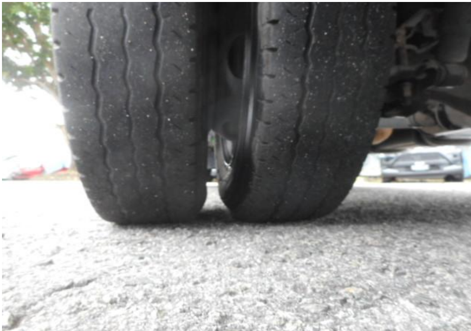
Photo 9 shows the condition of the rear left tyres of the Motor Lorry, which was observed to be in serviceable condition with remaining tread depth of approximately 1.7mm. The tyres, which were wrapped around standard steel wheel rim, were also observed to be sufficiently inflated for vehicular operation.
