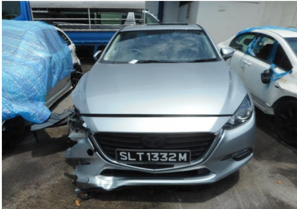
Photo 1 shows a general view of the Motor Car's front body at the time of my inspection. The Motor car was observed to have sustained damage at its front portion. Its front bonnet, front bumper, front right fender, front right headlamp was the body parts that were damaged as a result of the accident.
