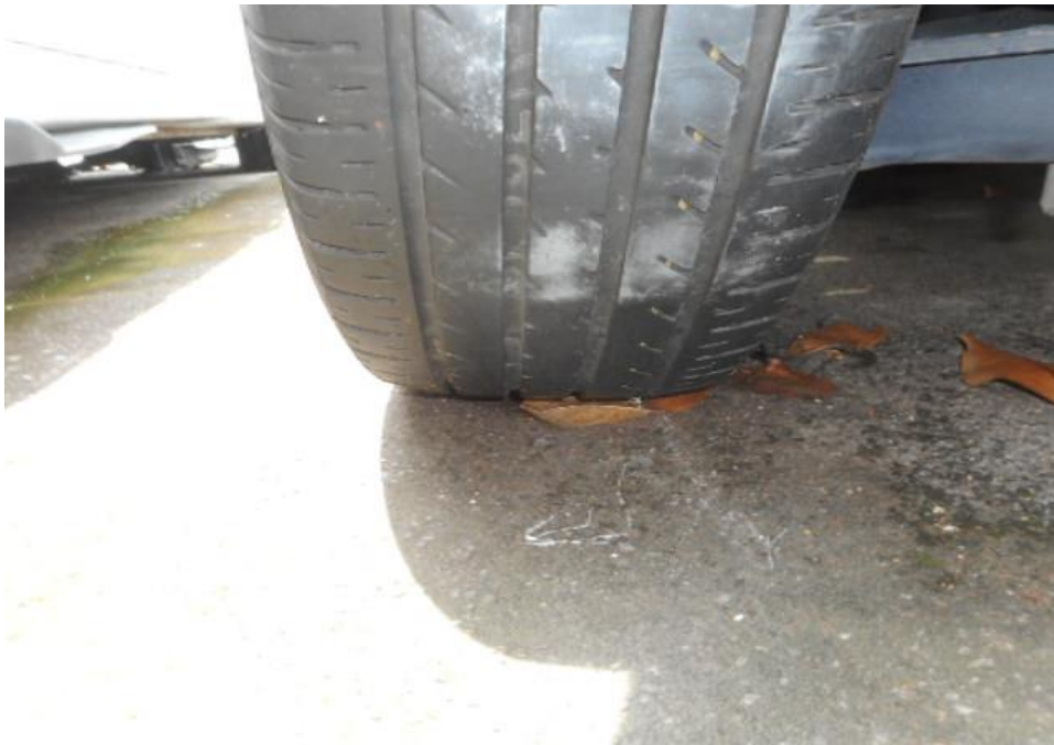
Photo 10 shows the condition of the rear left tyre of the Motor Car, which was observed to be in serviceable condition with remaining tread depth of approximately 3.8mm. The tyre was also observed to be sufficiently inflated for vehicular operation with no tear, cut or burst mark(s).
