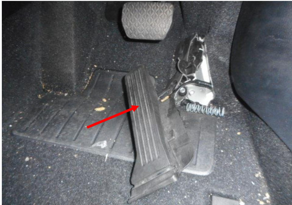
Photo 24 shows the general view of the accelerator pedal (arrowed) at the driver's foot well of the Motor Car. I observed that the accelerator pedal was broken due to the induced impact from the accident which had caused the body of the Motor Car to bent inwards and damage the accelerator at the time of my inspection of the Motor Car.
