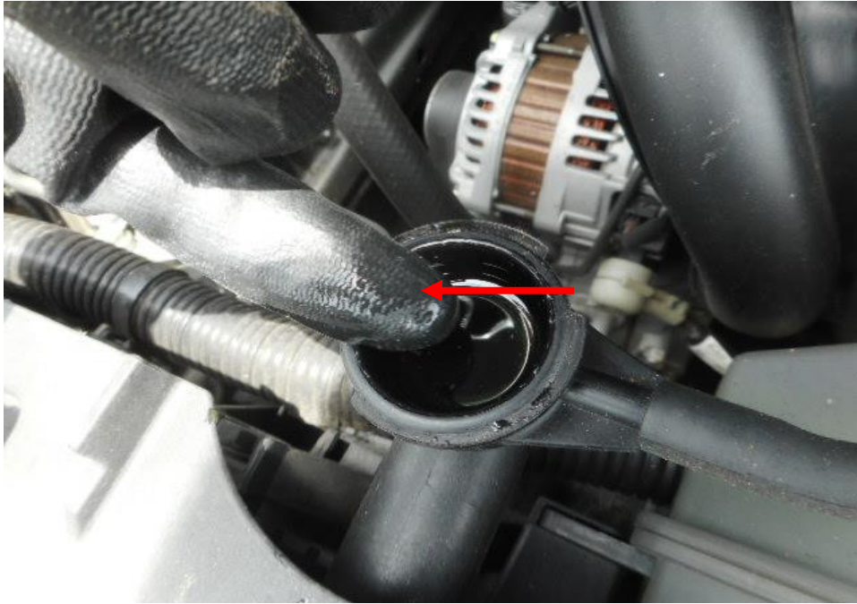
Photo 14 shows the engine coolant reservoir of the Motor Car at the time of my inspection. The coolant was observed to be of sufficient level (arrowed) and without any visible contamination.
