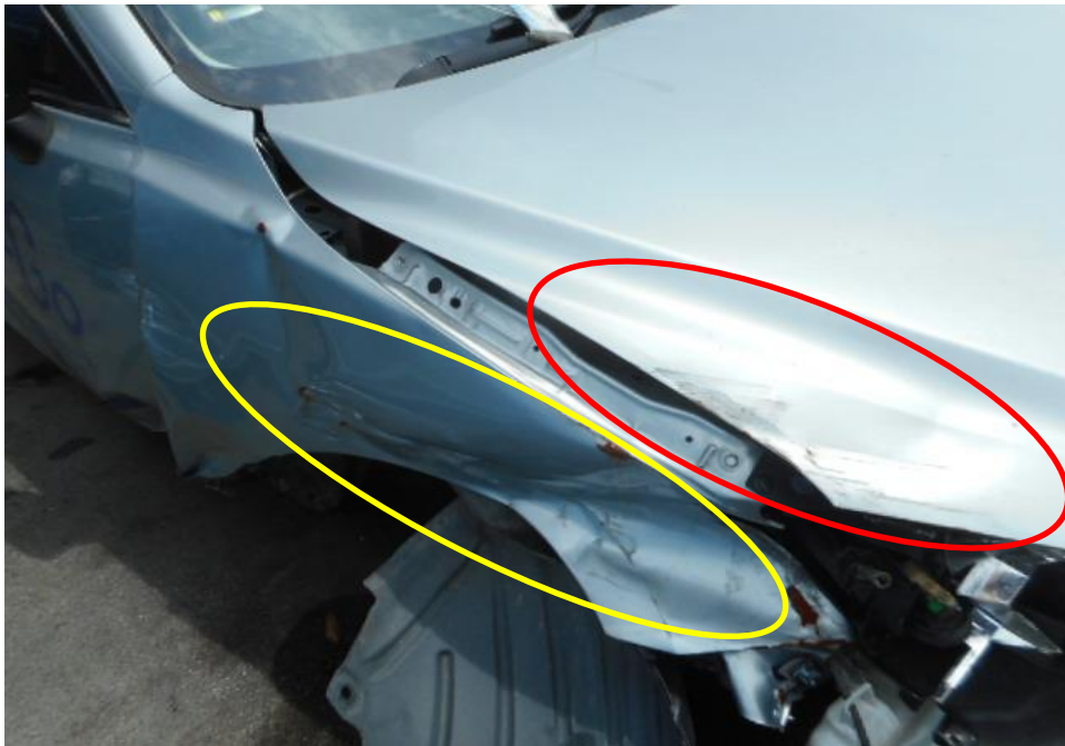
Photo 2 shows the close up view of the Motor Car's front body at the time of my inspection. The Motor car was observed to have sustained damage at its front portion. Its front bonnet (red circle) and its front right fender (yellow circle) was damaged as a result of the accident.
