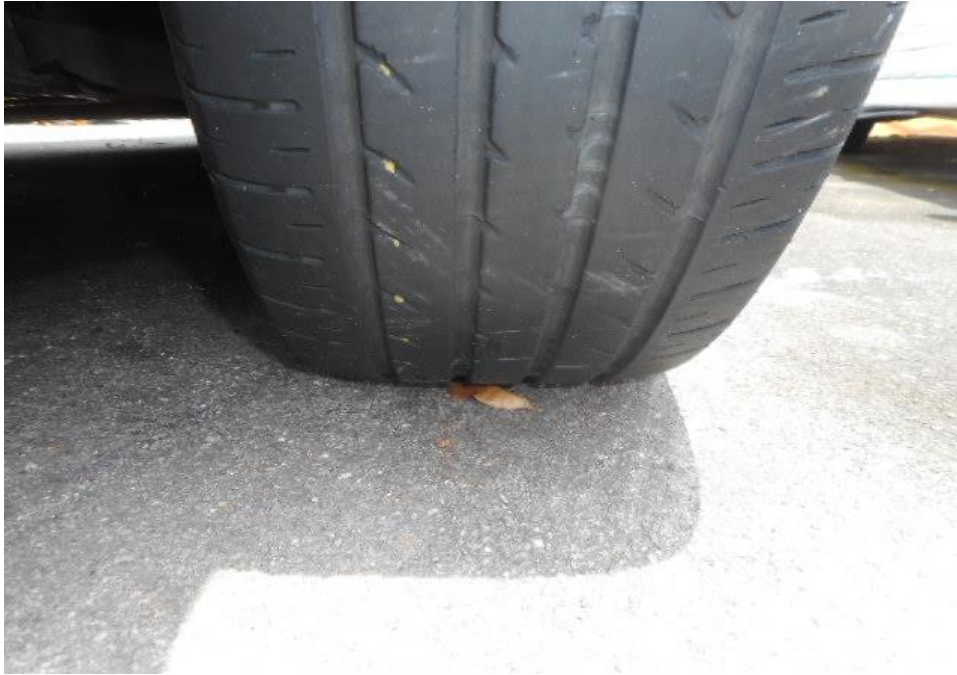
Photo 11 shows the condition of the front left tyre of the Motor Car, which was observed to be in serviceable condition with remaining tread depth of approximately 4mm. The tyre was also observed to be sufficiently inflated for vehicular operation with no tear, cut or burst mark(s).
