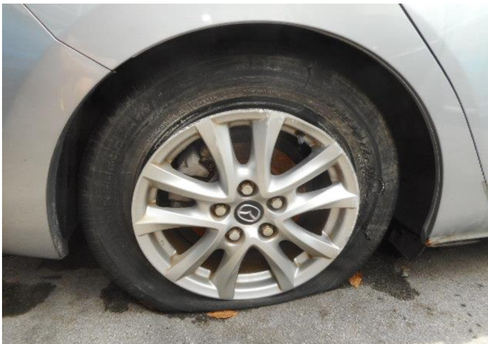
Photo 8 shows the general condition of the rear right tyre and wheel rim of the Motor Car, which was observed to be cut and deflated as a result of the accident with remaining tread depth of approximately 3.8mm.
