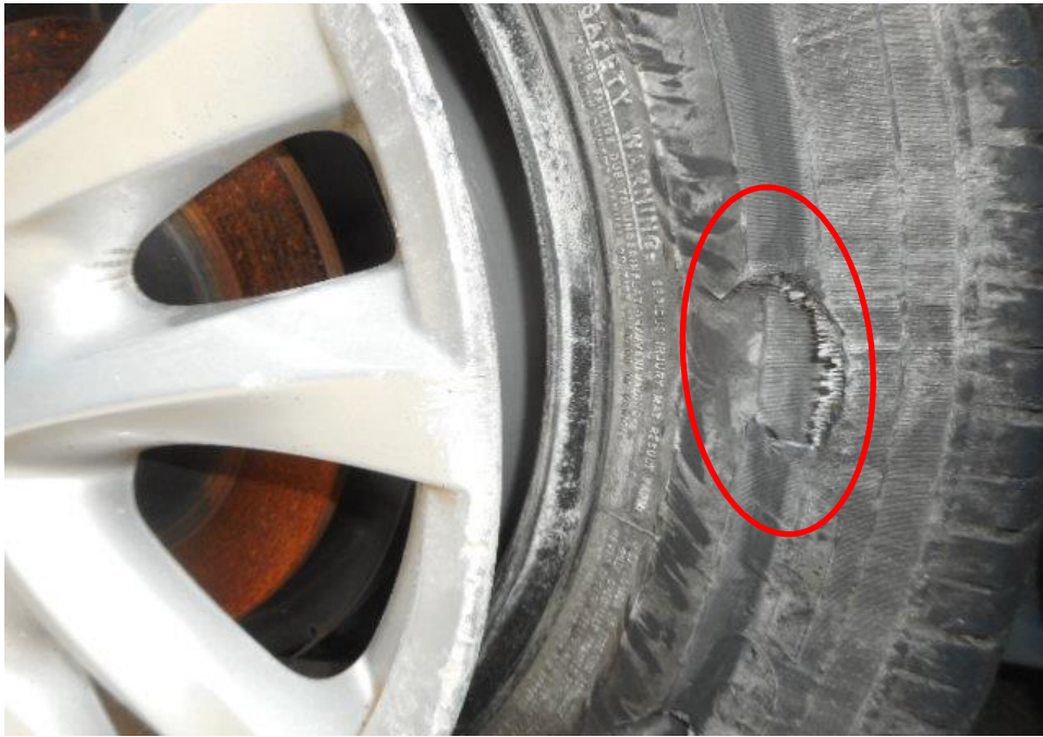
Photo 9 shows the close up condition of the rear right tyre and wheel rim of the Motor Car, which was observed to be cut and deflated (circled) as a result of the accident with remaining tread depth of approximately 3.8mm.
