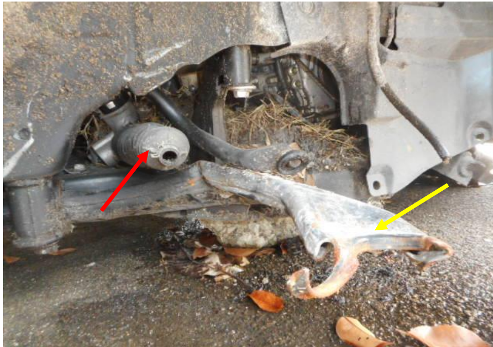
Photo 17 shows the various undercarriage components at the front right wheel of the Motor Car, in particular the steering tie rod (red arrow) and the lower control arm (yellow arrow) was observed to be missing and broken off as a result of the accident.
