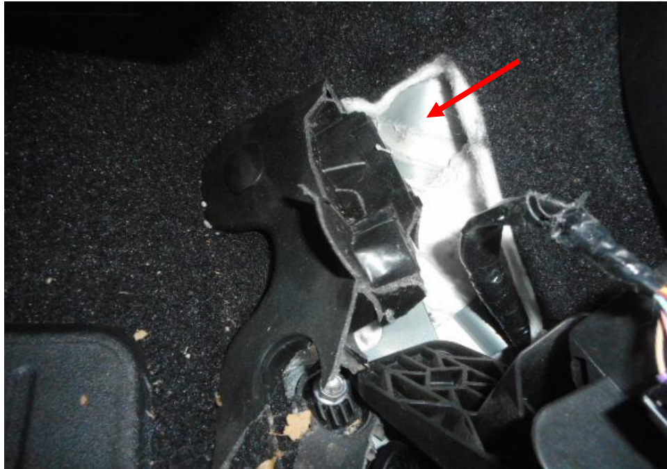
Photo 25 shows the close up view of the Motor Car's body that was bent inwards and damaged the accelerator pedal (arrowed) at the driver's foot well of the Motor Car also a result of the accident.
