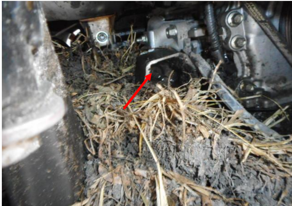
Photo 18 shows the various undercarriage components at the front right wheel of the Motor Car, in particular the driveshaft (arrowed) was observed to be missing as a result of the accident.
