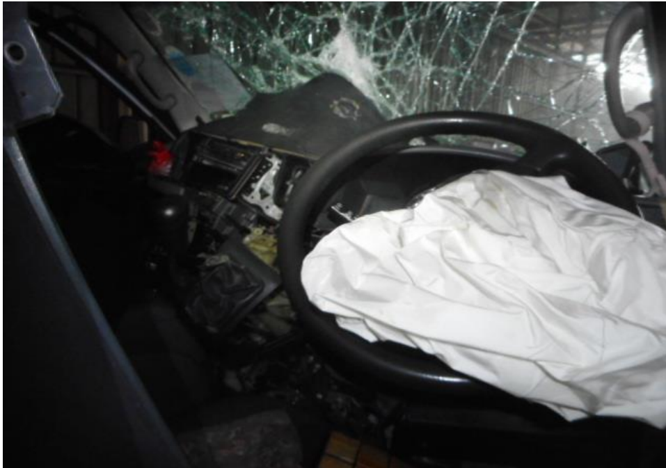
Photo 15 shows the deployment of the Supplemental Restraint System (SRS) airbag in the Motor Car as a result of the accident.
