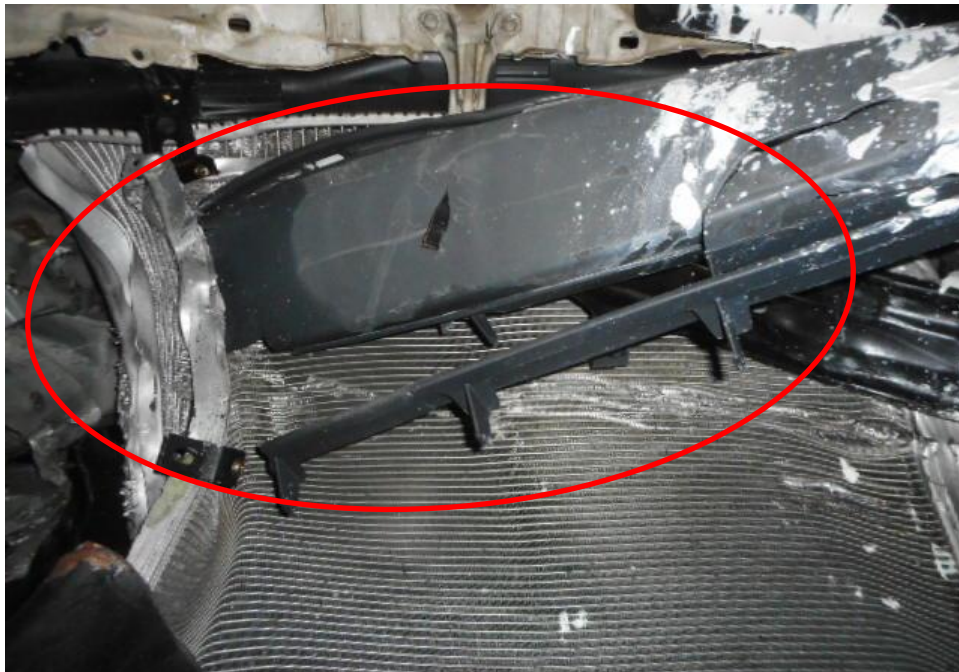
Photo 6 shows the close up view of the front portion of the Motor Van at the time of our inspection. The Motor Van was observed to have sustained major damages to its front engine coolant radiator (circled) was damaged as a result of the accident's impact.
