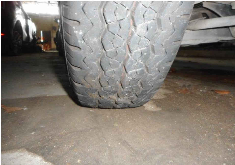
Photo 14 shows the condition of the front left tyre of the Motor Van, which were observed to be in serviceable condition with remaining, tread depth of approximately 7.4mm. There was also no tear, cut or burst mark(s) on the outer and the inner sidewalls as well as across the tread of the 4 tyres that were fitted on the Motor Van.
