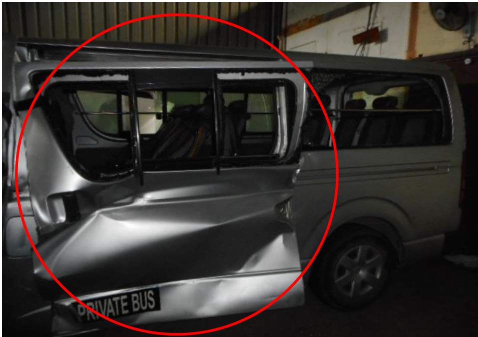
Photo 10 shows a general view of the Motor Van's left body at the time of my inspection. The Motor Van was observed to have sustained damages to its left rear door and windscreen (circled) as a result of the accident.
