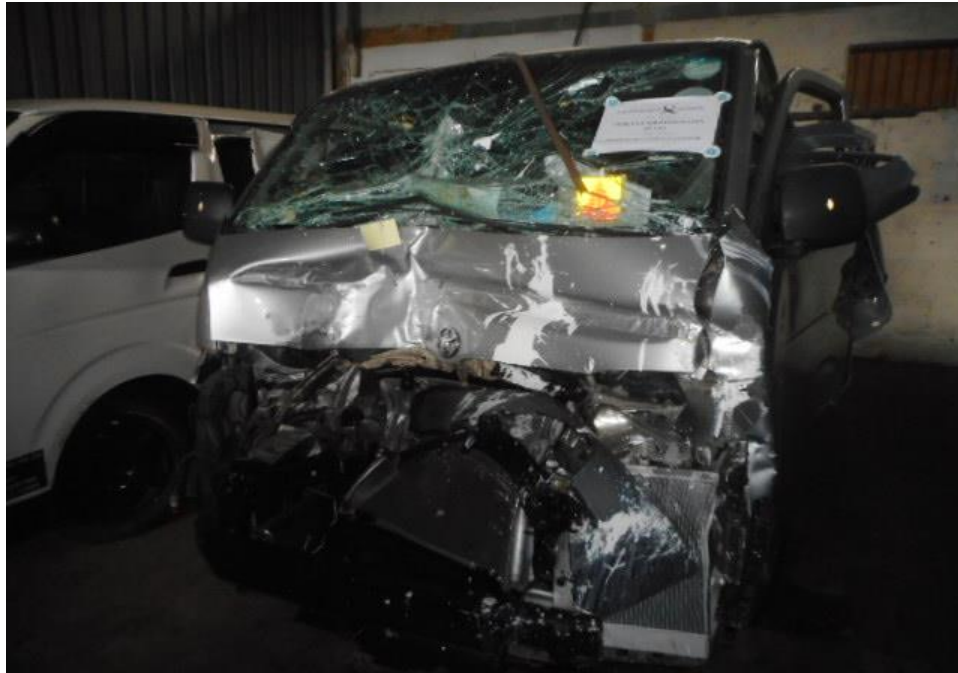
Photo 3 shows a general view of the front portion of the Motor Van at the time of our inspection. The Motor Van was observed sustained major damages to its front, right and left portion. Its front windscreen, front body panel, front grille, front bumper, right and left doors was the body parts that were damaged and various engine components was also damaged as a result of the accident. The Supplemental Restraint System (SRS) was activated as a result of the accident.
