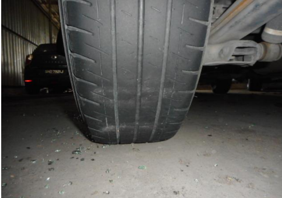
Photo 13 shows the condition of the rear left tyres of the Motor Van, which were observed to be in serviceable condition with remaining, tread depth of approximately 2mm.
