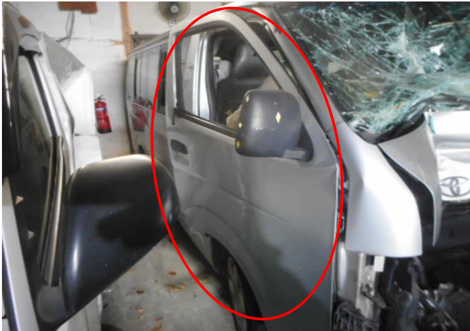
Photo 7 shows the close up view of the right door of the Motor Van at the time of our inspection. The Motor Van was observed to have sustained damages to its right door (circled) as a result of the accident.
