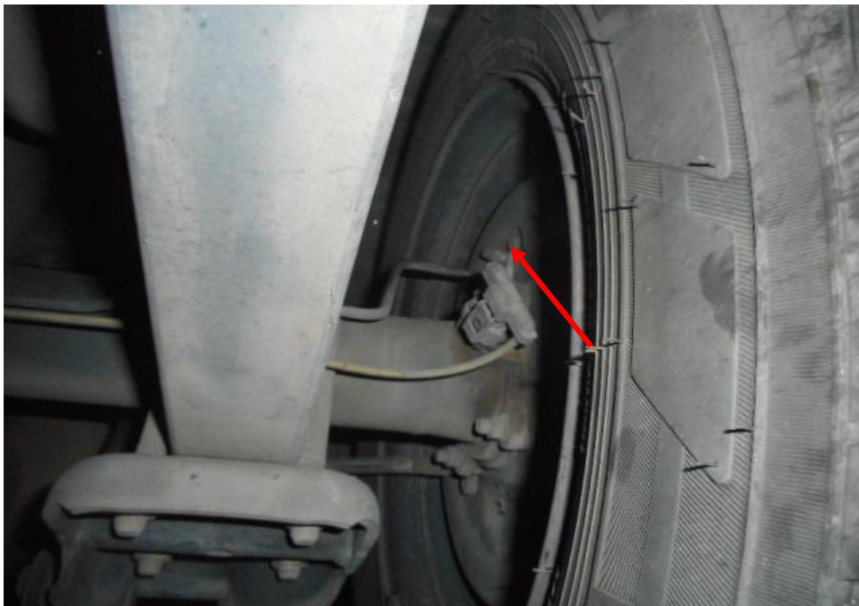
Photo 22 shows the brake pipe (arrowed) at the rear right wheel of the Motor Van. I did not observe any leakage of brake fluid at the time of my inspection of the Motor Van. My static tests of the Motor Van's braking system, along with my visual examination of the various mechanical components in the braking system, had indicated that there was no internal leakage of pressure/vacuum.
