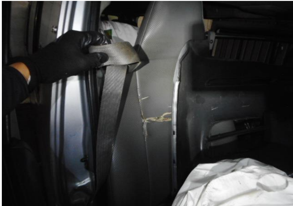
Photo 27 shows that the seat belt on the right seat was worn at the material time of accident as the safety pre-tensioners was activated at the moment of impact and caused the seat belt to be locked into the last position.
