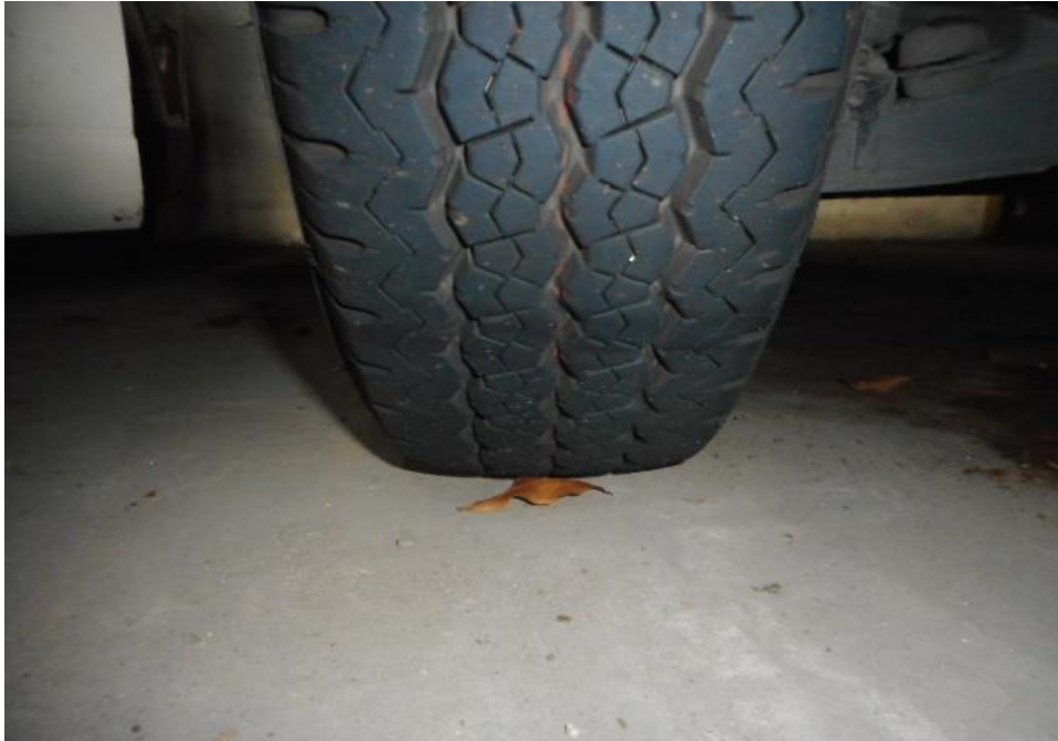
Photo 11 shows the condition of the front right tyre of the Motor Van, which were observed to be in serviceable condition with remaining, tread depth of approximately 7.7mm. The tyre, which was wrapped around standard steel wheel rim, it was observed to be sufficiently inflated for vehicular operation.
