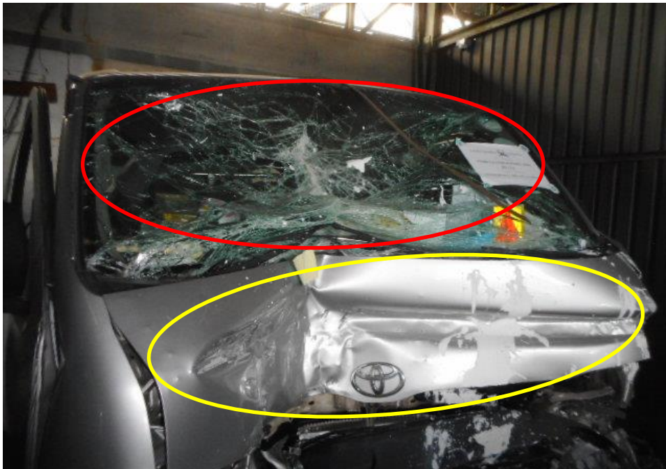
Photo 4 shows the close up view of the front portion of the Motor Van at the time of our inspection. The Motor Van was observed to have sustained major damages to its front windscreen (red circle) and front body panel (yellow circle) as a result of the accident.
