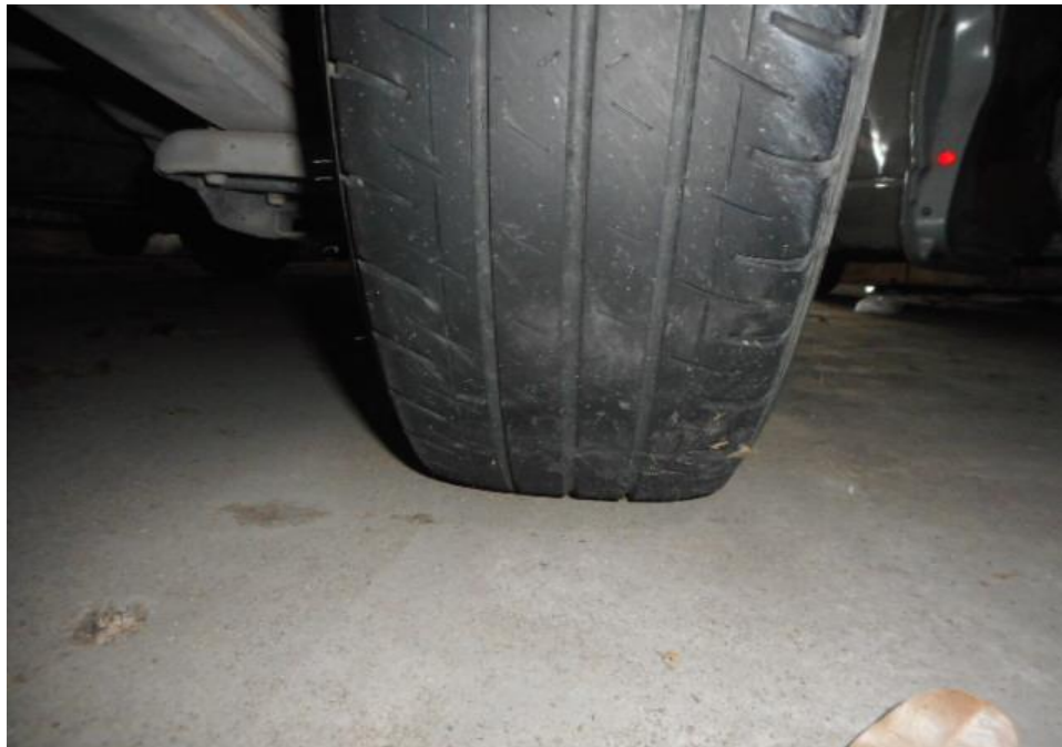
Photo 12 shows the condition of the rear right tyres of the Motor Van, which were observed to be in serviceable condition with remaining, tread depth of approximately 2.5mm. The tyre, which was wrapped around standard steel wheel rim, it was observed to be sufficiently inflated for vehicular operation.
