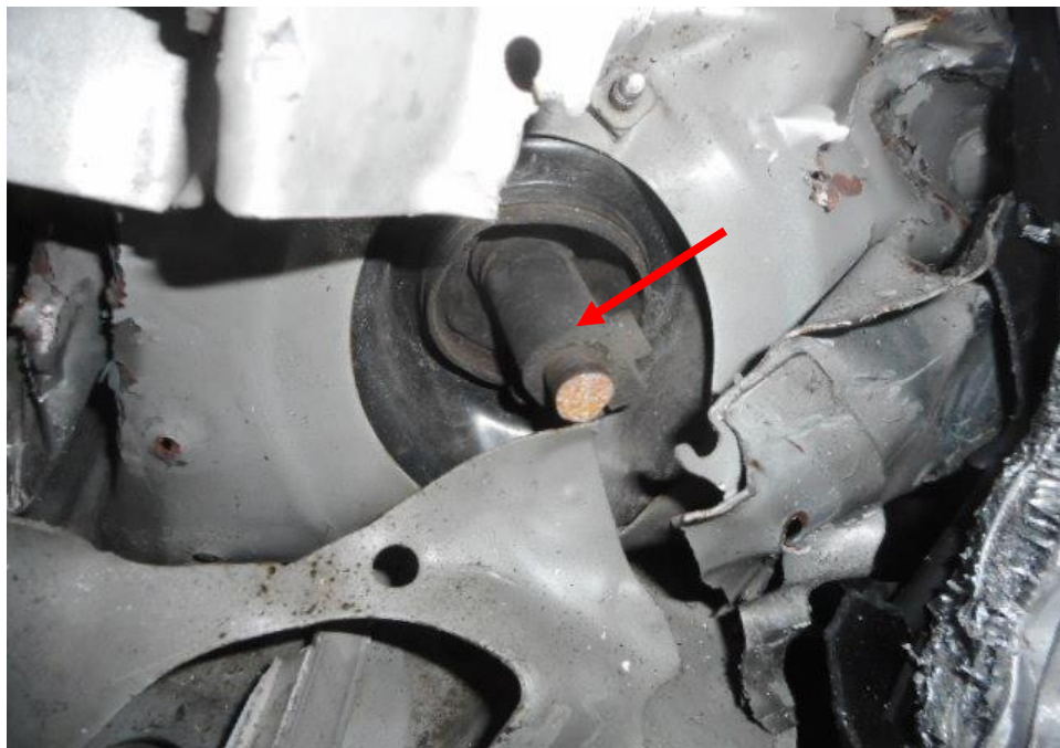
Photo 18 shows the steering box shaft (arrowed) of the Motor Van's steering system. The steering box was observed to sustained damages a result of the accident.
