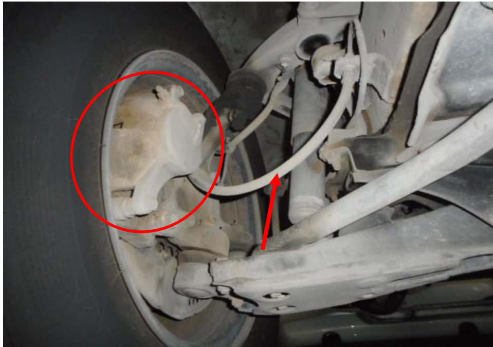
Photo 25 shows the brake hose/pipe (arrowed) at the front left wheel of the Motor Van. No leakage of brake fluid was observed. Visual examination of the various components of the braking system like the brake caliper (circled), brake booster, brake pedal etc had revealed all to be intact and without visible damage at the time of accident. There was also no sign of fluid stain(s) observed on the various undercarriage components.
