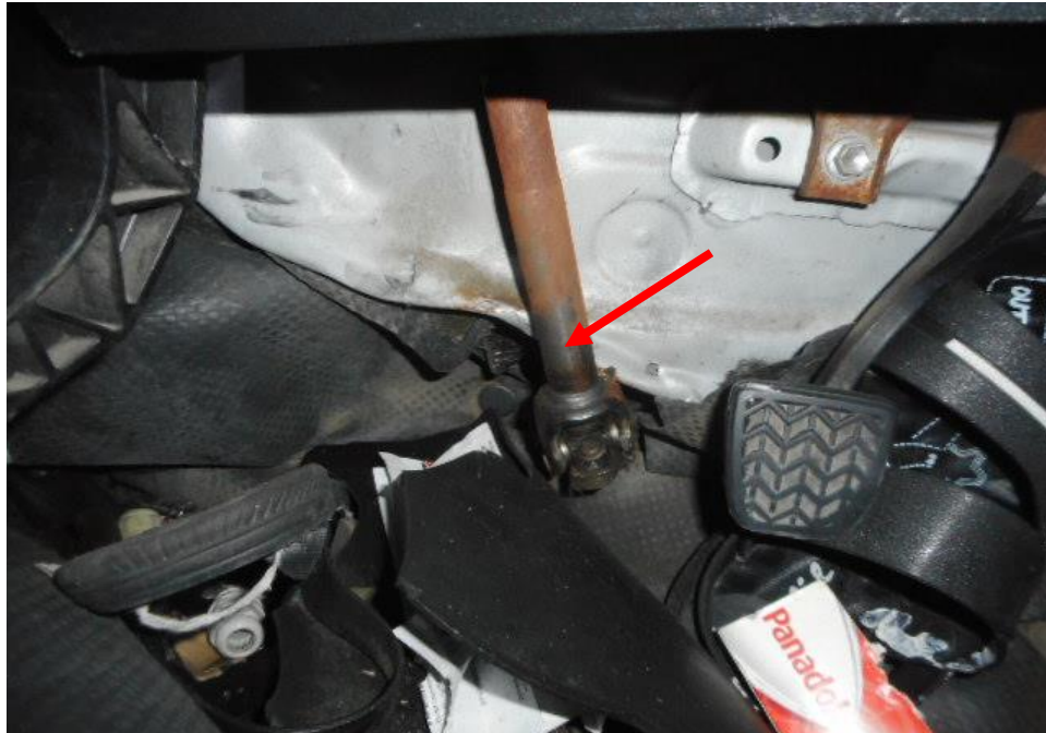
Photo 19 shows the steering box shaft (arrowed) of the Motor Van's steering system. The steering box was observed to sustained damages a result of the accident.
