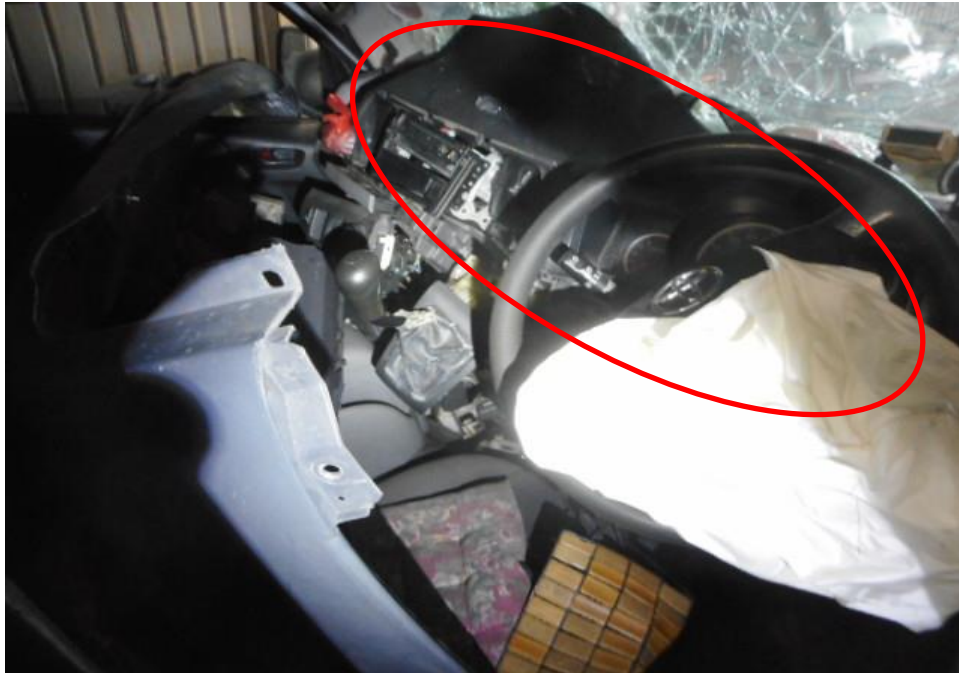
Photo 1 shows the close up view of the front portion of the Motor Van at the time of our inspection. The Motor Van was observed to have sustained major damages to its dashboard (circled) that was crushed due to the accident's impact.
