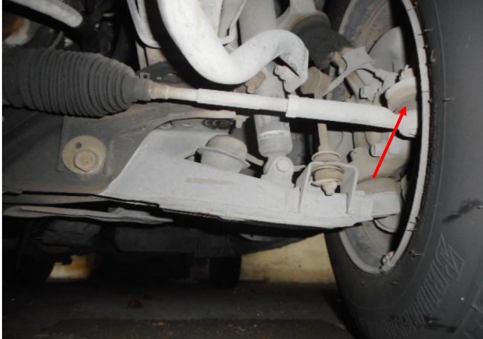
Photo 21 shows the various undercarriage components at the front left wheel of the Motor Van, in particular the steering tie rod end (arrowed). The various undercarriage components of the Motor Van were all found to be intact without any visible damage. There was also no sign of fluid stain(s) observed on the various undercarriage components.
