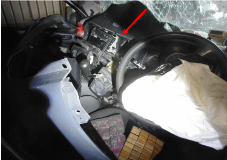
Photo 16 shows the induced damage to the dashboard of the front cabin (arrowed) of the Motor Van's which had immobilised the opening and viewing of the various parts and components inside the engine compartment a result of the accident.
