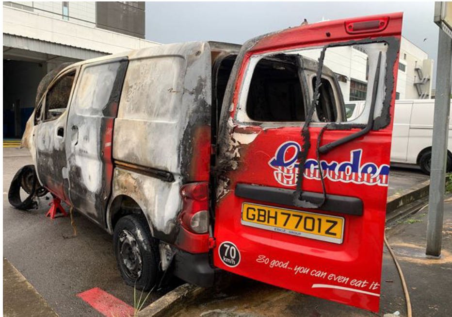
Photo 1 shows the general view of the left rear portion of the Insured Vehicle at the time of our inspection. The Insured Vehicle was observed to have sustained extensive fire damage all around. Rust had accumulated all over the Insured Vehicle as a result of exposure to environmental condition for a period of time.
