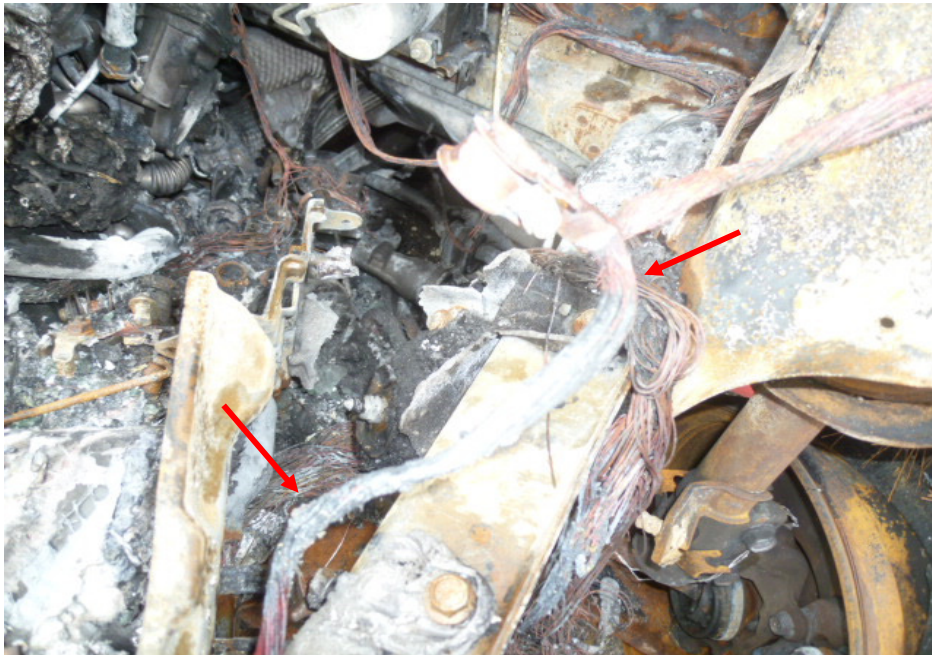
Photo 9 shows a closer view of the greenish residue found on several stretches of burnt wirings leading from the ECM (red arrows). The presence of such greenish residue suggests occurrence of an electrical short circuit.
