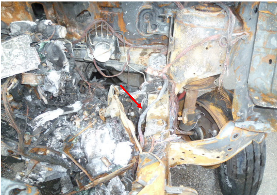
Photo 8 shows a closer view of the burnt wirings leading from the ECM around the left portion of the engine compartment, which is in the immediate vicinity where the fire to the Insured Vehicle had likely started. We noticed greenish residue on several stretches of burnt wirings (arrowed). The presence of greenish residue indicates internal heating of copper wires, a sign of an electrical short circuit occurring. The greenish residue is normally left behind from oxidation as a result of chemical reaction involving the copper wires.
