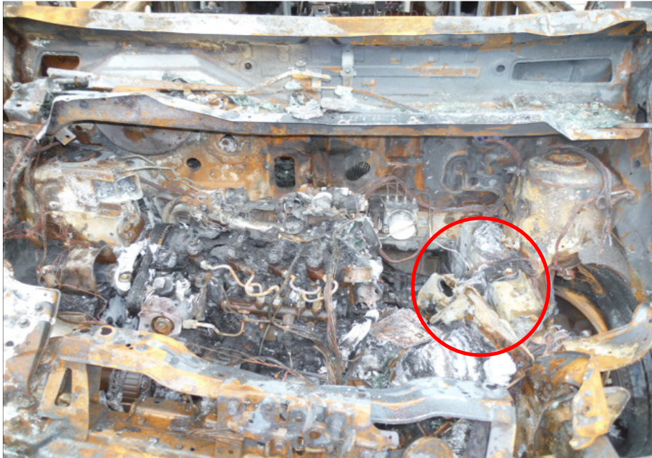
Photo 7 shows the burnt wirings leading from the ECM around the left portion of the engine compartment (circled), which is in the immediate vicinity where the fire to the Insured Vehicle had likely started.
