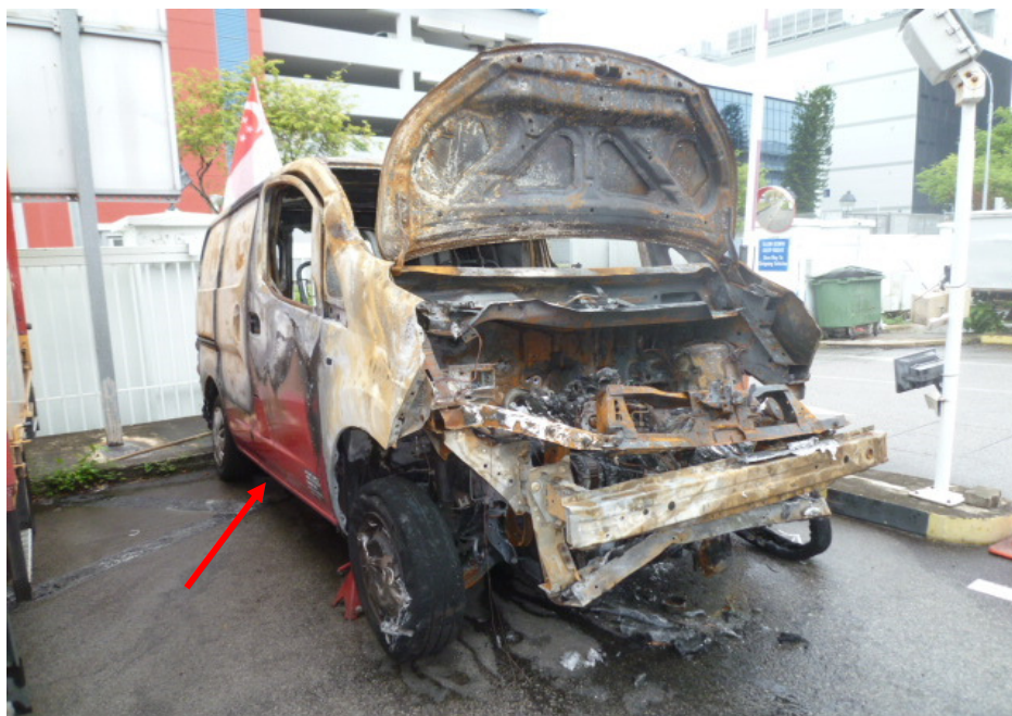
Photo 5 shows the right body of the Insured Vehicle. The nature of the fire damage was less extensive at the right portion (arrowed).
