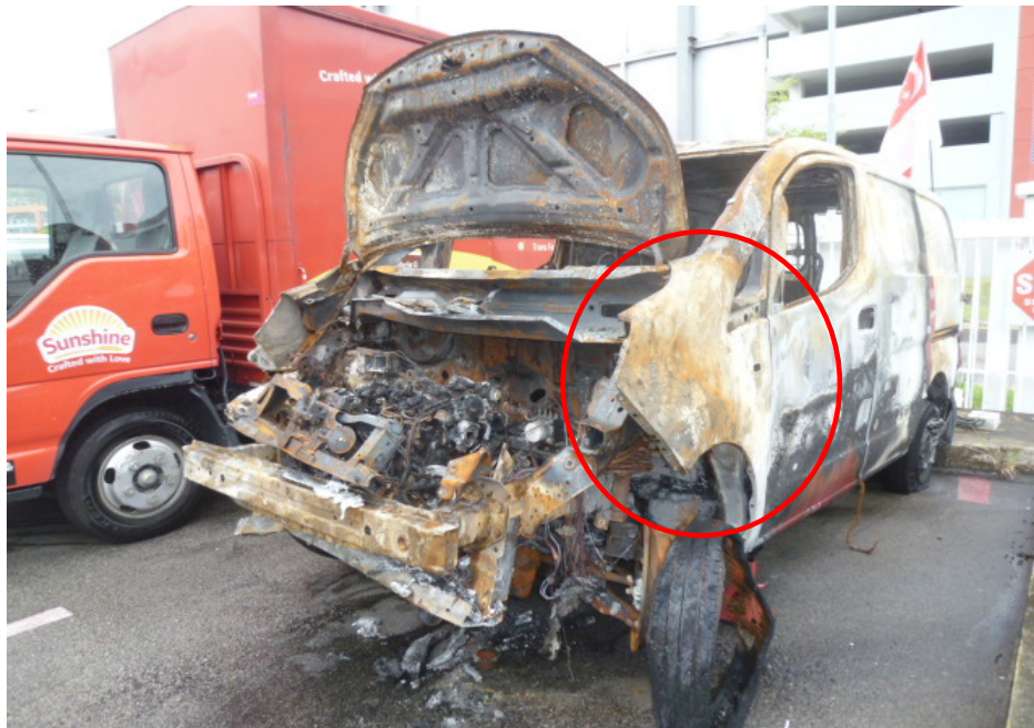
Photo 6 shows the burn pattern and whitish burn marks that were found on the left front fender of the Insured Vehicle (circled). Such whitish burn marks are a result of exposure to prolonged heat intensity, which may indicate where the fire had started.
