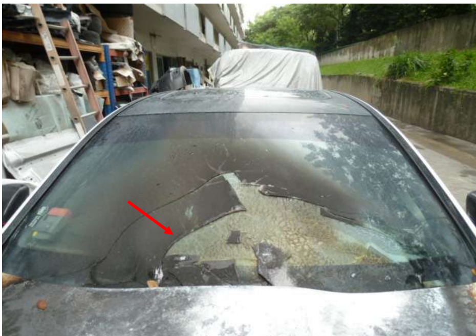
Photo 4 shows a closer view of the front windscreen of the Insured Vehicle at the time of our inspection. The front windscreen had sustained extensive fire damage (arrowed).
