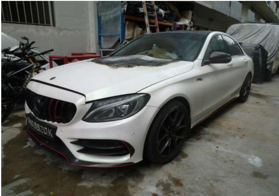
Photo 3 shows the general view of the left portion of the Insured Vehicle at the time of our inspection. The exterior body of the Insured Vehicle had sustained visible fire damage. This included its front windscreen, front bonnet, front windscreen wiper garnish and front windscreen wipers.
