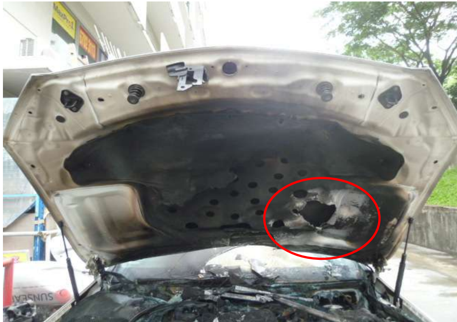
Photo 11 shows the rust that had developed on the underside of the front bonnet, around the bottom centre portion (circled). The development of rust is an indication that this area was subjected to prolonged exposure to high heat intensity, which had caused the steel/metal material of the front bonnet to be exposed to natural environmental condition. Hence the fire to the Insured Vehicle can be determined to have originated towards the rear centre portion of the engine compartment.
