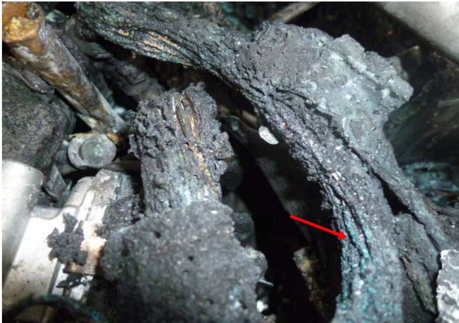
Photo 16 shows a close up view of the greenish residue on the wirings leading from the ECM of the Insured Vehicle (red arrows). The presence of such greenish residue suggests occurrence of an electrical short circuit.
