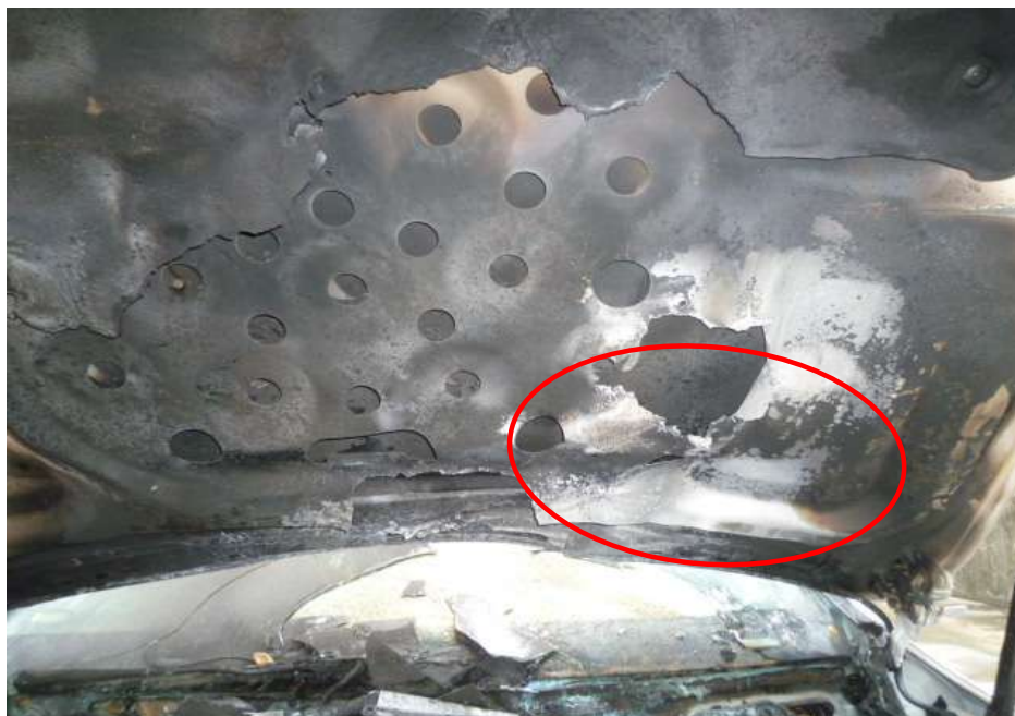
Photo 12 shows a closer view of the rust that had developed on the underside of the front bonnet, around the bottom centre portion (circled).
