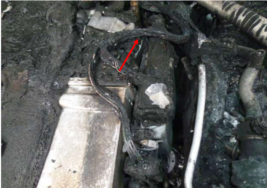
Photo 14 shows a closer view of the greenish residue on some of the burnt wirings leading from the ECM (arrowed).
