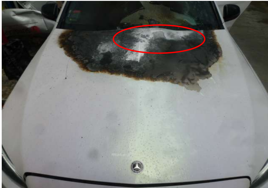
Photo 9 shows the burn pattern and whitish burn marks that were found on the rear centre portion of the front bonnet of the Insured Vehicle (circled). Such whitish burn marks are a result of exposure to prolonged heat intensity, which may indicate where the fire had started. Rust would also begin to develop on these areas soon after the fire.
