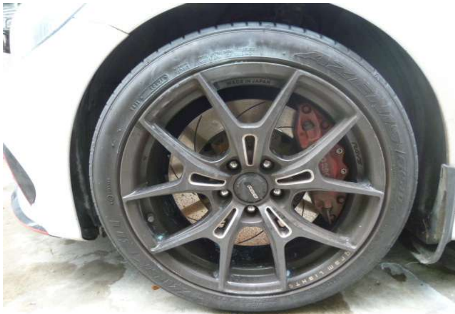
Photo 8 shows the non-standard rim found to be fitted on the Insured Vehicle at the time of our inspection. The 18- inch alloy rims fitted on the Insured Vehicle were not the standard type for the Insured Vehicle.
