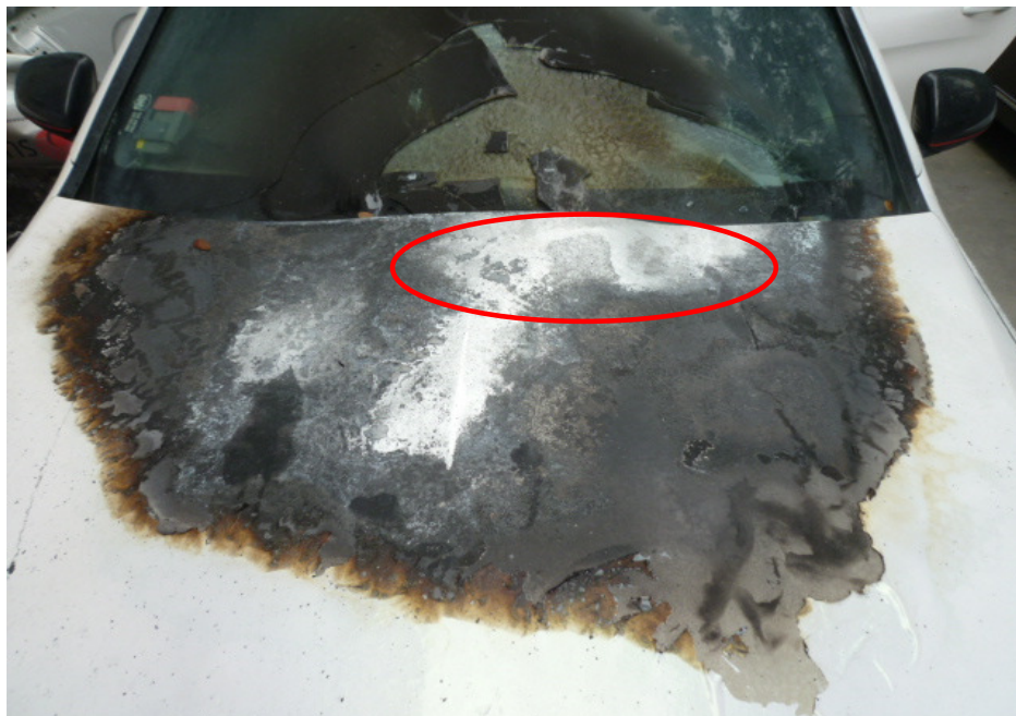
Photo 10 shows a closer view of the burn pattern and whitish burn marks that were found on the rear centre portion of the front bonnet of the Insured Vehicle (circled).
