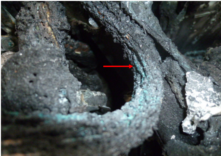
Photo 17 shows a close up view of the greenish residue on the wirings leading from the ECM of the Insured Vehicle (red arrows). The presence of such greenish residue suggests occurrence of an electrical short circuit.
