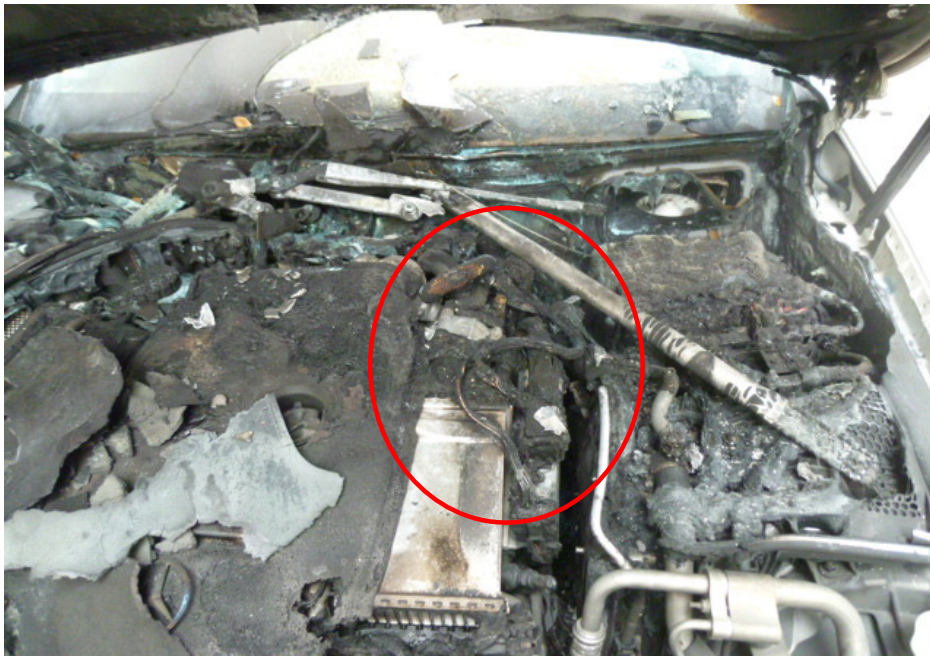
Photo 13 shows the wirings around the rear centre portion of the engine compartment which is near to the vicinity where the fire to the Insured Vehicle had likely started. We observed greenish residue on the wirings leading from the Engine Control Module (ECM) of the Insured Vehicle (circled). The presence of greenish residue indicates internal heating of copper wires, a sign of an electrical short circuit occurring. The greenish residue is normally left behind from oxidation as a result of chemical reaction involving the copper wires.
