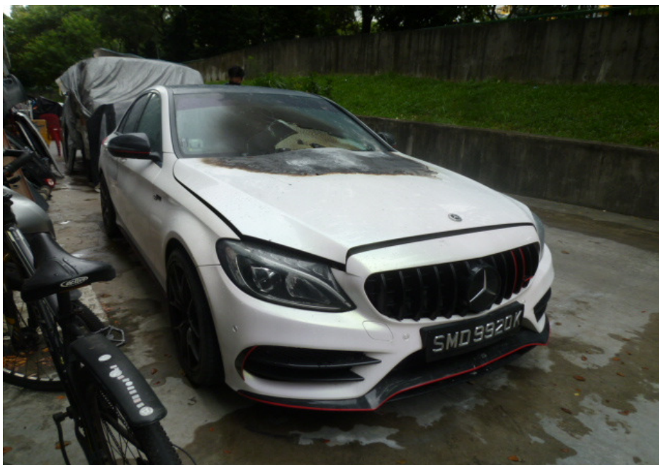
Photo 2 shows the general view of the right frontal portion of the Insured Vehicle at the time of our inspection. The exterior body of the Insured Vehicle had sustained visible fire damage. This included its front windscreen, front bonnet, front windscreen wiper garnish and front windscreen wipers.
