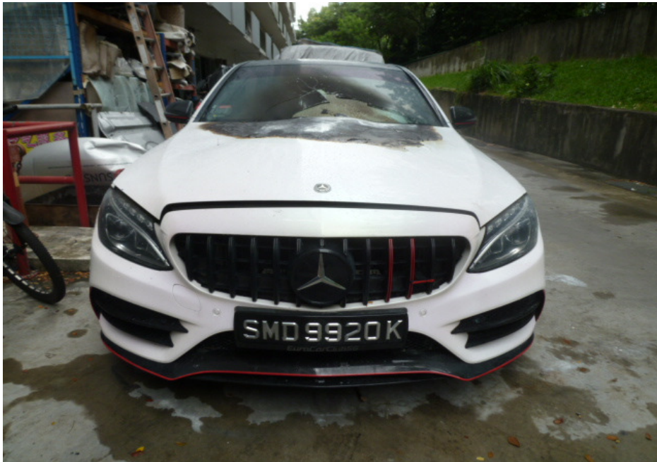
Photo 1 shows the general view of the frontal portion of the Insured Vehicle at the time of our inspection. The exterior body of the Insured Vehicle had sustained visible fire damage. This included its front windscreen, front bonnet, front windscreen wiper garnish and front windscreen wipers.
