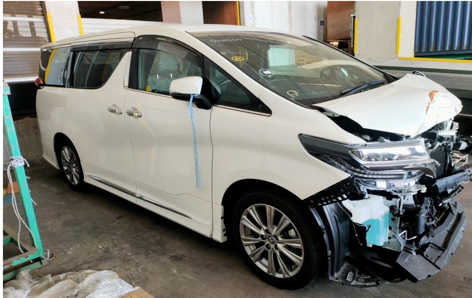
Photo 1 shows the front right body of the Motor Car (photograph provided to me). The photographs provided to me had showed damage to the frontal portion of the Motor Car. The front bumper, front bumper sensors, front bumper right chrome moulding, front bumper right lower grille, front right fog lamp, front right fender, front right headlamp and front bonnet were amongst the body parts that were observed to have been damaged. The airbag(s) of the Motor Car was not deployed as seen from the photographs that were provided to me.
