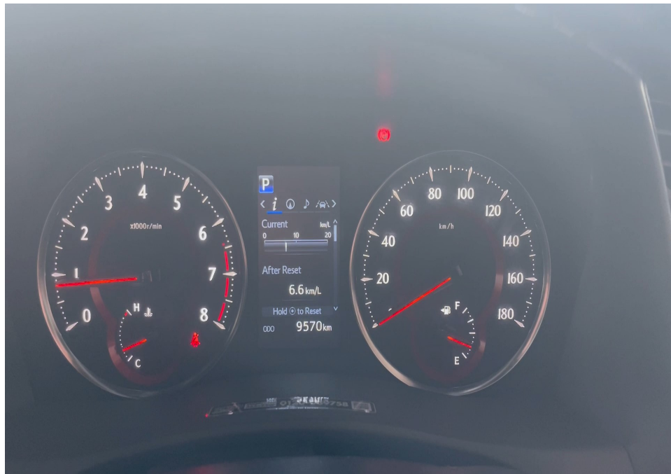
Photo 23 shows the respective warning lights no longer illuminated, indicating that there is no fault detected to the ABS, SRS, EPS, VSC systems of the Motor Car during the self-test. These electronic systems were hence in working condition at the time of my inspection.
