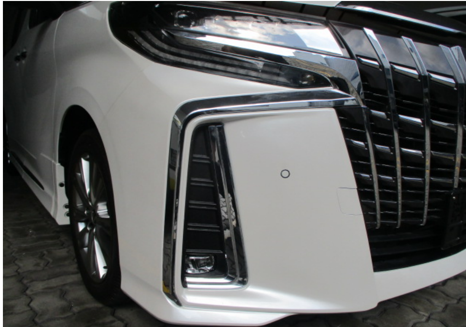
Photo 8 shows a closer view of the Motor Car's front bumper, front bumper right sensor, front bumper right chrome moulding, front bumper right lower grille and front right fog lamp. The body parts at the frontal portion of the Motor Car were visually examined and it was observed that the repair/restoration works carried out to the damaged area of the Motor Car (refer to photograph 1 - 3 above) were reasonably adequate and in order.
