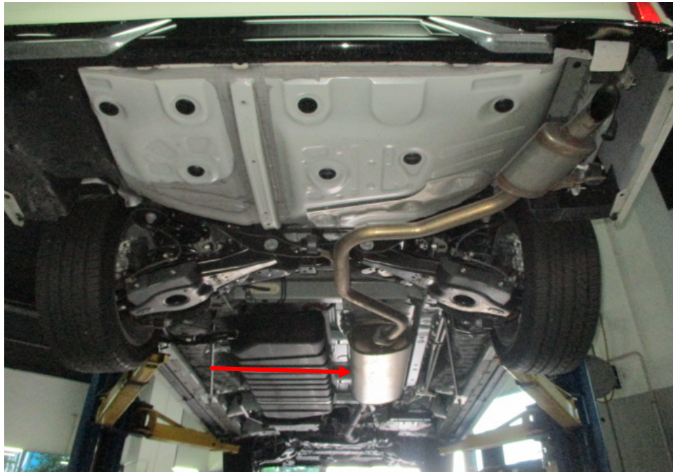
Photo 29 shows the rear section of the Motor Car's exhaust system. My examination of the Motor Car's exhaust system revealed no sign(s) or indication(s) of any cut or weld marks along its exhaust pipes, on its rear muffler, on its centre resonator box (arrowed) and on its catalytic converter.
