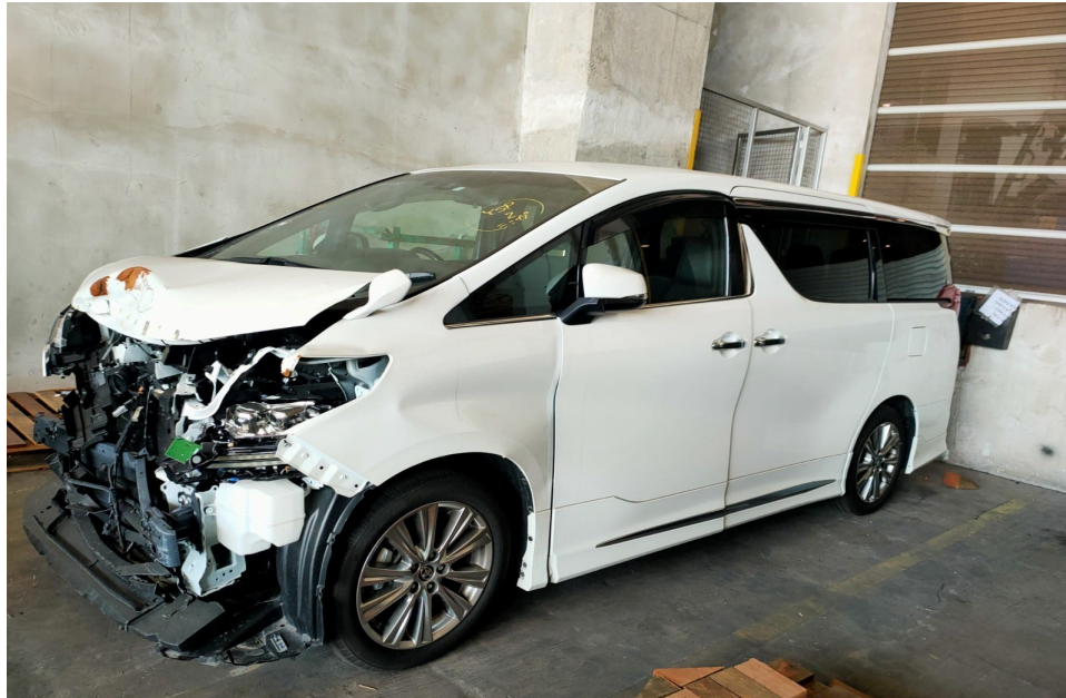
Photo 3 shows the front left body of the Motor Car (photograph provided to me). The photographs provided to me had showed damage to the frontal portion of the Motor Car. The front bumper, front bumper sensors, front bumper left chrome moulding, front bumper left lower grille, front left fog lamp, front left fender, front left headlamp, front left headlamp top panel, radiator grille, front bonnet and front bonnet lock were amongst the body parts that were observed to have been damaged. The airbag(s) of the Motor Car was not deployed as seen from the photographs that were provided to me.
