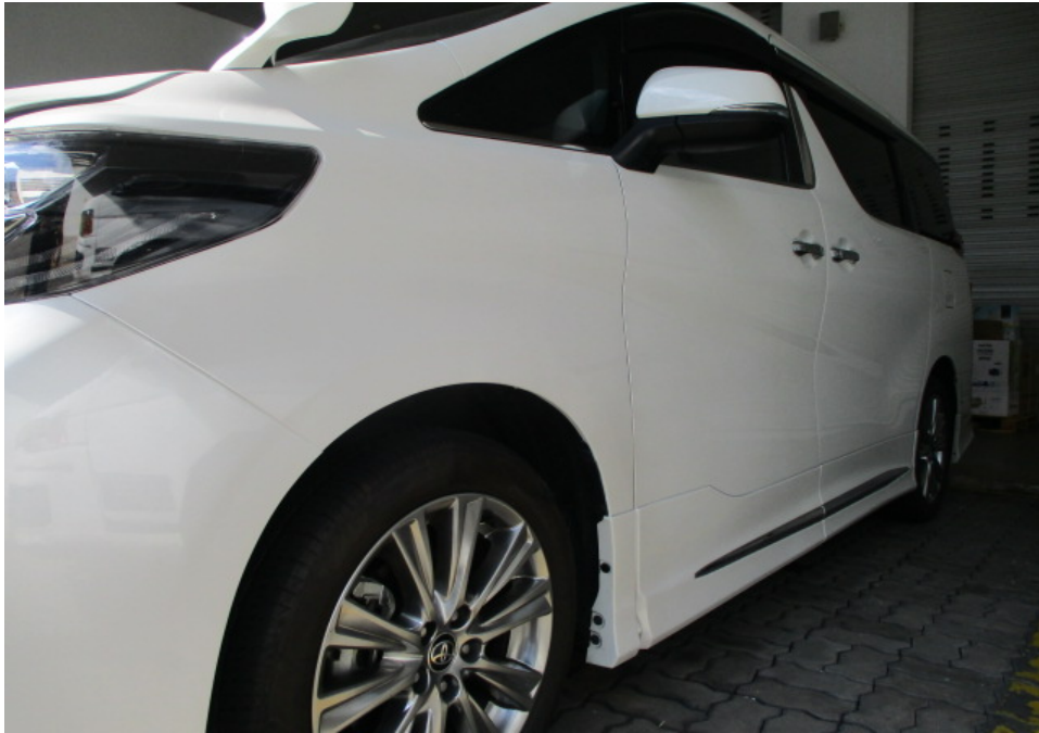
Photo 12 shows a closer view of the Motor Car's front left fender, front left wheel rim and front left door. The body parts at the frontal portion of the Motor Car were visually examined and it was observed that the repair/restoration works carried out to the damaged area of the Motor Car (refer to photograph 1 - 3 above) were reasonably adequate and in order.
