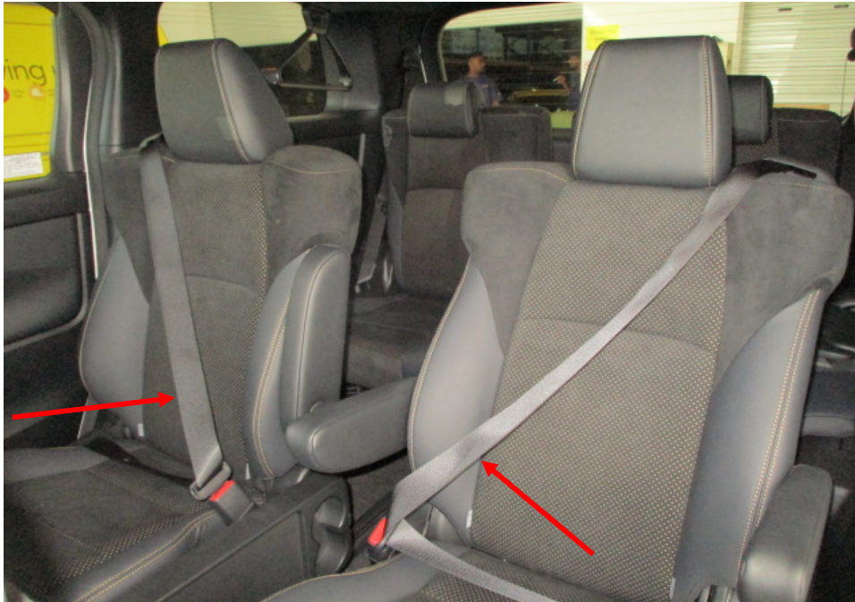
Photo 20 shows the rear seats at the 1 st row of the Motor Car. All the seats of the Motor Car were secured via seat rails to the floorboard. They were also fitted with a retractable seat belt reel and a pre-tensioner. The seat belts (arrowed) were tested and were able to be fastened into the respective pre-tensions that were fitted on the side of each individual seat.
