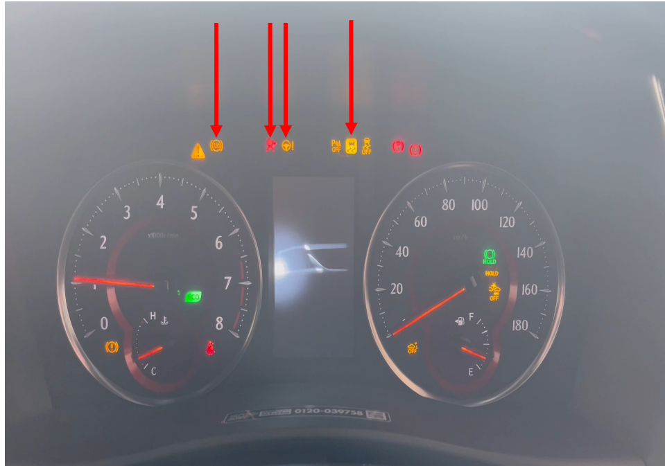
Photo 22 shows the warning lights for the various electronic safety features appearing on the instrument panel of the Motor Car during its self-test when the engine is cranked, in particular the ABS, SRS, EPS, VSC lights (arrowed).
