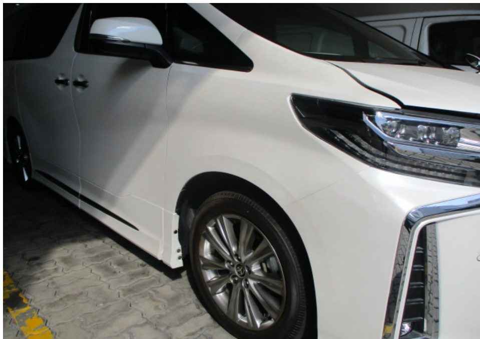
Photo 7 shows a closer view of the Motor Car's front right headlamp, front right fender and front right wheel rim. The body parts at the frontal portion of the Motor Car were visually examined and it was observed that the repair/restoration works carried out to the damaged area of the Motor Car (refer to photograph 1 - 3 above) were reasonably adequate and in order.
