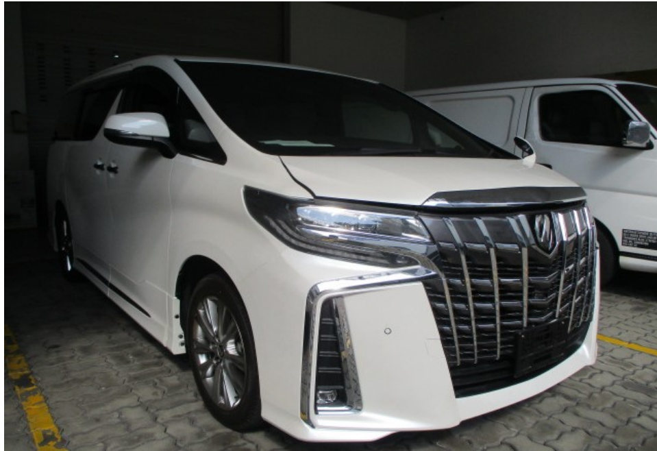
Photo 6 shows a general view of the front right body of the Motor Car at the time of my inspection. The Motor Car was observed to be in a relatively good general condition with no loose exterior fittings observed. The body parts at the frontal portion of the Motor Car were visually examined and it was observed that the repair/restoration works carried out to the damaged area of the Motor Car (refer to photograph 1 - 3 above) were reasonably adequate and in order.
