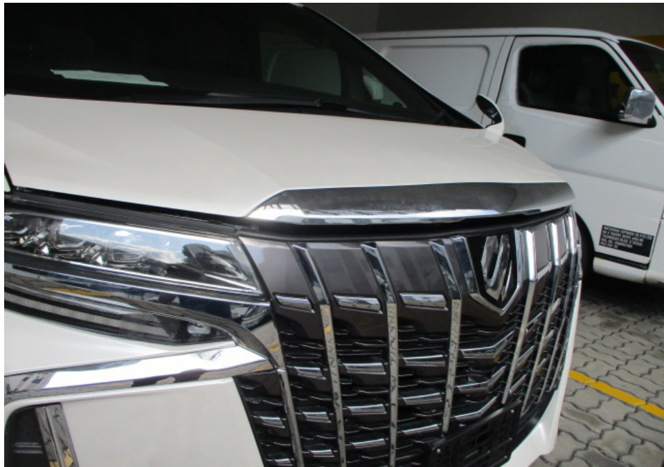
Photo 9 shows a closer view of the Motor Car's front right headlamp, front bonnet, front bonnet chrome moulding and radiator grille. The body parts at the frontal portion of the Motor Car were visually examined and it was observed that the repair/restoration works carried out to the damaged area of the Motor Car (refer to photograph 1 - 3 above) were reasonably adequate and in order.
