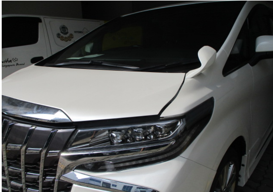
Photo 14 shows a closer view of the Motor Car's front left headlamp, front left fender, front bonnet and front bonnet chrome moulding. The body parts at the frontal portion of the Motor Car were visually examined and it was observed that the repair/restoration works carried out to the damaged area of the Motor Car (refer to photograph 1 - 3 above) were reasonably adequate and in order.
