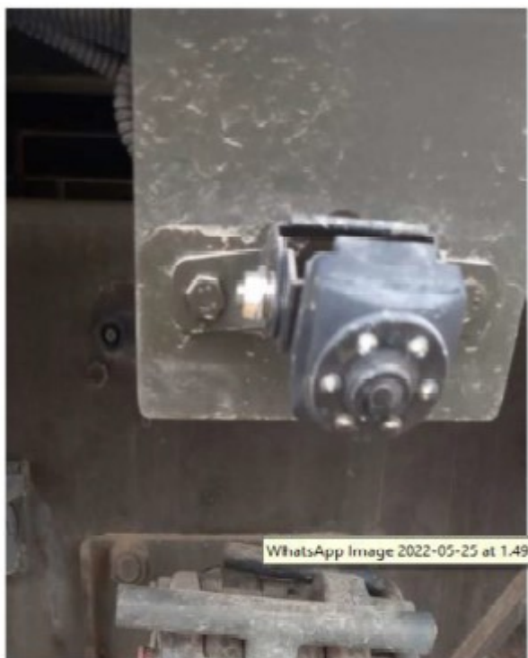
Figure 2G - Mounting bracket of reversing camera of MID20849
