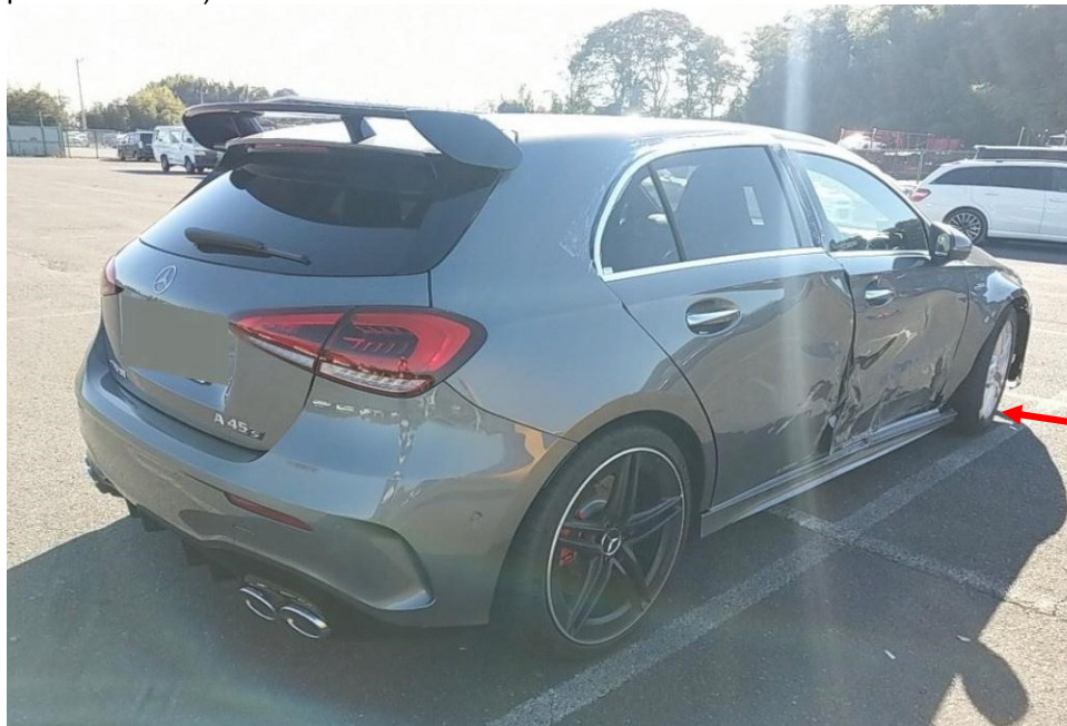
Photo 4 shows the rear right body of the Motor Car (photograph provided to me). The photographs provided to me had showed damage to the right side portion of the Motor Car. The front right door, rear right door and right side rocker panel garnish were amongst the body parts that were observed to have been damaged. The front right wheel (arrowed) was orientated slightly towards the left as compared to the front left wheel (refer to photograph 5 below), which was orientated in a straight direction. This would indicate damage to the undercarriage parts at the front right wheel of the Motor Car given that the front right wheel rim was seen to be different from the other wheel rims that were fitted on the Motor Car.
