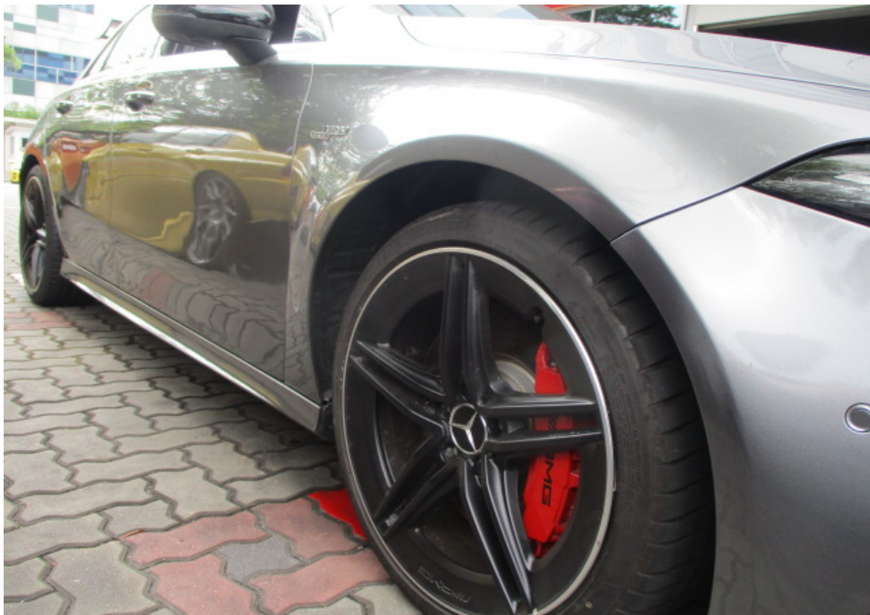
Photo 9 shows a closer view of the Motor Car's front bumper, front right wheel rim, front right fender and right side rocker panel garnish. The body parts at the right side portion of the Motor Car were visually examined and it was observed that the repair/restoration works carried out to the damaged area of the Motor Car (refer to photograph 1 - 3 above) were reasonably adequate and in order.
