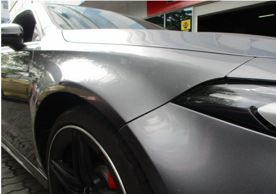
Photo 8 shows a closer view of the Motor Car's front bumper, front right headlamp and front right fender. The body parts at the right side portion of the Motor Car were visually examined and it was observed that the repair/restoration works carried out to the damaged area of the Motor Car (refer to photograph 1 - 3 above) were reasonably adequate and in order.
