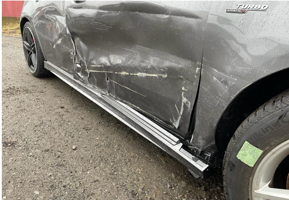
Photo 3 shows a closer view of the damaged front right fender, front right door, rear right door and right side rocker panel garnish of the Motor Car (photograph provided to me).
