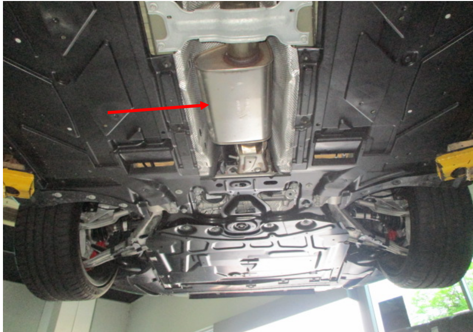
Photo 26 shows the front section of the Motor Car's exhaust system. My examination of the Motor Car's exhaust system revealed no sign(s) or indication(s) of any cut or weld marks along its exhaust pipes, on its rear muffler, on its centre resonator box (arrowed) and on its catalytic converter.
