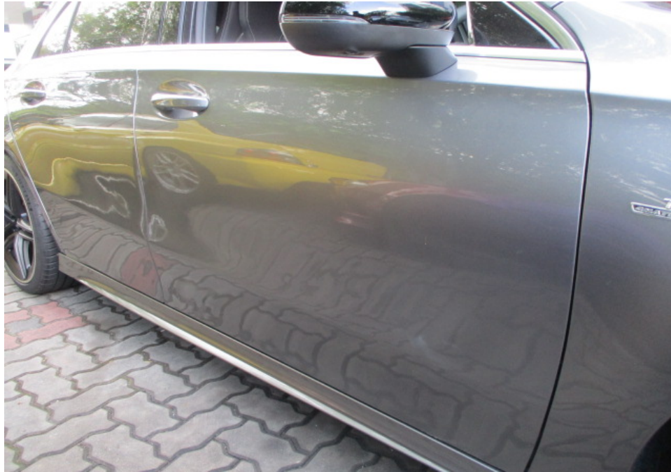
Photo 10 shows a closer view of the Motor Car's front right door, rear right door and right side rocker panel garnish. The body parts at the right side portion of the Motor Car were visually examined and it was observed that the repair/restoration works carried out to the damaged area of the Motor Car (refer to photograph 1 - 3 above) were reasonably adequate and in order.
