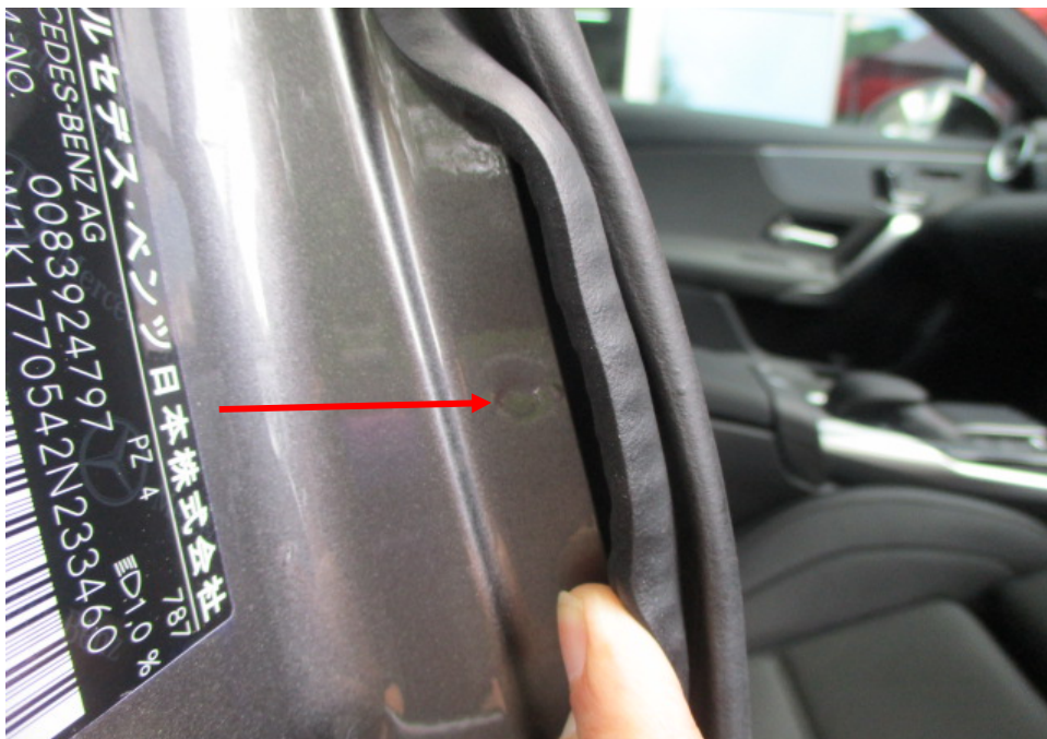
Photo 33 shows the right side “B” pillar of the Motor Car. I did not find any weld marks other than original spot weld marks (arrowed) on the right side “B” pillar of the Motor Car, which indicates that there was no re-welding works carried out. In general, I had found all the non-detachable body panels of the Motor Car to be originally fitted at the time of my inspection.
