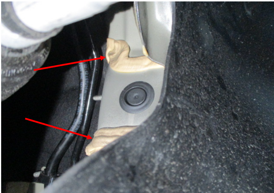
Photo 29 shows the chassis/structural body at the underside front left of the Motor Car. I did not find any weld marks other than original spot weld marks on the chassis/structural body of the Motor Car. The original factory sealant (arrowed) at the joints along the chassis/structural body was untouched, indicating no work was done on the chassis/structural body of the Motor Car and that the chassis/structural body was originally fitted.
