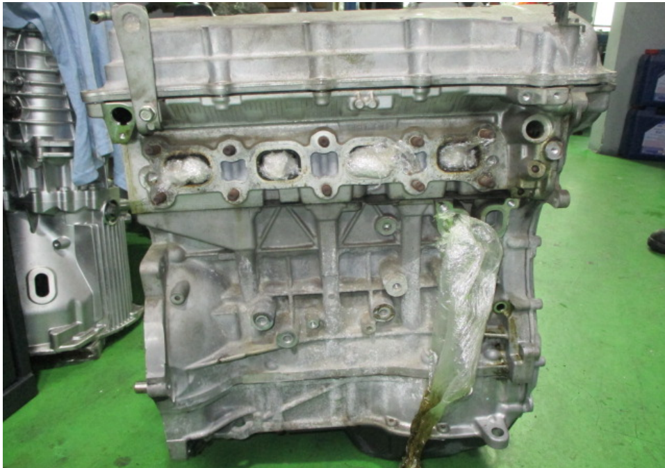
Photo 2 shows a closer view of the Mitsubishi engine that I had inspected. My visual examination of the engine housing revealed the housing to be of serviceable/satisfactory condition. There was no crack and/or hole observed on the engine housing.
