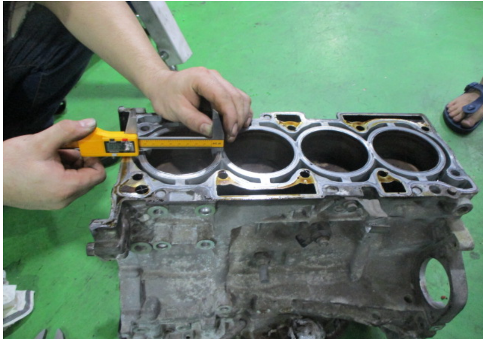
Photo 7 shows measurement being carried out to the bore of cylinder 1 of the Mitsubishi engine. The measurements were carried out using a digital Vernier Caliper that was calibrated before the start of the measurements.
