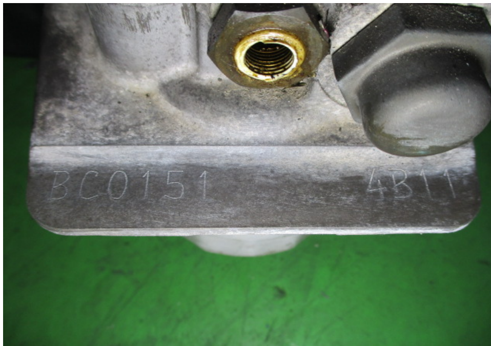
Photo 4 shows the engine number engraved on the housing of the Mitsubishi engine that I had inspected. The engine number was 4B11BC0151.
