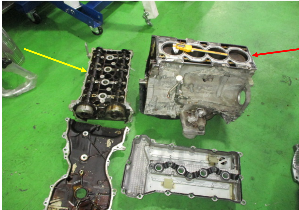
Photo 5 shows the top block (yellow arrow) of the Mitsubishi engine separated from its bottom block (red arrow). This was to enable me to carry out measurements of its cylinders, in particular the bore and stroke measurements of each cylinder, which typically can be used to determine the engine displacement or more commonly referred to as engine cc.
