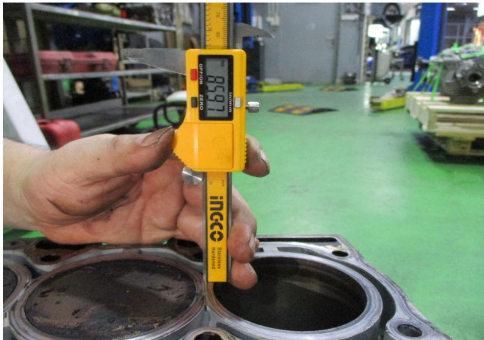
Photo 20 shows the stroke measurement of cylinder 4, which was recorded to be 85.97mm.
