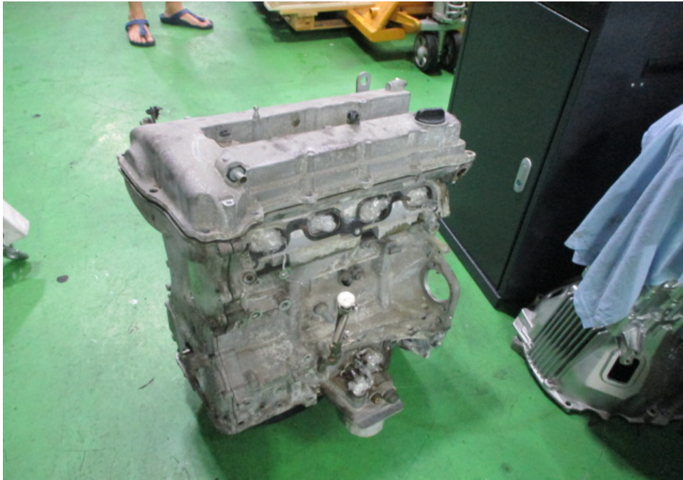
Photo 1 shows a general view of the Mitsubishi engine that I had inspected. The Mitsubishi engine was observed to be a used engine and was not fitted on any motor car. It was also observed to be a complete assembly with all mechanical parts still intact, within the engine housing.
