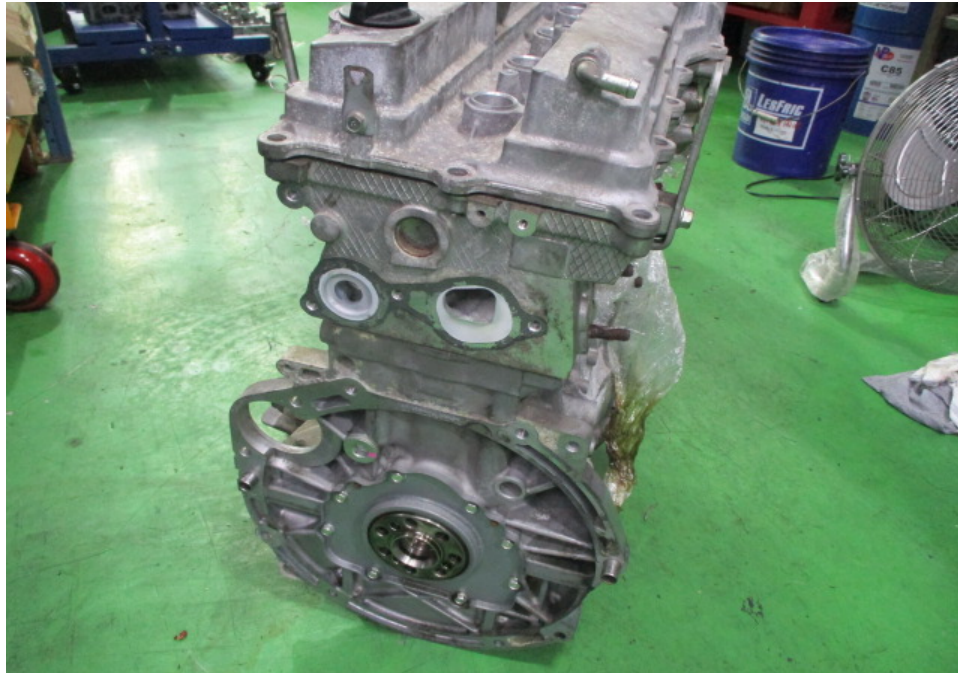
Photo 3 shows another view of the Mitsubishi engine that I had inspected. My visual examination of the engine housing revealed the housing to be of serviceable/satisfactory condition. There was no crack and/or hole observed on the engine housing.
