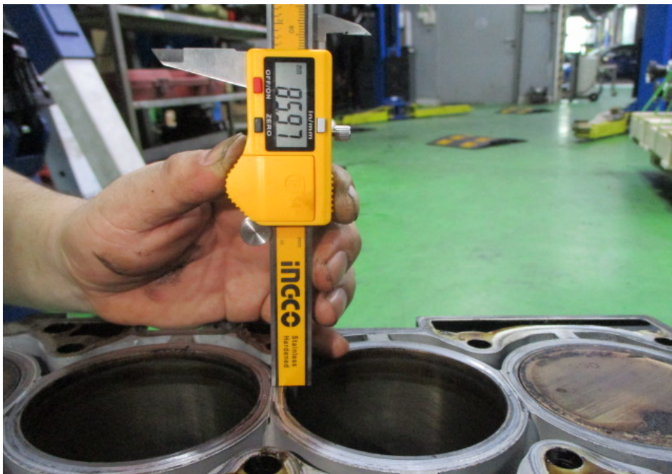
Photo 16 shows the stroke measurement of cylinder 3, which was recorded to be 85.97mm.
