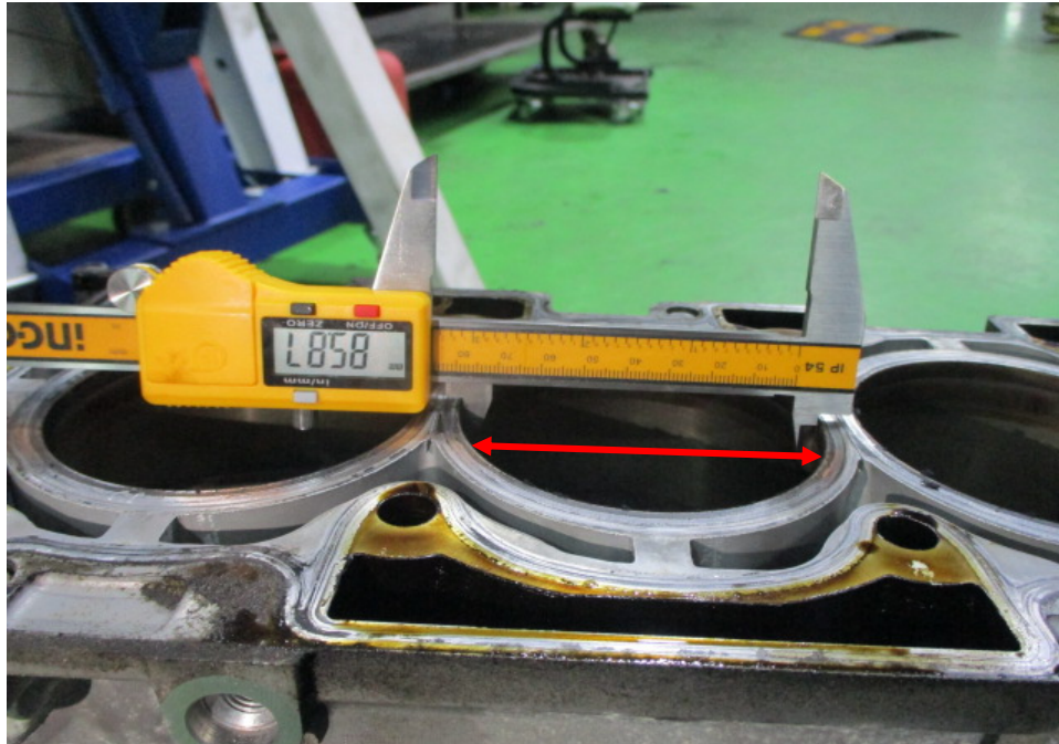
Photo 11 shows measurement being carried out to the bore (arrowed) of cylinder 2 of the Mitsubishi engine. The bore measurement of cylinder 2 was recorded to be 85.87mm.
