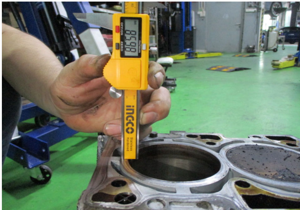
Photo 10 shows the stroke measurement of cylinder 1, which was recorded to be 85.98mm.
