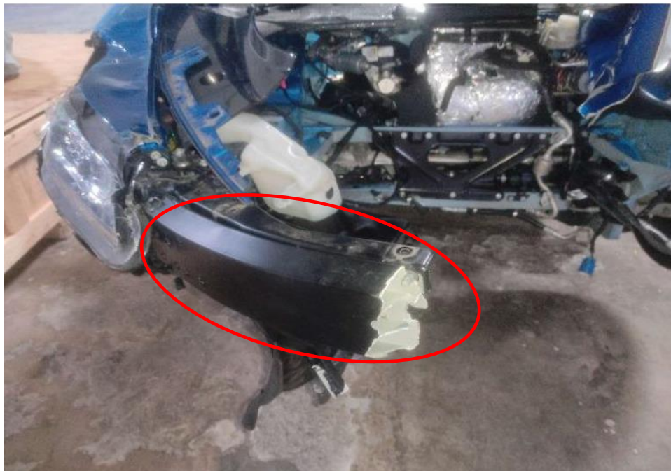
Photo 3 shows the close up view of the front portion of the Insured Vehicle at the time of our inspection. Its front bumper (circled) was the body parts that were damaged as a result of the accident.
