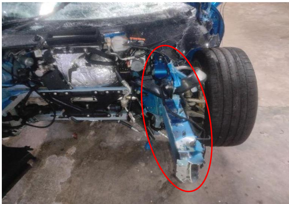
Photo 4 shows the close up view of the front portion of the Insured Vehicle at the time of our inspection. Its front vehicle chassis (circled) was the body parts that were damaged as a result of the accident.
