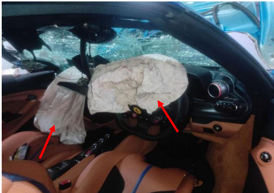
Photo 7 shows the close up view of the interior portion of the Insured Vehicle at the time of our inspection. Its airbag's deployed (circled) as a result of the accident.
