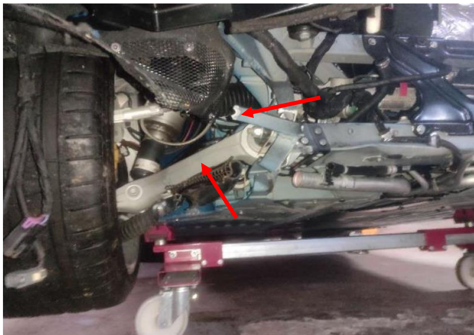
Photo 6 shows the close up view of the undercarriage portion of the Insured Vehicle at the time of our inspection. Its undercarriage suspension components (arrowed) were also damaged as a result of the accident.
