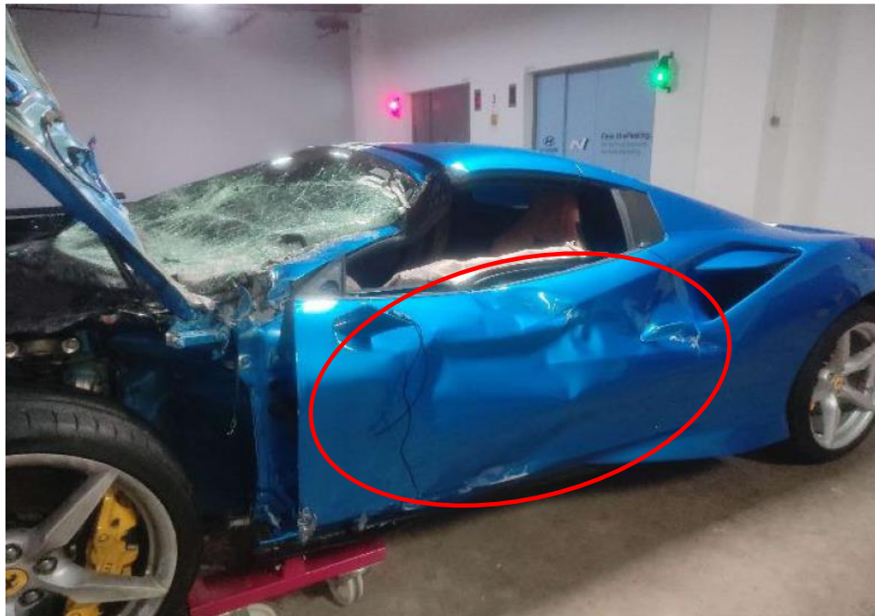
Photo 5 shows the close up view of the left portion of the Insured Vehicle at the time of our inspection. Its left door panel (circled) was the body parts that were damaged as a result of the accident.
