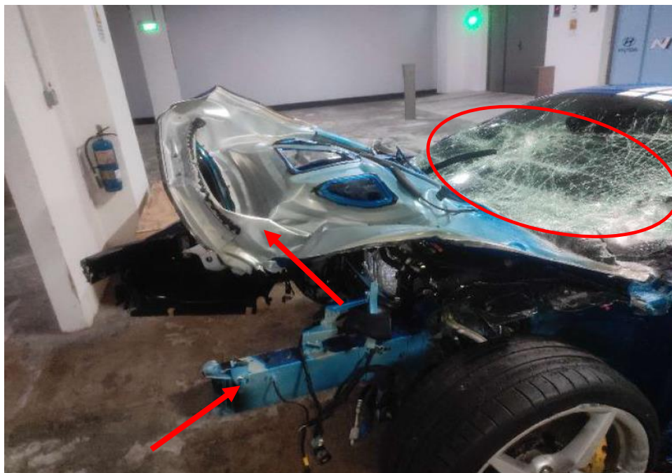
Photo 2 shows the close up view of the front portion of the Insured Vehicle at the time of our inspection. Its front windscreen (circled) and front bonnet (arrowed) was the body parts that were damaged as a result of the accident.
