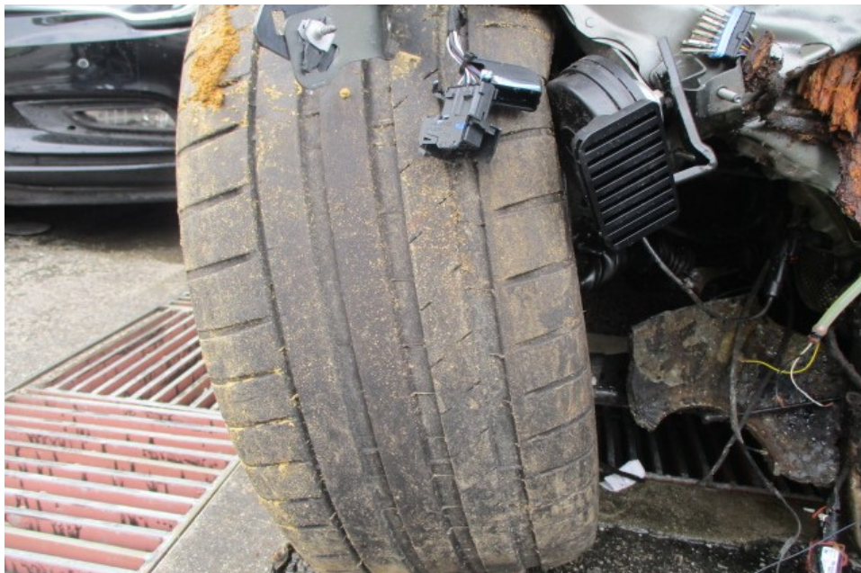
Photo 9 shows the condition of the Insured Vehicle's front right tyre. The front right tyre of the Insured Vehicle was found to be in serviceable condition given that the tread pattern was clearly visible.
