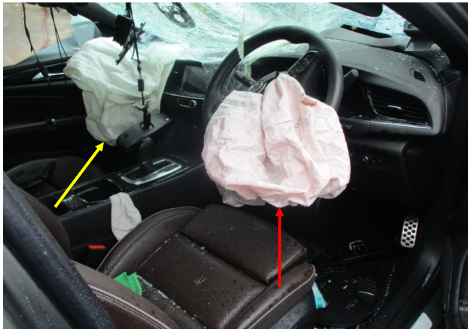
Photo 16 shows the interior compartment of the Insured Vehicle at the time of my inspection. The driver's airbag (red arrow) and front left passenger airbag (yellow arrow) were activated.
