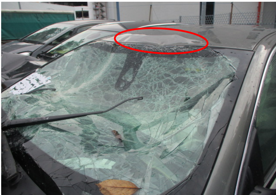
Photo 6 shows the front windscreen of the Insured Vehicle badly cracked. The roof panel was also observed to be dented (circled).
