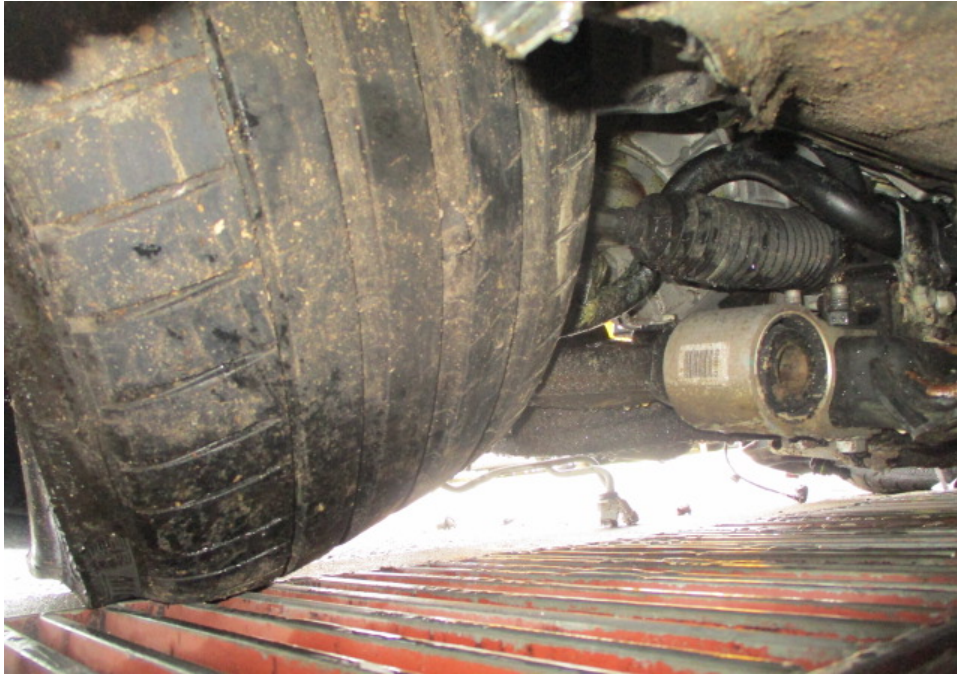
Photo 14 shows the condition of the undercarriage parts at the front left wheel of the Insured Vehicle. The undercarriage parts at the front left wheel of the Insured Vehicle were found to be damage as a result of the accident. The damage had prevented me from carrying out any meaningful tests to the steering system and braking system of the Insured Vehicle.
