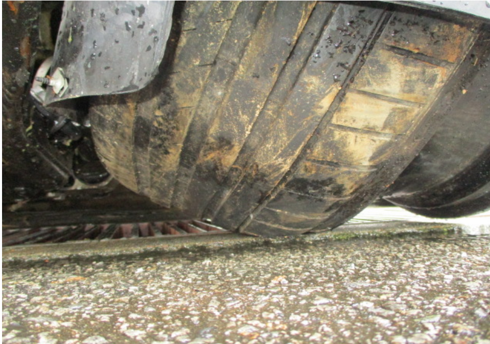
Photo 10 shows the condition of the Insured Vehicle's front left tyre. The front left tyre of the Insured Vehicle was found to be in serviceable condition given that the tread pattern was clearly visible.
