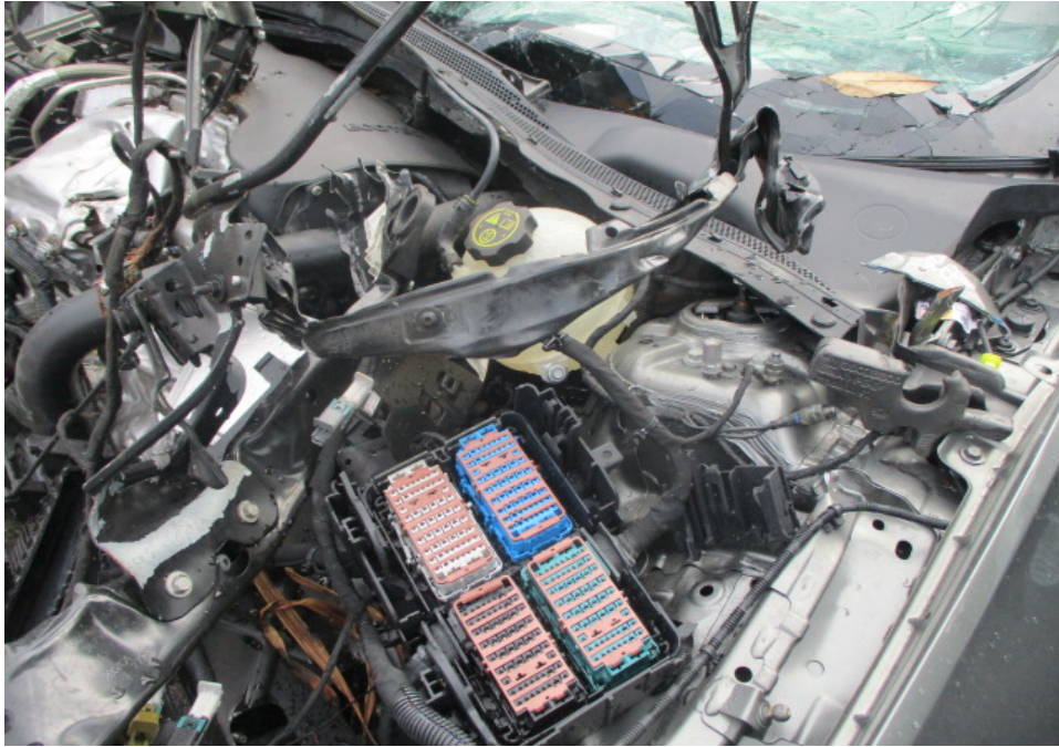
Photo 5 shows the engine fuse box, engine wiring harness, pipes and hoses within the engine compartment of the Insured Vehicle that were found to be damaged.
