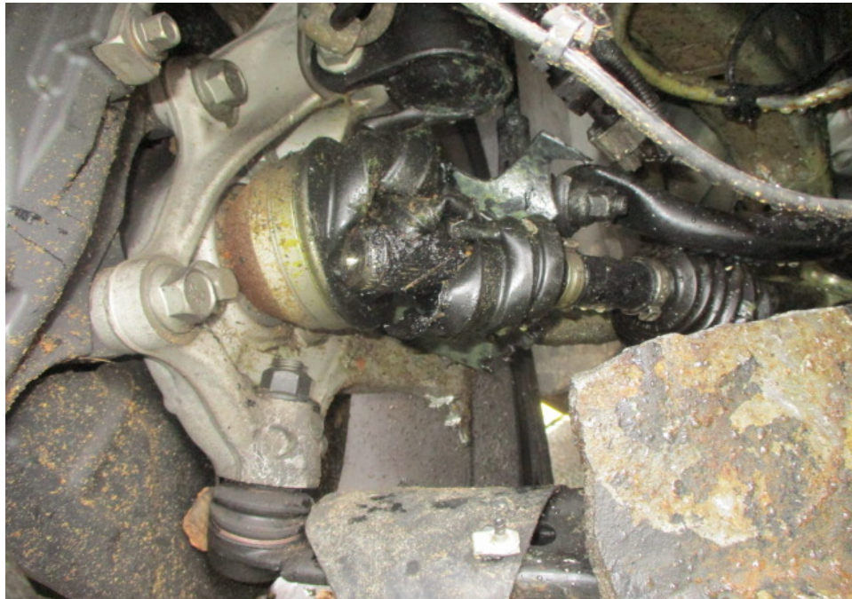
Photo 13 shows the condition of the undercarriage parts at the front right wheel of the Insured Vehicle. The undercarriage parts at the front right wheel of the Insured Vehicle were found to be damage as a result of the accident. The damage had prevented me from carrying out any meaningful tests to the steering system and braking system of the Insured Vehicle.
