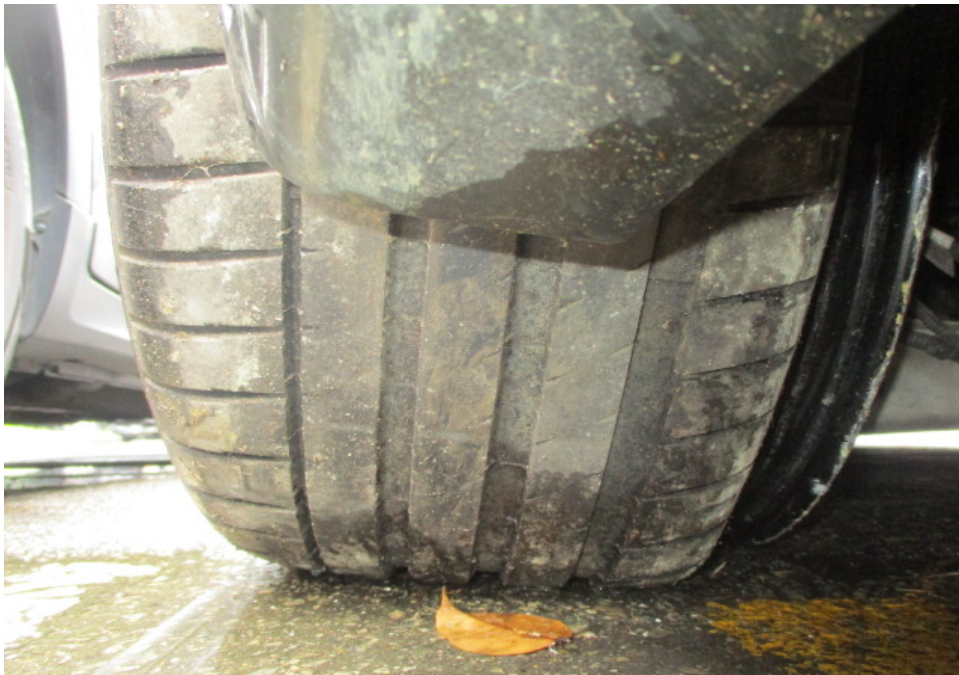
Photo 11 shows the condition of the Insured Vehicle's rear left tyre. The rear left tyre of the Insured Vehicle was found to be in serviceable condition given that the tread pattern was clearly visible.
