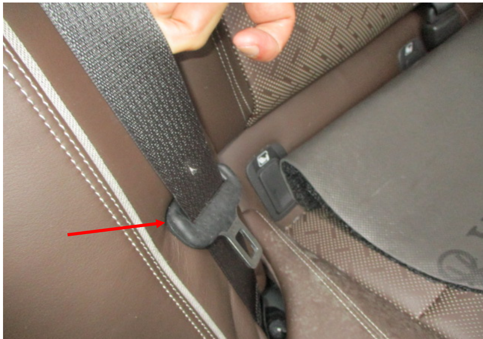
Photo 18 shows the rear passenger seat of the Insured Vehicle at the time of my inspection. The rear right passenger seat belt (arrowed) was activated in an unworn locked position. Apart for this, I had found the rear left passenger seat belt and front left passenger seat belt activated in a similar unworn locked position. As for the driver's seat belt, I had found it to be not activated.
