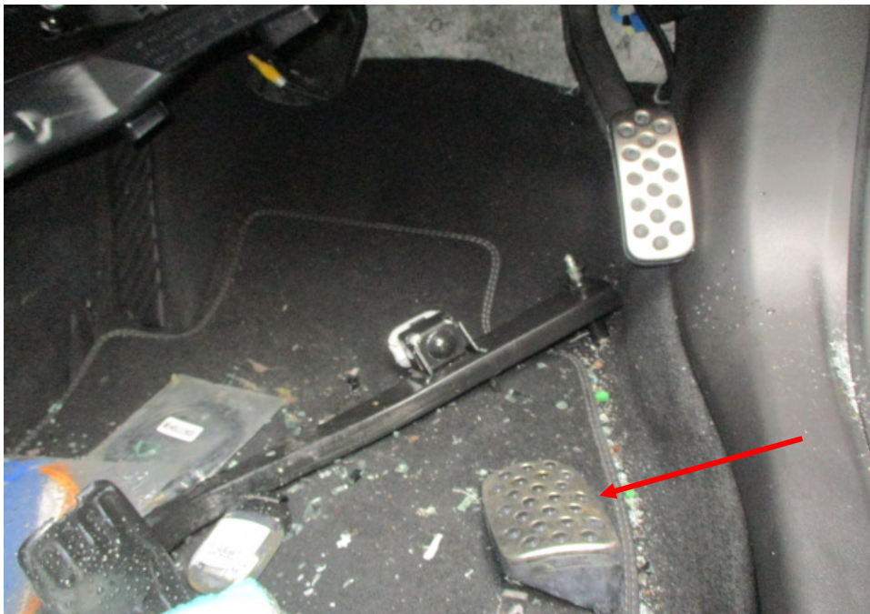
Photo 15 shows the foot brake pedal (arrowed) of the Insured Vehicle. The foot brake pedal was dislodged, which prevented me from carrying any meaningful test to the braking system of the Insured Vehicle.
