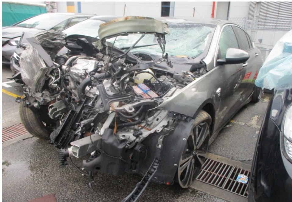
Photo 4 shows a general view of the front left body of the Insured Vehicle at the time of my inspection. The Insured Vehicle was observed to have sustained extensive collision damage at its frontal portion. Almost all the parts and components within the engine compartment were seen to be damaged/affected.
