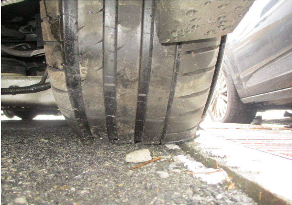
Photo 12 shows the condition of the Insured Vehicle's rear right tyre. The rear right tyre of the Insured Vehicle was found to be in serviceable condition given that the tread pattern was clearly visible.
