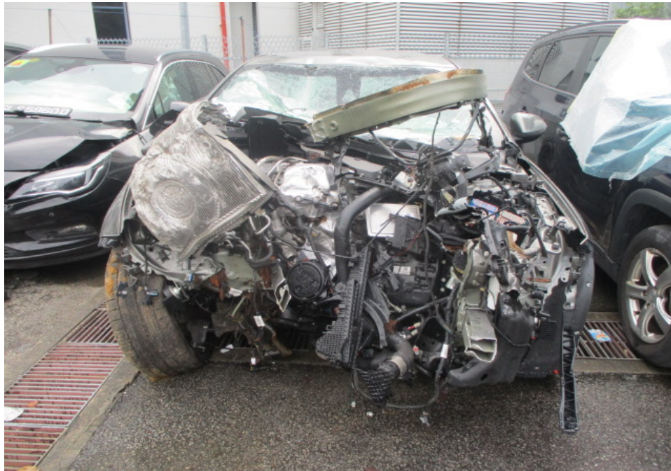
Photo 2 shows a general view of the frontal body of the Insured Vehicle at the time of my inspection. The Insured Vehicle was observed to have sustained extensive collision damage at its frontal portion. Almost all the parts and components within the engine compartment were seen to be damaged/affected.
