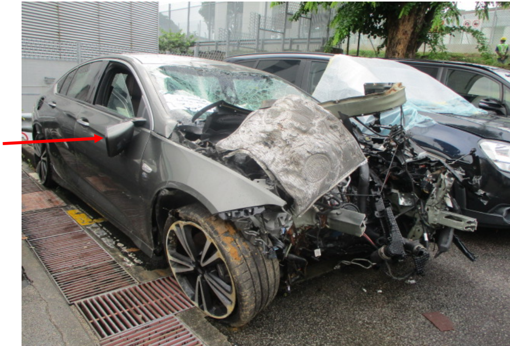
Photo 1 shows a general view of the front right body of the Insured Vehicle at the time of my inspection. The Insured Vehicle was observed to have sustained extensive collision damage at its frontal portion. Almost all the parts and components within the engine compartment were seen to be damaged/affected. Its right side wing mirror (arrowed) was also observed to be damaged.
