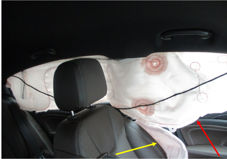
Photo 17 shows the interior compartment of the Insured Vehicle at the time of my inspection. The left curtain airbag (red arrow) and front left passenger seat airbag (yellow arrow) were activated.
