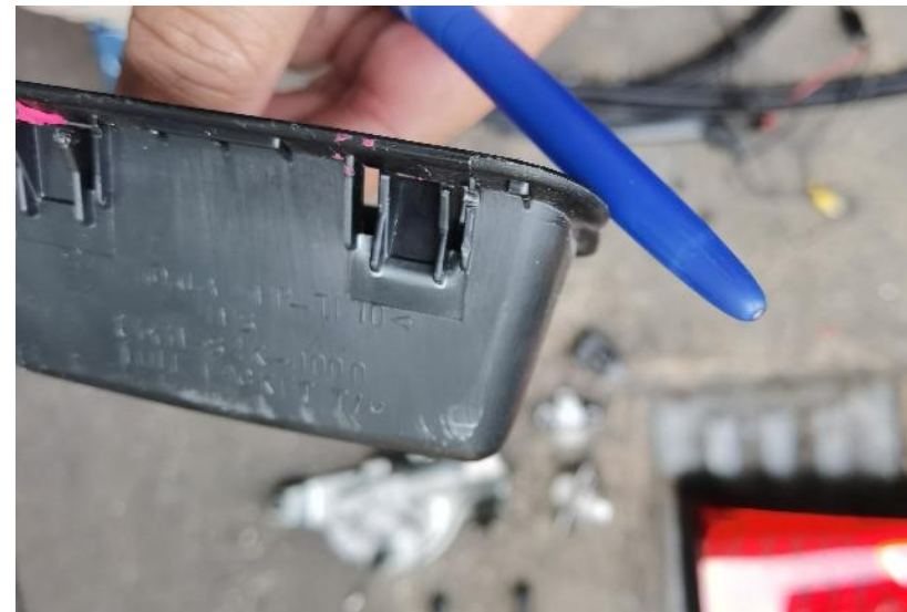
16/44: Tailgate Handle Grib - Cracked
