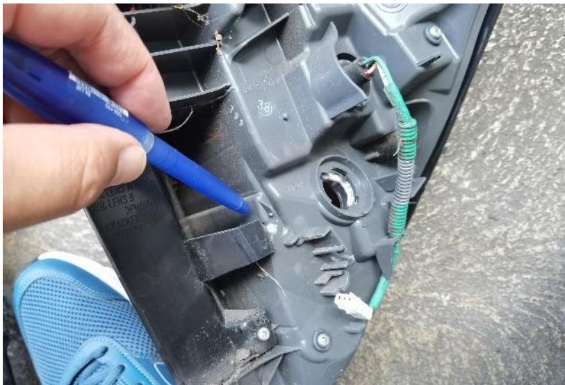
31/44: Taillamp LH - Studs Cracked
