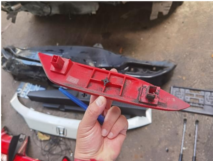
27/44: Rear Bumper Reflector RH - Stud Cracked
