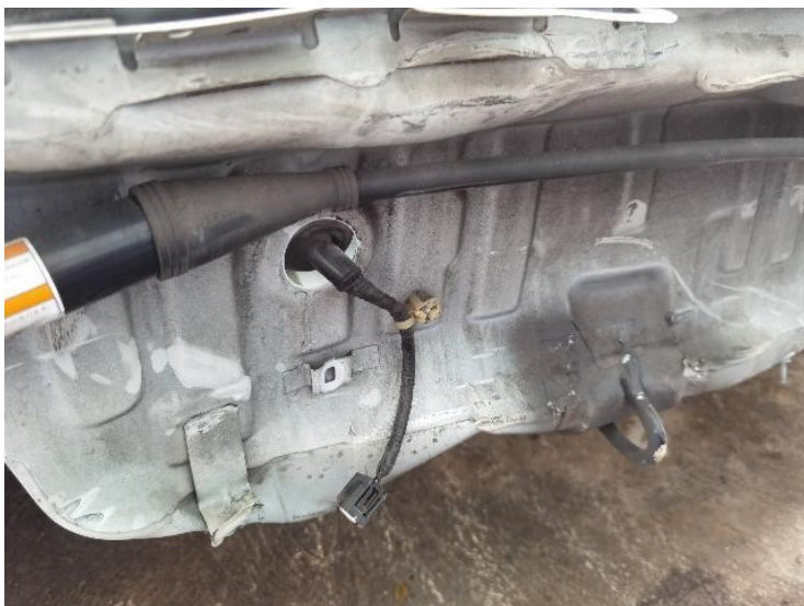
39/44: Rear End Panel - Dented/Deformed
