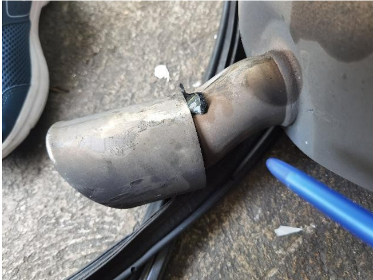
9/44: Rear Exhaust Assembly - Bent
