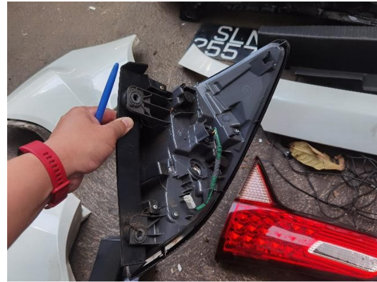
30/44: Taillamp LH - Studs Cracked
