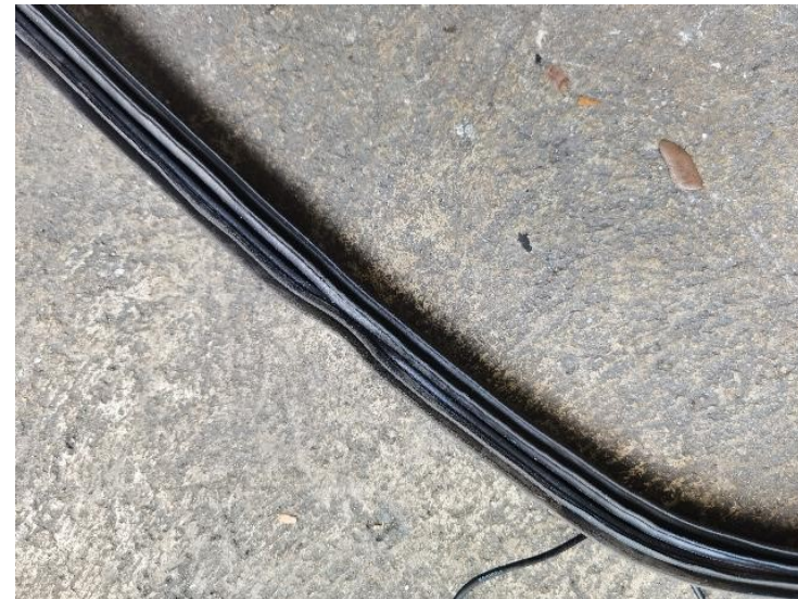
12/44: Tailgate Weather Moulding - Deformed
