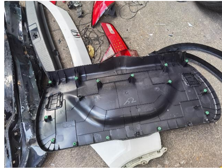
6/44: Tailgate Inner Trim - Studs Cracked
