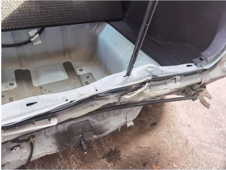
41/44: Rear End Panel - Dented/Deformed
