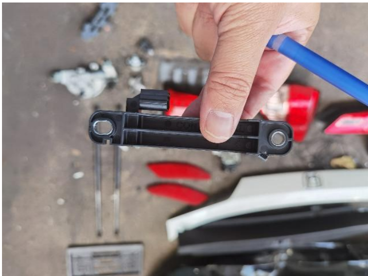
19/44: Tailgate Sensor - Cracked
