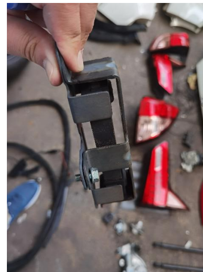
22/44: Tailgate Sensor Bracket - Cracked
