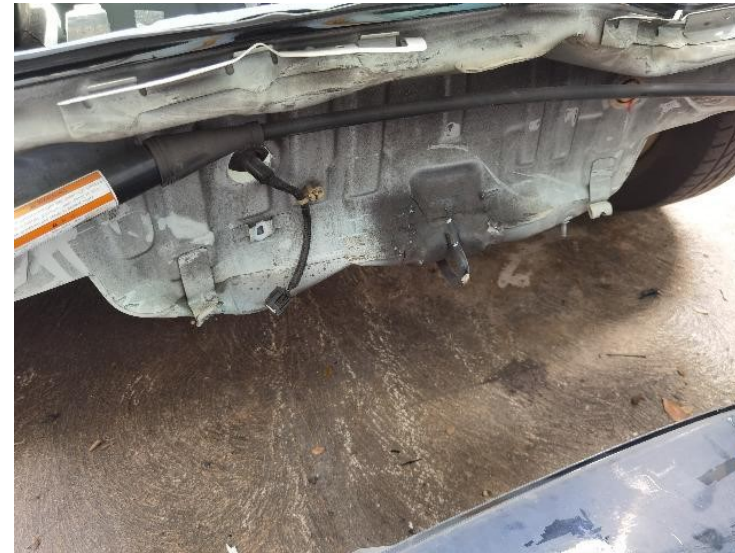
38/44: Rear End Panel - Dented/Deformed
