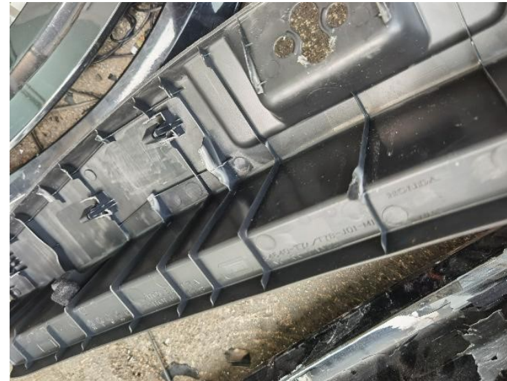
18/44: Rear End Panel Garnish - Dented/Deformed
