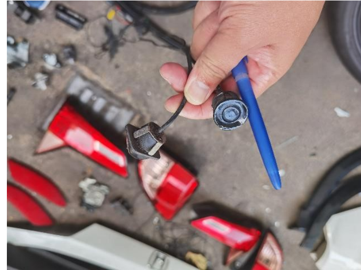
14/44: Reverse Sensoer - Cracked
