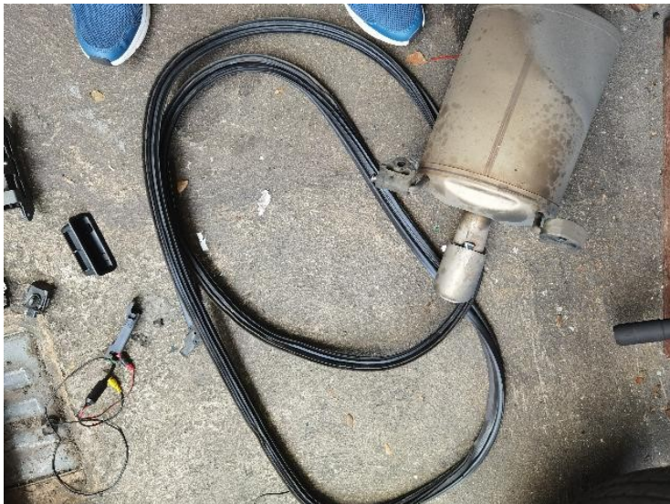
11/44: Tailgate Weather Moulding - Deformed
