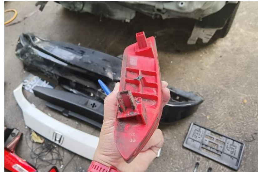
28/44: Rear Bumper Reflector RH - Stud Cracked
