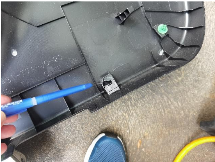
7/44: Tailgate Inner Trim - Studs Cracked
