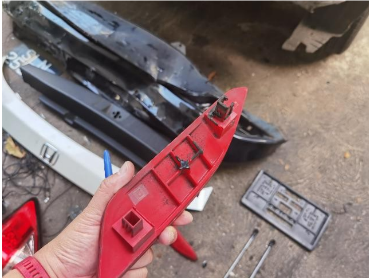
25/44: Rear Bumper Reflector LH - Stud Cracked
