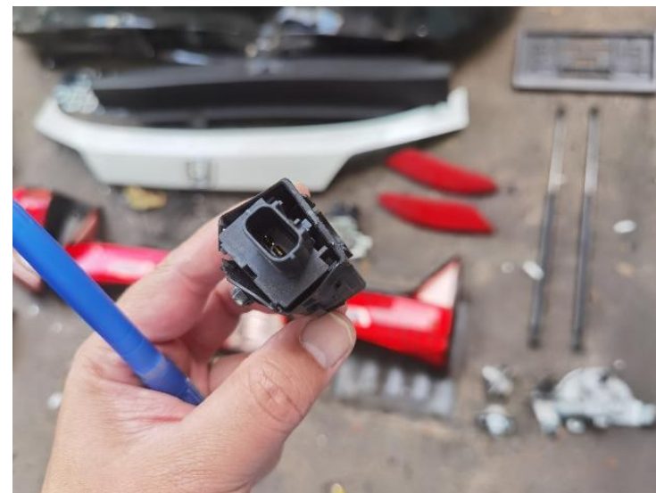
24/44: Tailgate Sensor - Electrical Plug Cracked
