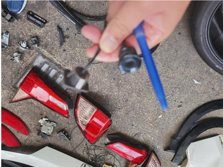
13/44: Reverse Sensoer - Cracked
