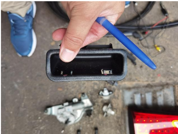
15/44: Tailgate Handle Grib - Cracked
