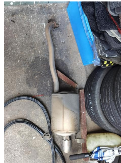
8/44: Rear Exhaust Assembly - Bent
