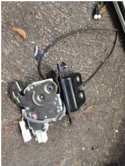
35/44: Tailgate Lock Assembly - Jammed
