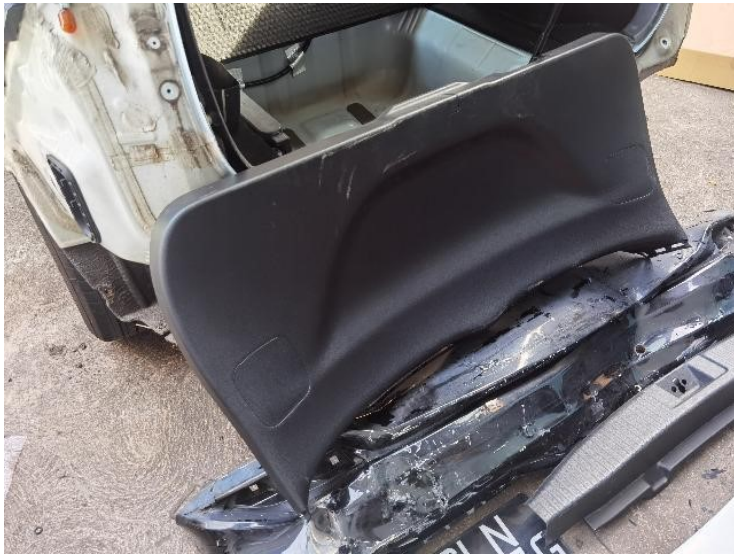
5/44: Tailgate Inner Trim - Studs Cracked
