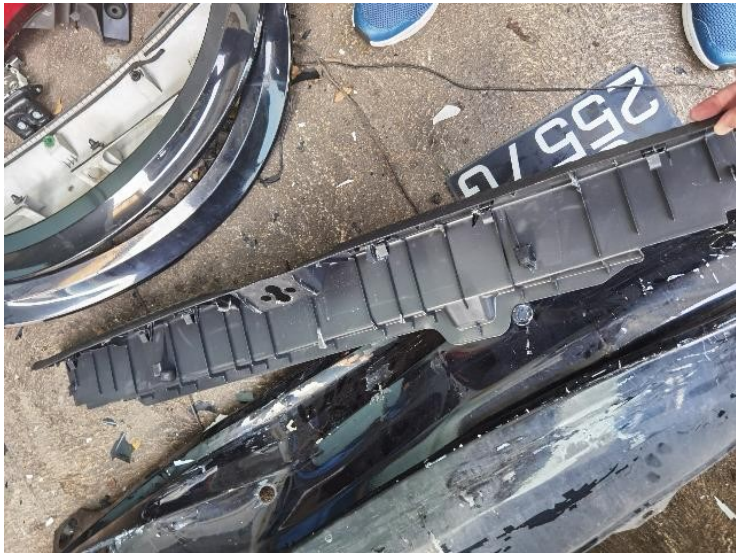
17/44: Rear End Panel Garnish - Dented/Deformed
