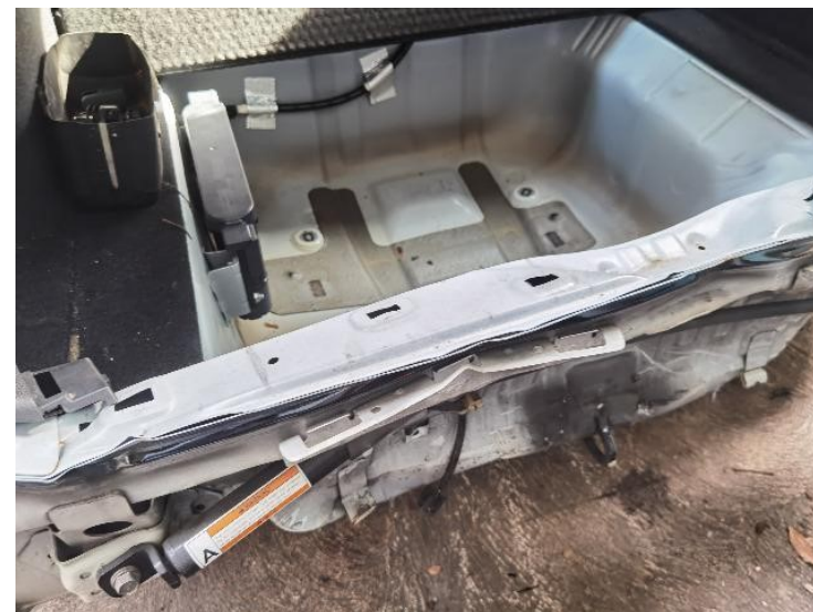
40/44: Rear End Panel - Dented/Deformed
