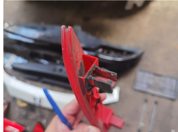
26/44: Rear Bumper Reflector LH - Stud Cracked
