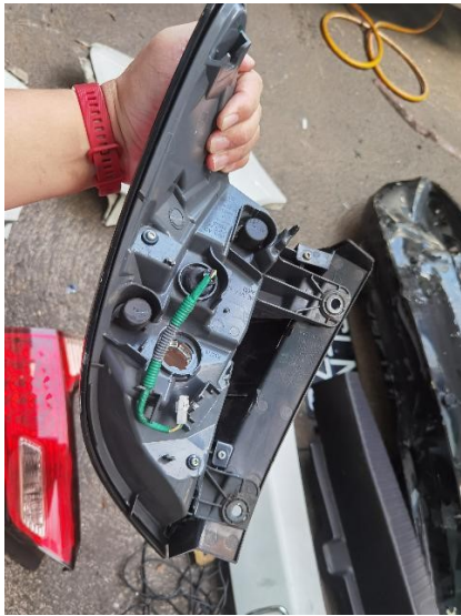
33/44: Taillamp RH - Studs Cracked
