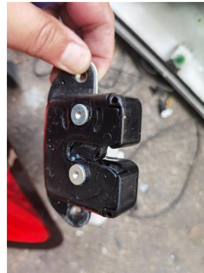
36/44: Tailgate Lock Assembly - Jammed
