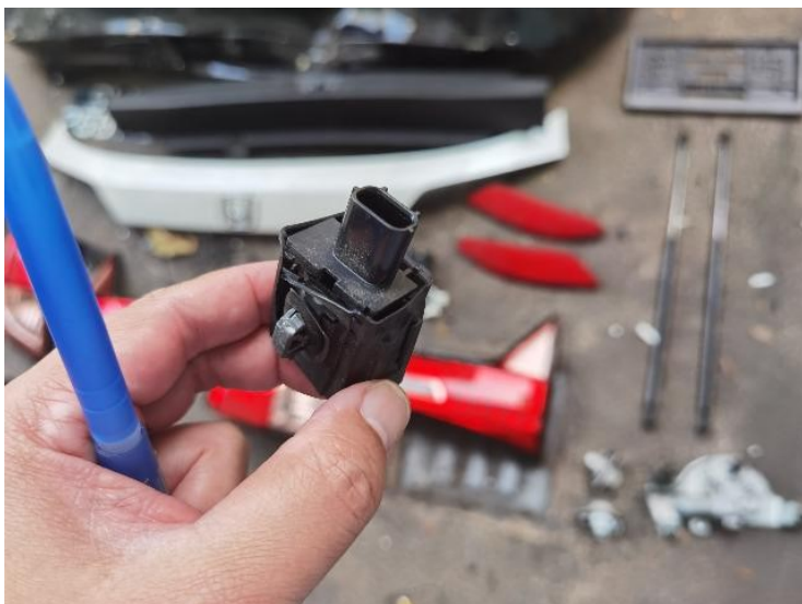
23/44: Tailgate Sensor - Electrical Plug Cracked
