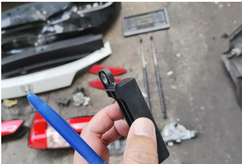
21/44: Tailgate Sensor - Cracked
