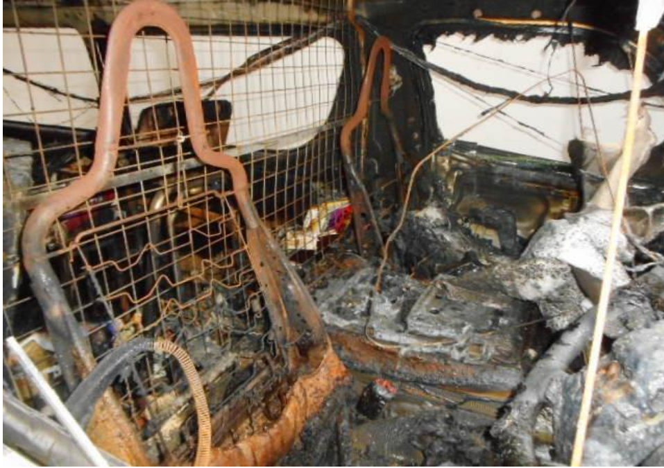
Photo 15 shows the close up view of the interior compartment of the Insured Vehicle at the time of our inspection. Its interior compartment had suffered heat, smoke damage and melted as a result of the fire.
