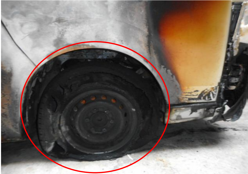
Photo 11 shows the fire damage at the front right wheel portion of the right side of the Insured Vehicle. The tyre and wheel rim had sustained fire damages to it. high heat intensity burn marks (whitish burn marks) found on the exterior surface of its right side as well as rust that had also developed on (circled) this indicates that the fire to the Insured Vehicle had originated from the exterior of the Insured Vehicle.
