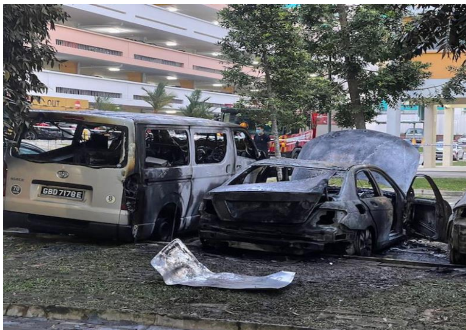
Photo 25 shows the exterior of the Insured Vehicle after the fire was put out. The high heat intensity burn marks (whitish burn marks) and rust that had development found on the right side exterior surface of the Insured Vehicle which was caused by the vehicle that was parked on the right side which had called fire. In general, the information that could be gathered from this photograph had corresponded to the events that were related to us by Mr Foong, location when the fire broke out.
