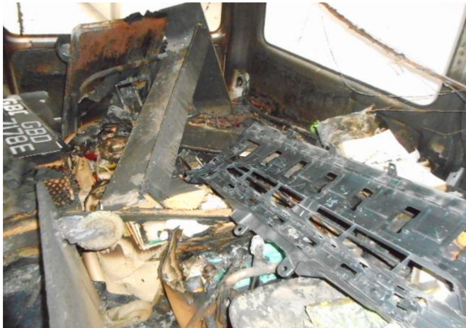
Photo 17 shows the close up view of the interior compartment of the Insured Vehicle at the time of our inspection. Its goods and materials in the Insured Vehicle were all damaged as a result of the fire.
