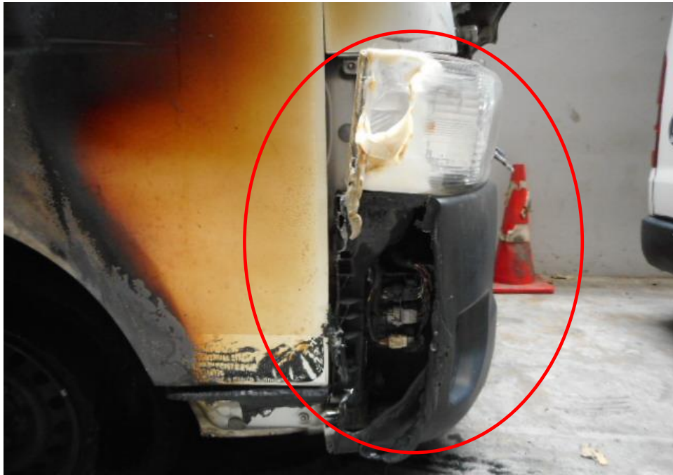
Photo 9 shows the fire damage at the front right headlamp and bumper portion of the Insured Vehicle. The front right headlamp and bumper had melted as a result of the fire as well as the high heat intensity burn marks (whitish burn marks) found on the exterior surface of its right side body panel as well as rust that had also developed on (circled) this indicates that the fire to the Insured Vehicle had originated from the exterior of the Insured Vehicle.
