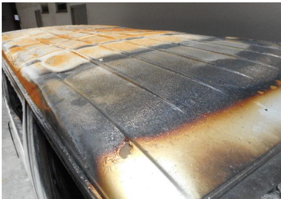
Photo 2 shows the top view of the Insured Vehicle at the time of our inspection. The roof top of the Insured Vehicle had sustained heat and smoke damage by as a result of the fire.
