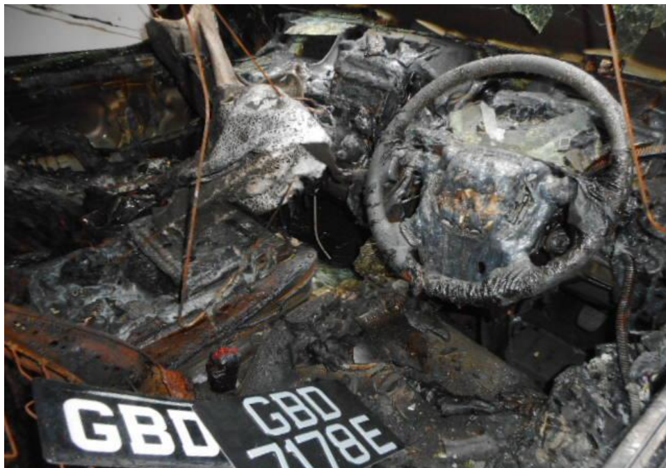
Photo 6 shows the general view of the interior compartment of the Insured Vehicle at the time of our inspection. Its interior compartment had suffered heat, smoke damage and melted as a result of the fire.
