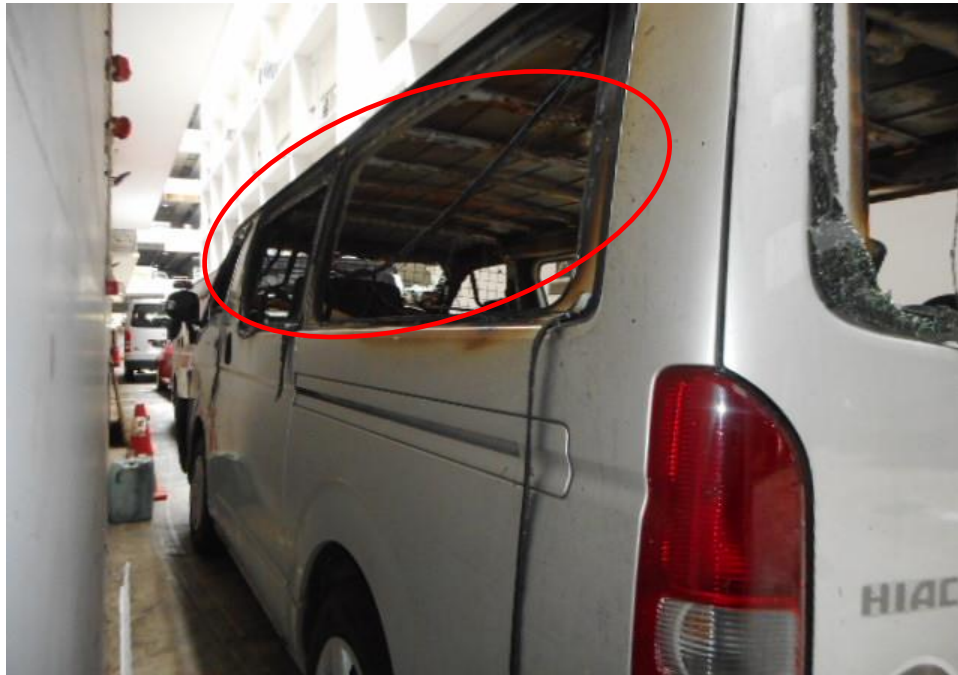
Photo 5 shows the up view of the right side of the Insured Vehicle at the time of our inspection. Only the rear windscreen (circled) of the Insured Vehicle was damaged as a result of the fire. However, the rear body portion of the Insured Vehicle was relatively unaffected by the fire.
