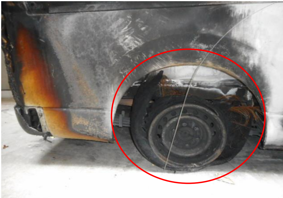
Photo 12 shows the fire damage at the rear right wheel portion of the right side of the Insured Vehicle. The tyre and wheel rim had sustained fire damages to it. high heat intensity burn marks (whitish burn marks) found on the exterior surface of its right side as well as rust that had also developed on (circled) this indicates that the fire to the Insured Vehicle had originated from the exterior of the Insured Vehicle.
