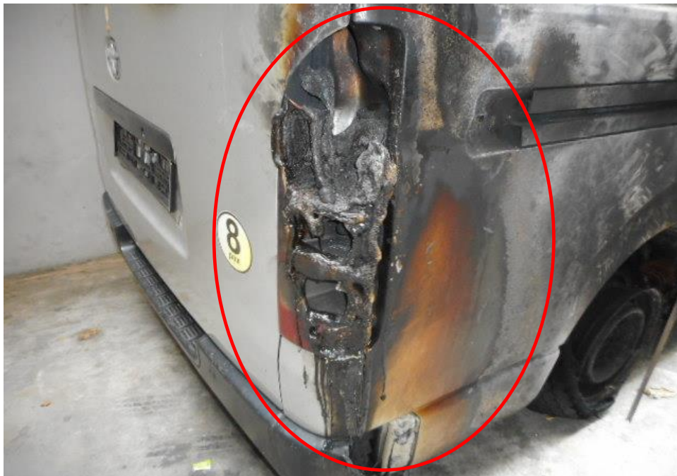
Photo 13 shows the fire damage at the rear right headlamp and bumper portion of the Insured Vehicle. The rear right headlamp and bumper had melted as a result of the fire as well as the high heat intensity burn marks (whitish burn marks) found on the exterior surface of its right side body panel as well as rust that had also developed on (circled) this indicates that the fire to the Insured Vehicle had originated from the exterior of the Insured Vehicle.
