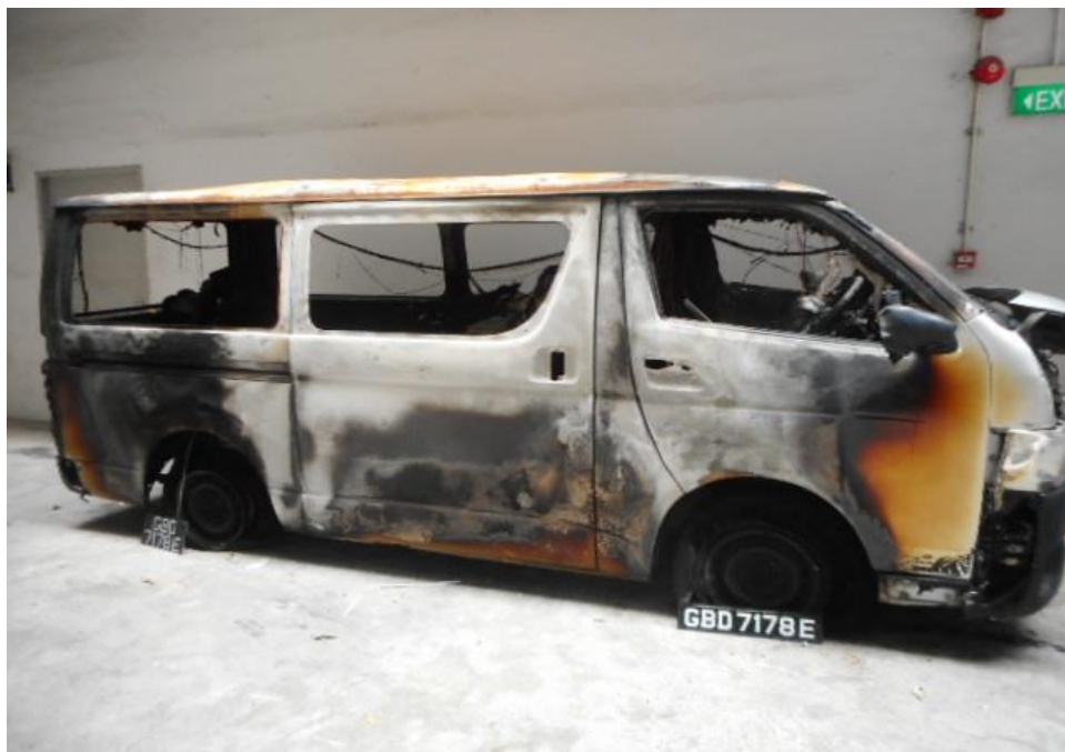
Photo 1 shows the right view of the Insured Vehicle at the time of our inspection. The right body panel of the Insured Vehicle had sustained heat and smoke damage by as a result of the fire.
