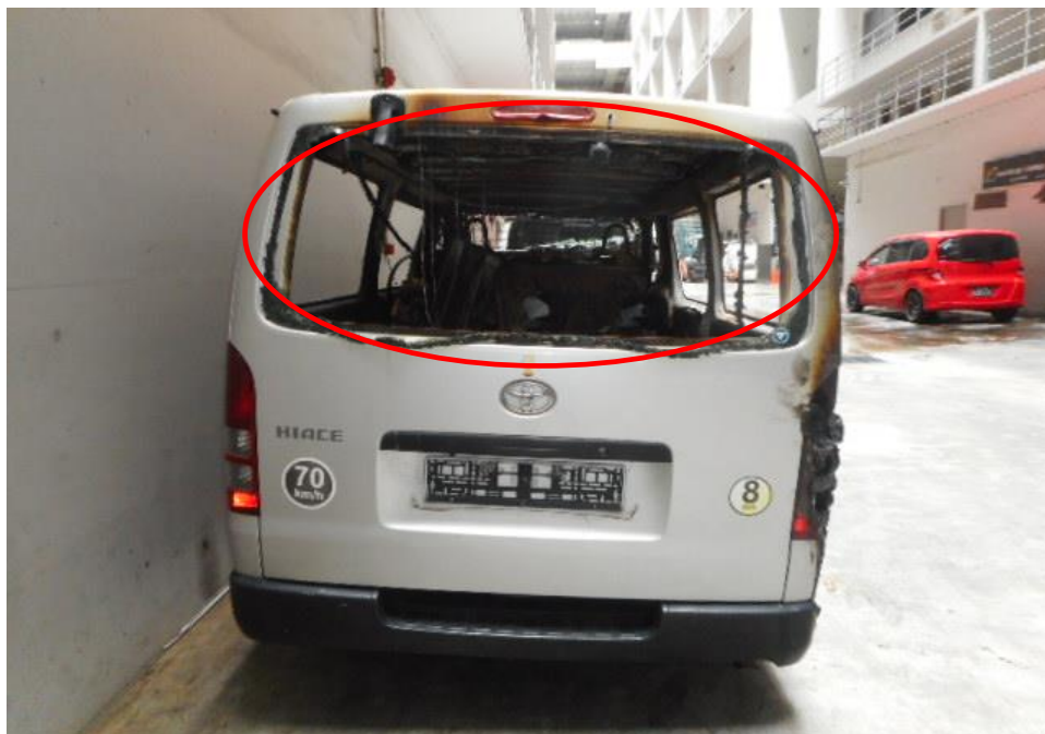
Photo 4 shows the rear view of the Insured Vehicle at the time of our inspection. Only the rear windscreen (circled) of the Insured Vehicle was damaged as a result of the fire. However, the rear body portion of the Insured Vehicle was relatively unaffected by the fire.
