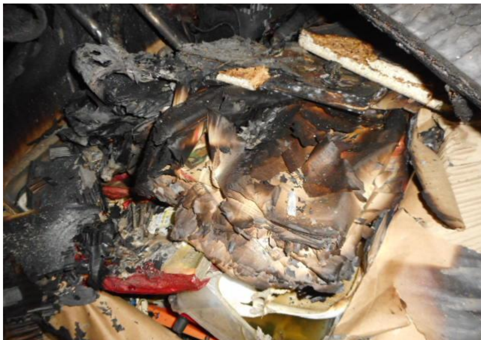
Photo 18 shows the close up view of the interior compartment of the Insured Vehicle at the time of our inspection. The Insured Vehicle was carrying combustible materials and that had resulted in the spread of the fire in the Insured Vehicle at the material time of incident.
