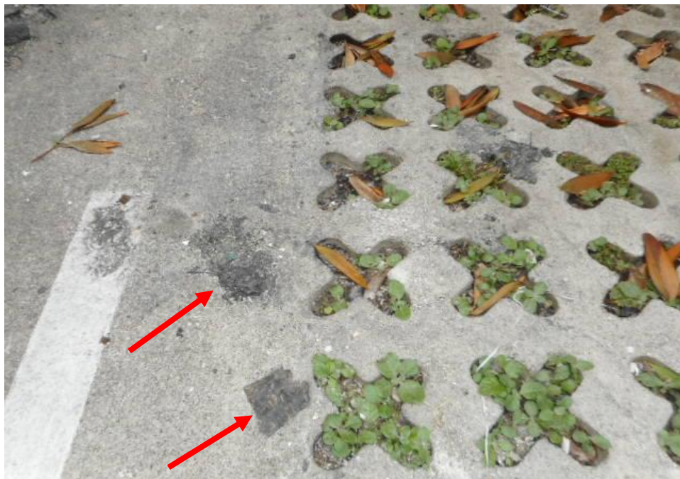
Photo 30 shows the general view of the carpark lot number 349 and 350 where the fire incident had occurred. The Insured Vehicle was parked at carpark lot 350 beside the vehicle that was on fire at carpark lot 349. From our observations, we observed two black residue spots on the ground which was from the right front and rear tyres of Insured Vehicle that had melted as a result of the fire. (arrowed)
