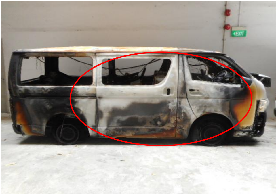
Photo 8 shows the fire damage at the exterior portion of the right side of the Insured Vehicle. The high heat intensity burn marks (whitish burn marks) found on the exterior surface of its right side as well as rust that had also developed on (circled) this indicates that the fire to the Insured Vehicle had originated from the exterior of the Insured Vehicle.
