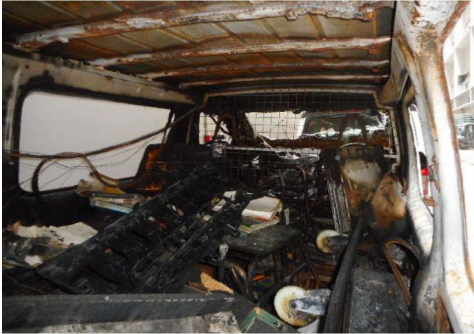
Photo 7 shows the general view of the interior compartment of the Insured Vehicle at the time of our inspection. Its interior compartment had suffered heat, smoke damage and melted as a result of the fire.
