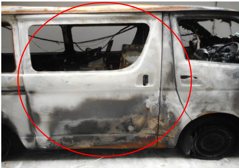
Photo 10 shows close up view of the fire damage at the exterior portion of the right side of the Insured Vehicle. The high heat intensity burn marks (whitish burn marks) found on the exterior surface of its right side as well as rust that had also developed on (circled) this indicates that the fire to the Insured Vehicle had originated from the exterior of the Insured Vehicle.
