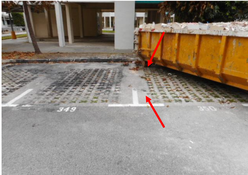
Photo 29 shows the general view of the carpark lot number 349 and 350 where the fire incident had occurred. The Insured Vehicle was parked at carpark lot 350 beside the vehicle that was on fire at carpark lot 349. From our observations, we observed two black residue spots on the ground which was from the right front and rear tyres of Insured Vehicle that had melted as a result of the fire. (arrowed)
