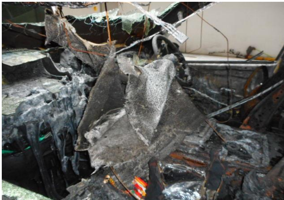
Photo 14 shows the general view of the interior compartment of the Insured Vehicle at the time of our inspection. Its interior compartment had suffered heat, smoke damage and melted as a result of the fire.
