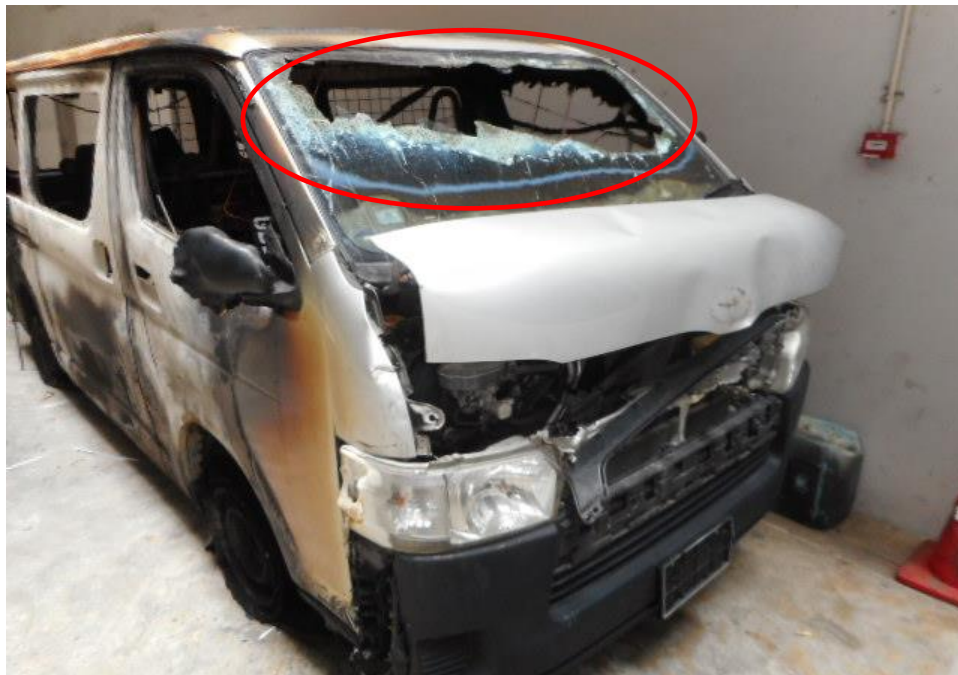
Photo 3 shows the front view of the Insured Vehicle at the time of our inspection. Only the front windscreen (circled) of the Insured Vehicle was damaged as a result of the fire. However, the front body portion of the Insured Vehicle was relatively unaffected by the fire.
