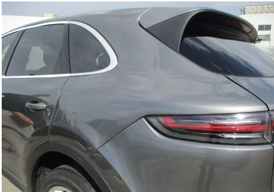
Photo 8 shows a closer view of the Motor Car's rear bootlid spoiler, rear left taillamp, rear left fender, rear left fender wheel arc garnish and rear left quarter glass chrome moulding. The body parts along the left side portion of the Motor Car were visually examined and it was observed that the repair/restoration works carried out to the damaged area of the Motor Car (refer to photograph 1 above) were reasonably adequate and in order.
