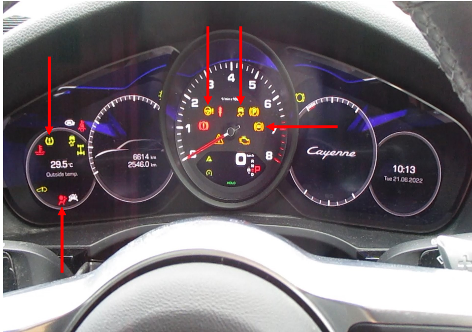
Photo 19 shows the warning lights for the various electronic safety features appearing on the instrument panel of the Motor Car during its self-test when the engine is cranked, in particular the ABS, SRS, EPS, TPM and TCS lights (arrowed).
