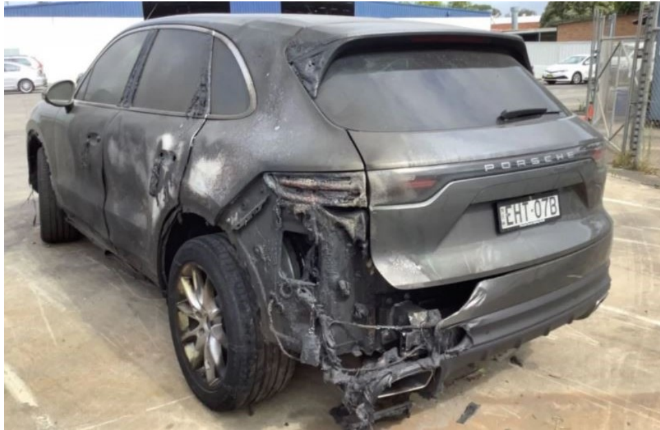
Photo 1 shows the rear left body of the Motor Car (photograph provided to me). The photographs provided to me had showed damage of burnt and/or smoke/heat nature to the exterior body parts along the left side portion of the Motor Car. The rear bumper, rear bumper lower cover, rear bumper left reflector, rear bootlid, rear left bootlid lamp, rear bootlid spoiler, rear left taillamp, rear left fender, rear left door and rear left door outer handle were amongst the exterior body parts that had sustained burnt and/or smoke/heat damage.
