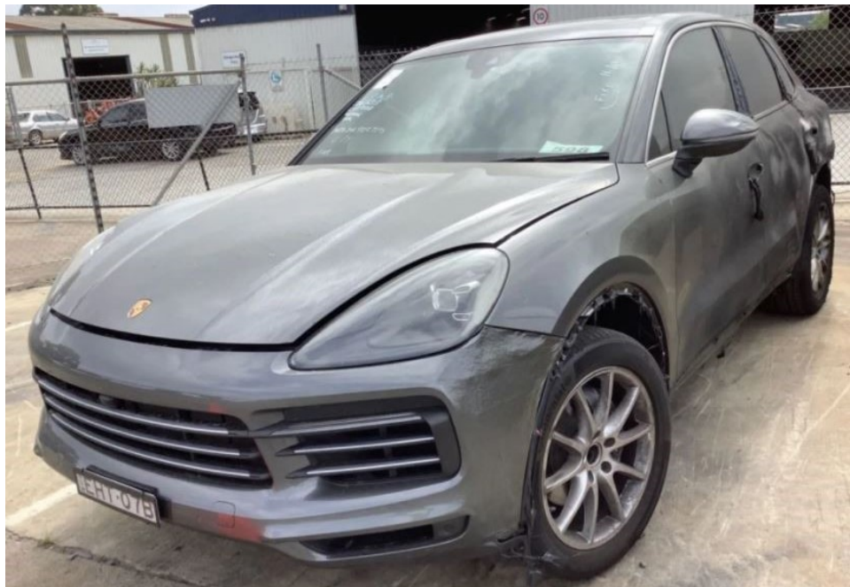
Photo 2 shows the front left body of the Motor Car (photograph provided to me). The photographs provided to me had showed damage of burnt and/or smoke/heat nature to the exterior body parts along the left side portion of the Motor Car. The front bumper, front left fender, front left fender wheel arc garnish, front left door and front left door outer handle were amongst the exterior body parts that had sustained burnt and/or smoke/heat damage.
