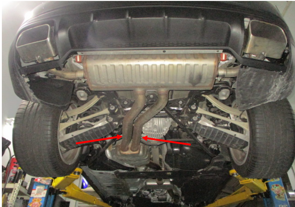
Photo 26 shows the rear section of the Motor Car's exhaust system. My examination of the Motor Car's exhaust system revealed no sign(s) or indication(s) of any cut or weld marks along its exhaust pipes (arrowed), on its rear muffler, on its centre resonator boxes and on its catalytic converter.
