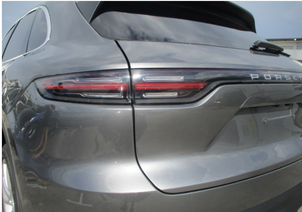
Photo 7 shows a closer view of the Motor Car's rear bumper, rear bootlid, rear left bootlid lamp and rear left taillamp. The body parts along the left side portion of the Motor Car were visually examined and it was observed that the repair/restoration works carried out to the damaged area of the Motor Car (refer to photograph 1 above) were reasonably adequate and in order.
