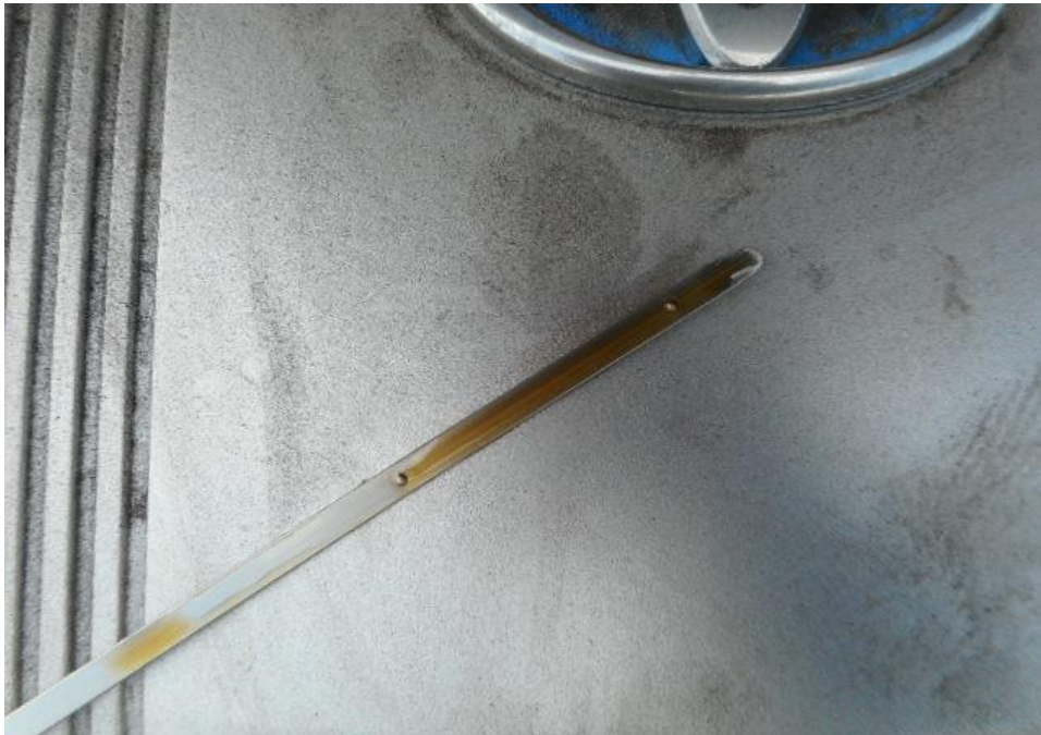
Photo 13 shows the engine oil dip stick of the Motor Taxi at the time of my inspection. The engine oil was observed to be of sufficient level and without any visible contamination.
