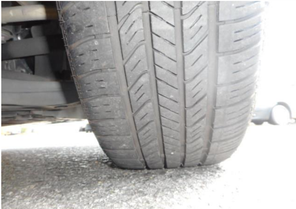
Photo 6 shows the condition of the front right tyre of the Motor Taxi, which was observed to be in serviceable condition with remaining tread depth of approximately 5.5mm. The tyre was sufficiently inflated for vehicular operation with no tear, cut or burst mark(s) on the outer and the inner sidewalls as well as across the tread. The 4 tyres of the Motor Taxi were wrapped around standard steel wheel rims without any damage.
