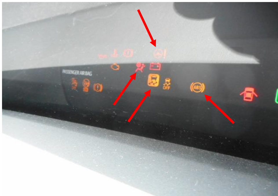
Photo 22 shows the warning light for Anti-Lock Brake System (ABS) and Power Steering System (EPS), Supplemental Restraint System (SRS) and Traction Control (TC) (arrowed) appearing on the instrument panel of the Motor Taxi during the self-test of its various electronic operating systems when its engine was cranked.
