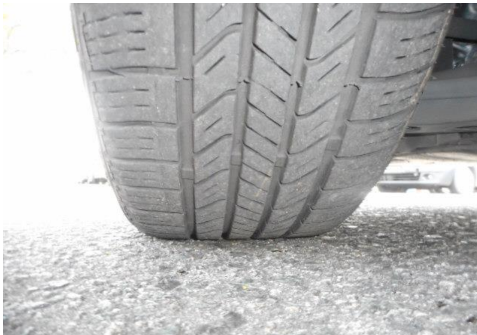
Photo 9 shows the condition of the front left tyre of the Motor Taxi, which was observed to be in serviceable condition with remaining tread depth of approximately 5.2mm. There was also no tear, cut or burst mark(s) on the outer and the inner sidewalls as well as across the tread of the Motor Taxi's 4 tyres.
