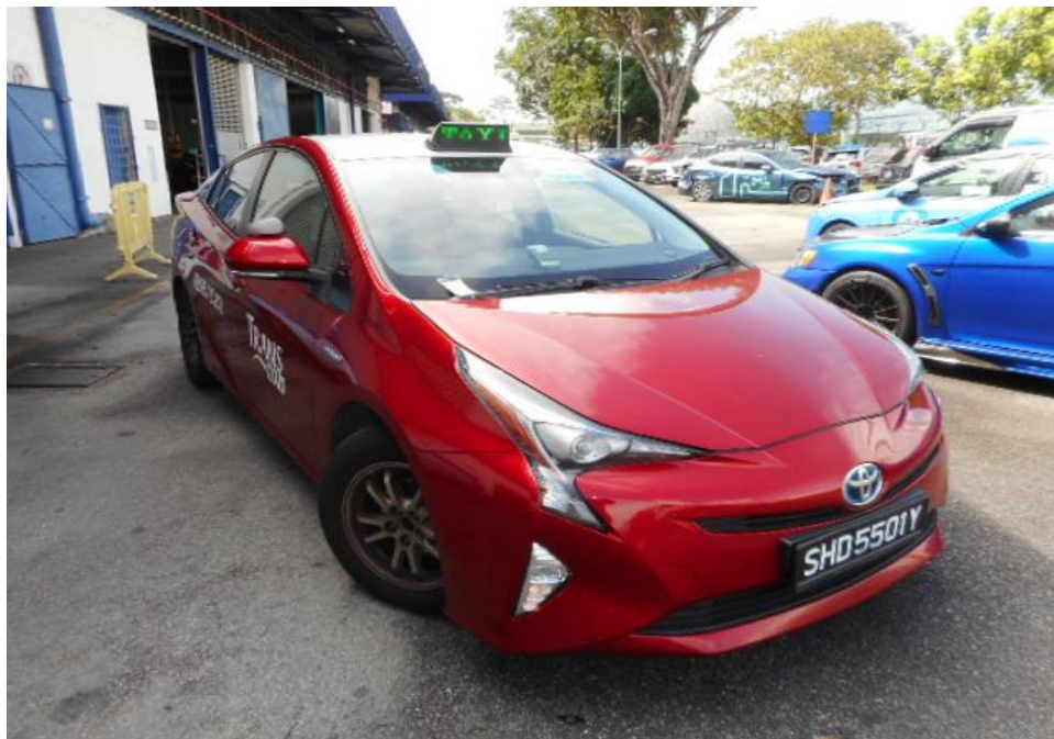
Photo 19 shows the front right wheel of the Motor Taxi turned to its full left. During my steering system test, I did not experience any abnormal free play and/or resistance when I had turned the steering wheel towards the left and right. This would suggest that the steering system of the Motor Taxi was likely to be in serviceable condition at the material time of accident.
