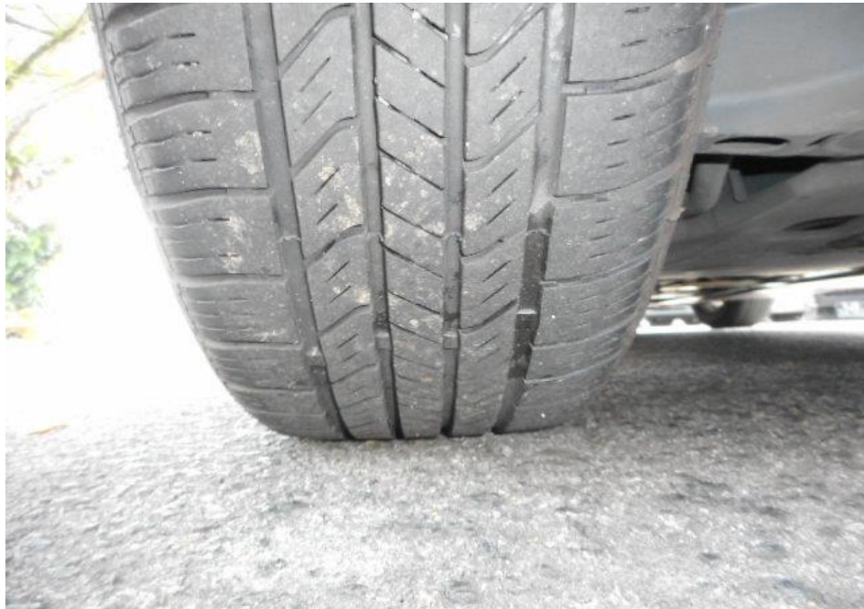
Photo 8 shows the condition of the rear left tyre of the Motor Taxi, which was observed to be in serviceable condition with remaining tread depth of approximately 5.1mm. The tyre, which was wrapped around steel wheel rim, was also observed to be sufficiently inflated for vehicular operation. The 4 tyres of the Motor Taxi were wrapped around standard steel wheel rims.
