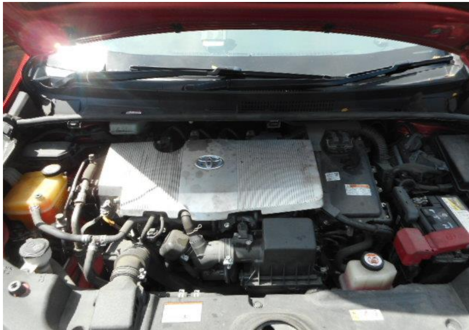
Photo 10 shows a general view of the Motor Taxi's engine compartment. The various parts and components inside the engine compartment were unaffected by the accident. There was also no sign(s) or indication(s) of fluid leakage and/or fluid stain within the engine compartment.
