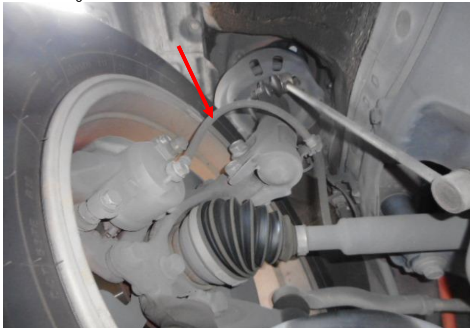
Photo 17 shows the brake hose/pipe (arrowed) at the front right wheel of the Motor Taxi. I did not observe any leakage of brake fluid at the time of my inspection of the Motor Taxi. Static tests of the Motor Taxi's braking system had indicated that there was no internal leakage of pressure/vacuum. The undercarriage components of the Motor Taxi were also all found to be intact and without any visible damage.
