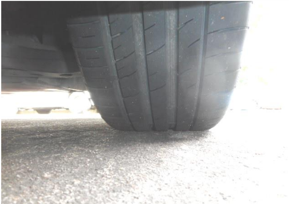
Photo 6 shows the condition of the front right tyre of the Motor Car, which was observed to be in serviceable condition with remaining tread depth of approximately 5.4mm. The tyre was sufficiently inflated for vehicular operation with no tear, cut or burst mark(s) on the outer and the inner sidewalls as well as across the tread. The 4 tyres of the Motor Car were wrapped around standard steel wheel rims without any damage.
