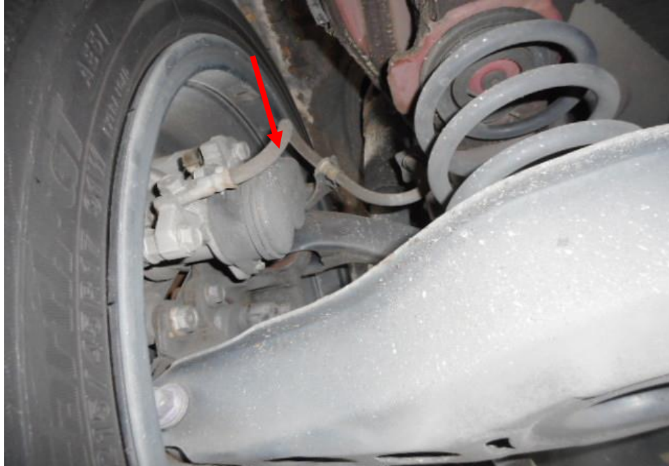
Photo 16 shows the brake hose/pipe (arrowed) at the rear left wheel of the Motor Car. I did not observe any leakage of brake fluid at the time of my inspection of the Motor Car. Static tests of the Motor Car's braking system had indicated that there was no internal leakage of pressure/vacuum. The undercarriage components of the Motor Car were also all found to be intact and without any visible damage.
