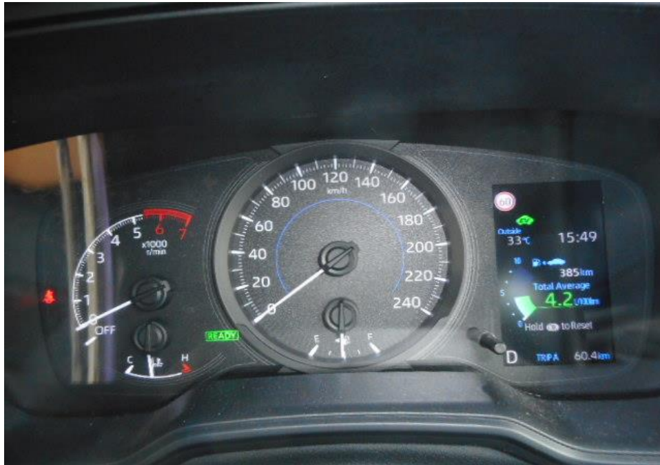
Photo 23 shows no warning lights illuminated on the instrument panel of the Motor Car after the engine was cranked. This would suggest that there was no abnormality to the electronic operating system of the Motor Car, like the ABS, EPS, SRS, and TC etc.
