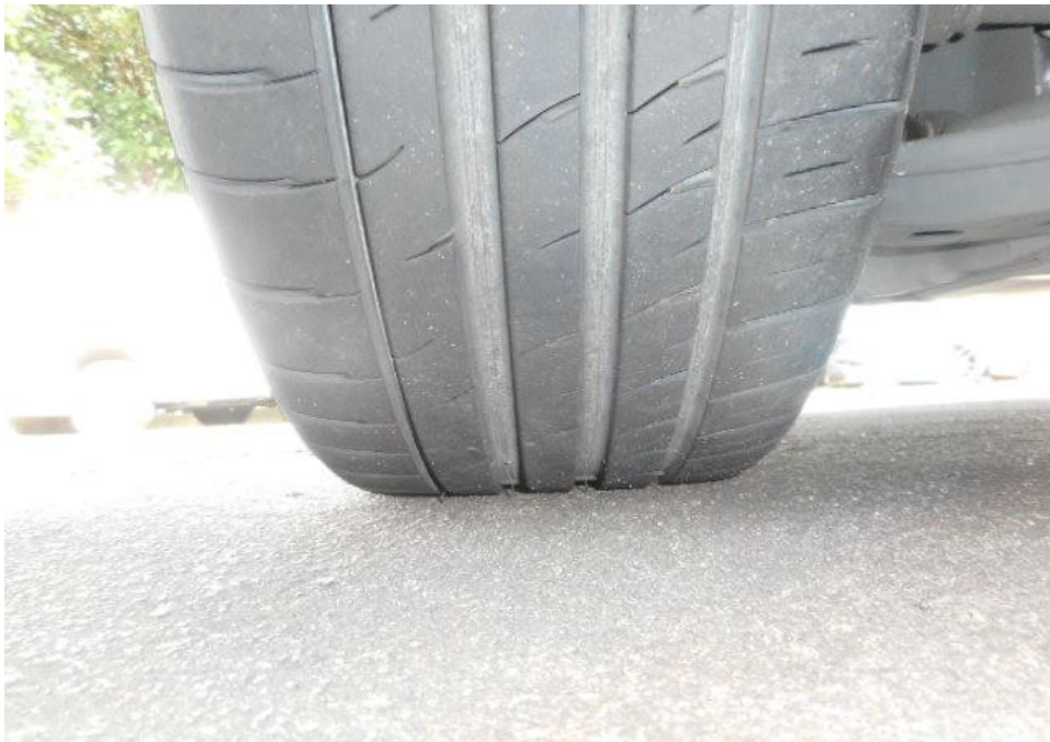
Photo 9 shows the condition of the front left tyre of the Motor Car, which was observed to be in serviceable condition with remaining tread depth of approximately 5.1mm. There was also no tear, cut or burst mark(s) on the outer and the inner sidewalls as well as across the tread of the Motor Car's 4 tyres.
