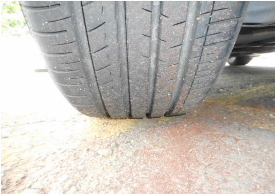
Photo 8 shows the condition of the rear left tyre of the Motor Car, which was observed to be in serviceable condition with remaining tread depth of approximately 6.5mm. The tyre, which was wrapped around steel wheel rim, was also observed to be sufficiently inflated for vehicular operation. The 4 tyres of the Motor Car were wrapped around standard steel wheel rims.
