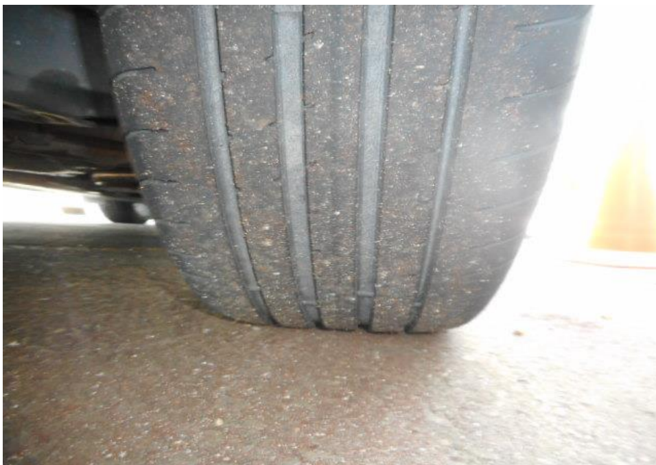
Photo 7 shows the condition of the rear right tyre of the Motor Car, which was observed to be in serviceable condition with remaining tread depth of approximately 5mm. The tyre was also observed to be sufficiently inflated for vehicular operation with no tear, cut or burst mark(s).
