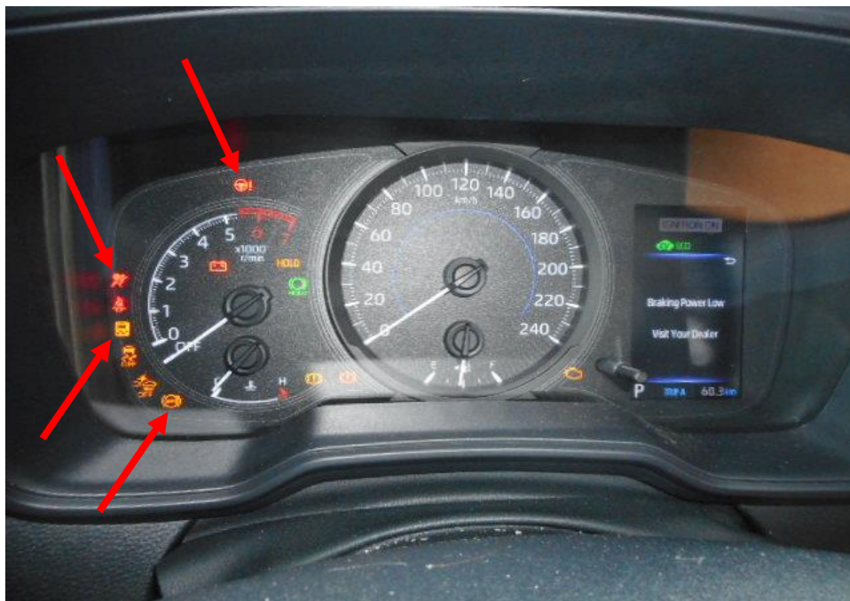
Photo 22 shows the warning light for Anti-Lock Brake System (ABS) and Power Steering System (EPS), Supplemental Restraint System (SRS) and Traction Control (TC) (arrowed) appearing on the instrument panel of the Motor Car during the self-test of its various electronic operating systems when its engine was cranked.
