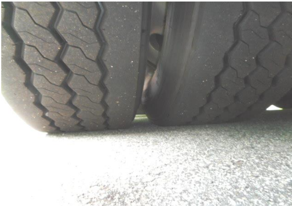
Photo 7 shows the condition of the rear right tyre of the Motor Bus, which was observed to be in serviceable condition with remaining tread depth of approximately 12.7mm. The tyre, which was wrapped around standard steel wheel rim, was also observed to be sufficiently inflated for vehicular operation.
