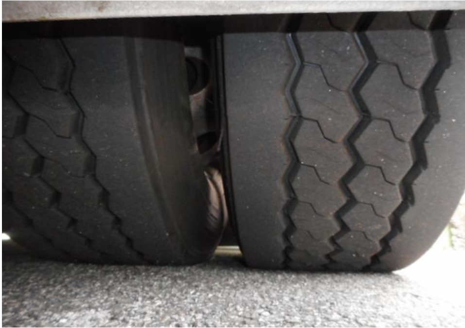
Photo 8 shows the condition of the rear left tyres of the Motor Bus, which was observed to be in serviceable condition with remaining tread depth of approximately 11.9mm. The tyres, which were wrapped around standard steel wheel rim, were also observed to be sufficiently inflated for vehicular operation. There was also no damage found on all 8 steel wheel rims of the Motor Bus.
