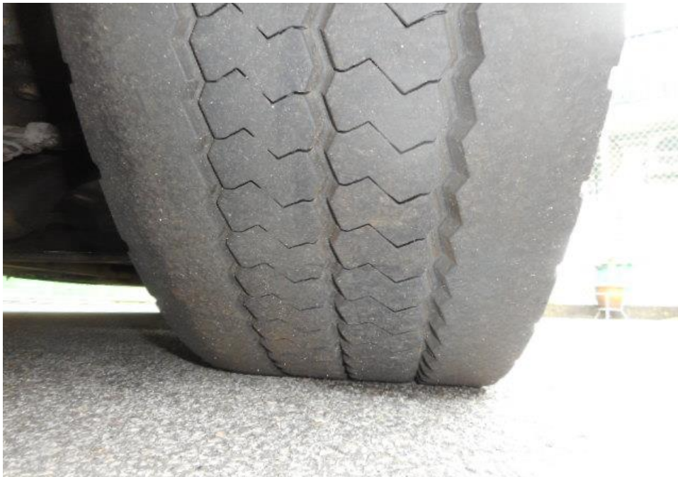
Photo 9 shows the condition of the front left tyres of the Motor Bus, which were observed to be in serviceable condition with remaining tread depth of approximately 8.7mm. There was also no tear, cut or burst mark(s) on the outer and the inner sidewalls as well as across the tread of the 8 tyres that were fitted on the Motor Bus.
