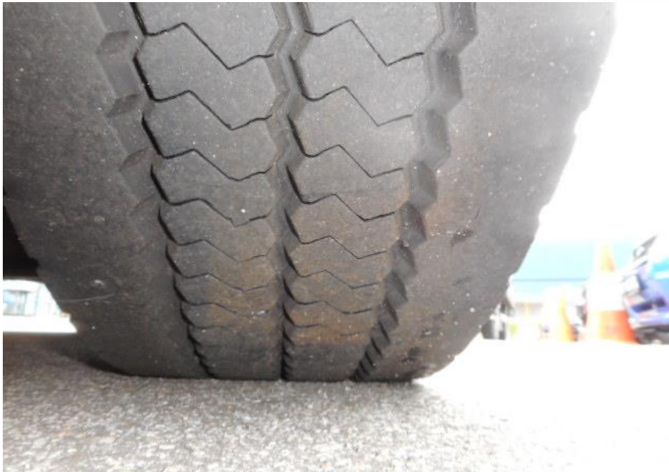
Photo 6 shows the condition of the front right tyre of the Motor Bus, which was observed to be in serviceable condition with remaining tread depth of approximately 11.3mm. The tyre, which was wrapped around standard steel wheel rim, was also observed to be sufficiently inflated for vehicular operation. There was no tear, cut or burst mark(s) on the outer and the inner sidewalls as well as across the tread of the 8 tyres that were fitted on the Motor Bus.
