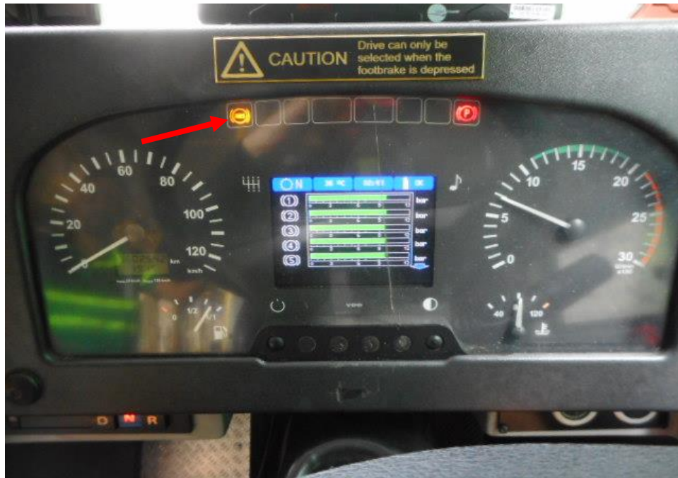
Photo 25 shows the Anti-Lock Braking System (arrowed) warning lights remained illuminated on the instrument panel of the Motor Bus after the engine was cranked, however during our operational test drive the system were in working condition and without abnormality.
