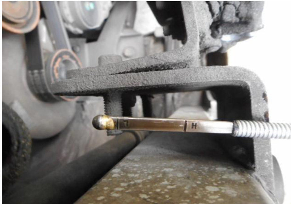
Photo 14 shows the engine oil dip stick system of the Motor Bus at the time of my inspection. The engine oil was observed to be sufficient for operation and without any visible contamination.
