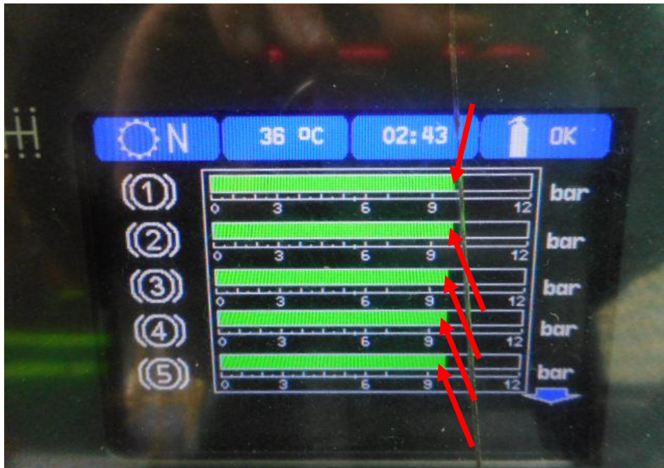
Photo 11 shows the air in the air brake cylinder of the Motor Bus at the time of my inspection. The air in the cylinder was observed to be of sufficient level & serviceable at the time of the accident.
