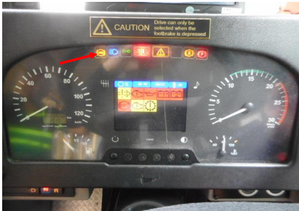
Photo 24 shows the warning light for Anti-Lock Braking System (ABS) appearing on the instrument panel of the Motor Bus during the self-test of its various electronic operating systems when its engine was cranked.
