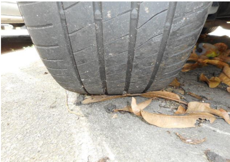
Photo 11 shows the condition of the rear left tyre of the Motor Car, which was observed to be in serviceable condition with remaining tread depth of approximately 4.7mm. The tyre, which was wrapped around steel wheel rim, was also observed to be sufficiently inflated for vehicular operation. The 4 tyres of the Motor Car were wrapped around standard steel wheel rims.
