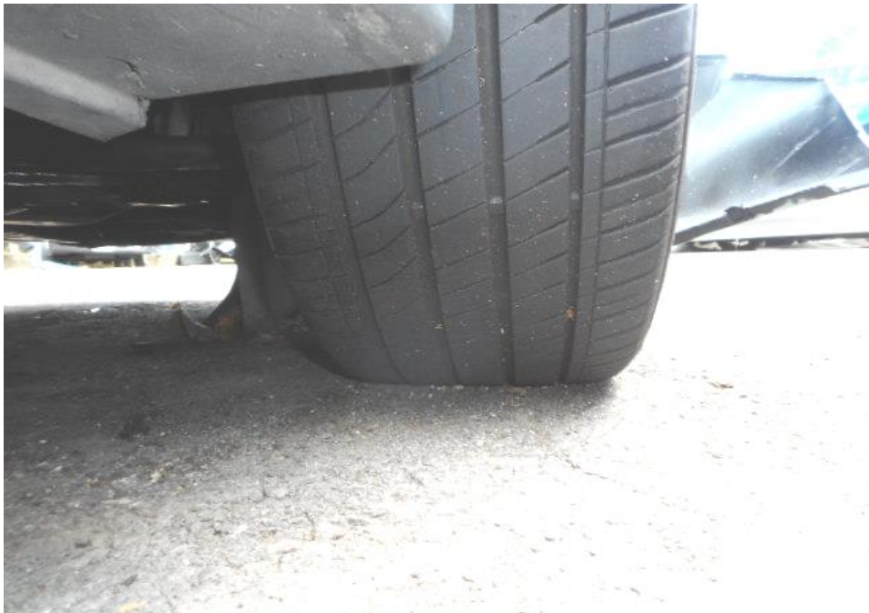
Photo 9 shows the condition of the front right tyre of the Motor Car, which was observed to be in serviceable condition with remaining tread depth of approximately 5.3mm. The tyre was sufficiently inflated for vehicular operation with no tear, cut or burst mark(s) on the outer and the inner sidewalls as well as across the tread. The 4 tyres of the Motor Car were wrapped around standard steel wheel rims without any damage.
