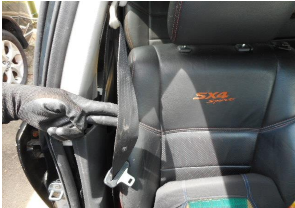
Photo 27 shows that the seat belt on the right seat was not worn at the material time of accident as the safety pre-tensioners was activated at the moment of impact and caused the seat belt to be locked into the last position.
