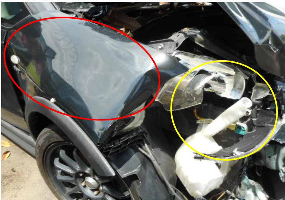
Photo 5 shows a close up view of the Motor Car's front body at the time of my inspection. The Motor Car was observed to have sustained damage at its front portion. Its front right fender (red circle) and front right headlamp (yellow circle) was the body part that were damaged as a result of the accident.
