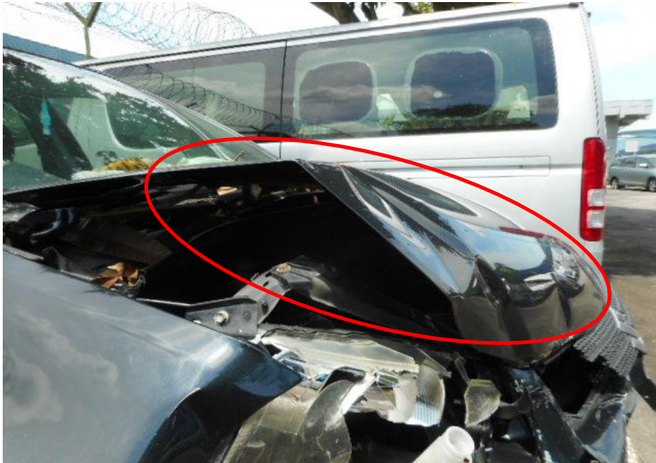
Photo 4 shows a close up view of the Motor Car's front body at the time of my inspection. The Motor Car was observed to have sustained damage at its front portion. Its front bonnet (circled) was the body part that were damaged as a result of the accident.
