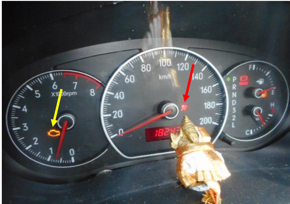
Photo 25 shows the Supplemental Restraint System (SRS) (red arrow) light remained illuminated on due to the deployment of the airbag as a result of the accident after the engine was cranked and we also observed the engine warning light remained illuminated up and this was due to an faulty O2 Sensor (Oxygen Sensor) (yellow arrow) on the engine exhaust piping. However, there was no abnormality to the other electronic operating system of the Motor Car, like the ABS, EPS and TCS etc.
