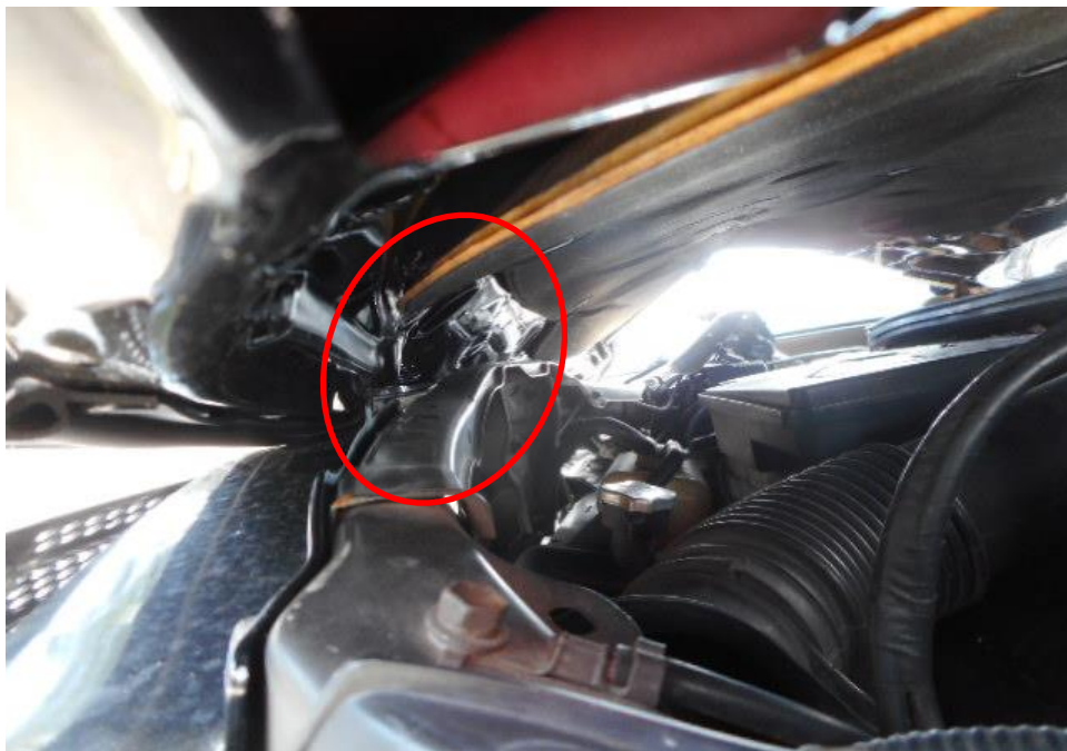
Photo 14 shows a close up view of the damaged front bonnet lock mechanism (circled) and the structure of the engine compartment of the Motor Car at the time of my inspection resulting it unable to open a result of the accident. (Unable to open)
