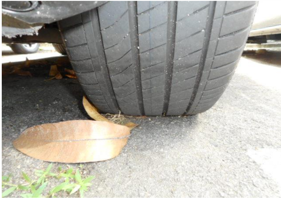
Photo 12 shows the condition of the front left tyre of the Motor Car, which was observed to be in serviceable condition with remaining tread depth of approximately 5.1mm. There was also no tear, cut or burst mark(s) on the outer and the inner sidewalls as well as across the tread of the Motor Car's 4 tyres.
