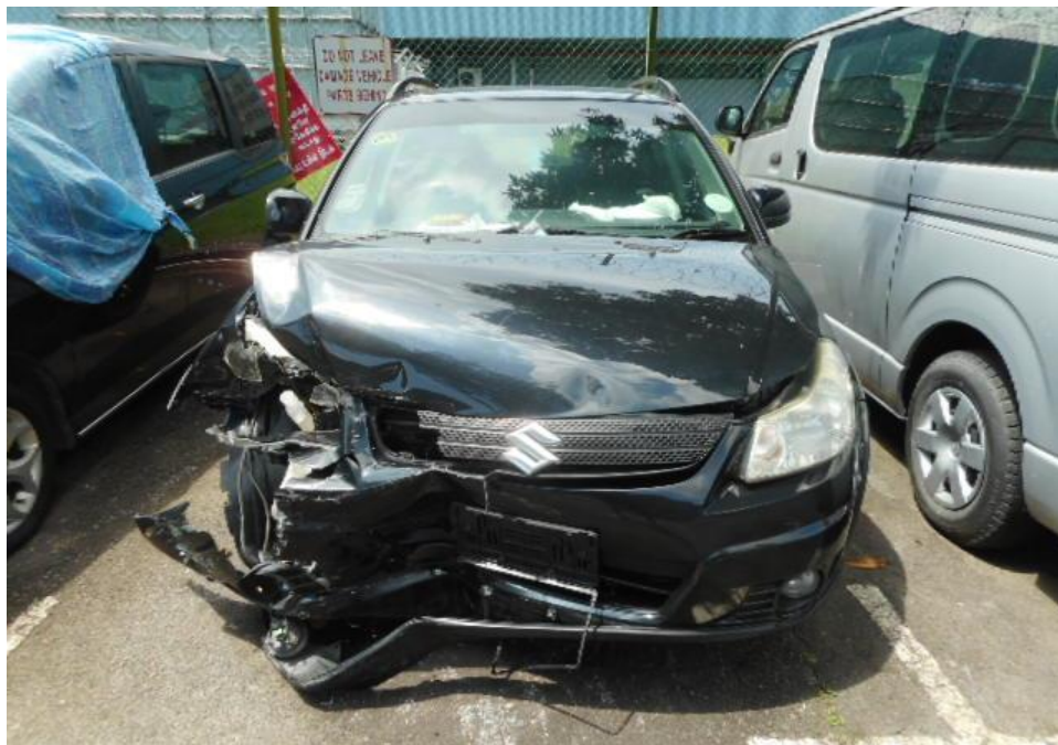
Photo 3 shows a general view of the Motor Car's front body at the time of my inspection. The front portion observed to have sustained damage. Its front bonnet, front right fender, front right headlamp and its front bumper was the body parts as well as its various engine components were also damaged as a result of the accident. The airbag of the Supplemental Restraint System (SRS) was activated as a result of the accident.
