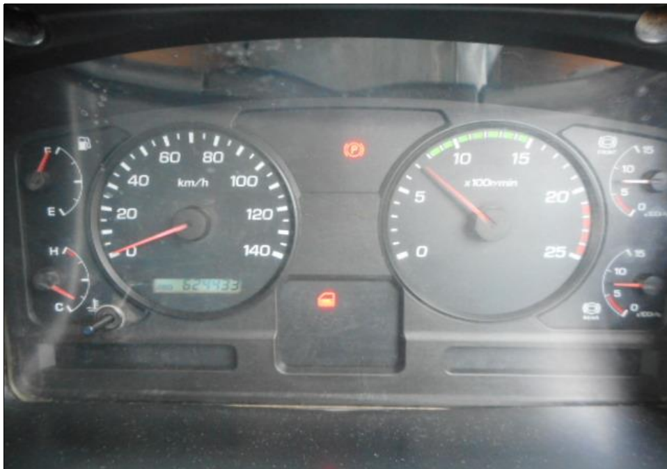
Photo 26 shows the Supplemental Restraint System (SRS) warning lights had went off on the instrument panel of the Prime Mover after the engine was cranked. This would suggest that there was no abnormality to the electronic operating system of the Prime Mover, like the SRS, and etc.
