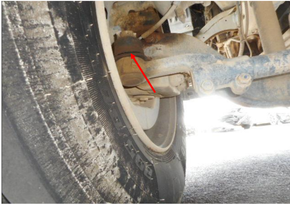
Photo 22 shows the various undercarriage components at the front left wheel of the Prime Mover, in particular the steering tie rod end (arrowed). The various undercarriage components of the Prime Mover were all found to be intact without any visible damage. There was also no sign of fluid stain(s) observed on the various undercarriage components.
