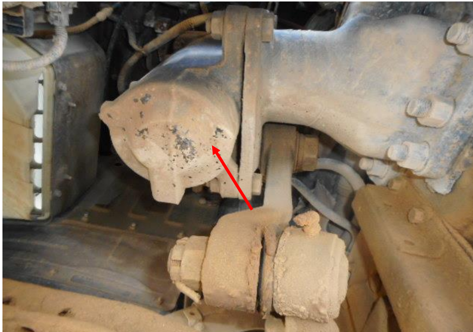
Photo 23 shows the steering box component (arrowed) at the undercarriage of the Prime Mover was found to be intact without any visible damage. There was also no sign of fluid stain(s) observed on the various undercarriage components.
