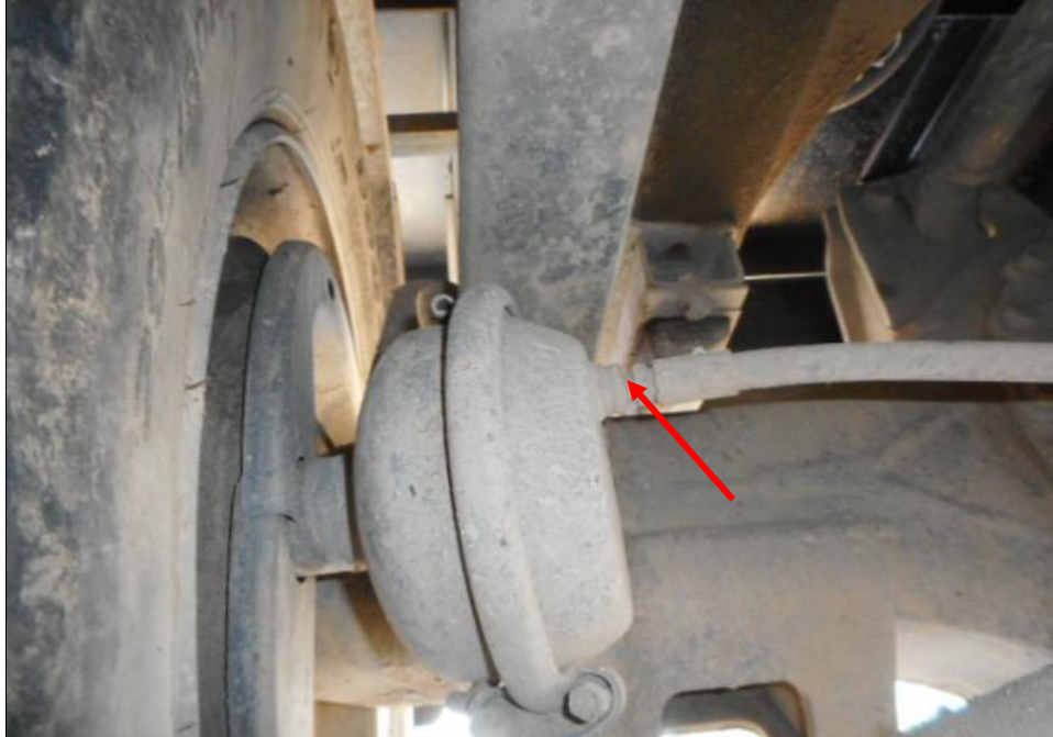
Photo 16 shows the brake pipe (arrowed) at the rear right wheel of the Prime Mover. I did not observe any leakage of brake fluid at the time of my inspection of the Prime Mover. My static tests of the Prime Mover's braking system, along with my visual examination of the various mechanical components in the braking system, had indicated that there was no internal leakage of pressure/vacuum. Hence the braking system of the Prime Mover was likely to be in serviceable condition at the material time of accident.
