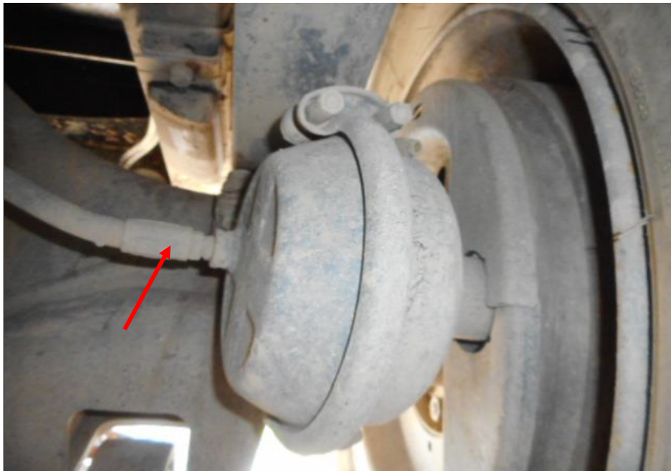
Photo 17 shows the brake pipe (arrowed) at the rear left wheel of the Prime Mover. I did not observe any leakage of brake fluid at the time of my inspection of the Prime Mover. My static tests of the Prime Mover's braking system, along with my visual examination of the various mechanical components in the braking system, had indicated that there was no internal leakage of pressure/vacuum. Hence the braking system of the Prime Mover was likely to be in serviceable condition at the material time of accident.
