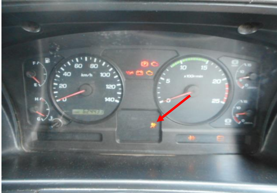
Photo 25 shows the warning light for Supplemental Restraint System (SRS) (arrowed) appearing on the instrument panel of the Prime Mover during the self-test of its various electronic operating systems when its engine was cranked.
