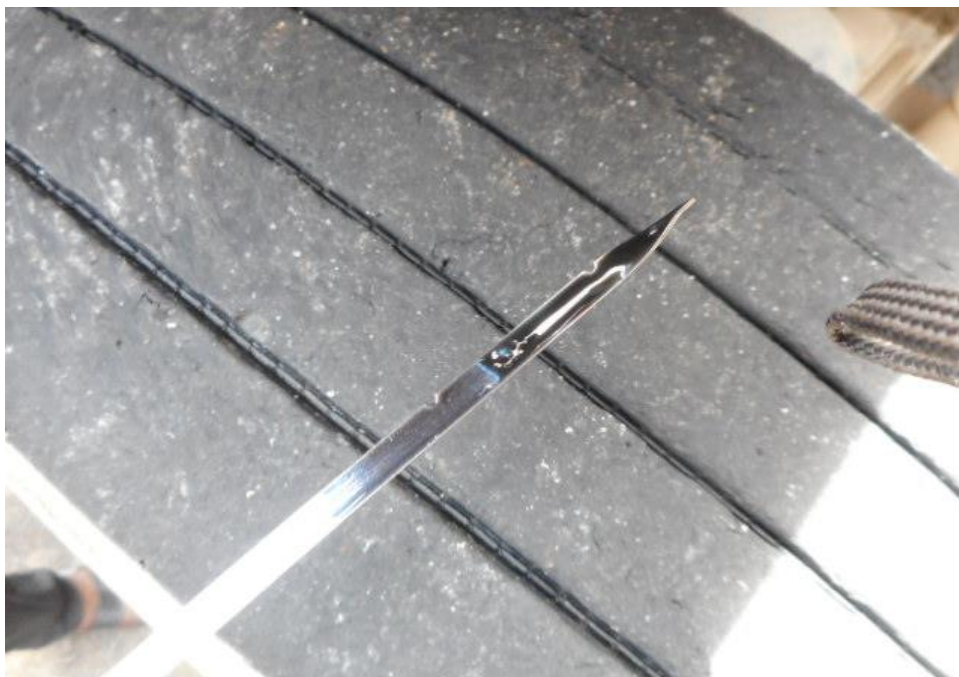
Photo 14 shows the engine oil dip stick of the Prime Mover at the time of my inspection. The engine oil was observed to be of insufficient level at the time of our inspection.
