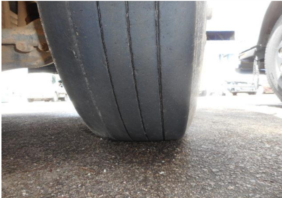
Photo 6 shows the condition of the front right tyre of the Prime Mover, which was observed to be in serviceable condition with remaining tread depth of approximately 5mm. The tyre, which was wrapped around standard steel wheel rim, was also observed to be sufficiently inflated for vehicular operation. There was no tear, cut or burst mark(s) on the outer and the inner sidewalls as well as across the tread of the 6 tyres that were fitted on the Prime Mover.
