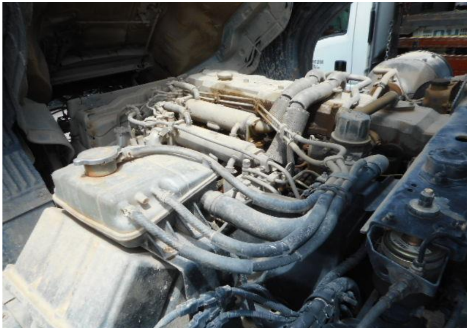
Photo 10 shows a general view of the Prime Mover's engine compartment, which was accessed by lifting the front cabin of the Prime Mover. The various parts and components inside the engine compartment were unaffected by the accident. There was also no sign(s) or indication(s) of fresh fluid leakage and/or fluid stain within the engine compartment
