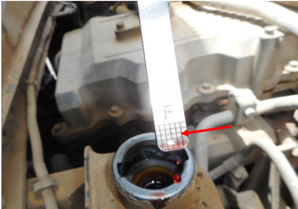
Photo 13 shows the power steering fluid reservoir of the Prime Mover at the time of my inspection. The power steering fluid was observed to be of sufficient level (arrowed) and without any visible contamination.
