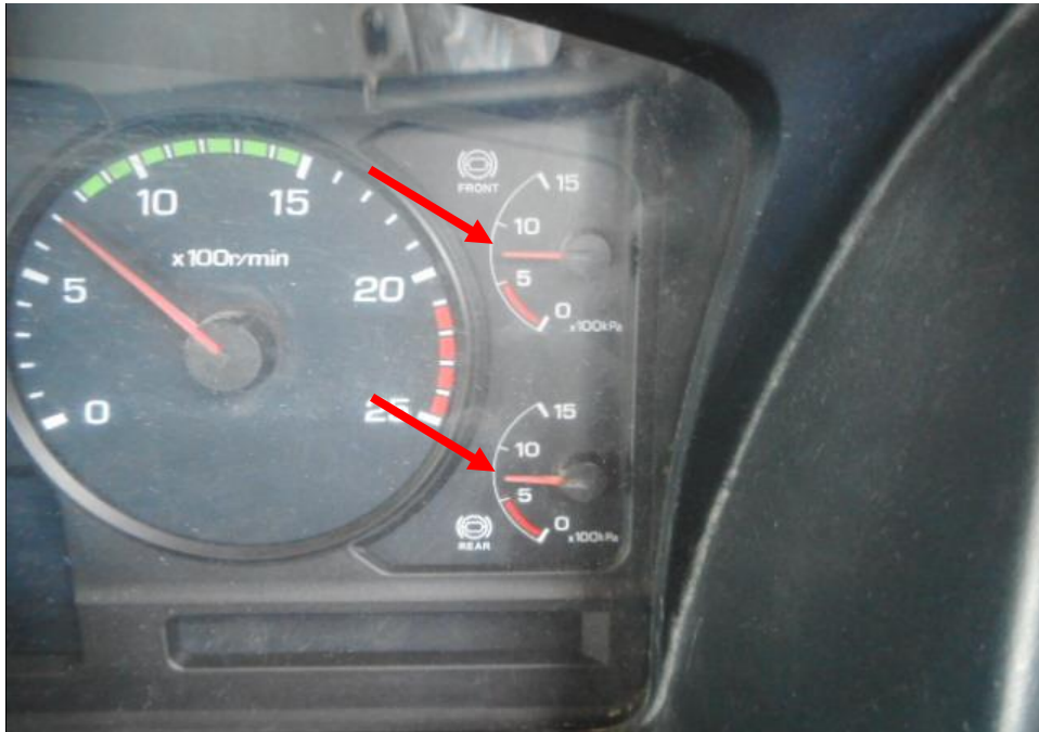
Photo 11 shows the air in the air brake cylinders of the Prime Mover at the time of my inspection. The air in the cylinder was observed to be of sufficient level & serviceable at the time of the accident.
