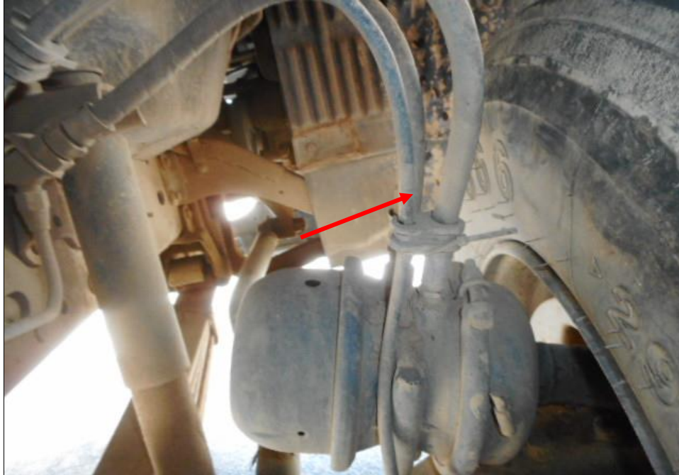
Photo 18 shows the brake pipe (arrowed) at the front right wheel of the Prime Mover. I did not observe any leakage of brake fluid at the time of my inspection of the Prime Mover. My static tests of the Prime Mover's braking system, along with my visual examination of the various mechanical components in the braking system, had indicated that there was no internal leakage of pressure/vacuum. Hence the braking system of the Prime Mover was likely to be in serviceable condition at the material time of accident.
