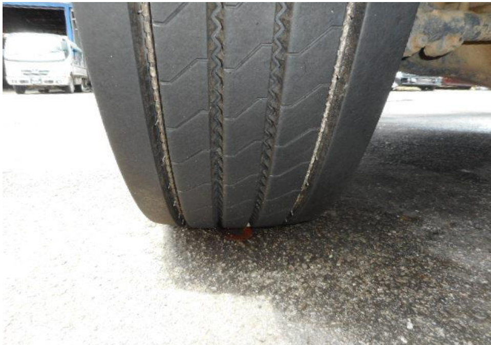
Photo 9 shows the condition of the front left tyres of the Prime Mover, which were observed to be in serviceable condition with remaining tread depth of approximately 13.7mm. There was also no tear, cut or burst mark(s) on the outer and the inner sidewalls as well as across the tread of the 6 tyres that were fitted on the Prime Mover.
