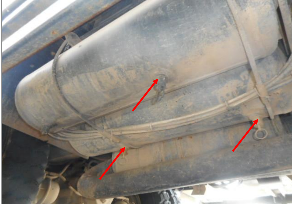
Photo 20 shows the air brake cylinders (arrowed) at the undercarriage of the Prime Mover. I did not observe any leakage of air brake fluid at the time of my inspection of the Prime Mover. My static tests of the Prime Mover's braking system, along with my visual examination of the various mechanical components in the braking system had indicated that there was no internal leakage of pressure/vacuum. Hence the braking system of the Prime Mover was likely to be in serviceable condition at the material time of accident.
