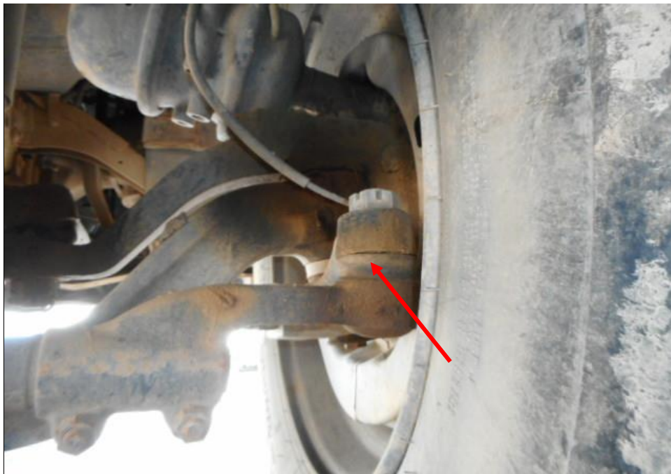
Photo 21 shows the various undercarriage components at the front right wheel of the Prime Mover, in particular the steering tie rod end (arrowed). The various steering components were all found to be intact, suggesting that the steering system of the Prime Mover was likely to be in serviceable condition at the material time of accident. There was also no sign of fluid stain(s) observed on the various undercarriage components.
