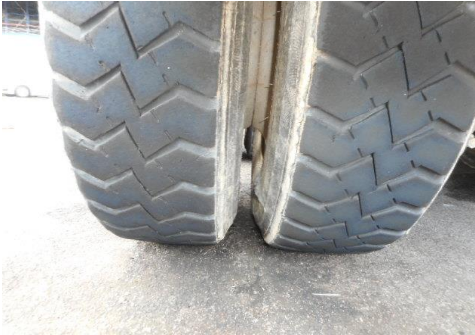
Photo 8 shows the condition of the rear left tyres of the Prime Mover, which was observed to be in serviceable condition with remaining tread depth of approximately 5.3mm. The tyres, which were wrapped around standard steel wheel rim, were also observed to be sufficiently inflated for vehicular operation. There was also no damage found on all 6 steel wheel rims of the Prime Mover.
