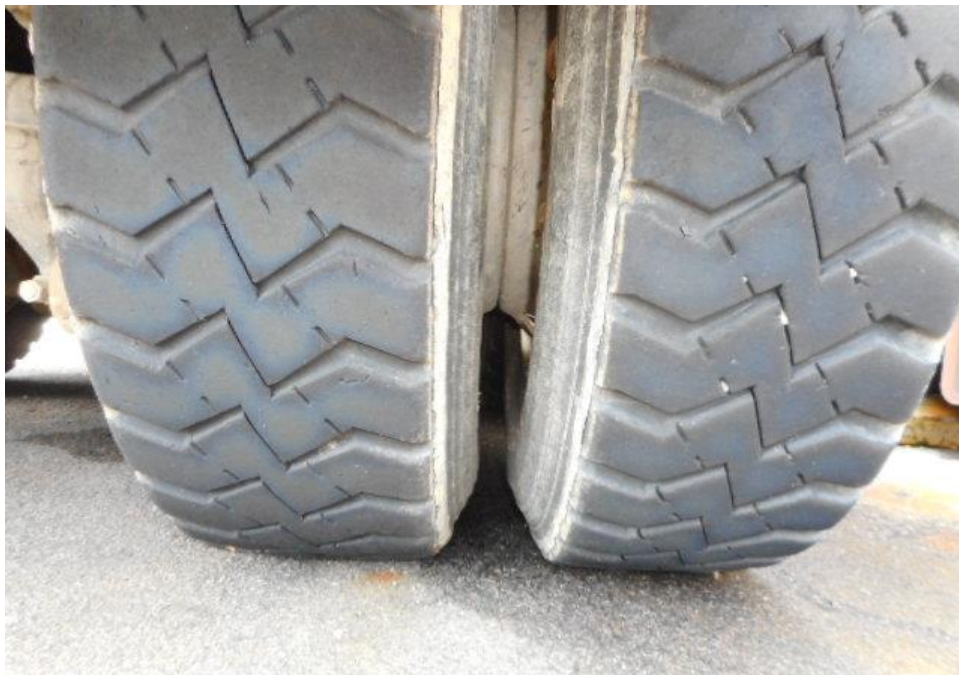
Photo 7 shows the condition of the rear right tyre of the Prime Mover, which was observed to be in serviceable condition with remaining tread depth of approximately 9.1mm. The tyre, which was wrapped around standard steel wheel rim, was also observed to be sufficiently inflated for vehicular operation.
