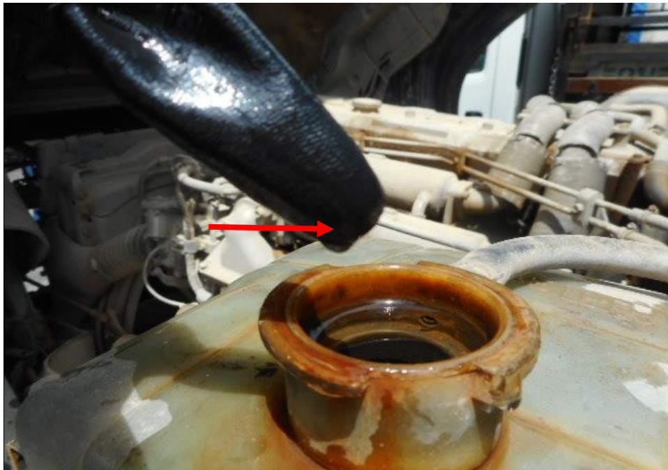
Photo 12 shows the engine coolant reservoir of the Prime Mover at the time of my inspection. The engine coolant was observed to be of sufficient level (arrowed) and without any visible contamination.
