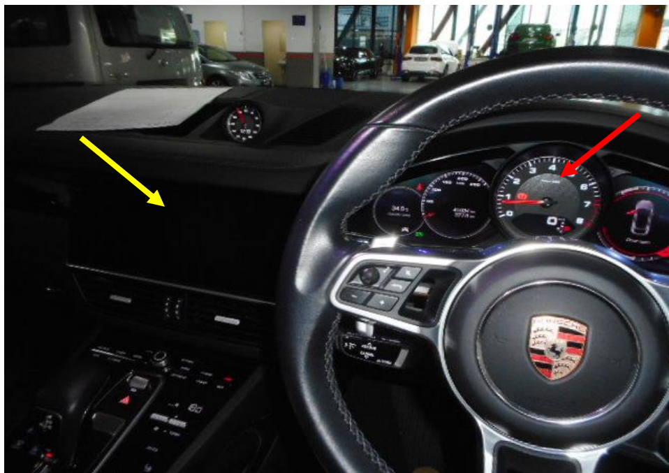
Photo 5 shows the close up view of the vehicle instrument portion of the Insured Vehicle at the time of our inspection. The driver's instrument display (red arrowed) would remained on after the vehicle's engine is turned on as compared to the centre display panel which did not turn on at all (yellow arrow).
