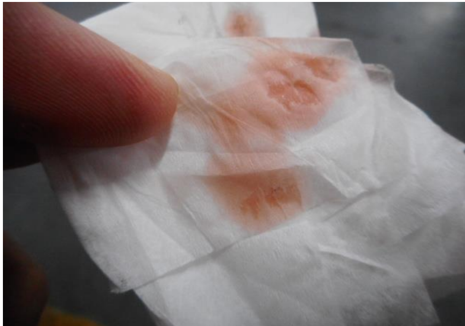
Photo 8 shows the close up view of the gearbox fluid of the Insured Vehicle at the time of our inspection. We observed that gearbox fluid was observed to be without any visible contamination.
