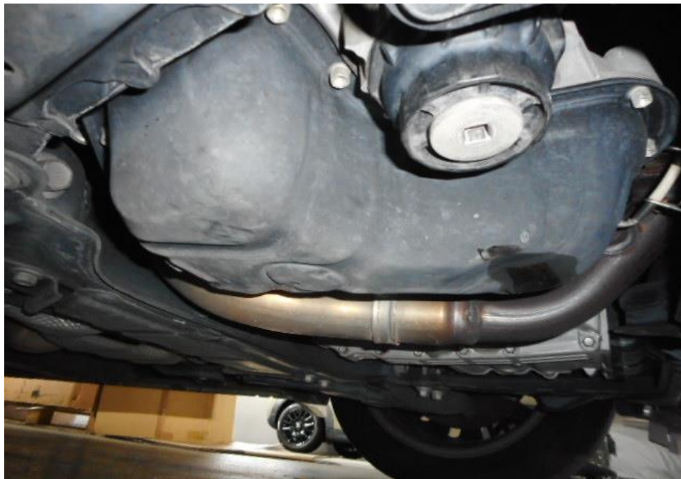
Photo 5 shows the general view of the engine and gearbox underside portion of the Insured Vehicle at the time of our inspection. The engine and transmission underside compartment is observed to be unaffected and by any signs of accident.
