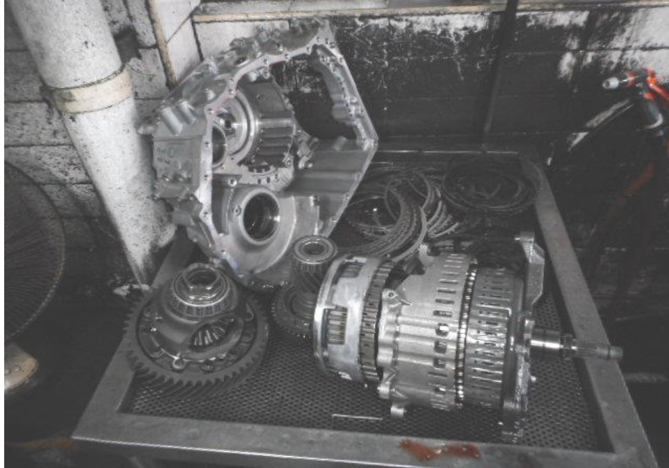
Photo 7 shows the general view of inside the gearbox unit of the Insured Vehicle at the time of our inspection. The components in the gearbox unit is observed to be unaffected and by any signs of accident.
