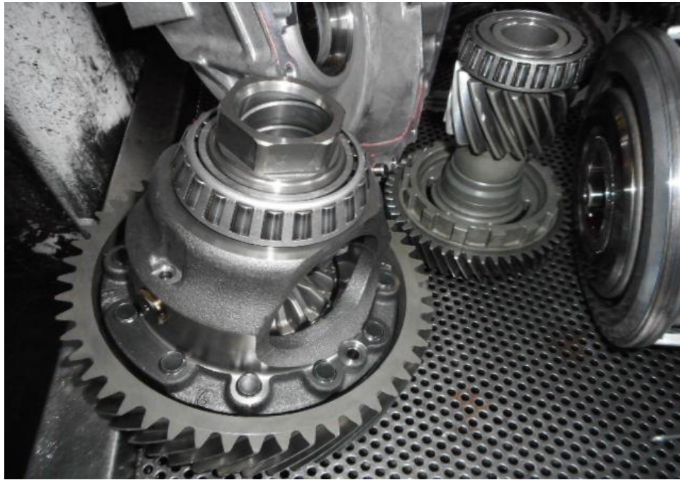
Photo 9 shows the general view of the gearbox unit of the Insured Vehicle at the time of our inspection. We observed that the gears was observed to be intact.
