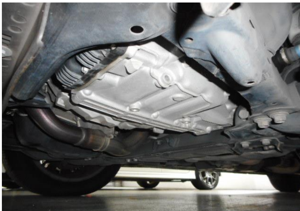
Photo 6 shows the general view of the gearbox underside portion of the Insured Vehicle at the time of our inspection. The gearbox unit was is observed unaffected and by any signs of accident.
