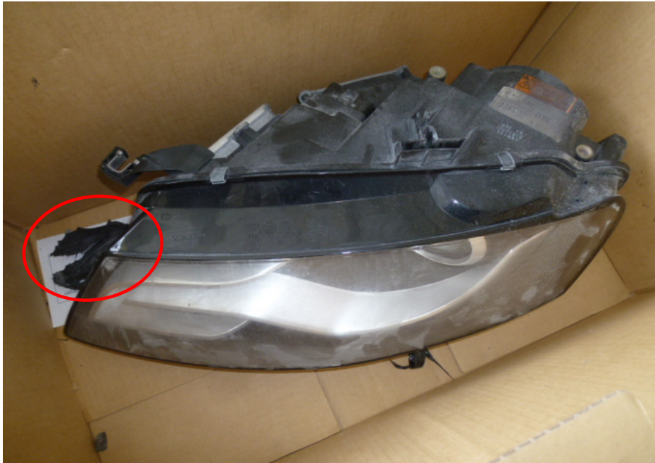
Photo 15 shows a closer view of the left front headlamp of the Insured Vehicle which had partially melted due to the heat intensity caused by the fire (circled).
