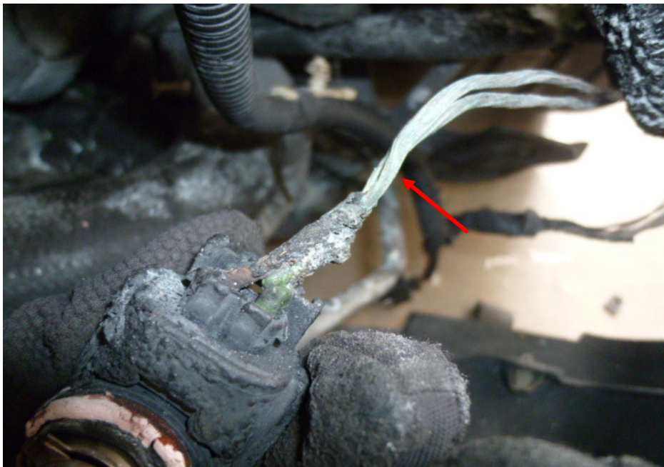
Photo 19 shows a closer view the greenish residue on the wirings leading from the left front fog lamp bulb socket of the Insured Vehicle (arrowed). The presence of such greenish residue suggests occurrence of an electrical short circuit.
