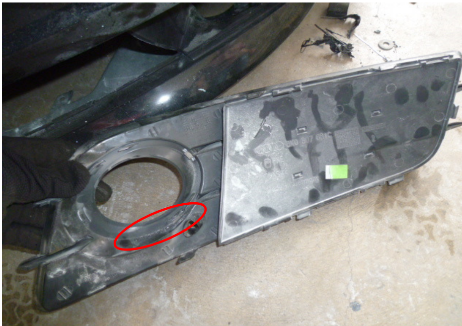
Photo 16 shows a closer view of the left front fog lamp cover of the Insured Vehicle which had partially melted due to the heat intensity caused by the fire (circled).
