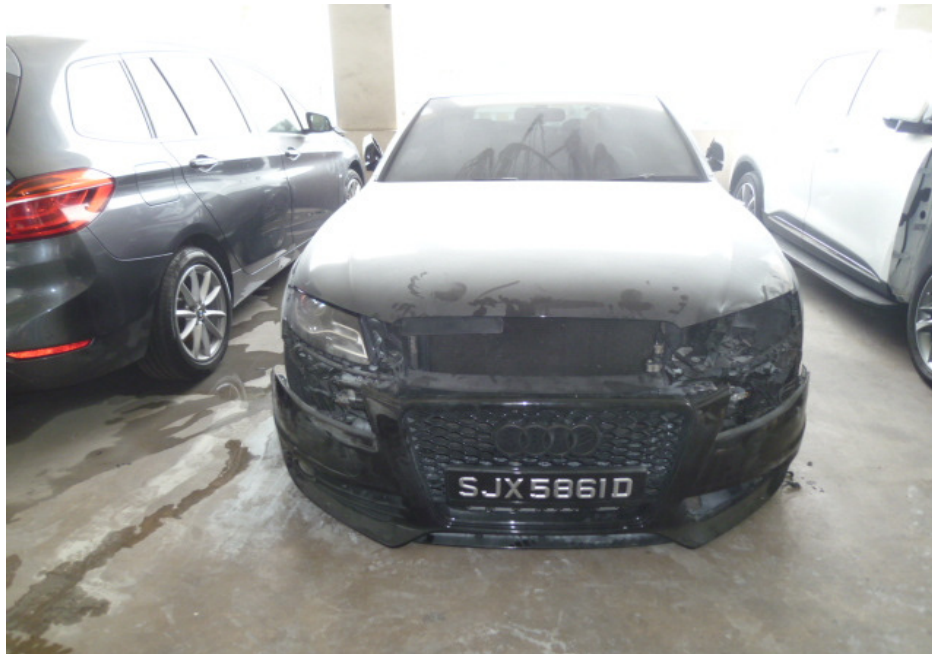
Photo 2 shows the general view of the frontal portion of the Insured Vehicle at the time of our inspection. The exterior body of the Insured Vehicle had sustained visible fire damage. This included its front bumper, front bonnet, left front headlamp and left front fog lamp.
