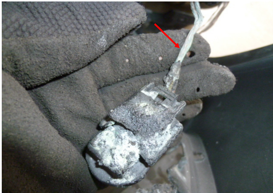
Photo 20 shows a close up view of the greenish residue on the wirings leading from the left front fog lamp bulb socket of the Insured Vehicle (arrowed). The presence of such greenish residue suggests occurrence of an electrical short circuit.
