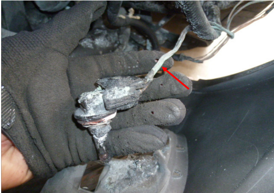
Photo 18 shows a closer view the greenish residue on the wirings leading from the left front fog lamp bulb socket of the Insured Vehicle (arrowed). The presence of such greenish residue suggests occurrence of an electrical short circuit.
