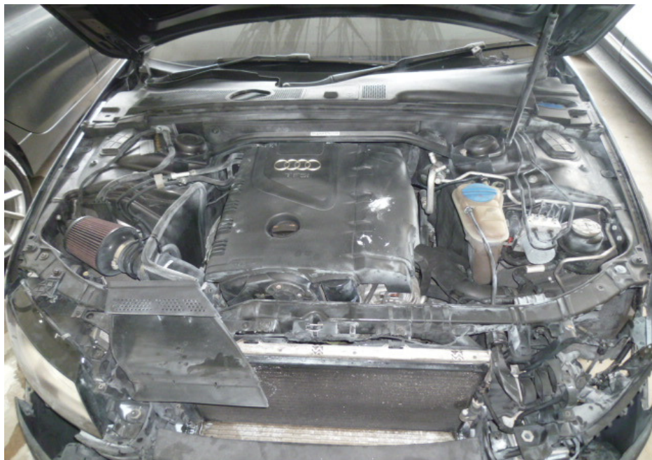
Photo 6 shows the general view of the engine compartment of the Insured Vehicle at the time of our inspection. The fire damage was confined to its interior compartment. The engine compartment of the Insured Vehicle was observed to be relatively unaffected by the fire.
