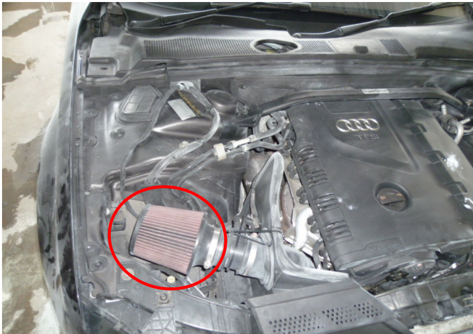
Photo 7 shows a close up view of the non- standard open- pod air filter fitted onto the Insured Vehicle upon our inspection (circled).
