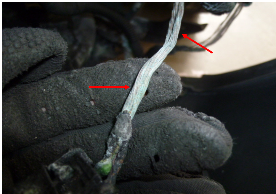
Photo 21 shows a close up view of the greenish residue on the wirings leading from the left front fog lamp bulb socket of the Insured Vehicle (arrowed). The presence of such greenish residue suggests occurrence of an electrical short circuit.
