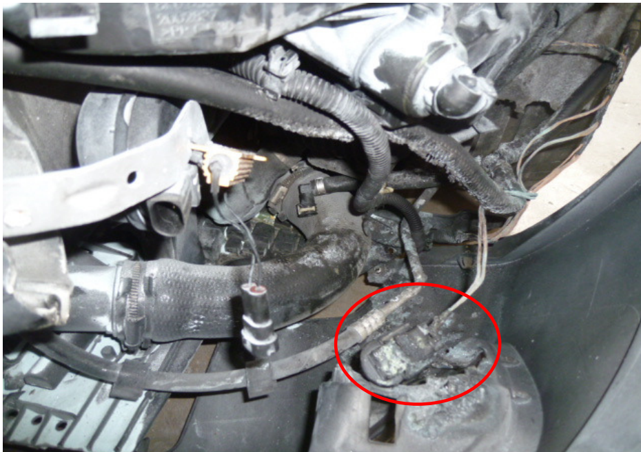
Photo 17 shows the wirings around the left front fog lamp which is near to the vicinity where the fire to the Insured Vehicle had likely started. We observed greenish residue on the wirings leading from the left front fog lamp bulb socket of the Insured Vehicle (circled). The presence of greenish residue indicates internal heating of copper wires, a sign of an electrical short circuit occurring. The greenish residue is normally left behind from oxidation as a result of chemical reaction involving the copper wires.
