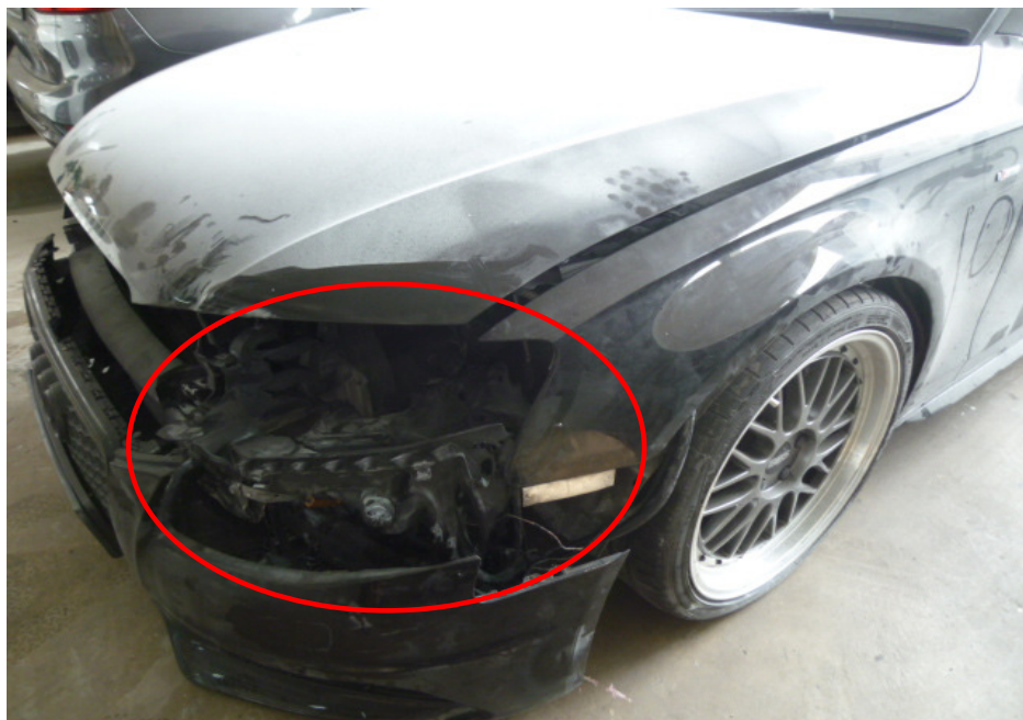
Photo 4 shows a closer view of the left front body of the Insured Vehicle at the time of our inspection. The exterior body of the Insured Vehicle had sustained visible fire damage. This included its front bumper, front bonnet, left front headlamp and left front fog lamp (circled).
