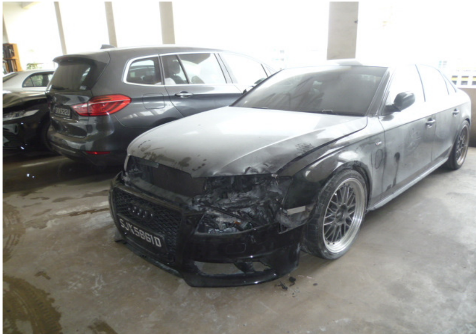
Photo 3 shows a closer view of the left front body of the Insured Vehicle at the time of our inspection. The exterior body of the Insured Vehicle had sustained visible fire damage. This included its front bumper, front bonnet, left front headlamp and left front fog lamp.
