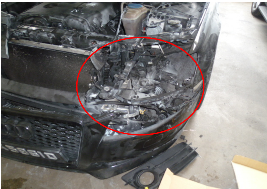
Photo 12 shows the burn pattern and the nature of fire damage on the left front portion of the Insured Vehicle. The heat intensity caused several plastic components which included the left front headlamp, left front fog lamp and left front fog lamp cover to melt (circled).
