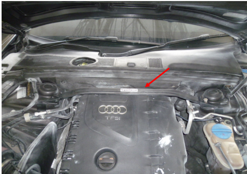
Photo 8 shows the aftermarket engine strut bar fitted on the Insured Vehicle (arrowed).
