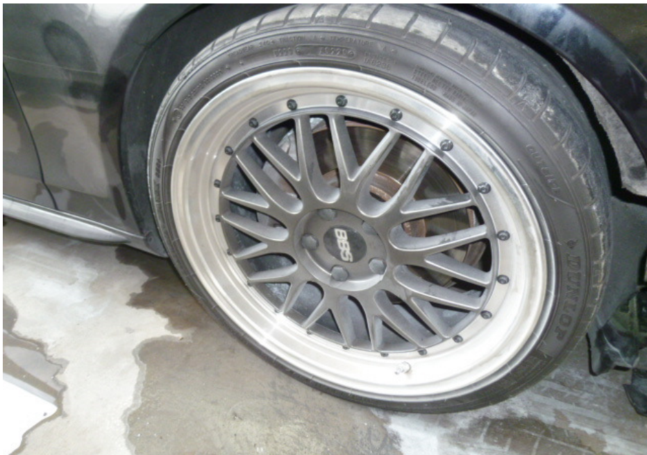
Photo 11 shows the non-standard rim found to be fitted on the Insured Vehicle at the time of our inspection. The 19- inch alloy rims fitted on the Insured Vehicle were not the standard type for the Insured Vehicle.
