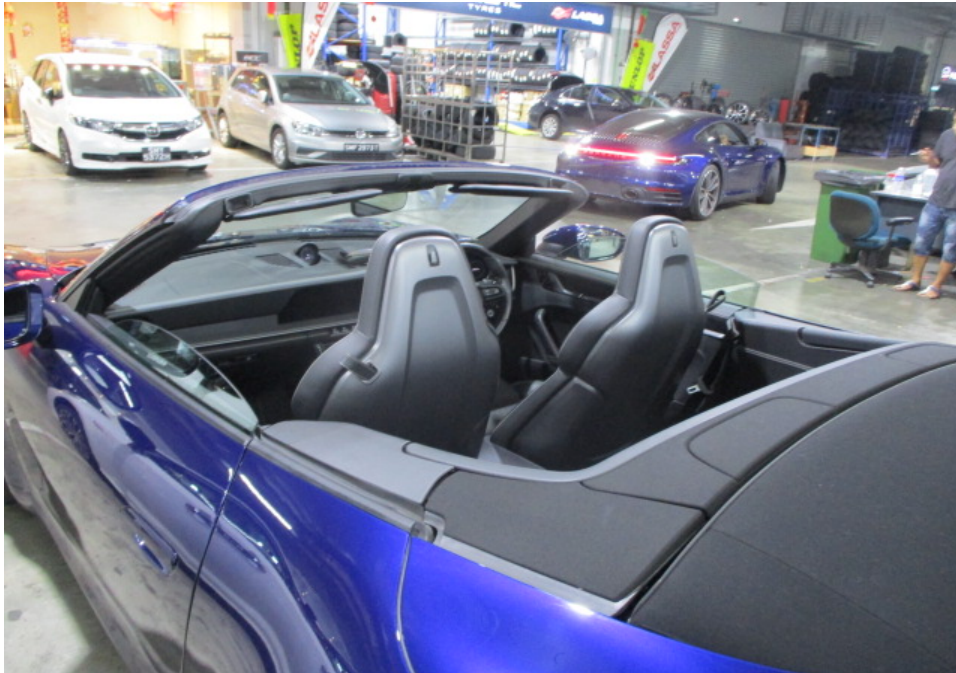
Photo 19 shows another view of the Motor Car with its soft top roof completely folded. It was observed that as a safety feature, the soft top roof could only open and close when the Motor Car was in a stationary position. When opened, the soft top roof is completely folded into the rear compartment with no parts protruding out of the Motor Car's body. The soft top roof was also found adequately secured to the "A" pillar after closing.
