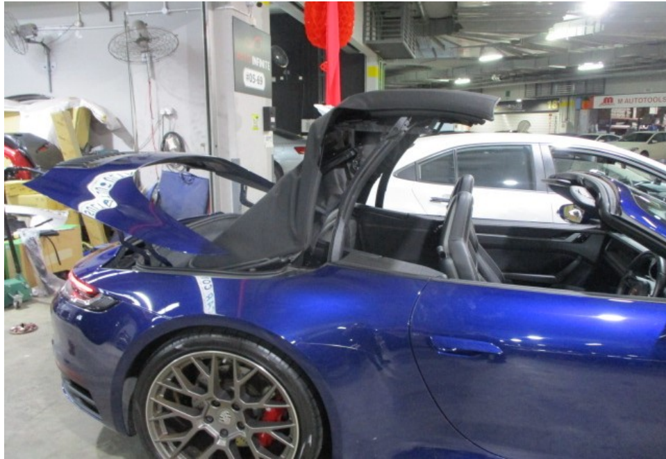
Photo 17 shows the Motor Car's soft top roof being tested. It was observed that as a safety feature, the soft top roof could only open and close when the Motor Car was in a stationary position. When opened, the soft top roof is completely folded into the rear compartment with no parts protruding out of the Motor Car's body. The soft top roof was also found adequately secured to the "A" pillar after closing.
