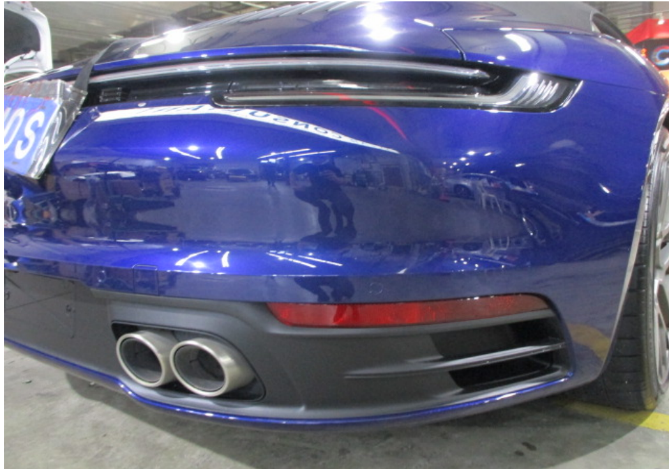
Photo 7 shows a closer view of the Motor Car's rear bumper, rear bumper right lower grille and rear bumper right reflector. The body parts at the rear right portion of the Motor Car were visually examined and it was observed that the repair/restoration works carried out to the damaged area of the Motor Car (refer to photograph 2 & 3 above) were reasonably adequate and in order.
