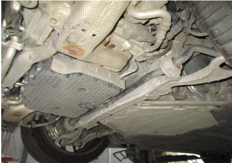
Photo 29 shows another view of the Motor Car's engine compartment. The engine compartment was at the rear underside of the Motor Car. The various parts and components within the engine compartment were all observed to be intact and properly fitted. There was also no sign(s) or indication(s) of fluid leak and/or fluid stain found inside the engine compartment.
