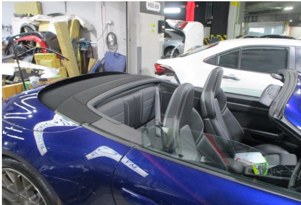
Photo 18 shows the Motor Car with its soft top roof completely folded. It was observed that as a safety feature, the soft top roof could only open and close when the Motor Car was in a stationary position. When opened, the soft top roof is completely folded into the rear compartment with no parts protruding out of the Motor Car's body. The soft top roof was also found adequately secured to the "A" pillar after closing.
