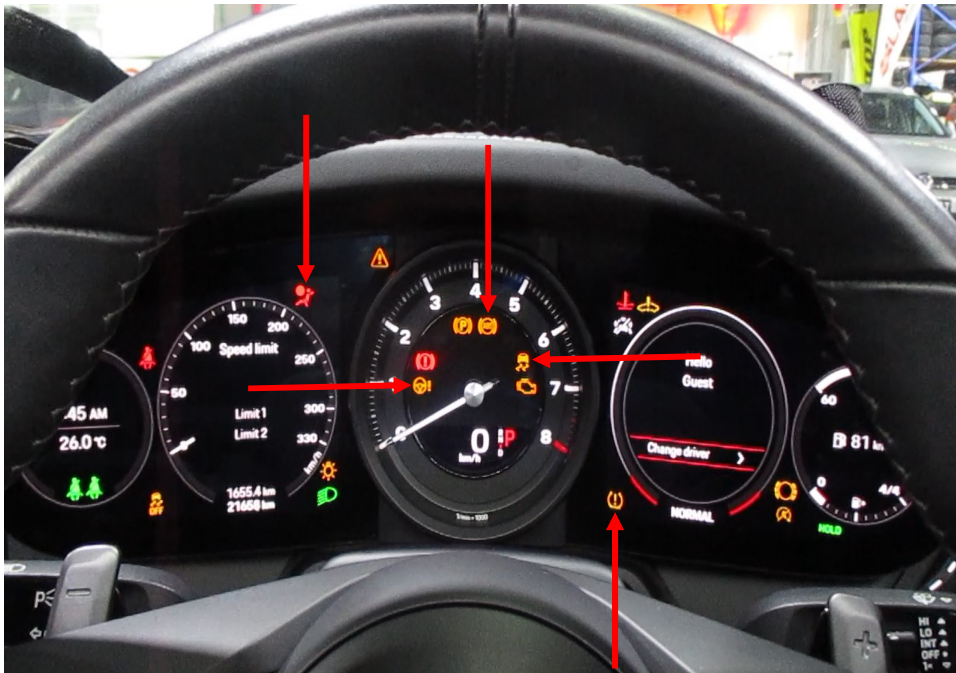
Photo 20 shows the warning lights for the various electronic safety features appearing on the instrument panel of the Motor Car during its self-test when the engine is cranked, in particular the ABS, SRS, EPS, TPM and TCS lights (arrowed).
