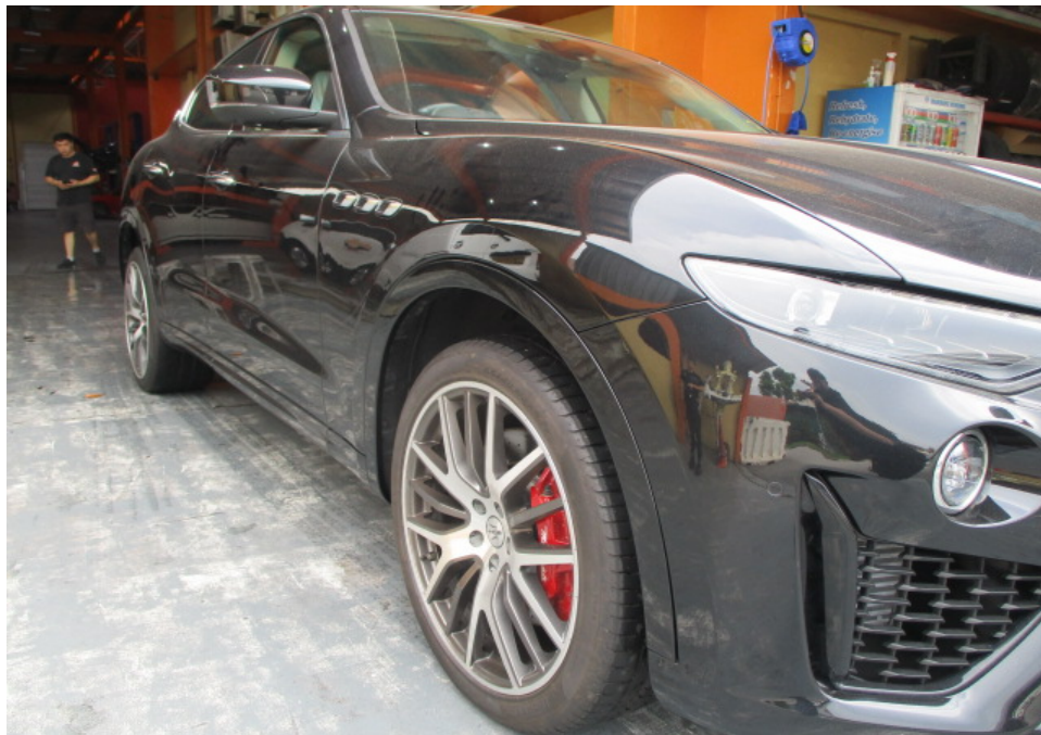
Photo 7 shows a closer view of the Motor Car's front bonnet, front right headlamp, front right fender, front right fender wheel arc garnish, front right wheel rim and front right tyre. The body parts at the front right portion of the Motor Car were visually examined and it was observed that the repair/restoration works carried out to the damaged area of the Motor Car (refer to photograph 1 above) were reasonably adequate and in order.
