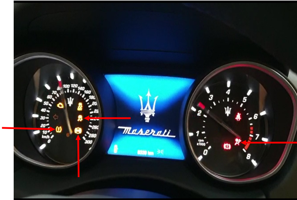
Photo 16 shows the warning lights for the various electronic safety features appearing on the instrument panel of the Motor Car during its self-test when the engine is cranked, in particular the ABS, SRS, TPM and TCS lights (arrowed).
