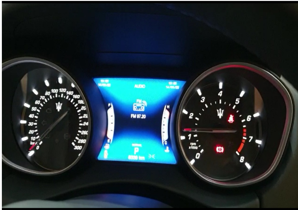
Photo 17 shows the respective warning lights no longer illuminated, indicating that there is no fault detected to the ABS, SRS, TPM and TCS lights systems of the Motor Car during the self-test. These electronic systems were hence in working condition at the time of my inspection.
