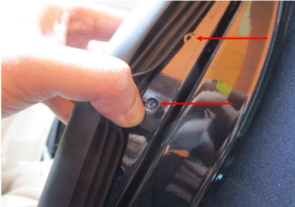
Photo 30 shows the left side “C” pillar of the Motor Car. I did not find any weld marks other than original spot weld marks (arrowed) on the left side “C” pillar of the Motor Car, which indicates that there was no re-welding works carried out. In general, I had found all the non-detachable body panels of the Motor Car to be originally fitted at the time of my inspection, except for the rear left body panel.
