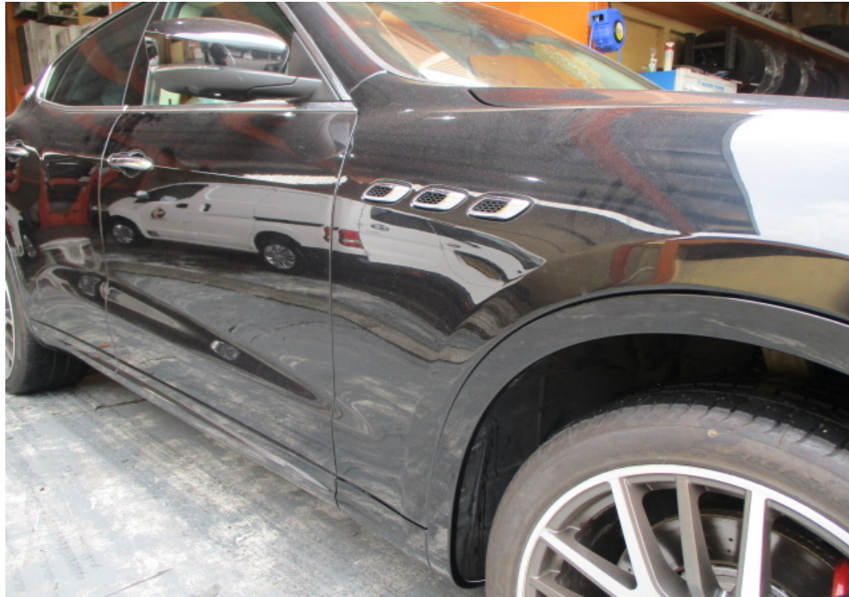
Photo 8 shows a closer view of the Motor Car's front right fender, front right fender wheel arc garnish and front right door at the time of my inspection. The body parts at the front right portion of the Motor Car were visually examined and it was observed that the repair/restoration works carried out to the damaged area of the Motor Car (refer to photograph 1 above) were reasonably adequate and in order.
