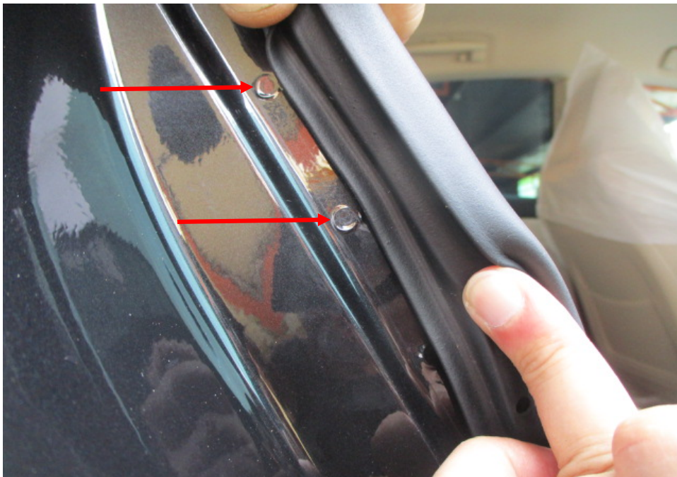
Photo 31 shows the right side “C” pillar of the Motor Car. I did not find any weld marks other than original spot weld marks (arrowed) on the right side “C” pillar of the Motor Car, which indicates that there was no re-welding works carried out. In general, I had found all the non-detachable body panels of the Motor Car to be originally fitted at the time of my inspection, except for the rear left body panel
