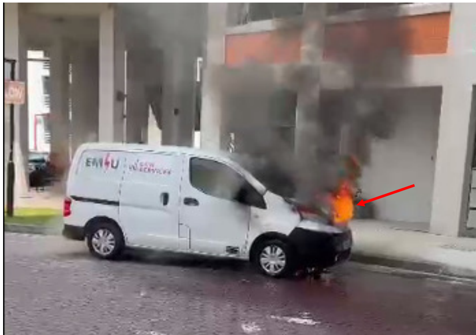
Photo 14 shows the Insured Vehicle on fire before the arrival of the SCDF. In general, the information that could be gathered from this photograph had corresponded to the events that were related to us by Mr Nur, which is the fire had started from the engine compartment of the Insured Vehicle (arrowed).
