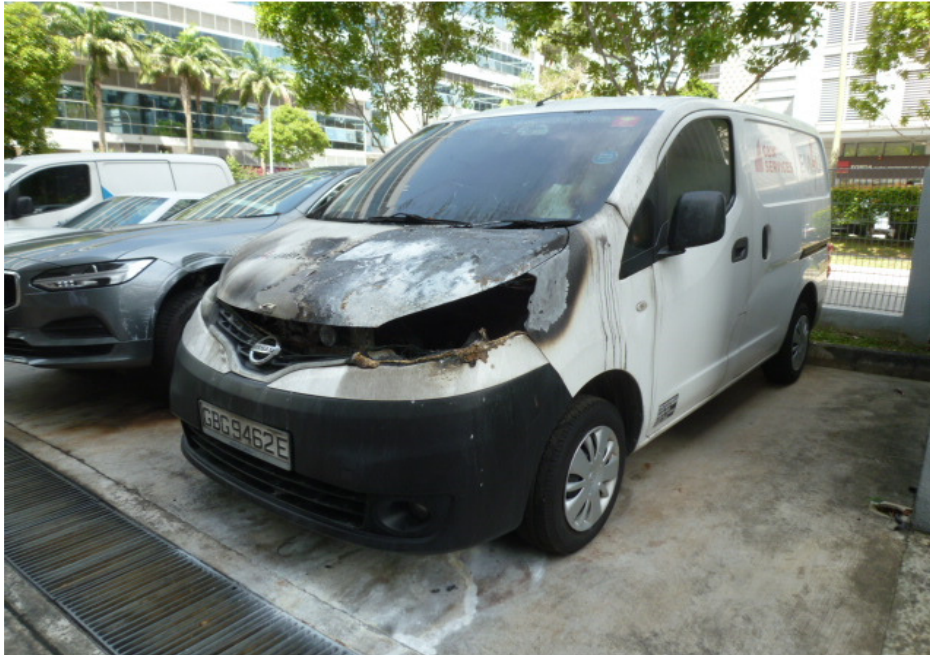
Photo 3 shows the closer view of the left front body of the Insured Vehicle at the time of our inspection. The fire damage to the Insured Vehicle was confined to its frontal portion. Its front bumper, front bonnet, front grille, front headlamps, front windscreen and front windscreen wipers were amongst the body parts that were found to have been affected by the fire.
