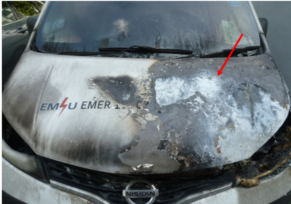
Photo 7 shows the burn pattern that was found on the left portion of the front bonnet of the Insured Vehicle (arrowed). Such whitish burn marks are a result of exposure to prolonged heat intensity, which may indicate where the fire had started. Rust would also begin to develop on these areas soon after the fire.
