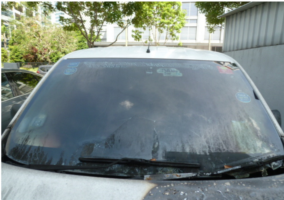
Photo 4 shows the general view of the front windscreen of the Insured Vehicle at the time of our inspection. The fire damage to the front windscreen was severe.
