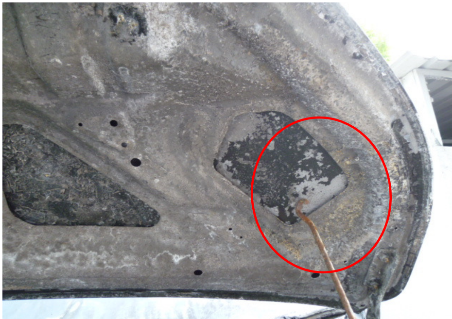
Photo 9 shows the rust that had developed on the underside of the front bonnet, around the left portion (circled). The development of rust is an indication that this area was subjected to prolonged exposure to high heat intensity, which had caused the steel/metal material of the front bonnet to be exposed to natural environmental condition. Hence the fire to the Insured Vehicle can be determined to have originated towards the left portion of the engine compartment.
