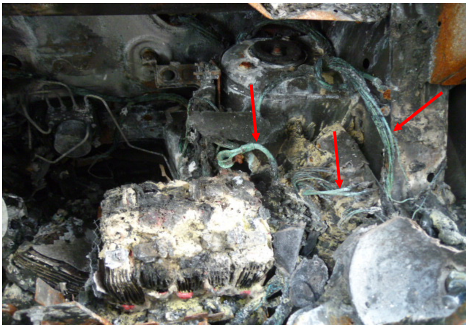
Photo 11 shows a closer view of the greenish residue found on some of the burnt stretches of original factory fitted wirings (arrowed). The presence of such greenish residue suggests occurrence of an electrical short circuit.
