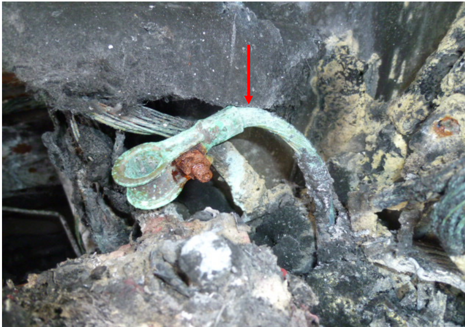
Photo 12 shows a close up view of the greenish residue found on some of the burnt stretches of original factory fitted wirings (arrowed). The presence of such greenish residue suggests occurrence of an electrical short circuit.
