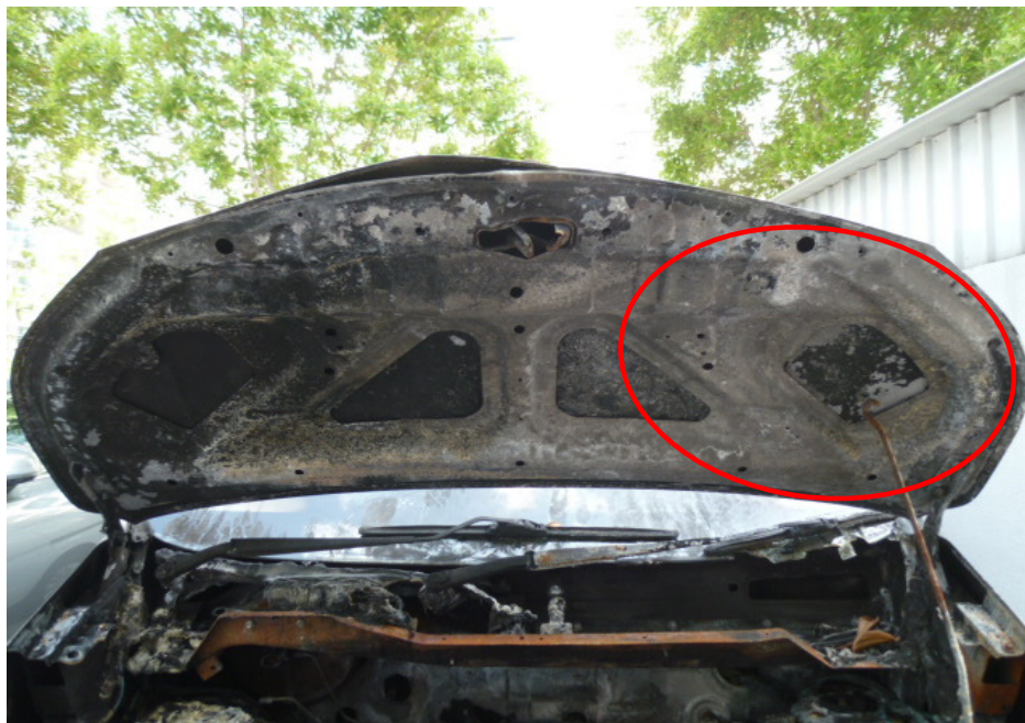
Photo 8 shows the whitish marks that were found on the underside of the front bonnet of the Insured Vehicle, at the left portion (circled). Such whitish burn marks are a result of exposure to prolonged heat intensity, which may indicate where the fire had started. Rust would also begin to develop on these areas soon after the fire.
