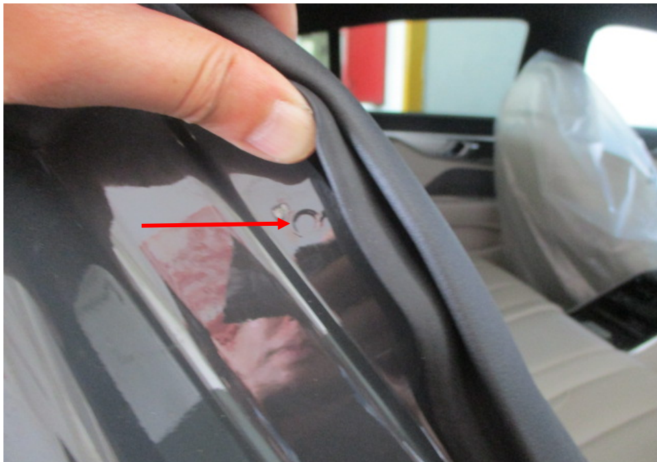
Photo 32 shows the right side "C" pillar of the Motor Car. I did not find any weld marks other than original spot weld marks (arrowed) on the right side "C" pillar of the Motor Car which, indicates that there was no re-welding works carried out. In general, I had found all the non-detachable body panels of the Motor Car to be originally fitted at the time of my inspection.
