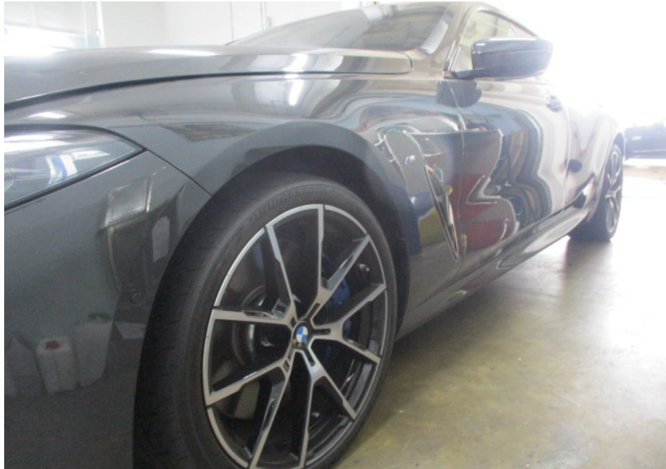
Photo 9 shows a closer view of the Motor Car's front left fender, front left wheel rim and front bonnet at the time of my inspection. The body parts at the front left portion of the Motor Car were visually examined and it was observed that the repair/restoration works carried out to the damaged area of the Motor Car (refer to photograph 1 - 3 above) were reasonably adequate and in order.
