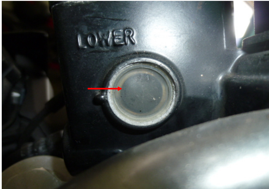
Photo 24 shows a close up view of the brake fluid reservoir for the front brake of the Motorcycle. The brake fluid was observed to be of sufficient level for operational purposes (arrowed).
