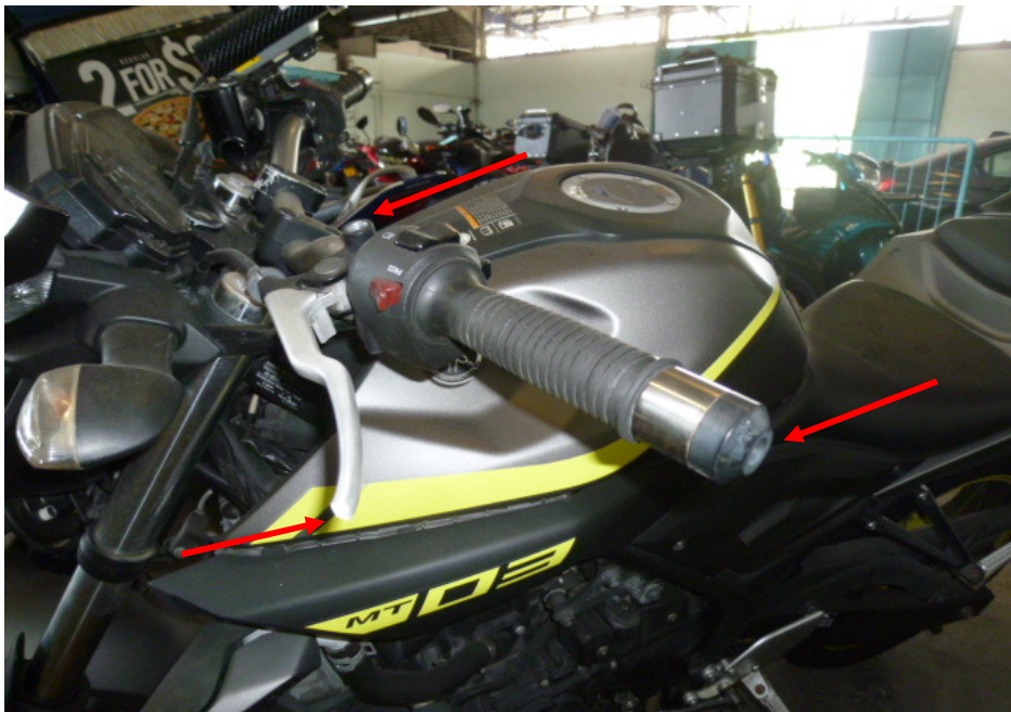
Photo 7 shows a closer view of the left handlebar end, left side mirror and clutch lever (arrowed) which were amongst the body parts of the Motorcycle that had sustained damage as a result of the accident.
