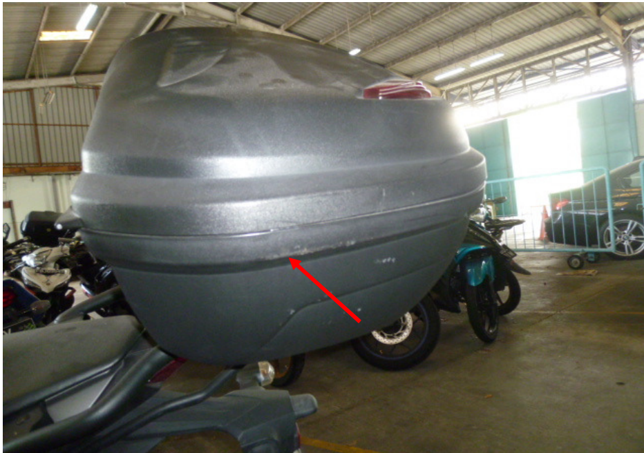
Photo 11 shows a closer view of the top box of the Motorcycle that had sustained damages of grazing nature as a result of the accident (arrowed).
