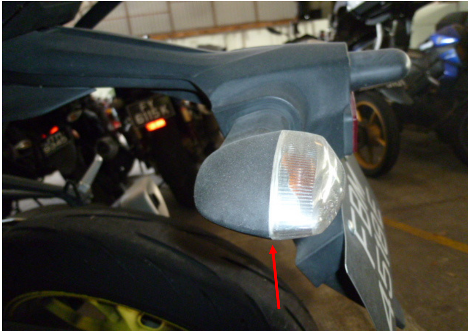
Photo 10 shows a closer view of the grazed left rear signal lamp of the Motorcycle as a result of the accident (accident).
