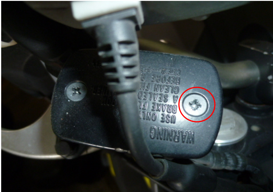
Photo 23 shows the brake fluid reservoir cover for the front brake of the Motorcycle. We were unable to examine whether the front brake fluid was without contamination due to the worn out screw (circled).
