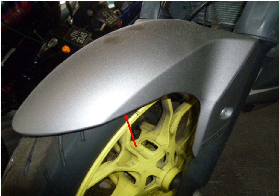
Photo 5 shows a closer view of the front mudguard (arrowed) which was amongst the body parts at the front body of the Motorcycle that had sustained damage as a result of the accident.
