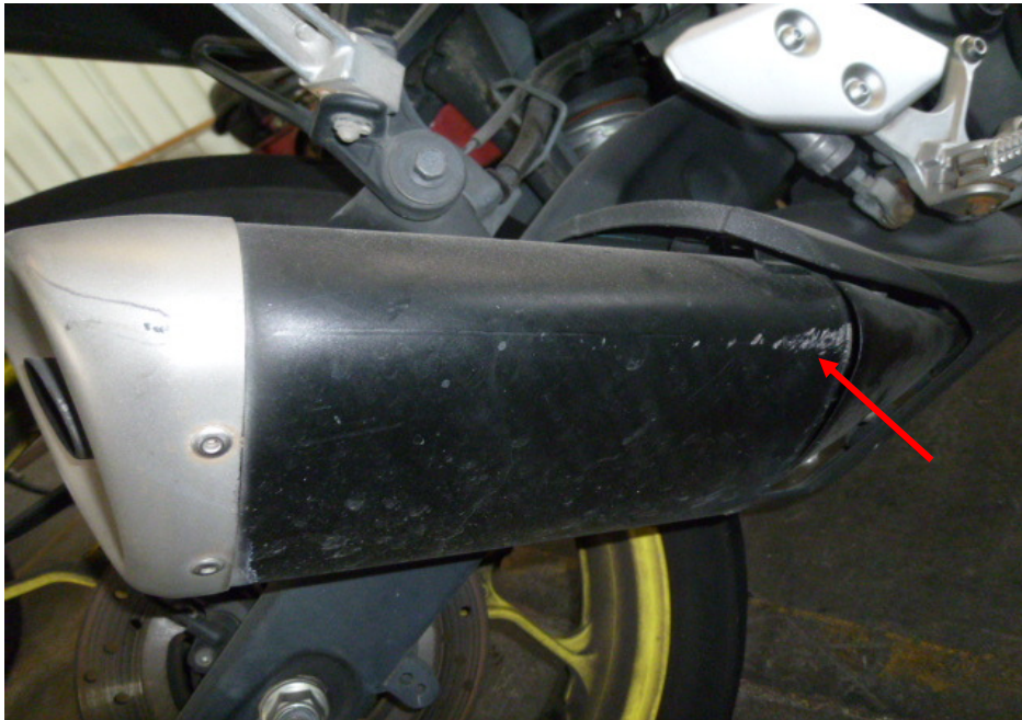
Photo 12 shows a closer view of the exhaust muffler of the Motorcycle that had sustained damages of grazing nature as a result of the accident (arrowed).
