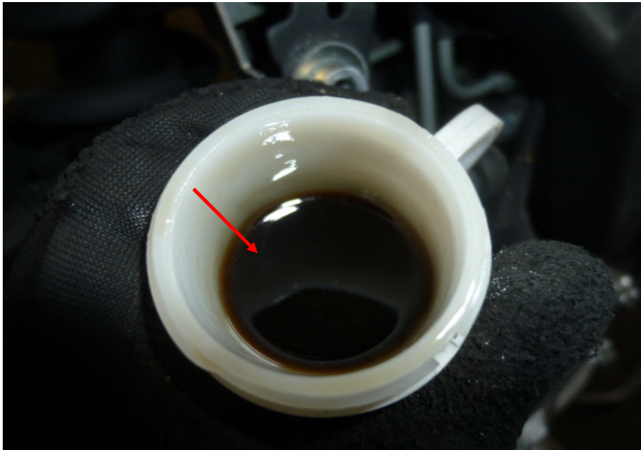
Photo 27 shows a close up view of the brake fluid reservoir for the rear brake of the Motorcycle. The brake fluid for the rear brake was observed to be of sufficient level for operational purposes. However it was found to be slightly contaminated (arrowed).
