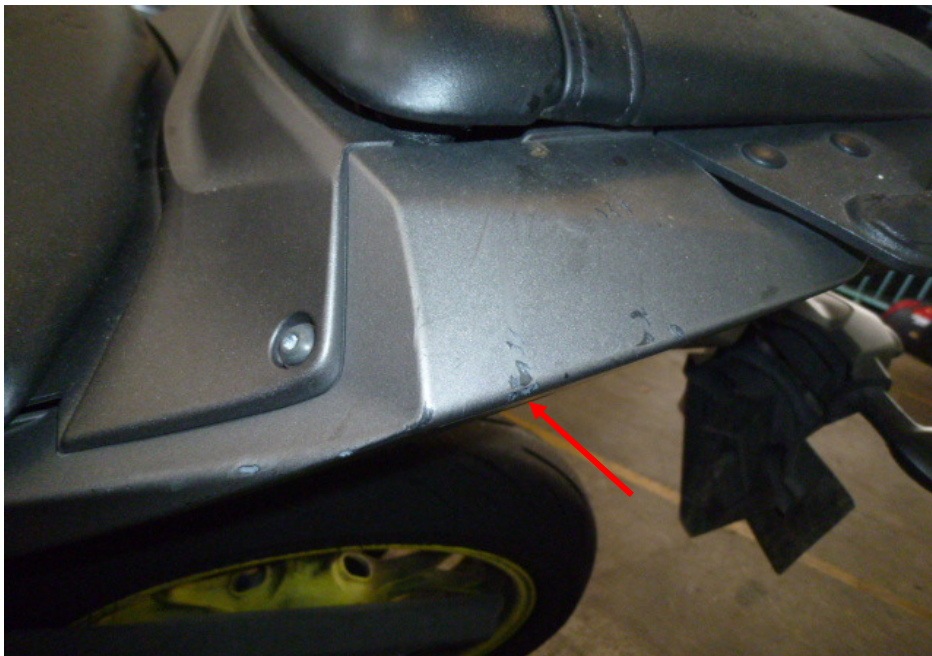
Photo 9 shows a closer view of the left rear side cover of the Motorcycle that had sustained damages of grazing nature as a result of the accident (arrowed).
