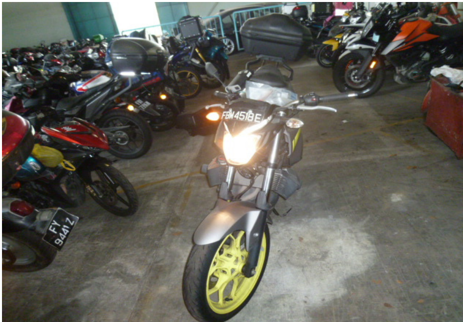
Photo 21 shows the front wheel of the Motorcycle turned towards its full right. Turning the Motorcycle's handle bar towards the left and right did not produce any abnormal free play and/or resistance. This would indicate that the steering system of the Motorcycle was in serviceable condition at the time of our inspection.
