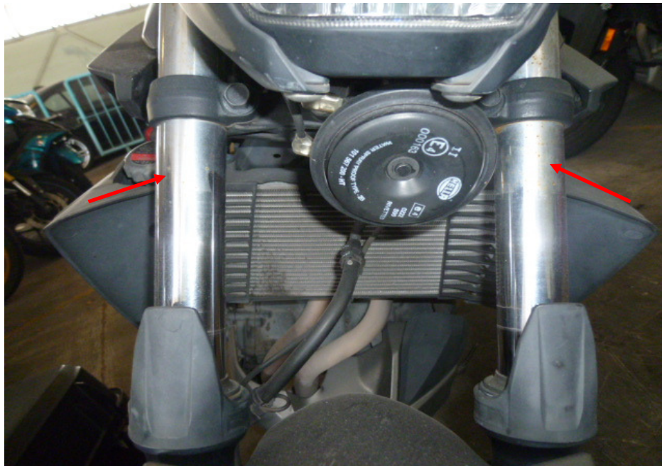
Photo 19 shows the front forks (arrowed) of the Motorcycle. The front fork and fork bracket of the Motorcycle were both found to be intact and undamaged. Turning the Motorcycle's handle bar towards the left and right did not produce any abnormal free play and/or resistance. The steering system of the Motorcycle was in serviceable condition at the time of our inspection.
