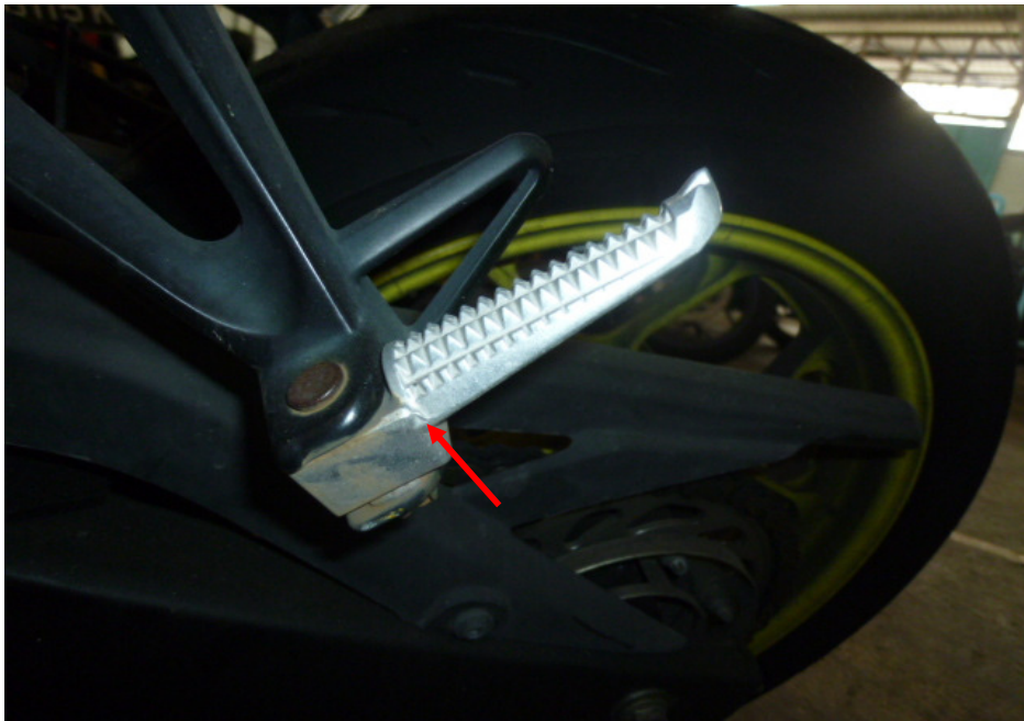
Photo 8 shows a closer view of the left pillion foot peg (arrowed) which was amongst the body parts of the Motorcycle that had sustained damage as a result of the accident
