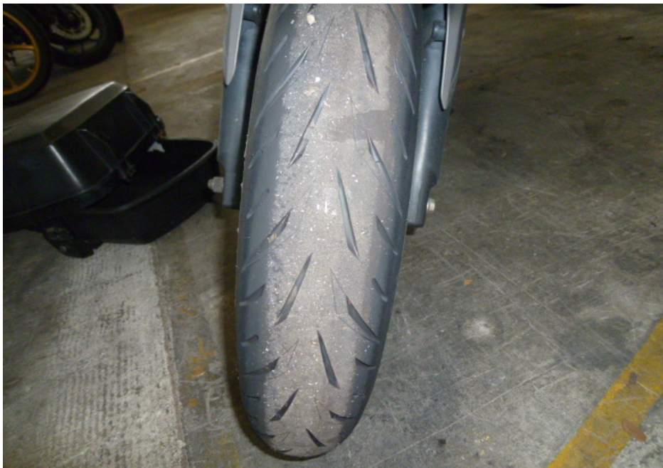
Photo 13 shows the condition of the Motorcycle's front tyre. The front tyre was observed to be in serviceable condition with remaining tread depth of approximately 3mm. There was no tear, burst mark(s) and/or punctured hole(s) on the sidewalls as well as across the tread of the front tyre.
