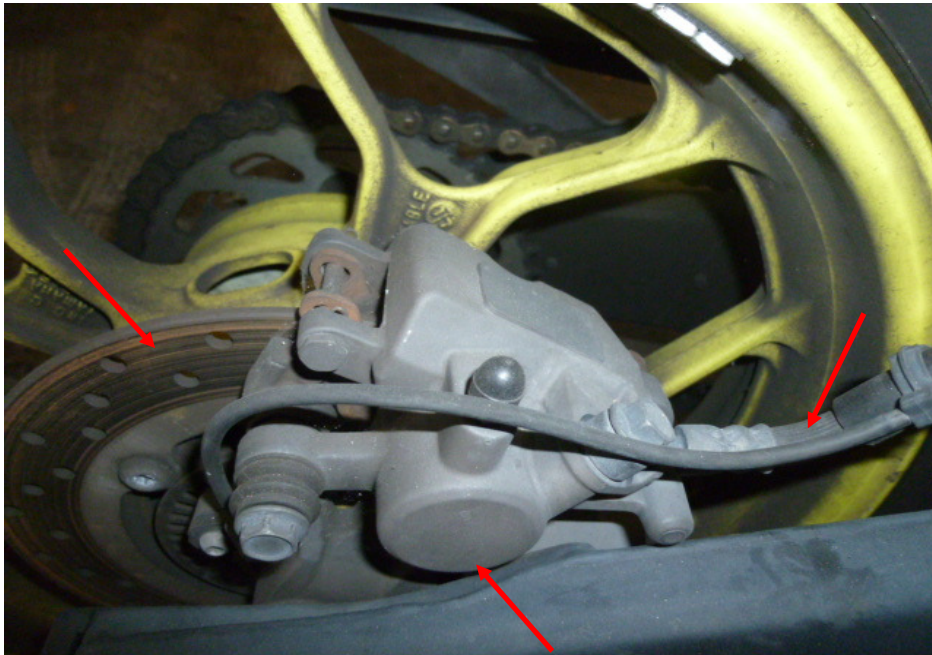
Photo 26 shows a close up view of the rear brake caliper, rear brake disc and rear brake hose (arrowed) of the Motorcycle, which are all part of the components in the hydraulic rear brake system of the Motorcycle. Our visual checks of these various components had revealed all to be intact with no visible damage. No leakage of brake fluid was also observed.
