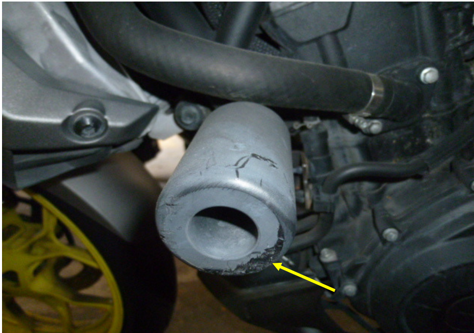
Photo 6 shows a closer view of the left frame slider of the Motorcycle that had sustained damages of grazing nature as a result of the accident (arrowed).
