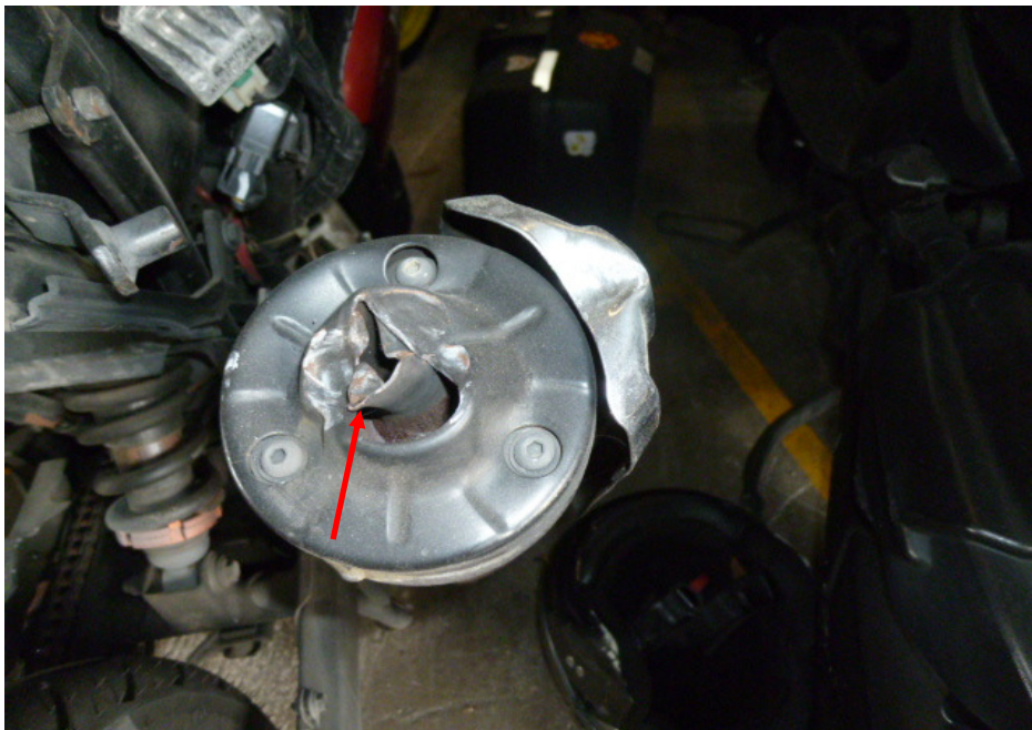
Photo 11 shows a closer view of the dented exhaust muffler of the Motorcycle as a result of the accident (arrowed).
