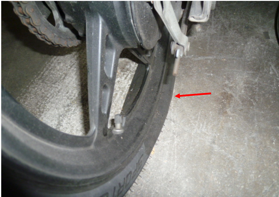
Photo 16 shows the deflated rear tyre (arrowed) of the Motorcycle at the time of our inspection.
