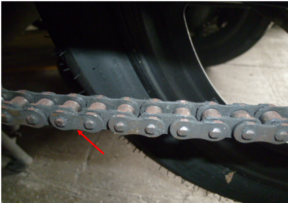
Photo 22 shows a closer view of the gear train (arrowed) of the Motorcycle, which was observed to be intact with no misalignment. It was also adequately lubricated for operating purposes.
