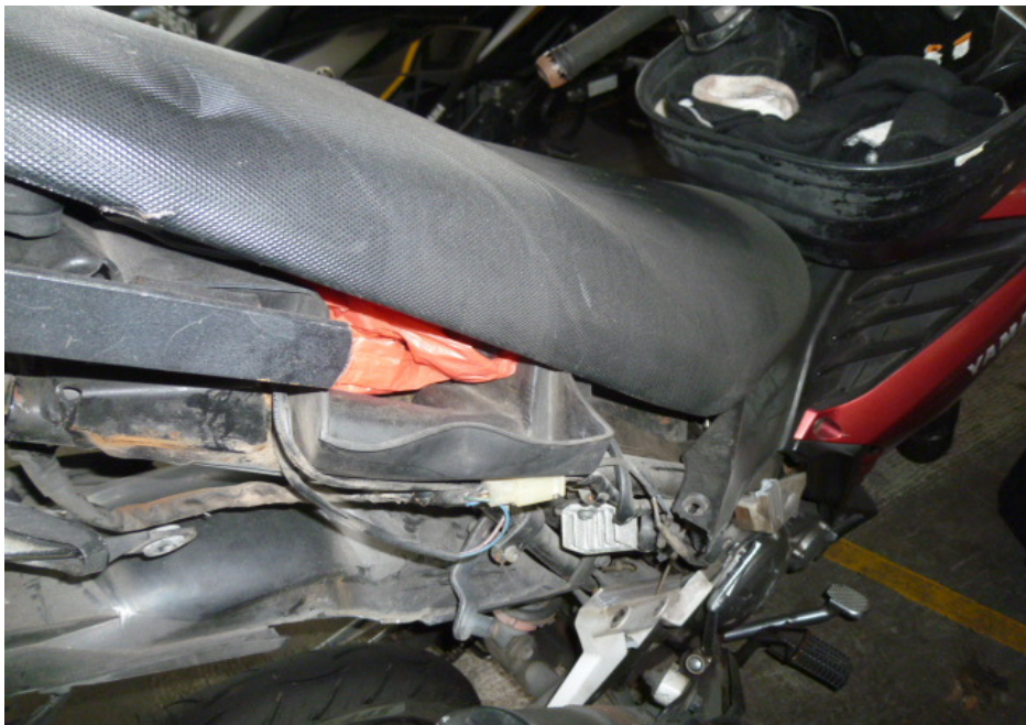
Photo 14 shows a closer view of the missing right rear side cover of the Motorcycle as a result of the accident.
