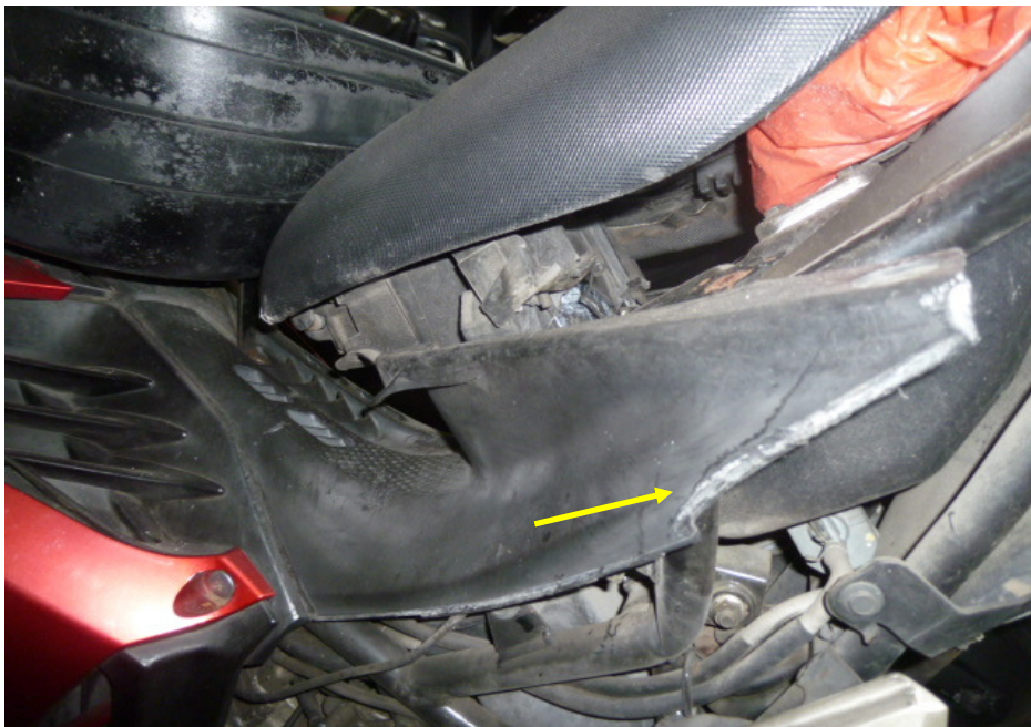
Photo 10 shows a closer view of the deformed centre cowling of the Motorcycle as a result of the accident (arrowed).
