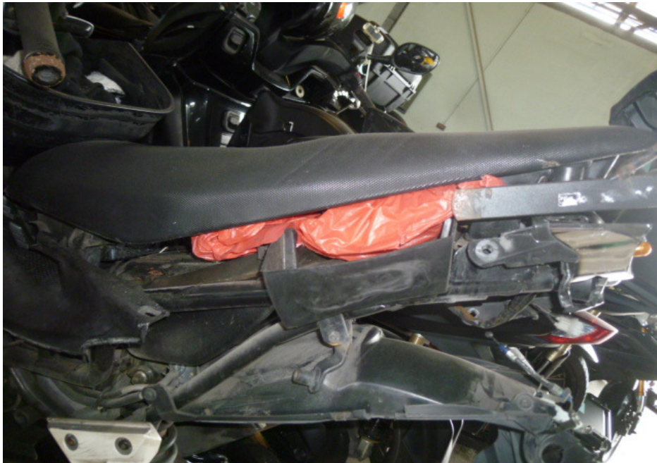
Photo 16 shows a closer view of the missing left rear side cover of the Motorcycle as a result of the accident.
