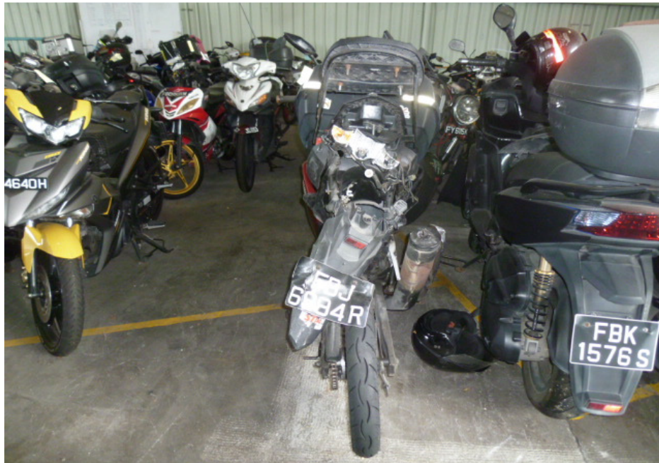
Photo 4 shows a general view of the rear portion of the Motorcycle at the time of our inspection. The Motorcycle was observed to have sustained damages all around. The body parts that were found to have been damaged include its headlight assembly, front cowling, front mudguard, centre cowling, left cowling, side mirrors, front brake lever, handlebar ends, gear shift pedal, rear brake pedal, left front footrest, right pillion foot peg bracket, rear side covers, exhaust muffler and tail light assembly, amongst others.
