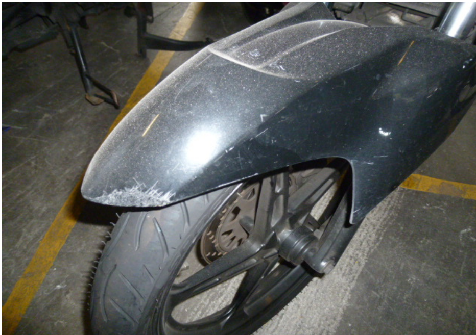
Photo 5 shows a closer view of the front mudguard which was amongst the body parts of the Motorcycle that had sustained damage as a result of the accident.
