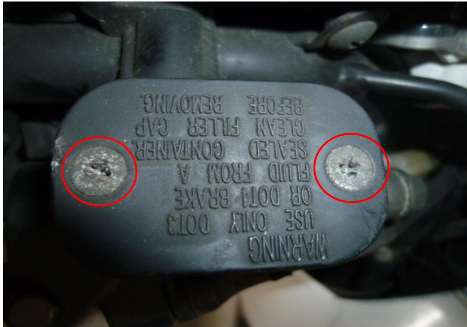
Photo 26 shows the brake fluid reservoir cover for the front brake of the Motorcycle. We were unable to examine whether the front brake fluid was without contamination due to worn out screws (circled).
