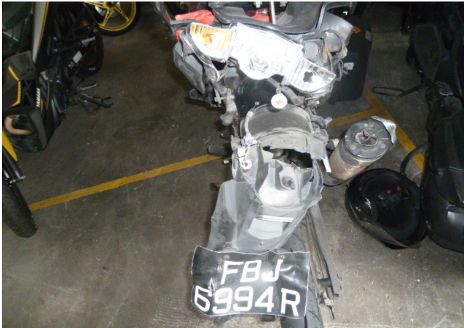
Photo 15 shows a closer view of the deformed tail light assembly of the Motorcycle as a result of the accident.
