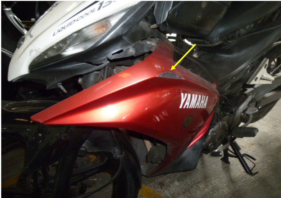
Photo 10 shows a closer view of the grazed left cowling of the Motorcycle as a result of the accident (arrowed).
