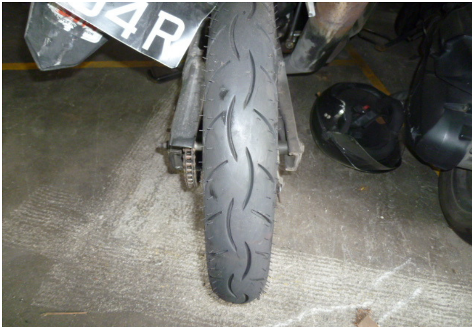
Photo 18 shows the condition of the Motorcycle's rear tyre. The rear tyre was observed to be in serviceable condition with remaining tread depth of approximately 5mm. There was no tear, burst mark(s) and/or punctured hole(s) on the sidewalls as well as across the tread of the rear tyre. However the rear tyre was observed to be deflated.
