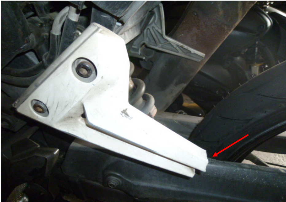
Photo 12 shows the broken left pillion foot peg bracket of the Motorcycle as a result of the accident (arrowed).
