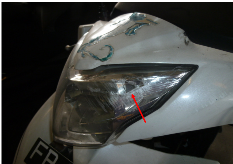
Photo 7 shows the headlight assembly (arrowed), which was amongst the body parts of the Motorcycle that had sustained damage as a result of the accident.
