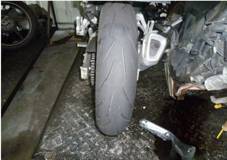
Photo 18 shows the condition of the Motorcycle's rear tyre. The rear tyre was observed to be in serviceable condition with remaining tread depth of approximately 6mm. The tyre was also observed to be sufficiently inflated for vehicular operation. We did not observe any tear, burst mark(s) and/or punctured hole(s) on the sidewalls as well as across the tread of the rear tyre.
