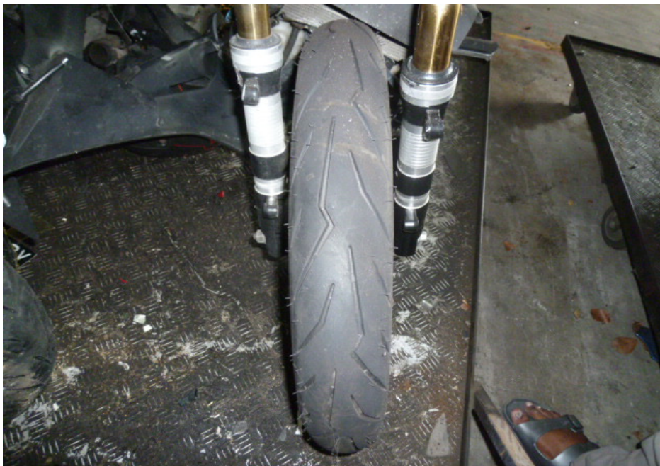
Photo 16 shows the condition of the Motorcycle's front tyre. The front tyre was observed to be in serviceable condition with remaining tread depth of approximately 4mm. There was no tear, burst mark(s) and/or punctured hole(s) on the sidewalls as well as across the tread of the front tyre. However the front tyre was observed to be deflated.
