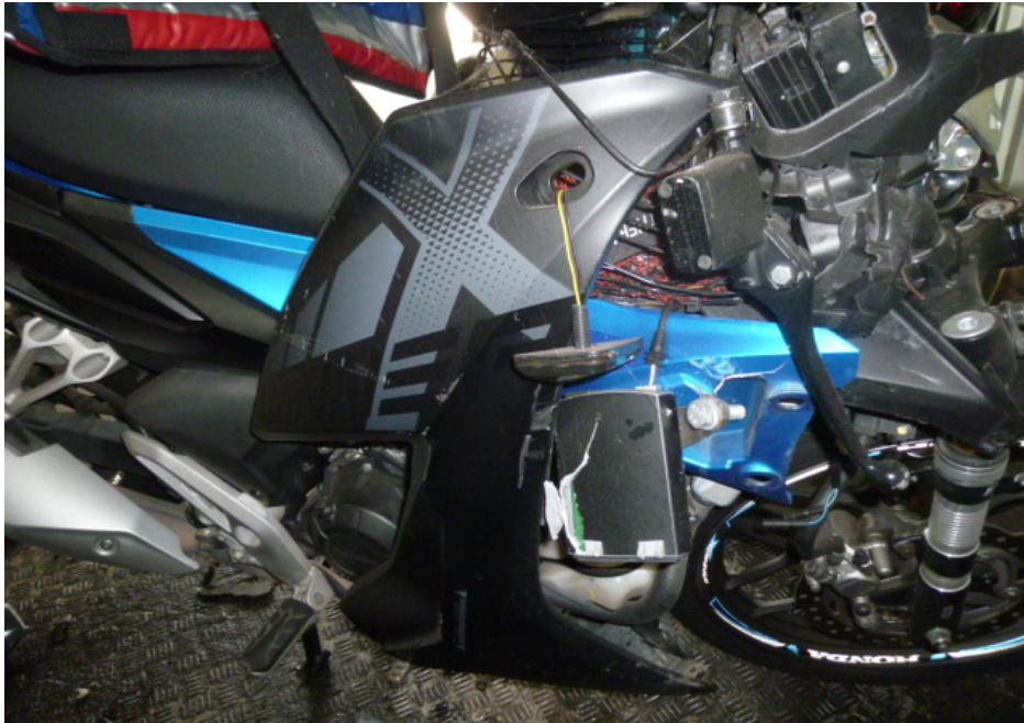
Photo 11 shows the cracked right cowling which was amongst the body of the Motorcycle that had sustained damage as a result of the accident.
