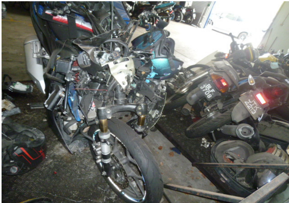
Photo 4 shows a general view of the frontal portion of the Motorcycle at the time of our inspection. The Motorcycle was observed to have sustained damages all around. The body parts that were found to have been damaged include its speedometer gauge, headlight assembly, side cowlings, handlebar, side mirrors, clutch lever, front brake lever, handlebar ends, radiator, front basket, gear shift pedal, left front footrest, rear side covers and exhaust muffler, amongst others.
