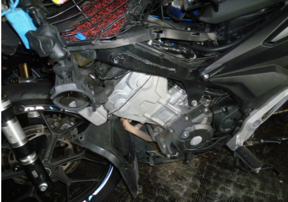
Photo 10 shows the missing left cowling which was amongst the body of the Motorcycle that had sustained damage as a result of the accident.
