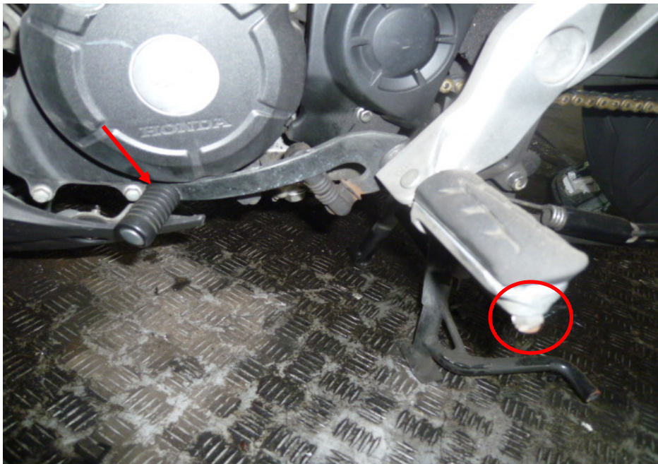
Photo 12 shows a closer view of the gear shift pedal (arrowed) and left front footrest (circled) which was amongst the body parts of the Motorcycle that had sustained damage as a result of the accident.
