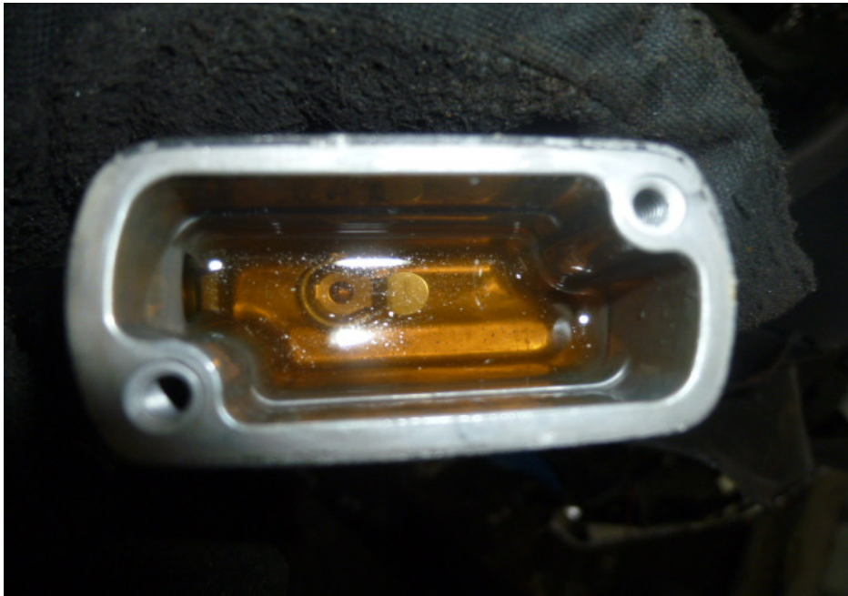
Photo 25 shows the brake fluid reservoir for the front brake of the Motorcycle. The brake fluid was observed to be of sufficient level for operational purposes and without contamination.
