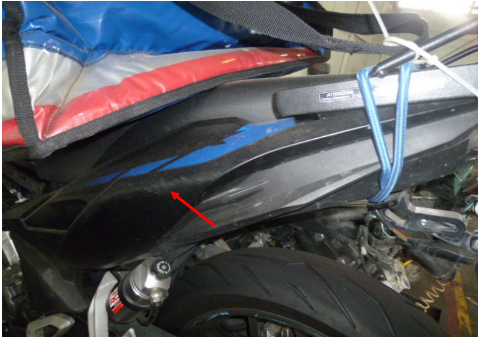
Photo 13 shows a closer view of the grazed left rear side cover (arrowed) which was amongst the body parts of the Motorcycle that had sustained damage as a result of the accident.
