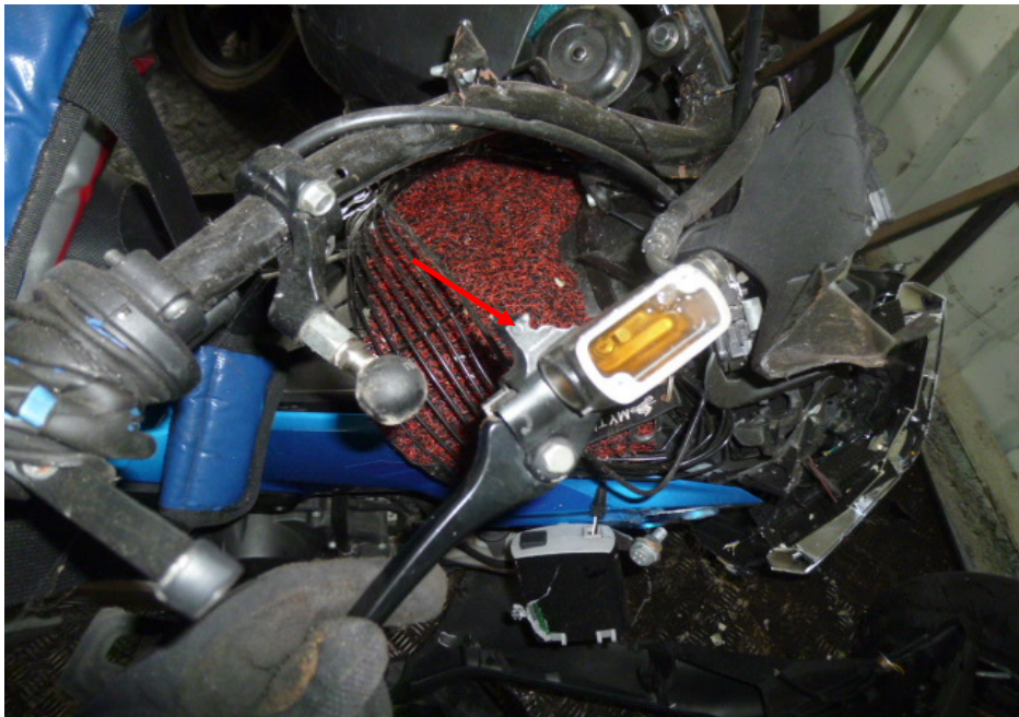
Photo 26 shows the front brake reservoir. We were unable to depress the front brake lever as part of front brake master pump had broken off as a result of the accident (arrowed). Hence we were unable to determine if there was any leakage of pressure/vacuum in the front brake system.
