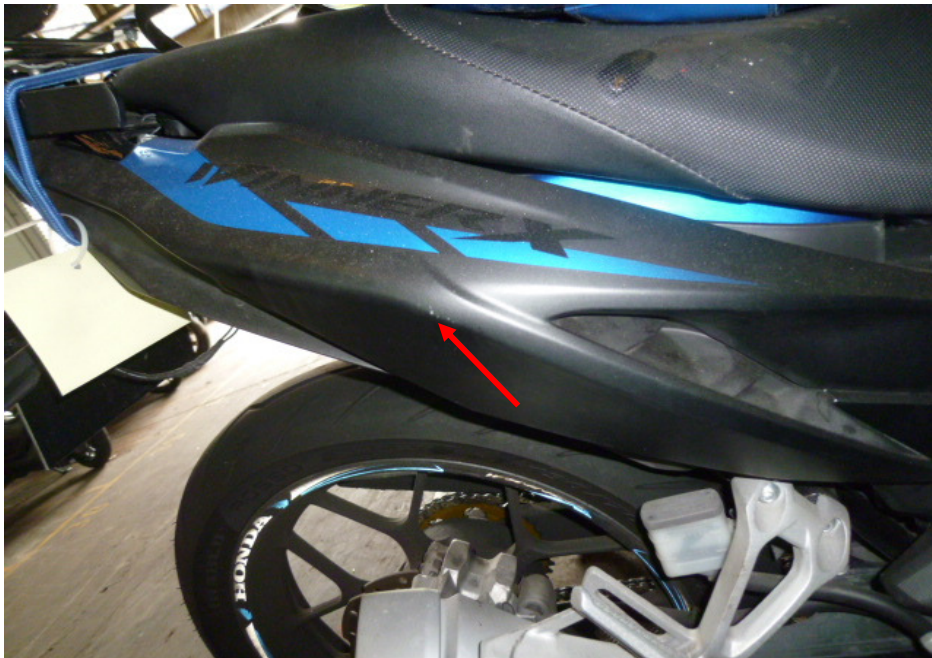
Photo 14 shows a closer view of the grazed right rear side cover (arrowed) which was amongst the body parts of the Motorcycle that had sustained damage as a result of the accident.
