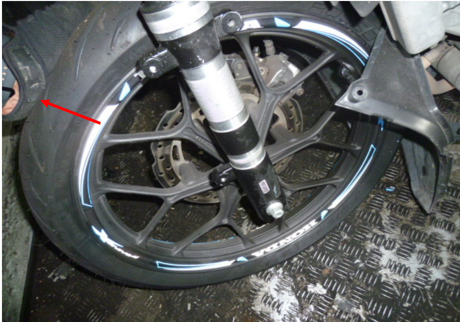
Photo 17 shows the deflated front tyre (arrowed) of the Motorcycle at the time of our inspection.
