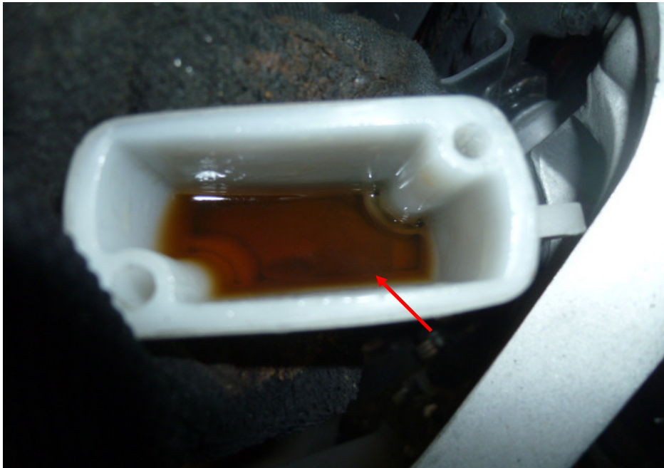
Photo 28 shows a close up view of the brake fluid reservoir for the rear brake of the Motorcycle. The rear brake fluid was observed to be of sufficient level for operational purposes. However it was found to be slightly contaminated (arrowed).
