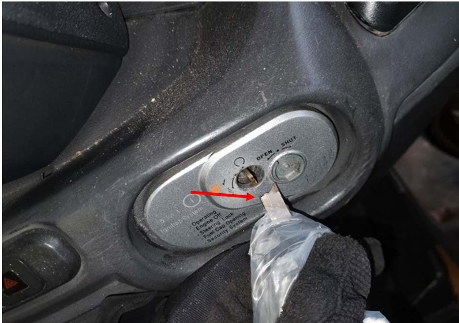
Photo 1 shows the ignition of the Motorcycle at the time of our inspection. The mileage of the Motorcycle could not be recorded at the time of our inspection due to a broken key (arrowed).
