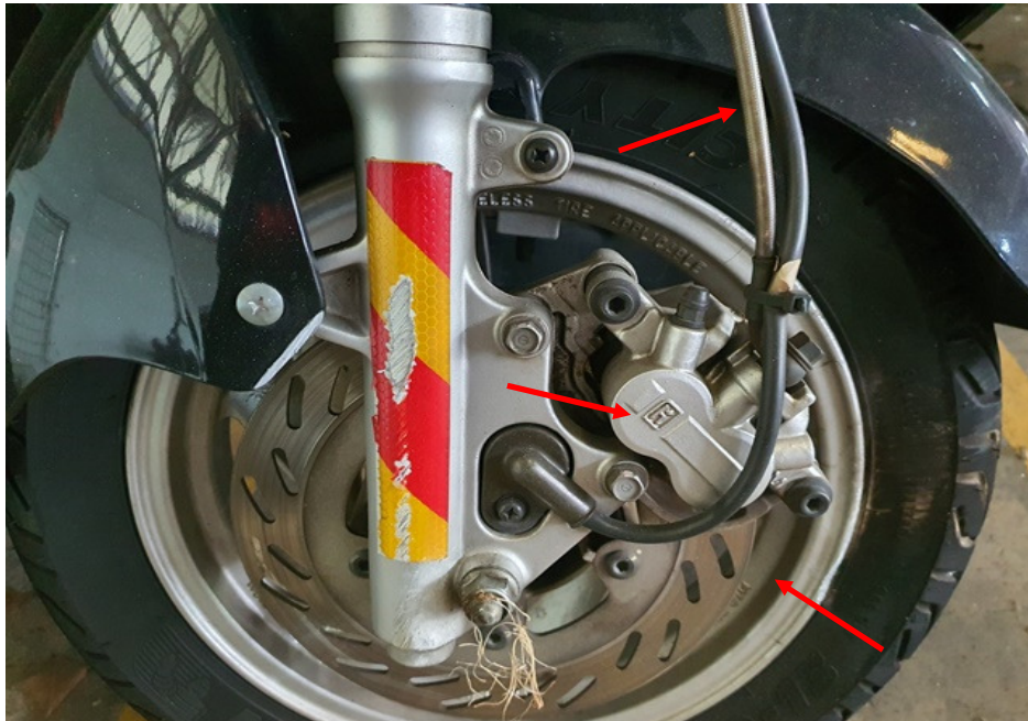
Photo 26 shows a close up view of the front brake caliper, front brake disc and front brake hose (arrowed) of the Motorcycle, which are all part of the components in the hydraulic front brake system of the Motorcycle. Our visual checks of these various components had revealed all to be intact with no visible damage. No leakage of brake fluid was also observed.
