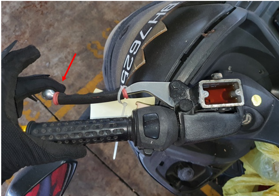
Photo 30 shows the rear brake lever being depressed. There was some resistance felt (spongy like feel) upon pressing the front brake lever (arrowed). This would indicate that there is no leakage of pressure/vacuum in the brake system.
