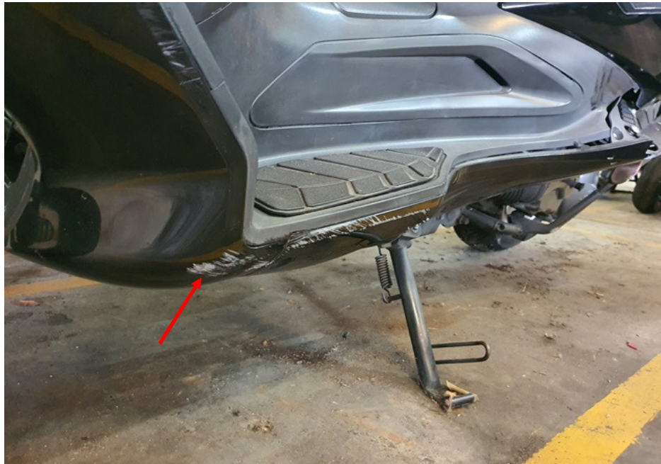
Photo 13 shows a close-up view of the grazed left lower side cowling of the Motorcycle as a result of the accident (arrowed).
