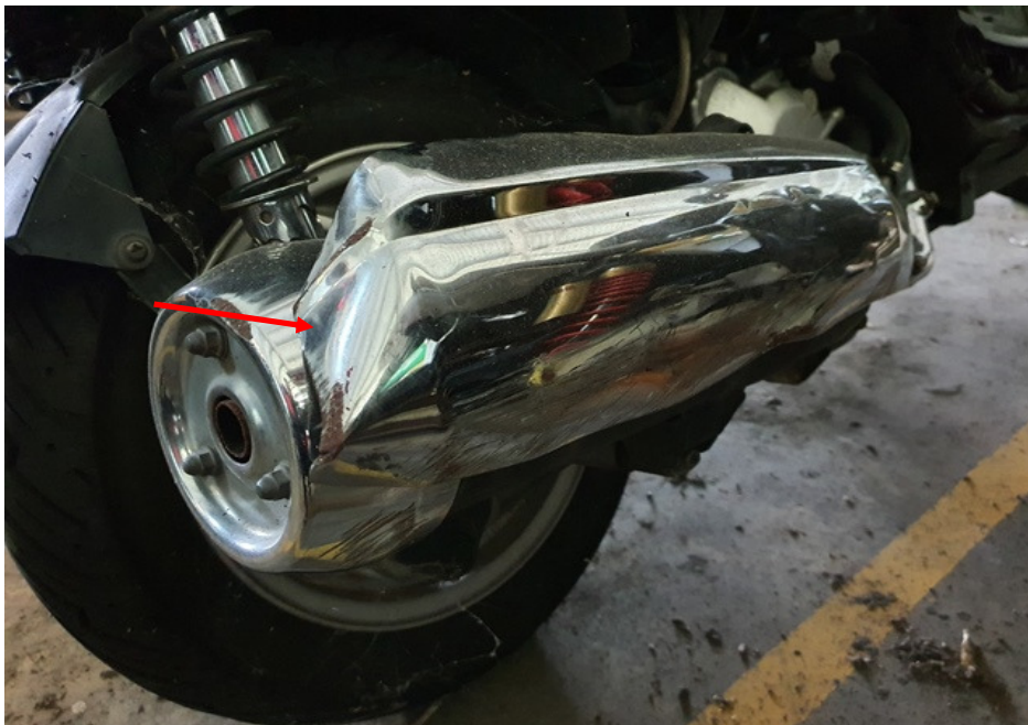
Photo 18 shows a close-up view of the dented exhaust muffler heat shield of the Motorcycle as a result of the accident (arrowed).
