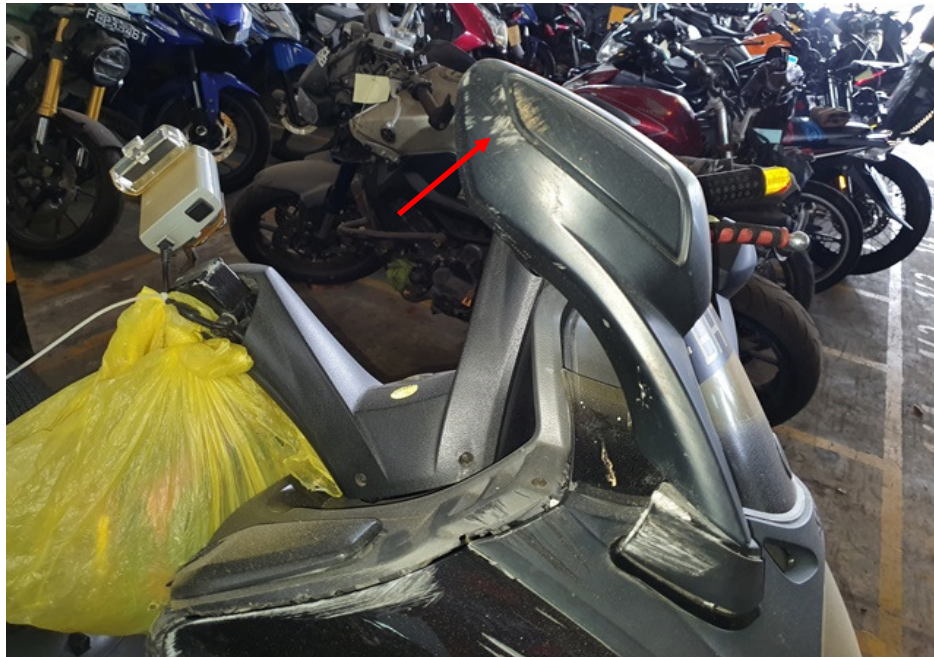
Photo 9 shows a closer view of the right side mirror of the Motorcycle which was observed to be damaged due to the accident (arrowed).
