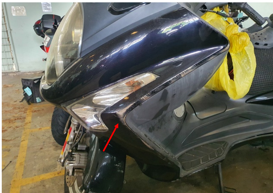
Photo 10 shows the grazed left side cowling of the Motorcycle as a result of the accident (arrowed).
