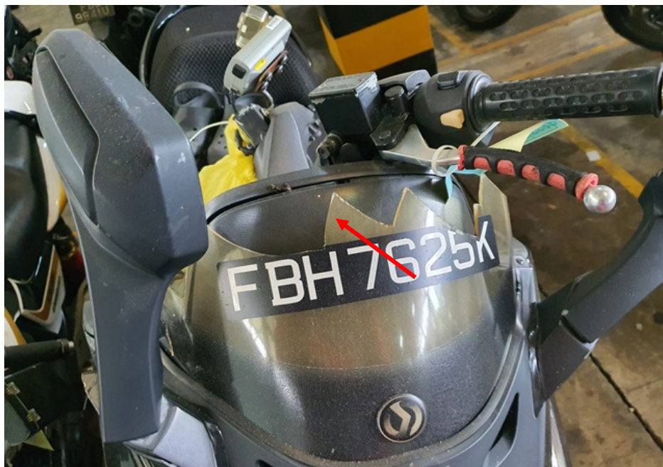
Photo 5 shows a closer view of the cracked windshield of the Motorcycle at the time of our inspection (arrowed).
