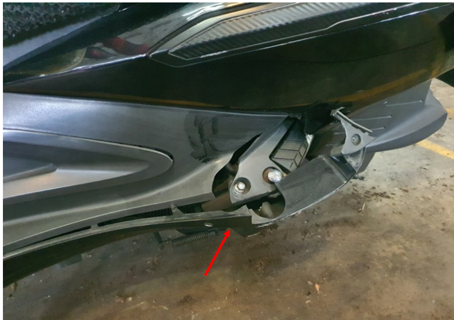
Photo 14 shows a general view of the cracked left pillion step panel of the Motorcycle as a result of the accident (arrowed).
