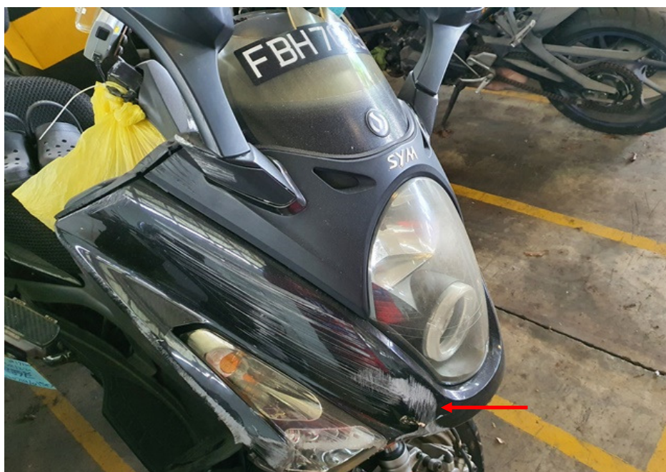
Photo 6 shows a closer view of the grazed head cowl of the Motorcycle as a result of the accident (arrowed).
