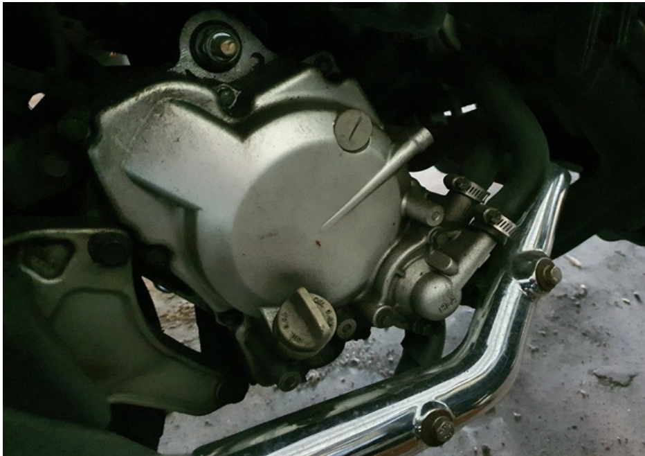
Photo 21 shows the right side of the engine of the Motorcycle at the time of our inspection. The various engine related parts and components were found to be intact with no visible damage. There was also no sign(s) or indication(s) of fluid leak observed around the right engine area of the Motorcycle.
