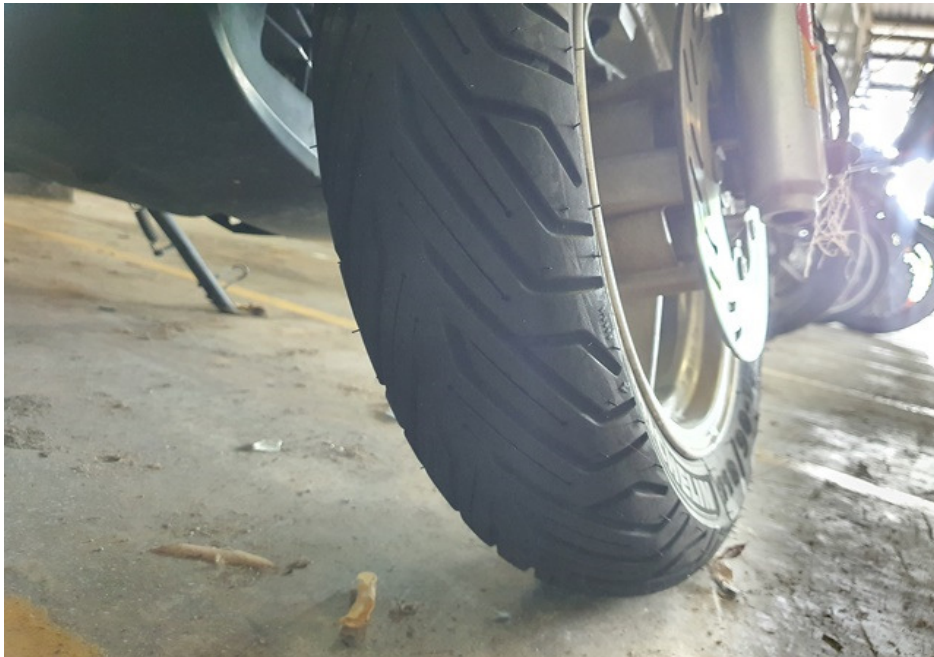
Photo 19 shows the condition of the Motorcycle's front tyre. The front tyre was observed to be in serviceable condition with remaining tread depth of approximately 4mm. There was no tear, burst mark(s) and/or punctured hole(s) on the sidewalls as well as across the tread of the front tyre.
