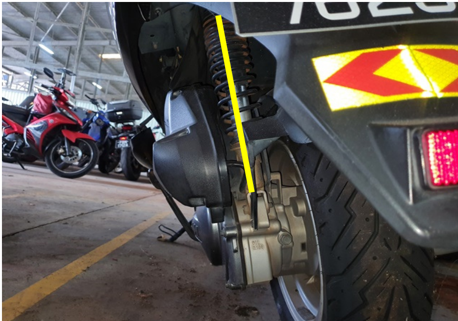
Photo 23 shows the left shock absorber of the Motorcycle which was found to be intact without any misalignment.
