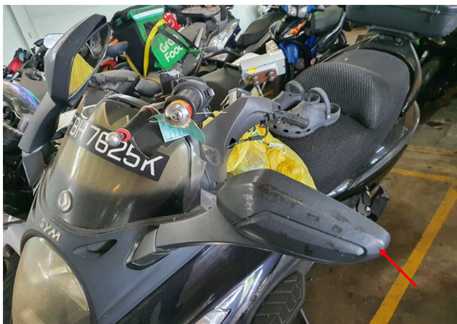
Photo 8 shows a closer view of the left side mirror of the Motorcycle which was observed to be damaged due to the accident (arrowed).
