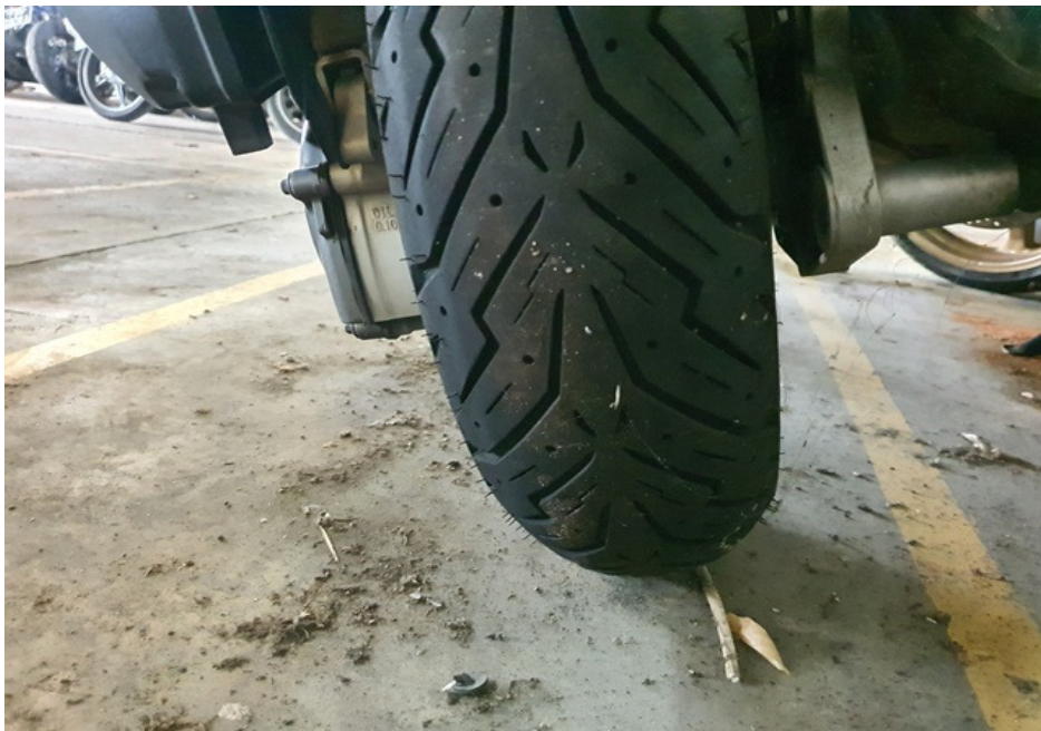
Photo 20 shows the condition of the Motorcycle's rear tyre. The rear tyre was observed to be in serviceable condition with remaining tread depth of approximately 4mm. The tyre was also observed to be sufficiently inflated for vehicular operation. We did not observe any tear, burst mark(s) and/or punctured hole(s) on the sidewalls as well as across the tread of the rear tyre.
