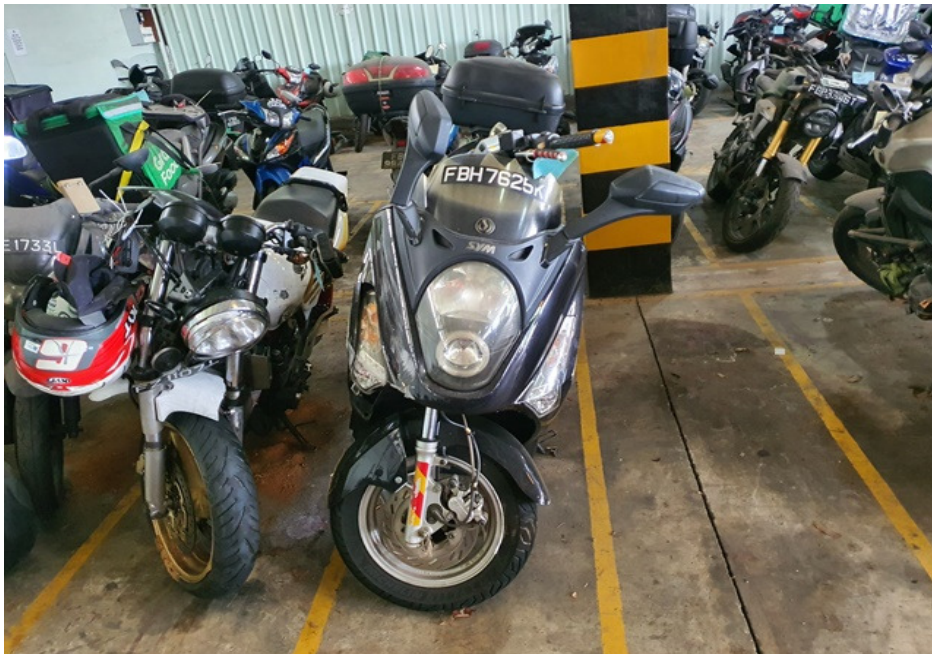
Photo 4 shows a general view of the frontal portion of the Motorcycle at the time of our inspection. The Motorcycle was observed to have sustained damages all around. The body parts that were found to have been damaged include its windshield, head cowl, front mudguard, fork assembly, side mirrors, side cowlings, lower side cowlings, left pillion step panel, rear side covers, top box and exhaust muffler heat shield, amongst others as a result of the accident.
