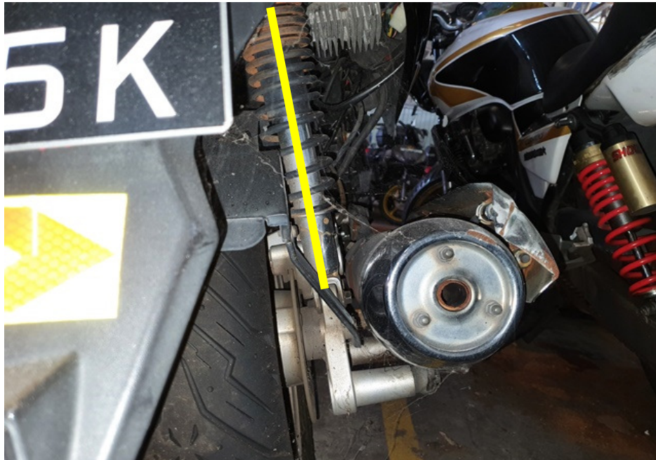
Photo 24 shows the right shock absorber of the Motorcycle which was found to be intact without any misalignment.
