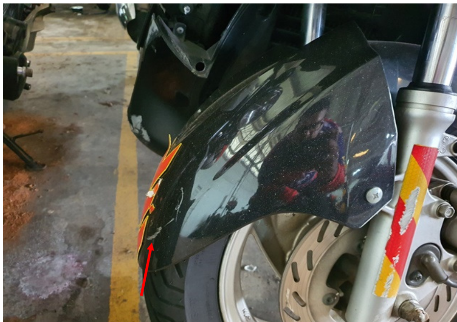
Photo 7 shows a closer view of the grazed front mudguard of the Motorcycle as a result of the accident (arrowed).
