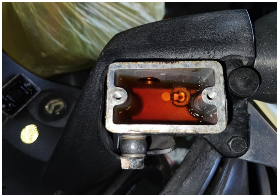
Photo 27 shows the brake fluid reservoir for the front brake of the Motorcycle. The brake fluid was observed to be of sufficient level for operational purposes and without contamination.
