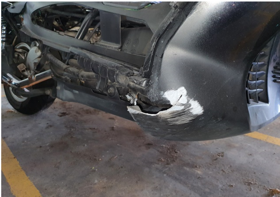
Photo 12 shows a close-up view of the cracked right lower side cowling of the Motorcycle as a result of the accident.
