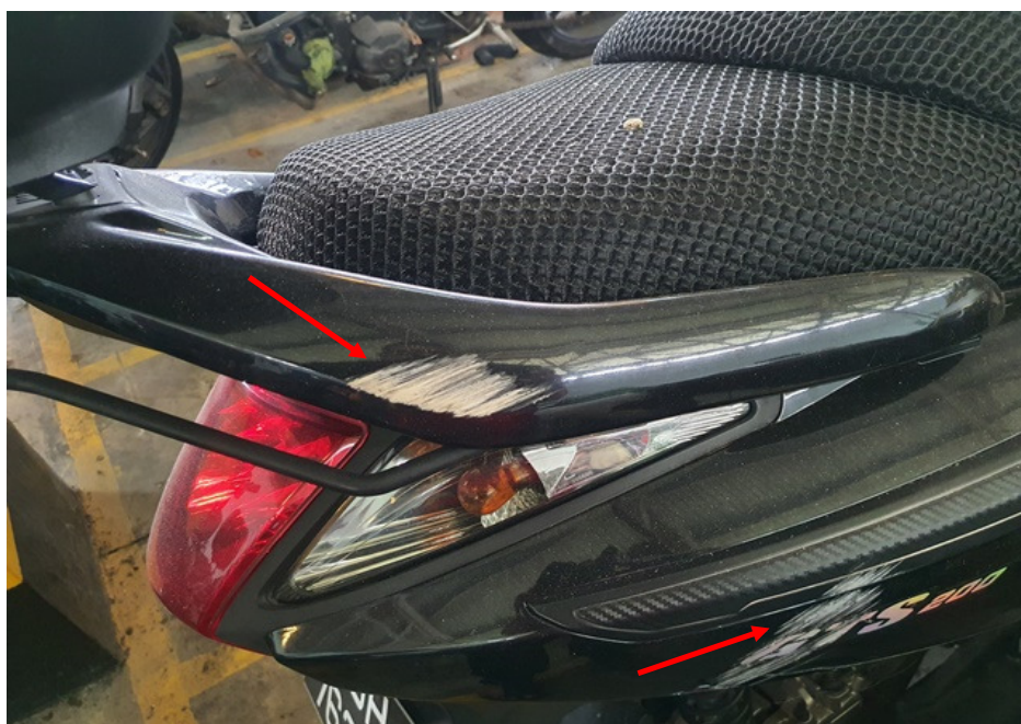
Photo 16 shows a close-up view of the grazed right rear side cover and right pillion grab rail of the Motorcycle as a result of the accident (arrowed).
