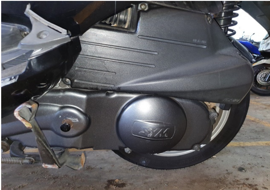
Photo 22 shows the drive train cover of the Motorcycle which was found to be intact without any misalignment.
