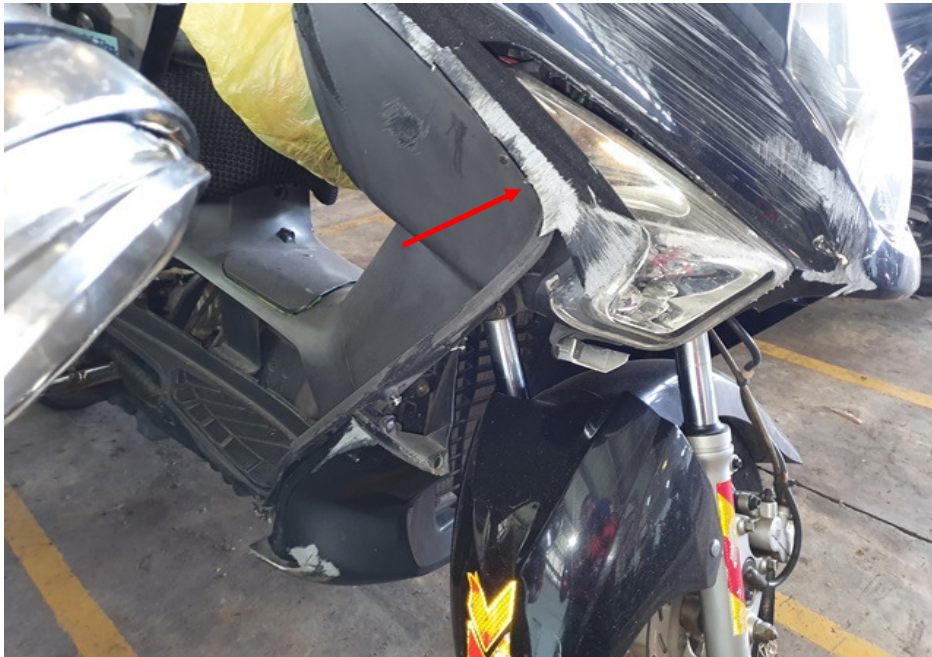
Photo 11 shows the grazed right side cowling of the Motorcycle as a result of the accident (arrowed).
