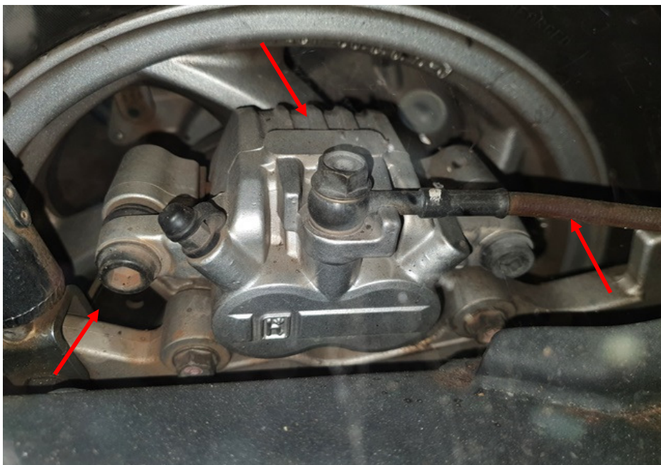
Photo 31 shows a close up view of the rear brake caliper, rear brake disc and rear brake hose (arrowed) of the Motorcycle, which are all part of the components in the hydraulic rear brake system of the Motorcycle. Our visual checks of these various components revealed all to be intact with no visible damage. No leakage of brake fluid was also observed.
