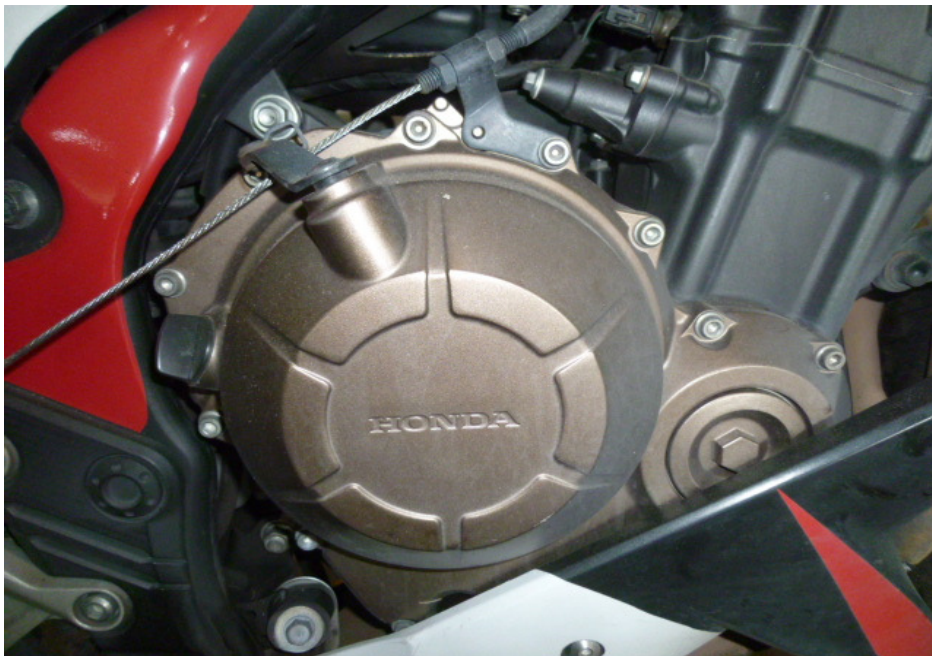
Photo 19 shows the right side of the engine of the Motorcycle at the time of our inspection. The various engine related parts and components were found to be intact with no visible damage. There was also no sign(s) or indication(s) of fluid leak observed around the right engine area of the Motorcycle.
