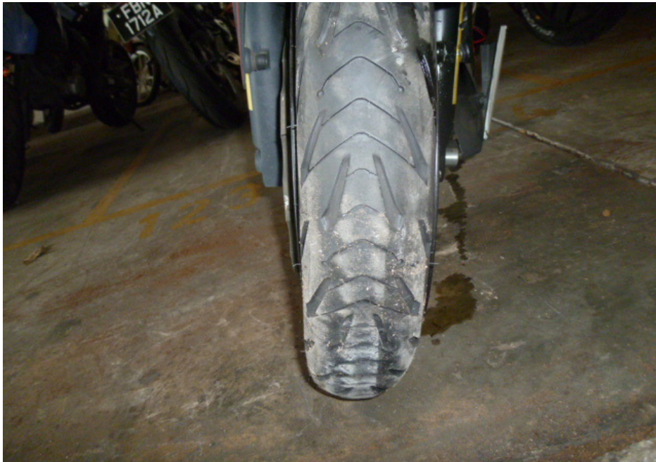
Photo 15 shows the condition of the Motorcycle's front tyre. The front tyre was observed to be in serviceable condition with remaining tread depth of approximately 3mm. There was no tear, burst mark(s) and/or punctured hole(s) on the sidewalls as well as across the tread of the front tyre. However the front tyre was observed to be deflated.
