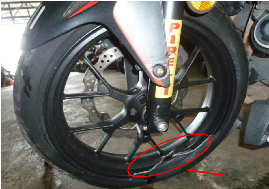
Photo 16 shows the broken front wheel rim (circled) and deflated front tyre (arrowed) of the Motorcycle at the time of our inspection.
