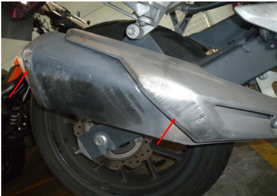
Photo 12 shows a closer view of the grazed exhaust muffler heat shield and exhaust muffler (arrowed) of the Motorcycle as a result of the accident.
