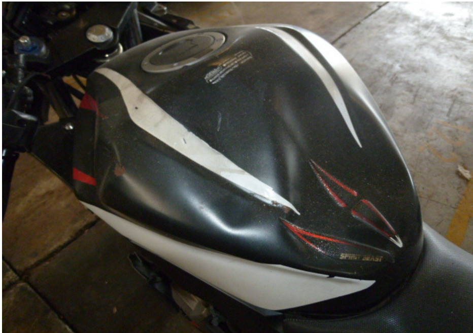
Photo 11 shows a closer view of the dented petrol tank of the Motorcycle as a result of the accident.
