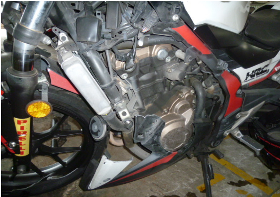
Photo 9 shows a closer view of the missing left cowling of the Motorcycle as a result of the accident.
