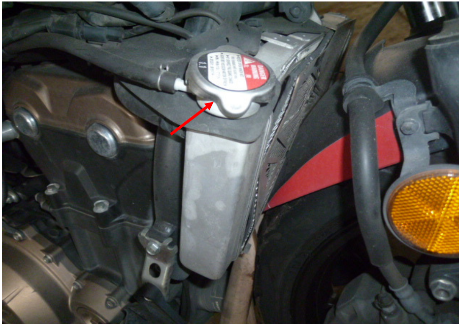
Photo 7 shows a closer view of the deformed radiator (arrowed) of the Motorcycle as a result of the accident.
