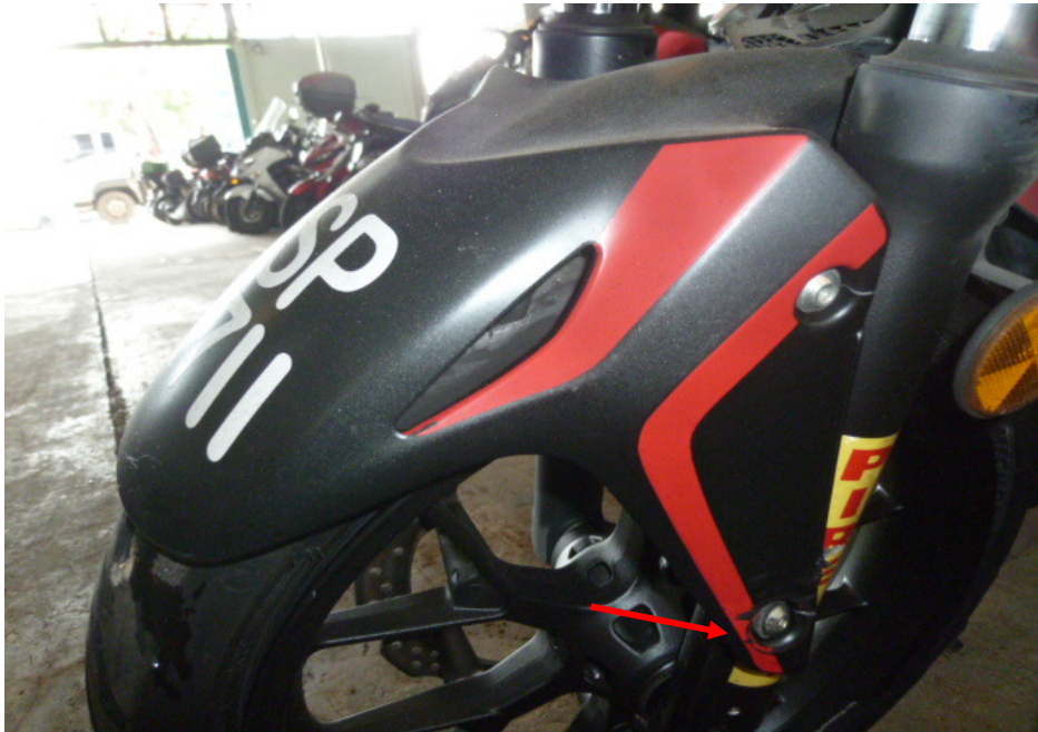
Photo 5 shows a closer view of the front mudguard (arrowed) which was amongst the body parts of the Motorcycle that had sustained damage as a result of the accident.
