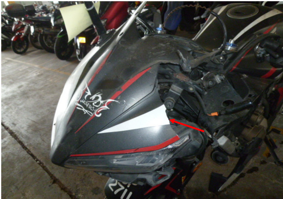
Photo 6 shows the cracked head cowl (arrowed) of the Motorcycle as a result of the accident.
