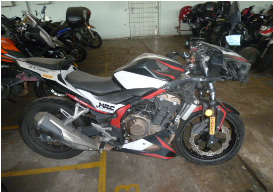
Photo 4 shows a general view of the right body of the Motorcycle at the time of our inspection. The Motorcycle was observed to have sustained damages all around. The body parts that were found to have been damaged include its speedometer gauge, head cowl, front mudguard, side cowlings, right handlebar end, right side mirror, front brake lever, petrol tank, radiator, rear brake pedal, right front footrest, right rear side cover, exhaust muffler heat shield and exhaust muffler, amongst others.
