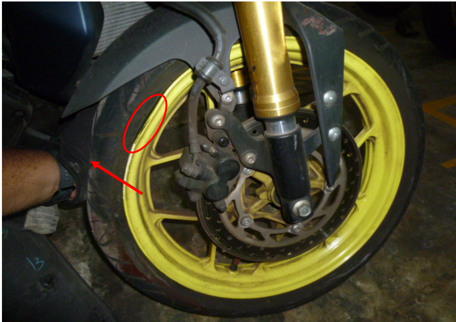
Photo 21 shows the bent front wheel rim (circled) and deflated front tyre (arrowed) of the Motorcycle at the time of our inspection.
