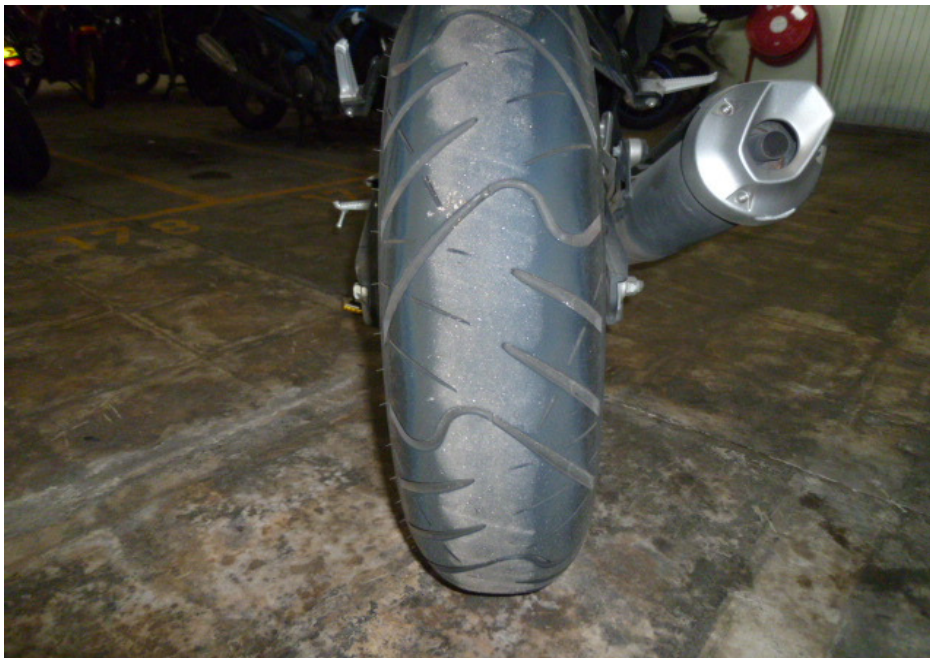
Photo 22 shows the condition of the Motorcycle's rear tyre. The rear tyre was observed to be in serviceable condition with remaining tread depth of approximately 4mm. The tyre was also observed to be sufficiently inflated for vehicular operation. We did not observe any tear, burst mark(s) and/or punctured hole(s) on the sidewalls as well as across the tread of the rear tyre.
