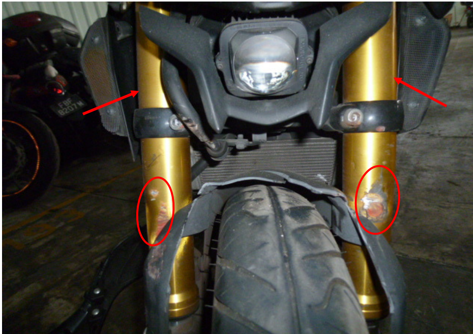
Photo 27 shows the front forks (arrowed) of the Motorcycle. The front forks and fork bracket of the Motorcycle were both found to be intact. However the front forks had sustained damages of grazing nature as a result of the accident (circled). Turning the Motorcycle's handle bar towards the left and right did not produce any abnormal free play. The steering system of the Motorcycle was in serviceable condition at the time of our inspection.
