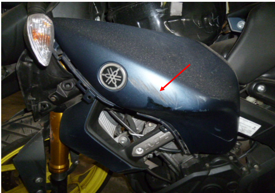
Photo 14 shows a closer view of the grazed left cowling of the Motorcycle as a result of the accident (arrowed).
