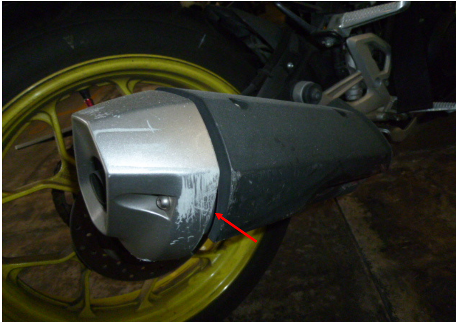
Photo 19 shows the grazed exhaust muffler heat shield of the Motorcycle as a result of the accident (arrowed).
