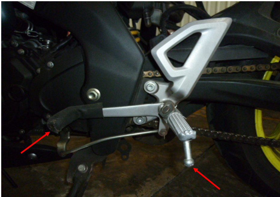
Photo 18 shows the gear shift pedal and left front footrest of the Motorcycle that had sustained damage as a result of the accident (arrowed).
