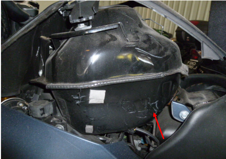
Photo 13 shows a closer view of the dented petrol tank of the Motorcycle as a result of the accident (arrowed).
