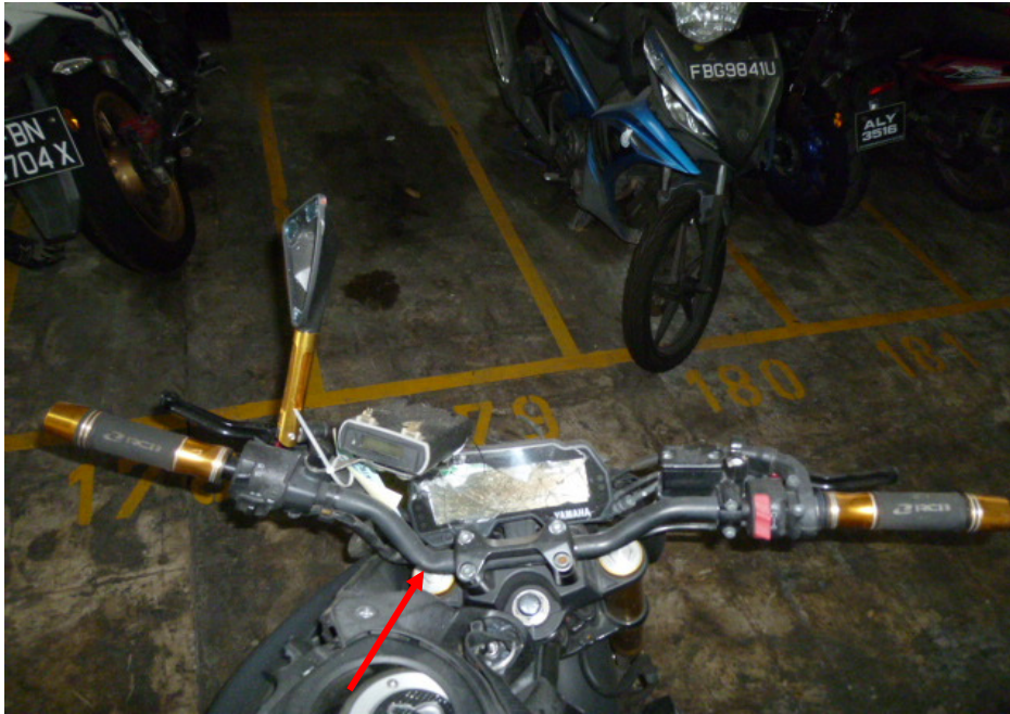
Photo 9 shows a closer view of the bent handlebar of the Motorcycle as a result of the accident (arrowed).
