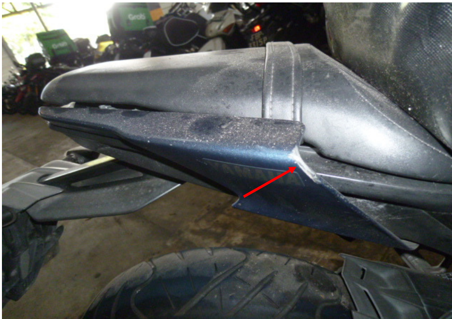
Photo 16 shows a closer view of the grazed right rear side cover of the Motorcycle as a result of the accident (arrowed).
