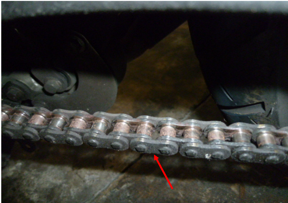
Photo 26 shows a closer view of the gear chain (arrowed) of the Motorcycle, which was observed to be intact with no misalignment. It was also adequately lubricated for operating purposes.
