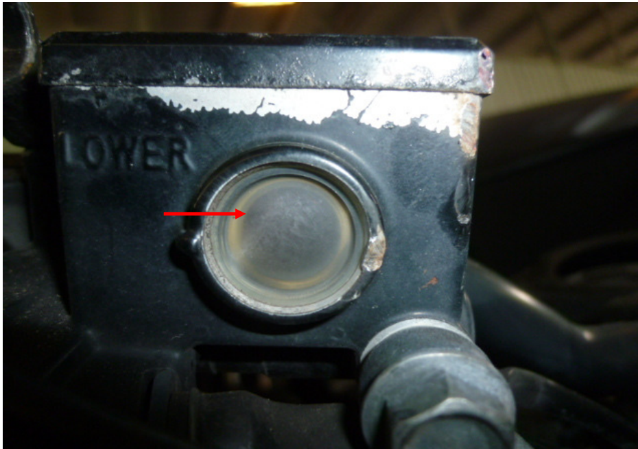
Photo 32 shows a close up view of the brake fluid reservoir for the front brake of the Motorcycle. The brake fluid was observed to be of sufficient level for operational purposes (arrowed).
