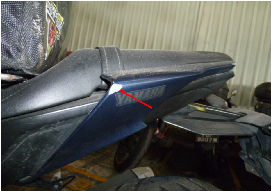
Photo 15 shows a closer view of the grazed left rear side cover of the Motorcycle as a result of the accident (arrowed).
