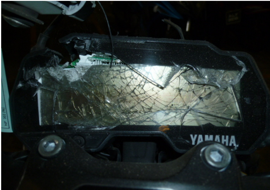
Photo 1 shows the damaged speedometer gauge of the Motorcycle as a result of the accident. Hence the mileage of the Motorcycle could not be recorded at the time of our inspection.
