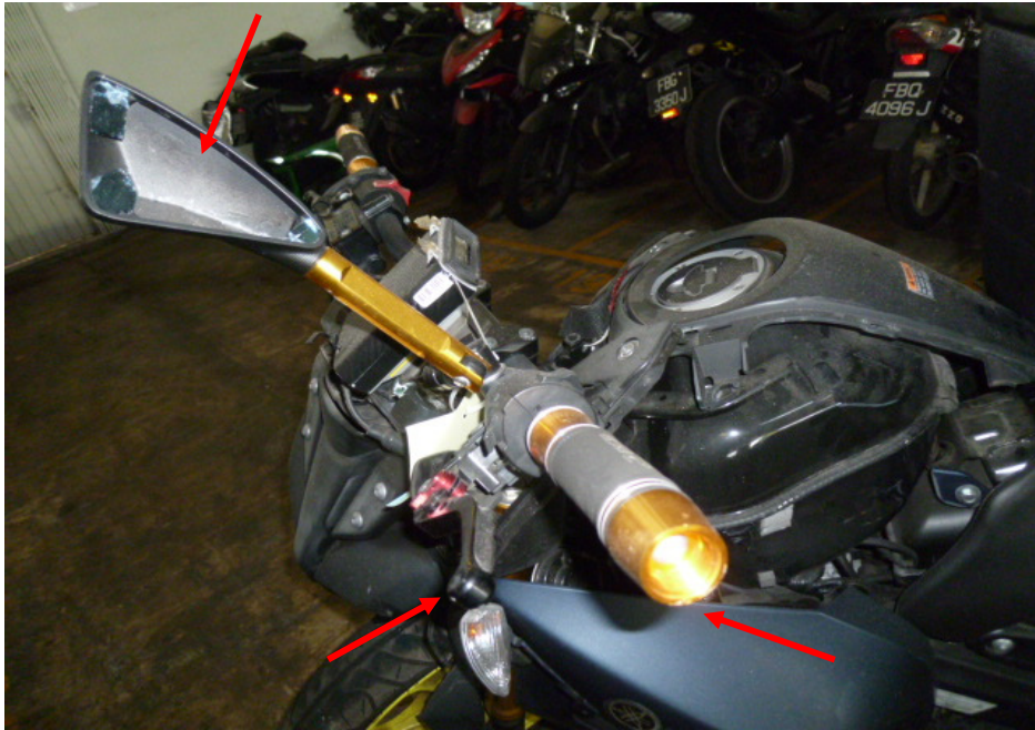
Photo 11 shows the left handlebar end, clutch brake lever and left side mirror (arrowed), which were amongst the body parts of the Motorcycle that had sustained damage as a result of the accident.
