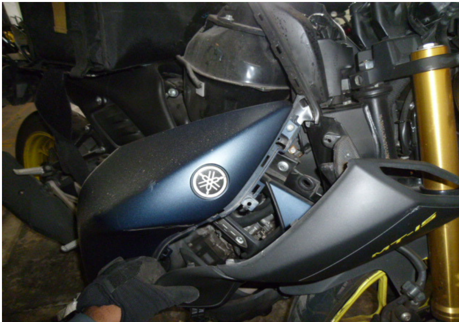
Photo 8 shows a closer view of the cracked right cowling which was amongst the body parts of the Motorcycle that had sustained damage as a result of the accident.
