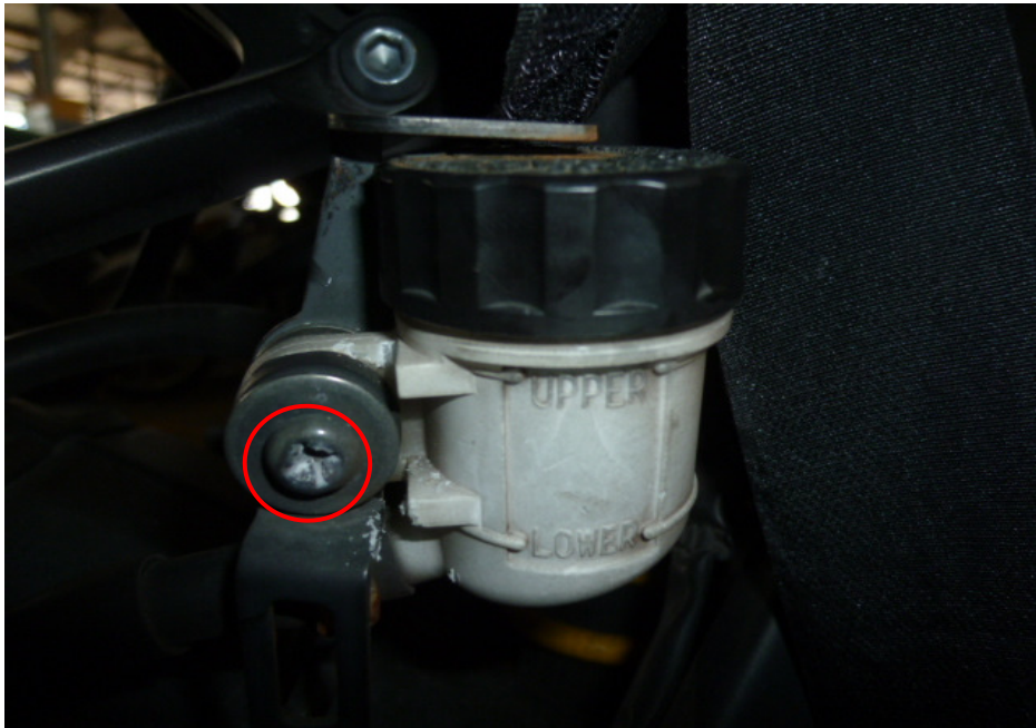
Photo 35 shows the brake fluid reservoir cover for the rear brake of the Motorcycle. We were unable to examine whether the front brake fluid was of sufficient level for operational purposes and without contamination due to the worn out screw (circled).
