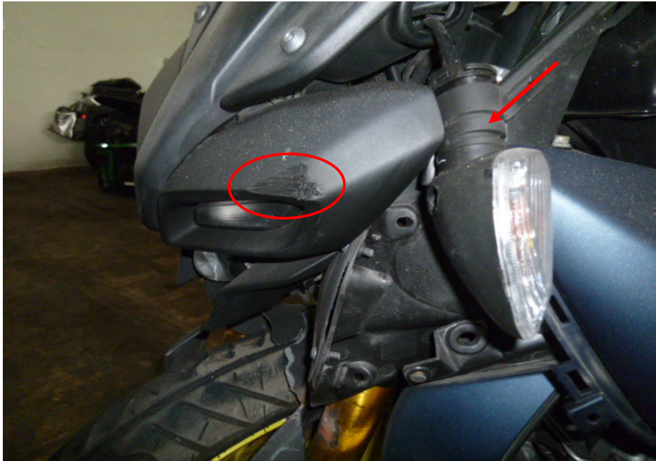
Photo 7 shows the grazed front cowling (circled) and broken left front signal lamp (arrowed), which were amongst the body parts of the Motorcycle that had sustained damage as a result of the accident.
