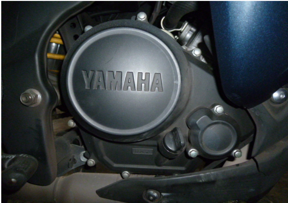
Photo 24 shows the right side of the engine of the Motorcycle at the time of our inspection. The various engine related parts and components were found to be intact with no visible damage. There was also no sign(s) or indication(s) of fluid leak observed around the right engine area of the Motorcycle.
