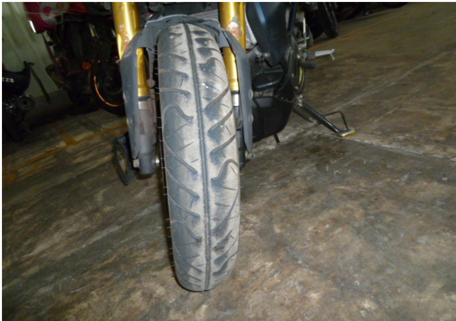
Photo 20 shows the condition of the Motorcycle's front tyre. The front tyre was observed to be in serviceable condition with remaining tread depth of approximately 3mm. There was no tear, burst mark(s) and/or punctured hole(s) on the sidewalls as well as across the tread of the front tyre. However the front tyre was observed to be deflated.
