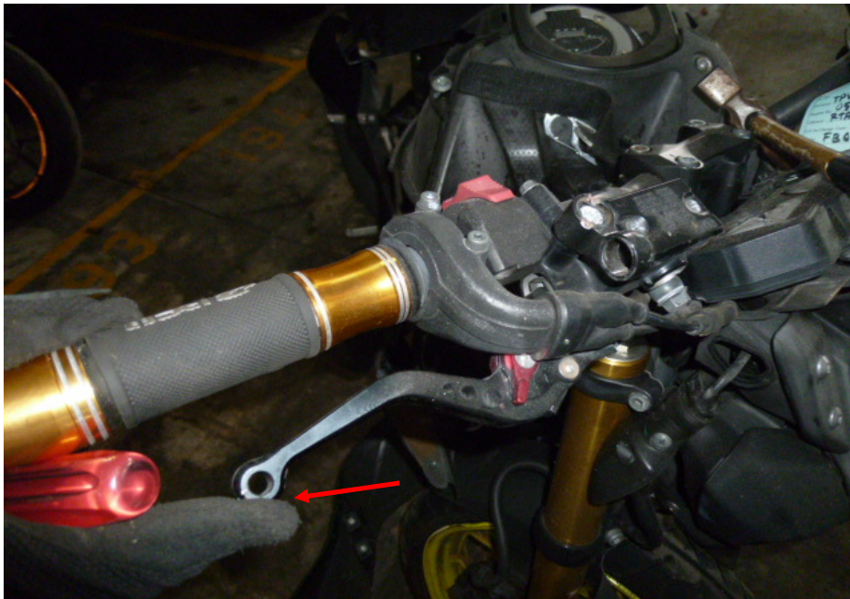
Photo 33 shows the front brake lever being depressed. There was some resistance felt (spongy like feel) upon pressing the front brake lever (arrowed). This would indicate that there is no leakage of pressure/vacuum in the front brake system.
