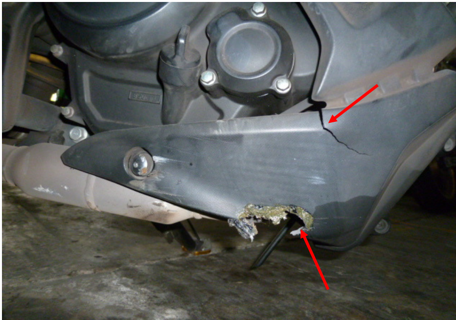
Photo 12 shows a closer view of the cracked belly pan (arrowed) which was amongst the body parts of the Motorcycle that had sustained damage as a result of the accident.
