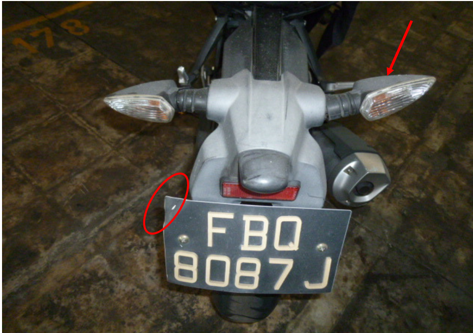
Photo 17 shows a closer view of the deformed right rear signal lamp (arrowed) and dented rear number plate (circled) of the Motorcycle as a result of the accident.
