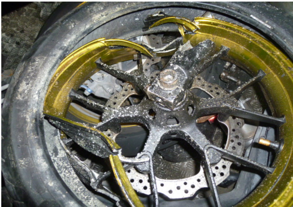
Photo 18 shows the broken front wheel rim of the Motorcycle at the time of our inspection.
