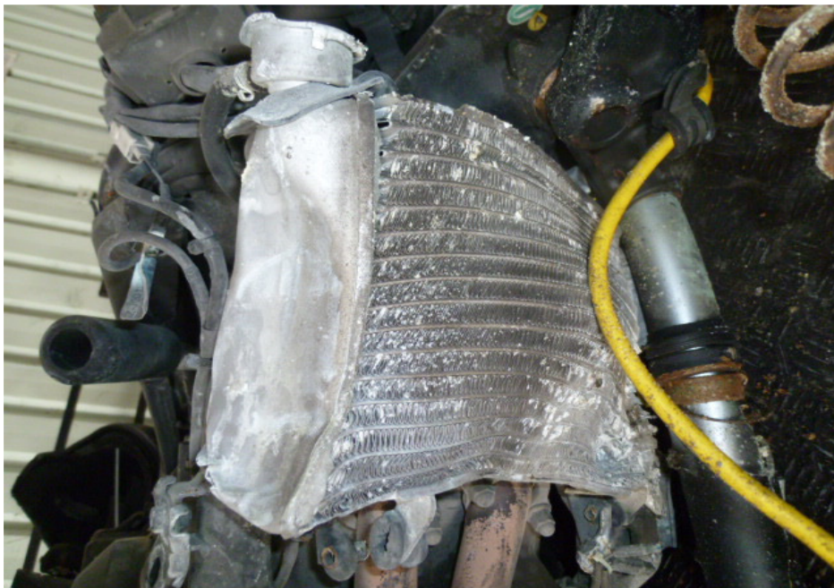
Photo 8 shows the deformed radiator of the Motorcycle as a result of the accident.
