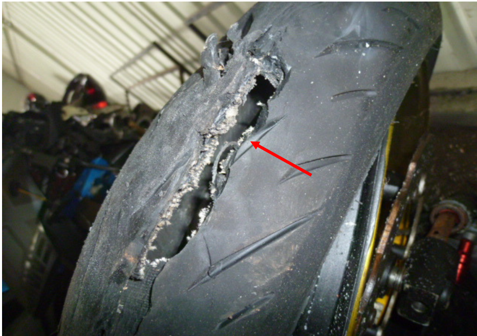
Photo 17 shows a closer view of the tear on the front tyre as a result of the accident (arrowed).
