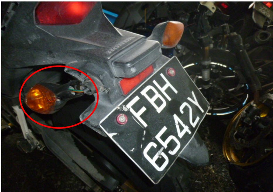
Photo 14 shows the left rear signal lamp (circled) which was amongst the body parts of the Motorcycle that had sustained damage as a result of the accident.
