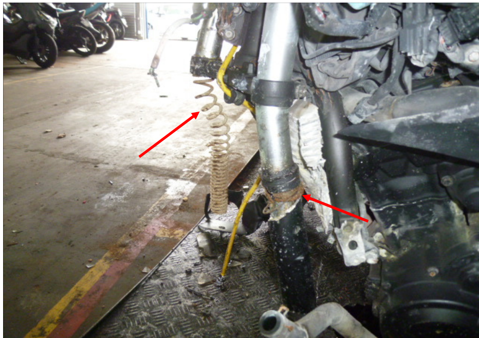
Photo 26 shows the front forks of the Motorcycle. The front forks (arrowed) were observed to be broken as a result of the accident. We were hence not able to conduct any tests on the steering system of the Motorcycle.
