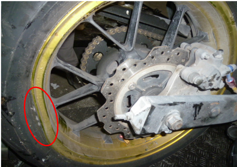
Photo 20 shows the bent rear wheel rim (circled) of the Motorcycle at the time of our inspection.
