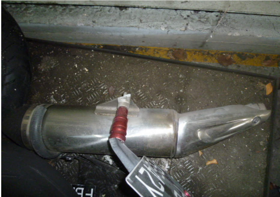
Photo 15 shows the dislodged exhaust muffler of the Motorcycle as a result of the accident.
