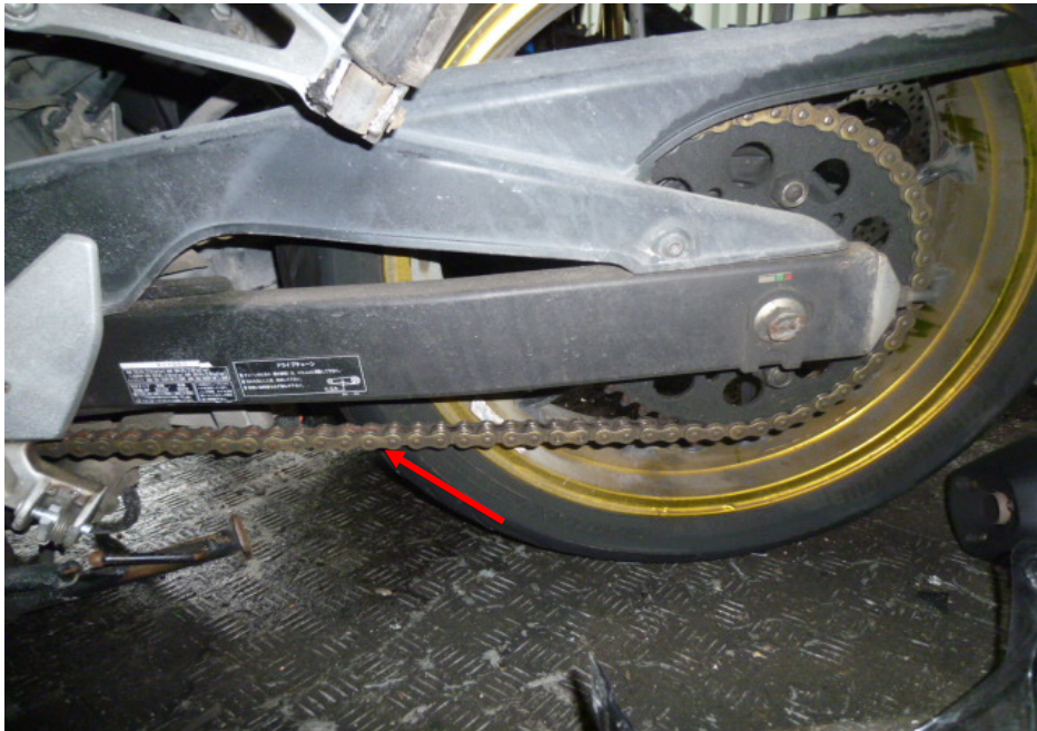
Photo 24 shows the general view of the gear train (arrowed) of the Motorcycle, which was observed to be intact with no misalignment. It was also adequately lubricated for operating purposes.
