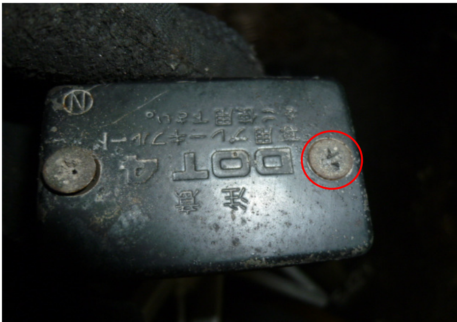
Photo 32 shows the brake fluid reservoir cover for the rear brake of the Motorcycle. We were unable to examine whether the rear brake fluid was without contamination due to the worn out screw (circled). However the rear brake fluid was observed to be of sufficient level for operational purposes.
