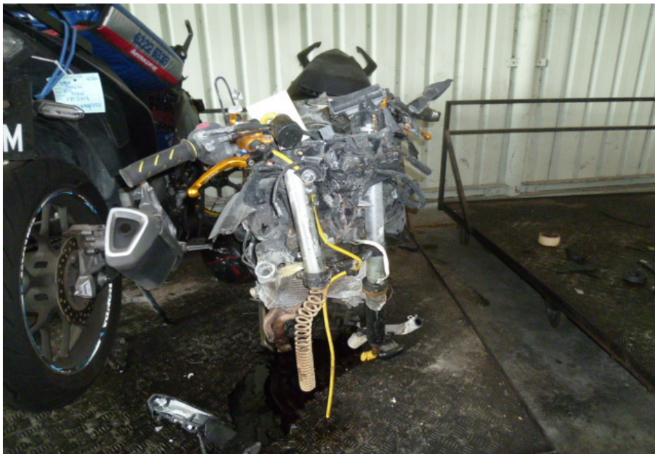
Photo 4 shows a general view of the frontal portion of the Motorcycle at the time of our inspection. The Motorcycle was observed to have sustained damages all around. The body parts that were found to have been damaged include its speedometer gauge, headlight assembly, side cowlings, handlebar, side mirrors, clutch lever, front brake lever, handlebar ends, radiator, exhaust headers, petrol tank, gear shift pedal, left front footrest, left rear side cover, left pillion grab rail and exhaust muffler, amongst others.
