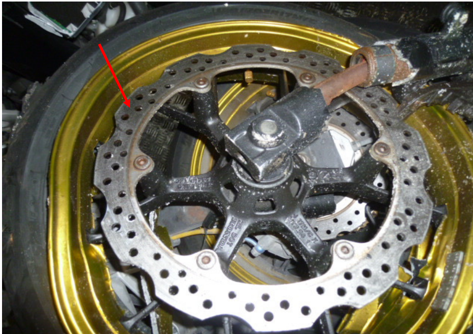
Photo 27 shows a close up view of the front brake caliper, front brake disc and front brake hose of the Motorcycle's front wheel, which are all part of the components in the hydraulic front brake system of the Motorcycle. The front brake caliper and front brake hose were observed to be missing upon our inspection. Our visual checks of the front brake disc (arrowed) had revealed it to be intact with no visible damage. No leakage of brake fluid was also observed.
