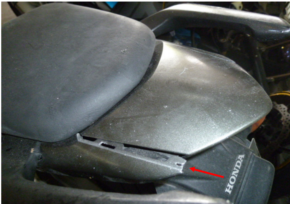
Photo 12 shows a closer view of the left rear side cover (arrowed) which was amongst the body parts of the Motorcycle that had sustained damage as a result of the accident.
