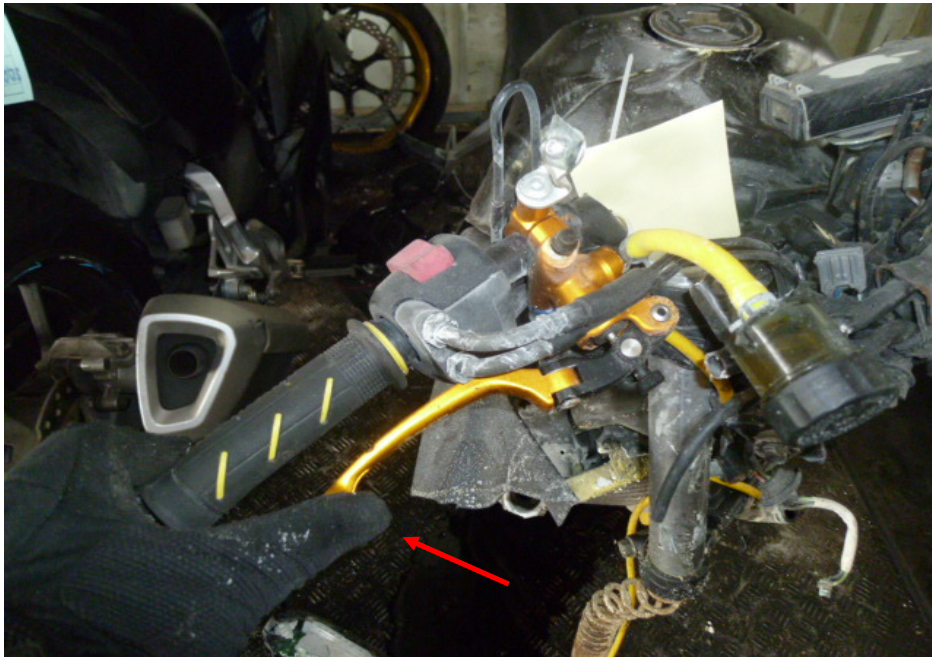
Photo 29 shows the front brake lever being depressed. There was no resistance felt (spongy like feel) upon pressing the front brake lever (arrowed). This would indicate that there is leakage of pressure/vacuum in the front brake system. Upon closer examination, we observed that the front brake hose of the Motorcycle was cut.
