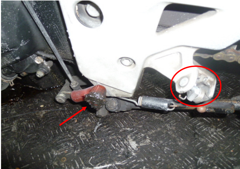
Photo 11 shows a closer view of the gear shift pedal (arrowed) and left front footrest (circled) which was amongst the body parts of the Motorcycle that had sustained damage as a result of the accident.
