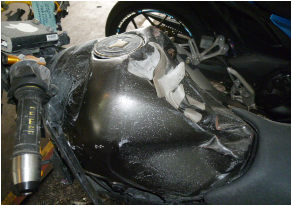
Photo 10 shows a closer view of the petrol tank, which was amongst the body parts of the Motorcycle that had sustained damage as a result of the accident.
