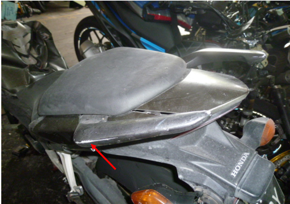
Photo 13 shows the left pillion grab rail (arrowed) which was amongst the body parts of the Motorcycle that had sustained damage as a result of the accident.
