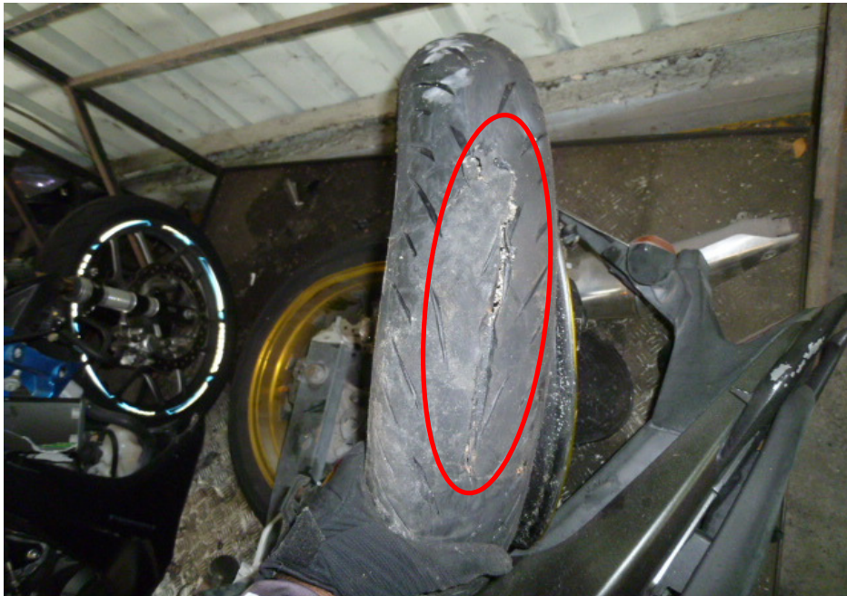
Photo 16 shows the condition of the Motorcycle's front tyre. The front tyre was observed to be in serviceable condition with remaining tread depth of approximately 4mm. However the tyre was observed to be deflated. We also observed a tear on the front tyre as a result of the accident (circled).
