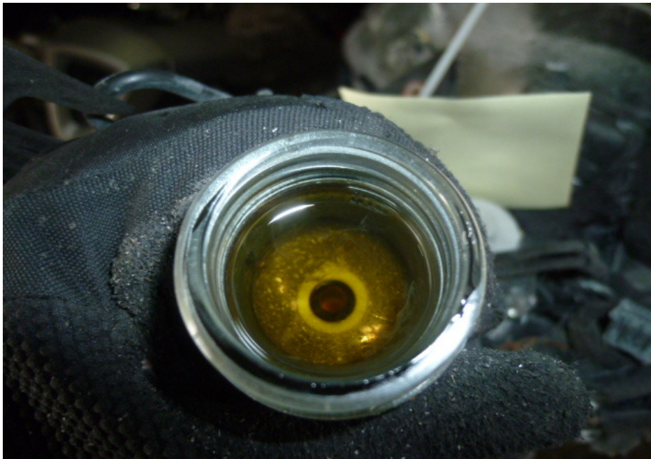
Photo 28 shows the brake fluid reservoir for the front brake of the Motorcycle. The brake fluid was observed to be of sufficient level for operational purposes and without contamination.
