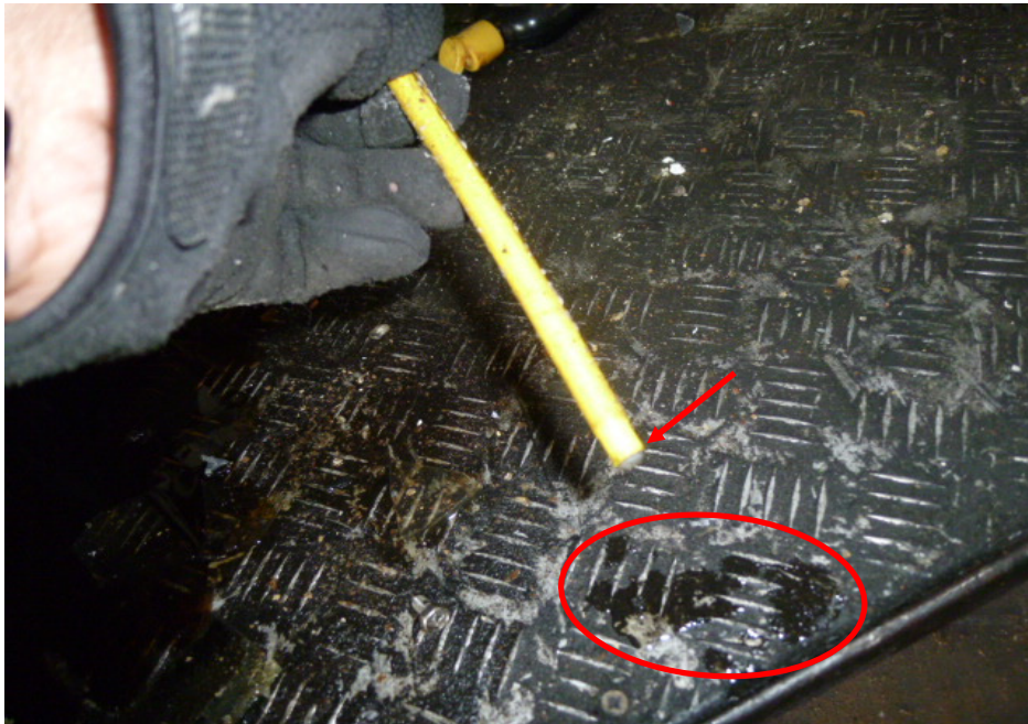
Photo 30 shows the front brake hose for the front brake of the Motorcycle. The front brake hose was observed to be cut as a result of the accident (arrowed). Brake fluid was also found to be leaking from the cut front brake hose (circled).
