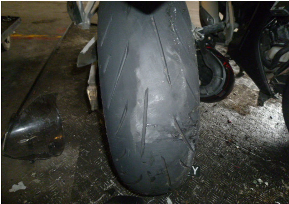
Photo 19 shows the condition of the Motorcycle's rear tyre. The rear tyre was observed to be in serviceable condition with remaining tread depth of approximately 4mm. The tyre was also observed to be sufficiently inflated for vehicular operation. We did not observe any tear, burst mark(s) and/or punctured hole(s) on the sidewalls as well as across the tread of the rear tyre.
